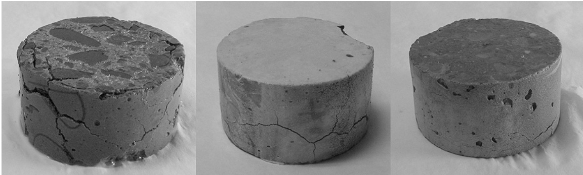
Figure 35. Photographs of 4 inch (100 mm) diameter 0.45 w/c OPC concrete specimens after 500 days in high concentration brines. From left to right: CaCl 2 , MgCl 2 , and MBAP brines.
