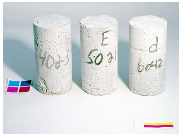
Figure 16. Cylinders exposed to CMA solution after 84 days of constant low temperature test. From left to right: 0.40, 0.50, and 0.60 w/c mortar cylinders.
