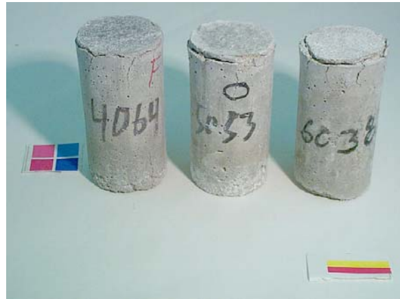
Figure 14. Cylinders exposed to MgCl 2 solution after 84 days of constant low temperature test. From left to right: 0.40, 0.50, and 0.60 w/c mortar cylinders.
