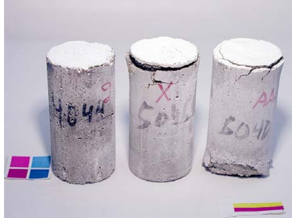
Figure 28. Cylinders exposed to \text{CaCl}_2 solution after 56 days of constant low temperature test. From left to right: 0.40, 0.50, and 0.60 w/c mortar cylinders. Solution strength was 17% \text{CaCl}_2 .
