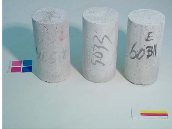
Figure 17. Control cylinders exposed to lime water solution after 84 days of constant low temperature test. From left to right: 0.40, 0.50, and 0.60 w/c mortar cylinders.
