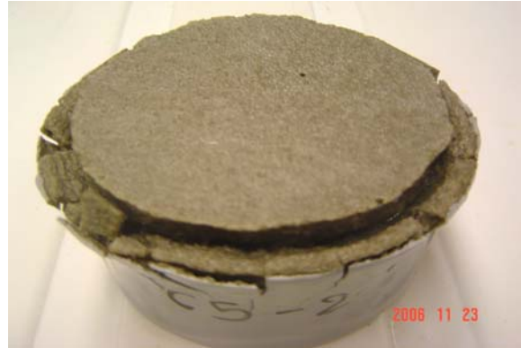
Figure 34. Deteriorated disc sample exposed to 28% CaCl 2 after 150d of exposure.
