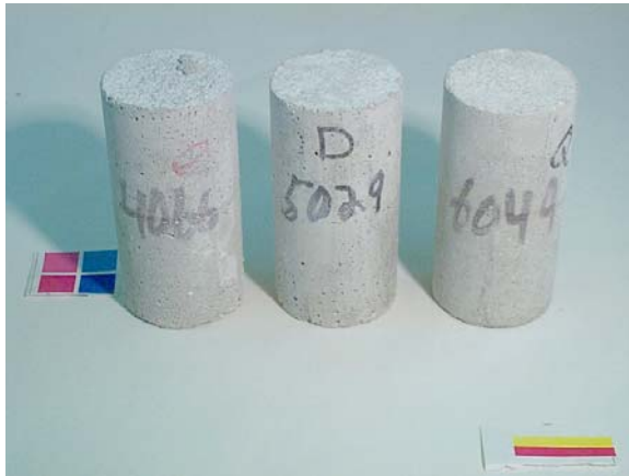
Figure 13. Cylinders exposed to NaCl solution after 84 days of constant low temperature test. From left to right: 0.40, 0.50, and 0.60 w/c mortar cylinders.
