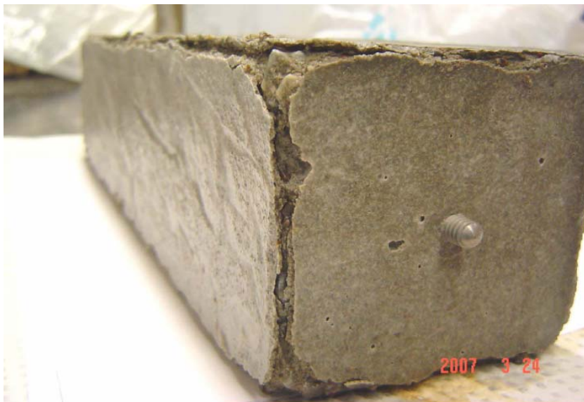
Figure 49. Photographs of concrete prisms subjected to 133 freezing and thawing cycles in 15% CaCl 2 solution.
