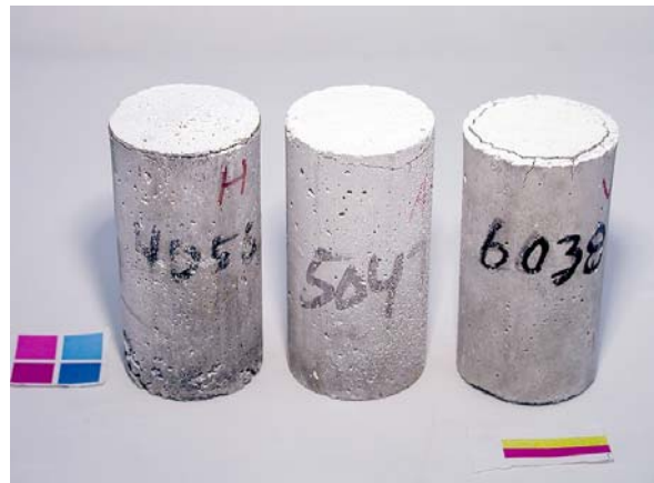
Figure 27. Cylinders exposed to \text{CaCl}_2 solution after 56 days of constant low temperature test. From left to right: 0.40, 0.50, and 0.60 w/c mortar cylinders. Solution strength was 14% \text{CaCl}_2 .
