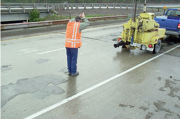
Figure 7. Photographs of core site (left) and from beneath bridge deck (right) after coring operation. Hole from core T-2 is visible. Dampness permeating through cracks visible beneath the area of core T-1. White efflorescence common directly below regions covered with cold patch material.
