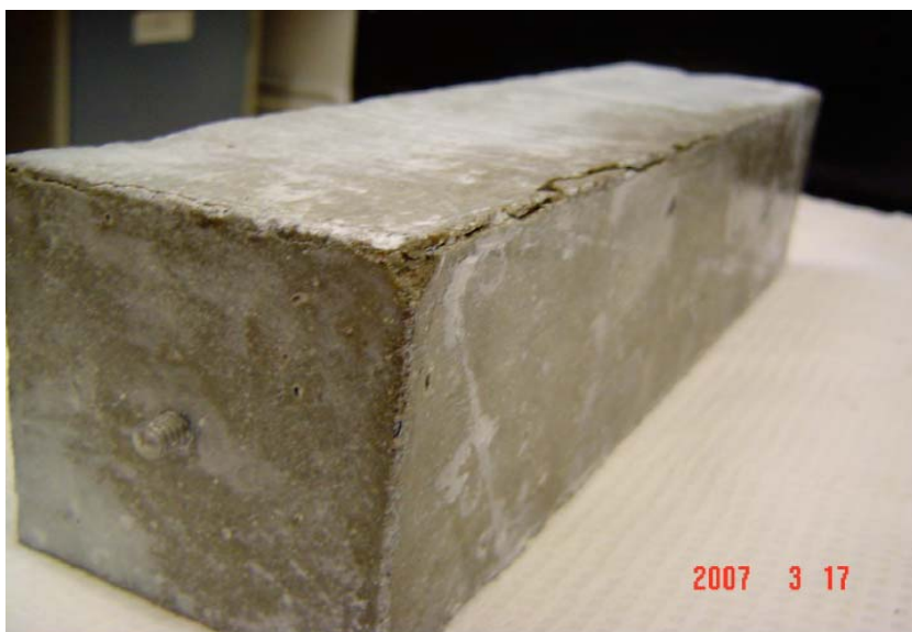
Figure 50. Photographs of concrete prisms subjected to 133 freezing and thawing cycles in 14% MgCl 2 solution.
