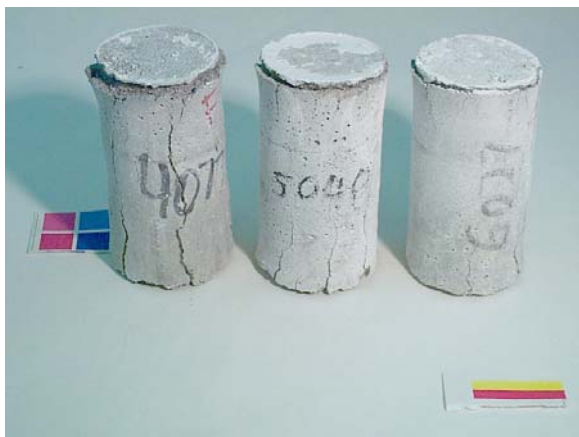
Figure 15. Cylinders exposed to CaCl 2 solution after 84 days of constant low temperature test. From left to right: 0.40, 0.50, and 0.60 w/c mortar cylinders.
