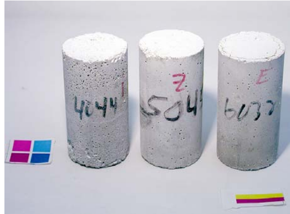
Figure 25. Cylinders exposed to \text{CaCl}_2 solution after 56 days of constant low temperature test. From left to right: 0.40, 0.50, and 0.60 w/c mortar cylinders. Solution strength was 7% \text{CaCl}_2 .
