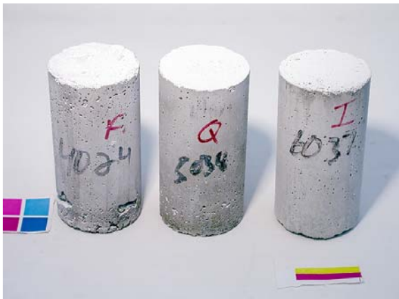
Figure 26. Cylinders exposed to \text{CaCl}_2 solution after 56 days of constant low temperature test. From left to right: 0.40, 0.50, and 0.60 w/c mortar cylinders. Solution strength was 10% \text{CaCl}_2 .
