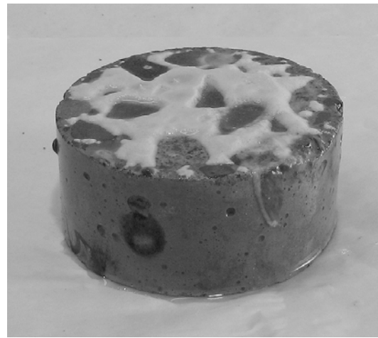
Figure 37. White precipitate on exterior of 4 inch (100 mm) diameter concrete specimen after 500 days immersion in low-concentration CMA solution.
