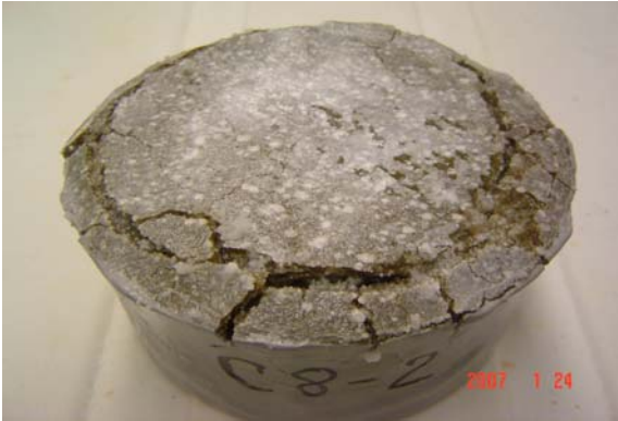
Figure 33. Deteriorated disc sample exposed to 20% MgCl 2 after 150d of exposure.
