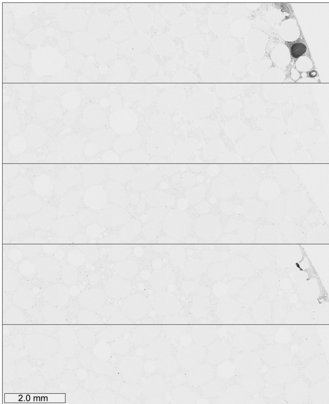
Figure 21. Elemental map for magnesium collected from thin sections prepared from mortar cylinders immersed in chemical solutions. From top to bottom: magnesium chloride, calcium chloride, sodium chloride, calcium magnesium acetate, and lime water. Dark areas indicate higher concentrations.
