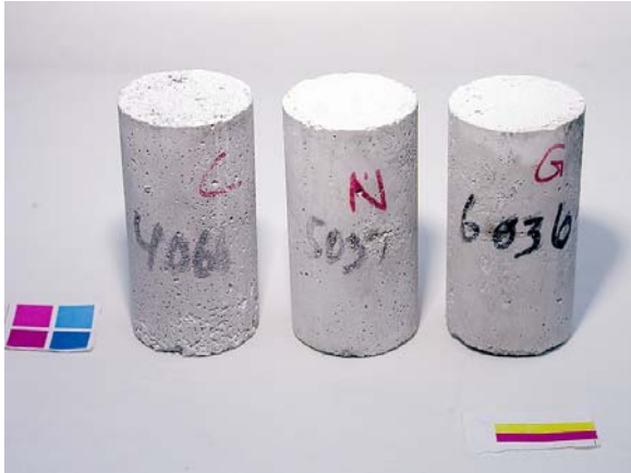
Figure 24. Cylinders exposed to \text{CaCl}_2 solution after 56 days of constant low temperature test. From left to right: 0.40, 0.50, and 0.60 w/c mortar cylinders. Solution strength was 3% \text{CaCl}_2 .
