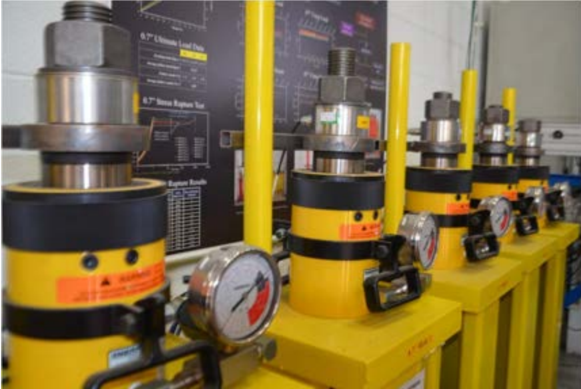
Figure 3.3-2 In-line load cells and hydraulic pressure systems to monitor the force loss
