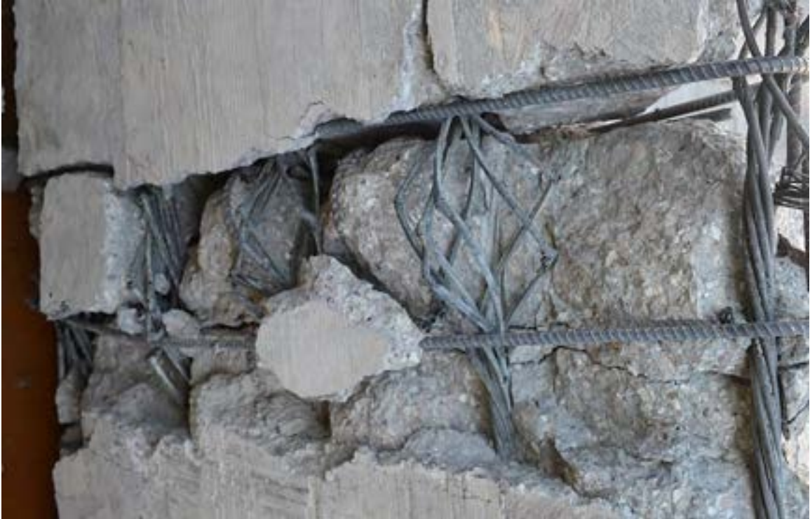
Figure 6.3-90 Rupture of CFCC strand at failure
