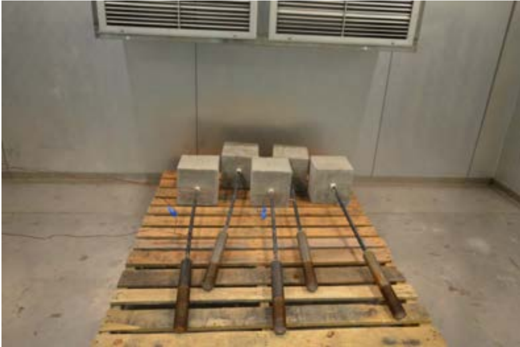
Figure 4.2-17 CFCC specimens exposed to 150 cycles of heating and cooling
