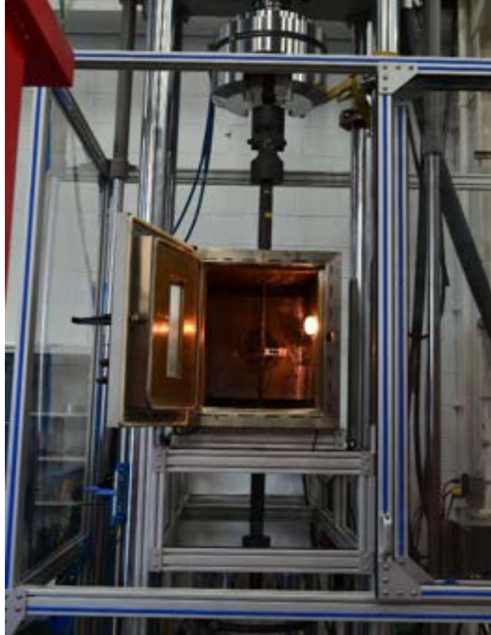
Figure 6.2-4 Test specimens inside the environmental chamber before the heating phase
