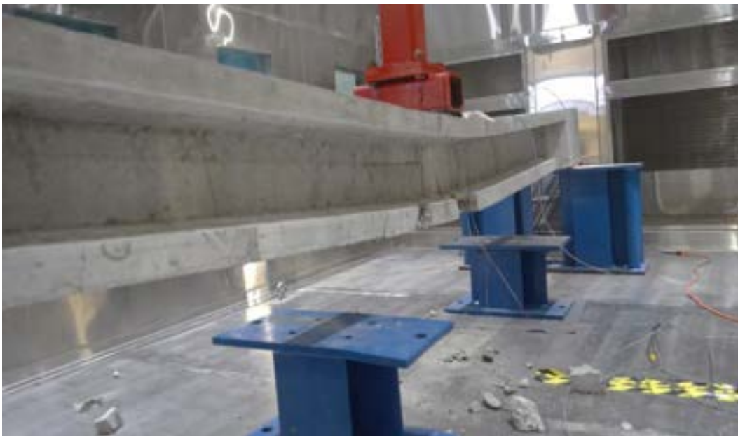
Figure 7.3-53 Failure of Beam C1 under three-point loading
