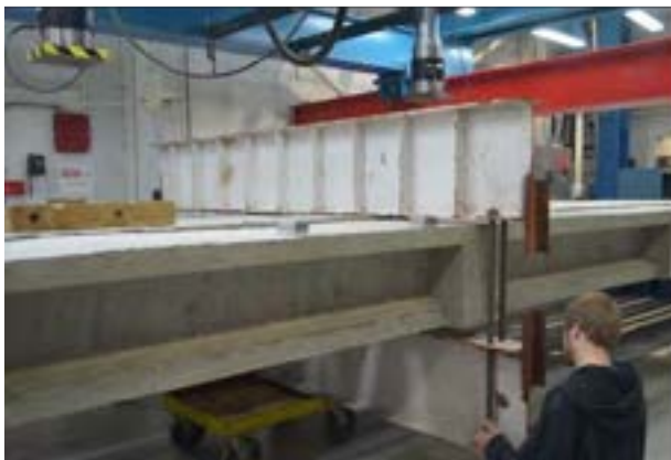
Figure 8.5-7 Beam leveling and wooden end plates at the beam ends
