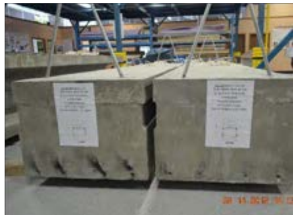
Figure 6.3-15 Prestressed CFCC bulb T beam (left) and box beam (right)
