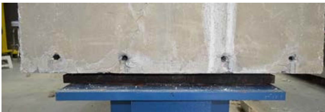
Figure 6.3-78 Close-up view showing CFCC strand debonded from concrete
