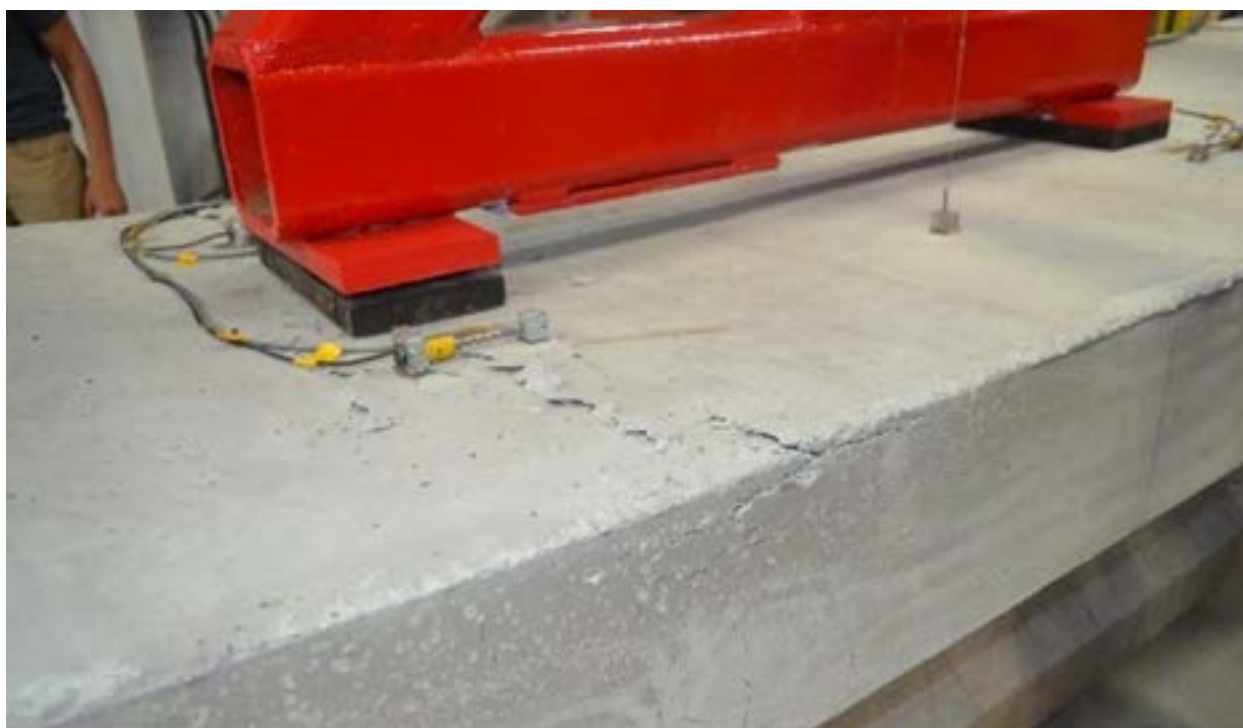
Figure 5.5-12 Spalling of concrete at the top surface of the deck slab at failure of Beam C0.6
