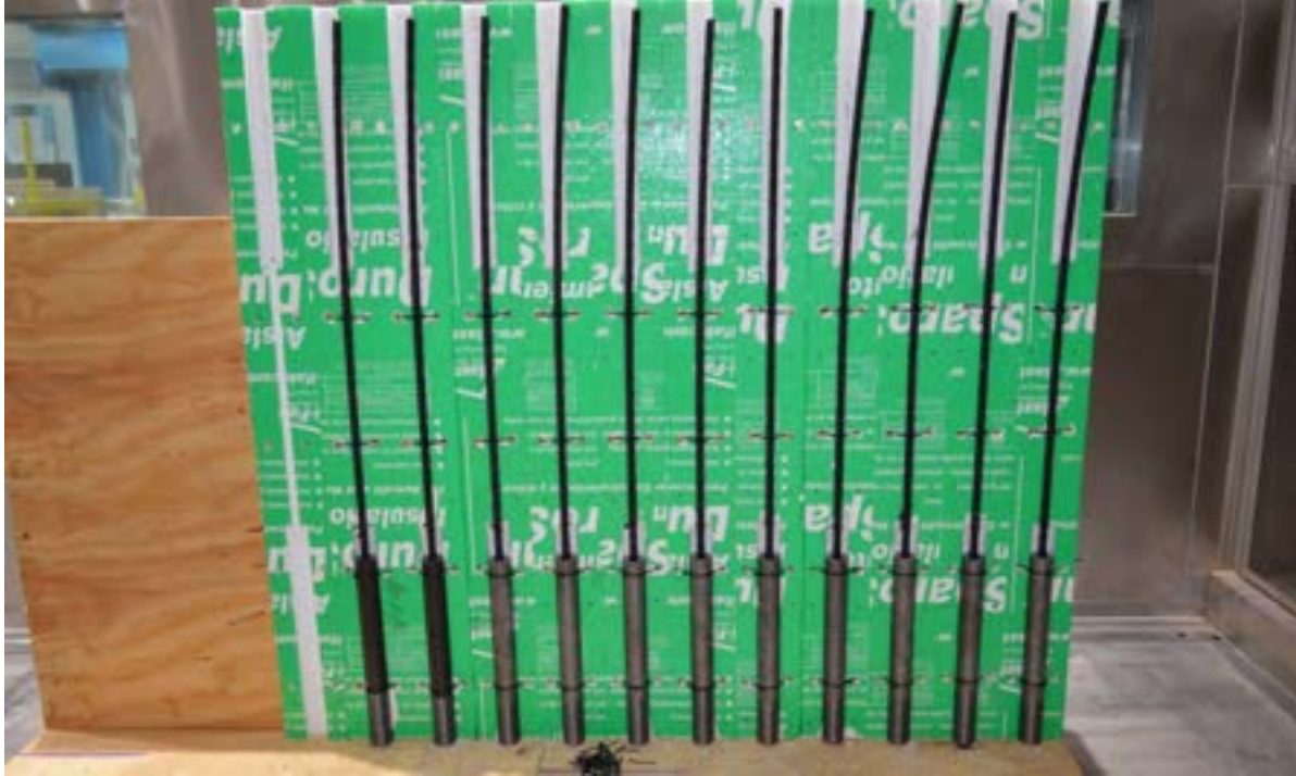
Figure 2.4-3 Placing anchors with CFCC strands in a custom-made wooden stand
