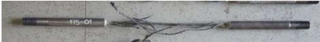
Figure 6.2-7 Failure of CFCC specimen at 347 °F (175 °C)
