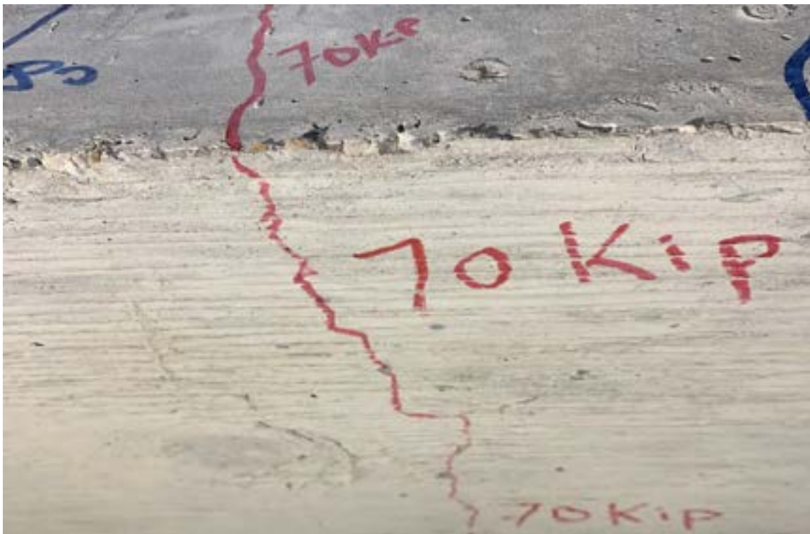
Figure 8.8-8 First flexural crack at the bottom of the bridge model after 70 kip (312 kN) load cycle
