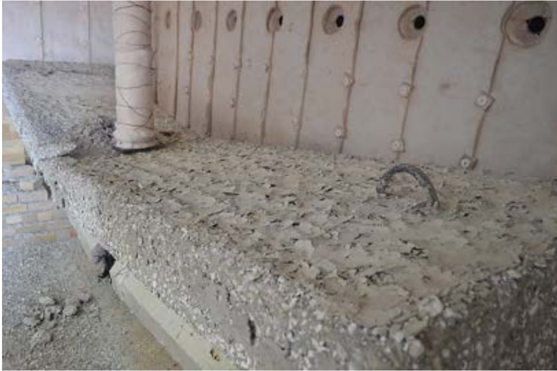
Figure 6.3-55 Excessive spalling of concrete 48 hours after fire test
