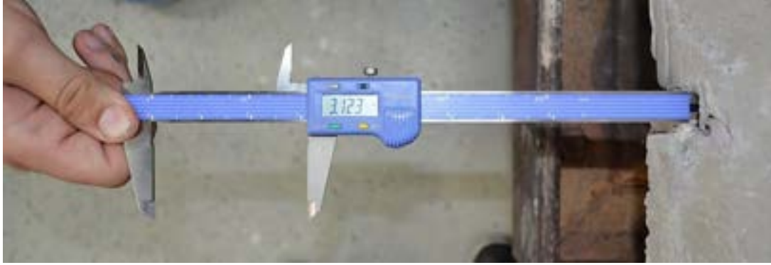
Figure 6.3-79 Measuring depth of slippage from the end of the beam
