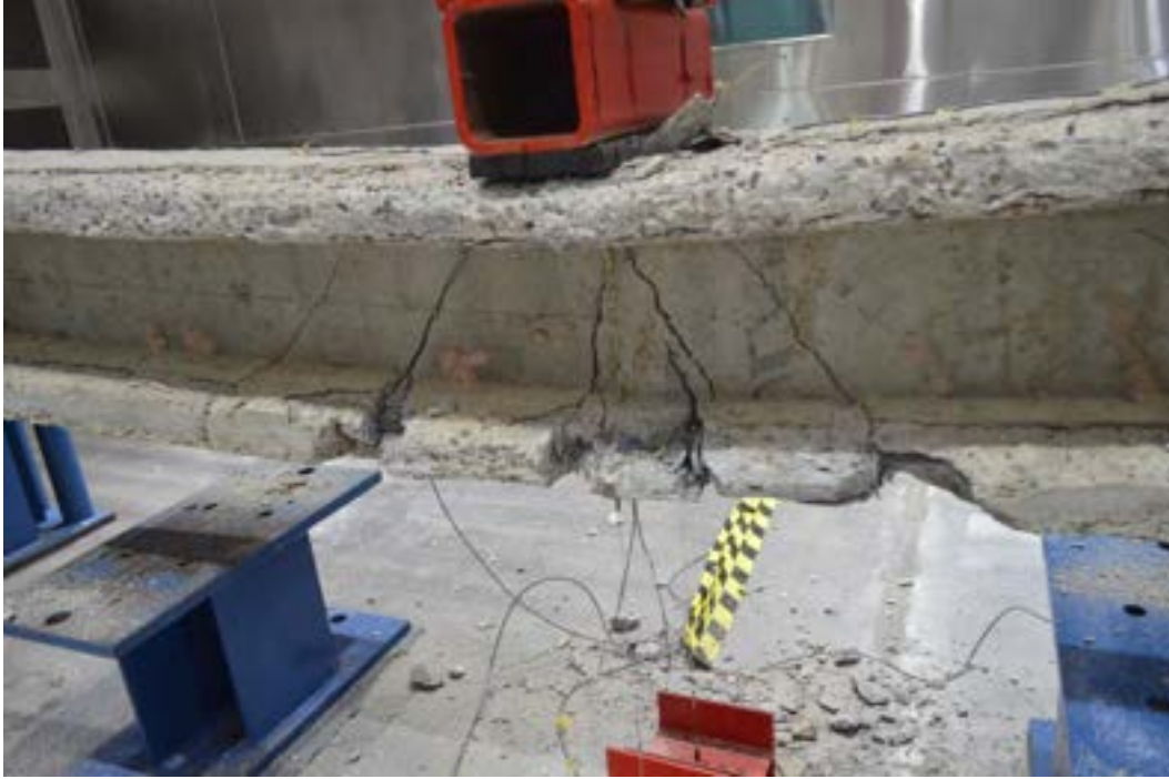
Figure 7.3-80 Failure of Beam H2 under three-point loading
