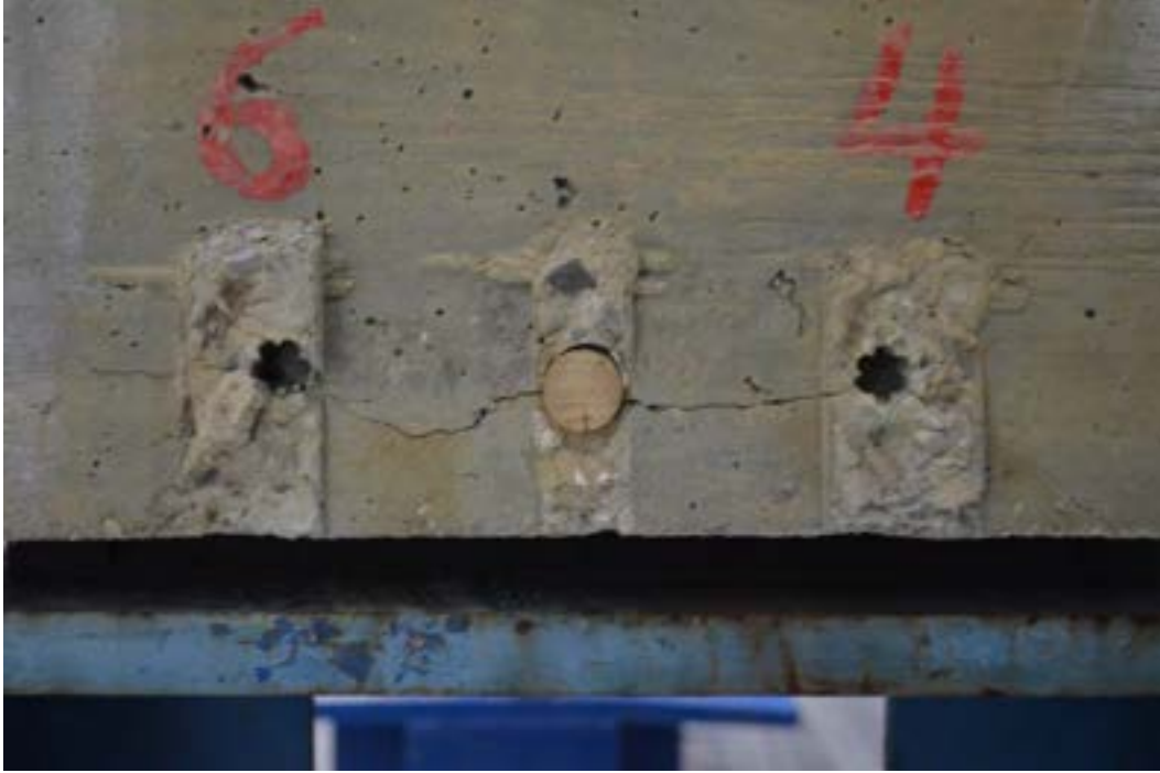
Figure 7.3-70 End view showing slippage of CFCC strands in Beam F2 after failure
