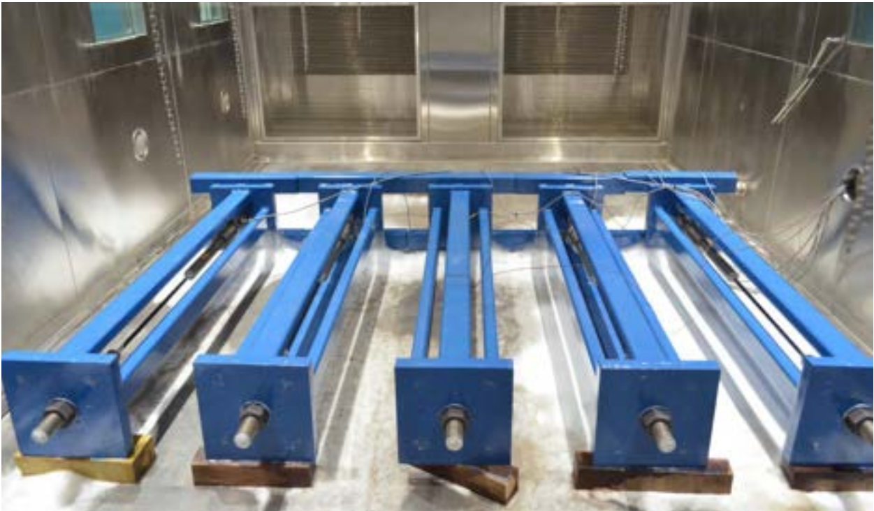
Figure 7.2-3 Stressed CFCC strands exposed to 150 freeze-thaw cycles
