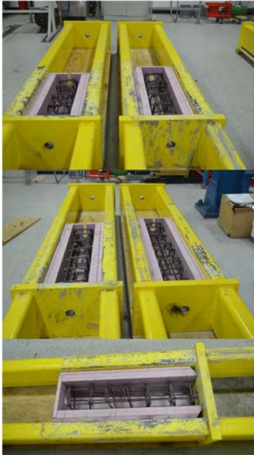
Figure 4.4-6 Second set of development length specimens, measuring 8 in. \times 8 in. with lengths of 24, 30, 36, 42, and 48 in. (No. 3 steel stirrups every 6 in.), prior to pouring concrete
