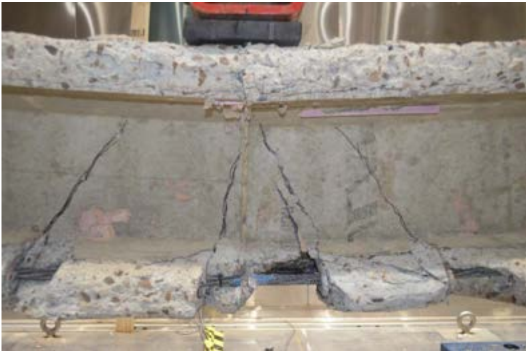
Figure 7.3-81 Debonding of CFCC strands and spalling of concrete at midspan of Beam H2
