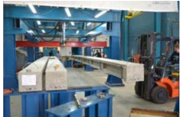
Figure 8.5-6 Lifting and placing the beams on steel supports with 3-in. (76-mm) gaps
