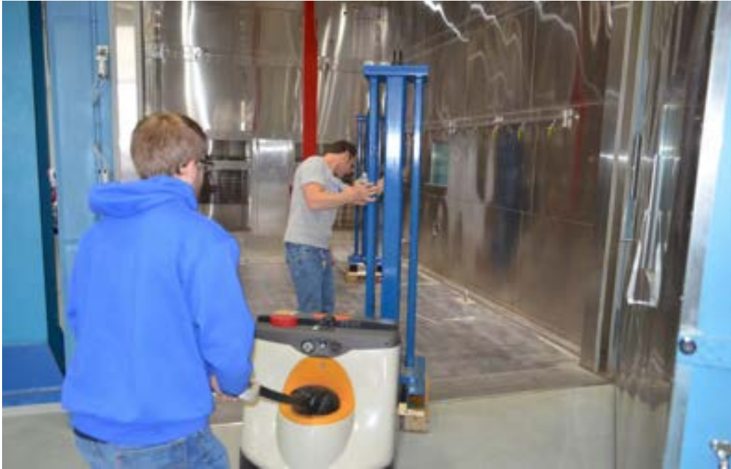
Figure 7.3-33 Placing two stressed CFCC strands in the environmental chamber to be exposed to a temperature of 176 °F (80 °C) for 24 hours
