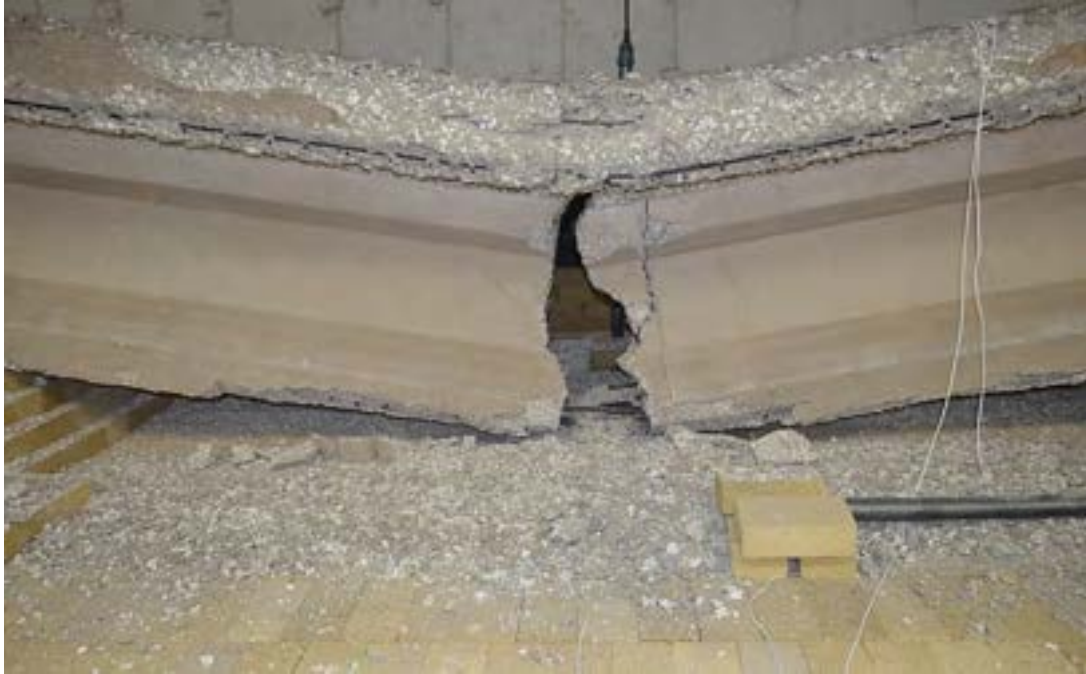
Figure 6.3-65 Excessive spalling of concrete after 48 hours
