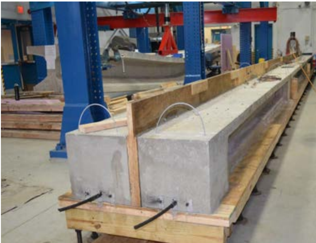
Figure 7.3-11 Beams after prestress release with the middle strand in each beam fully debonded
