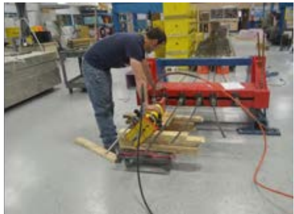
Figure 6.3-9 Installation of prestressing anchorage and prestressing of strand
