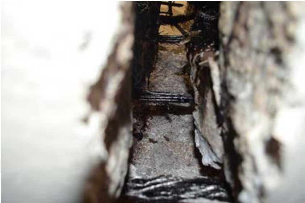
Figure 6.3-36 CFCC strand exposed at midspan at failure
