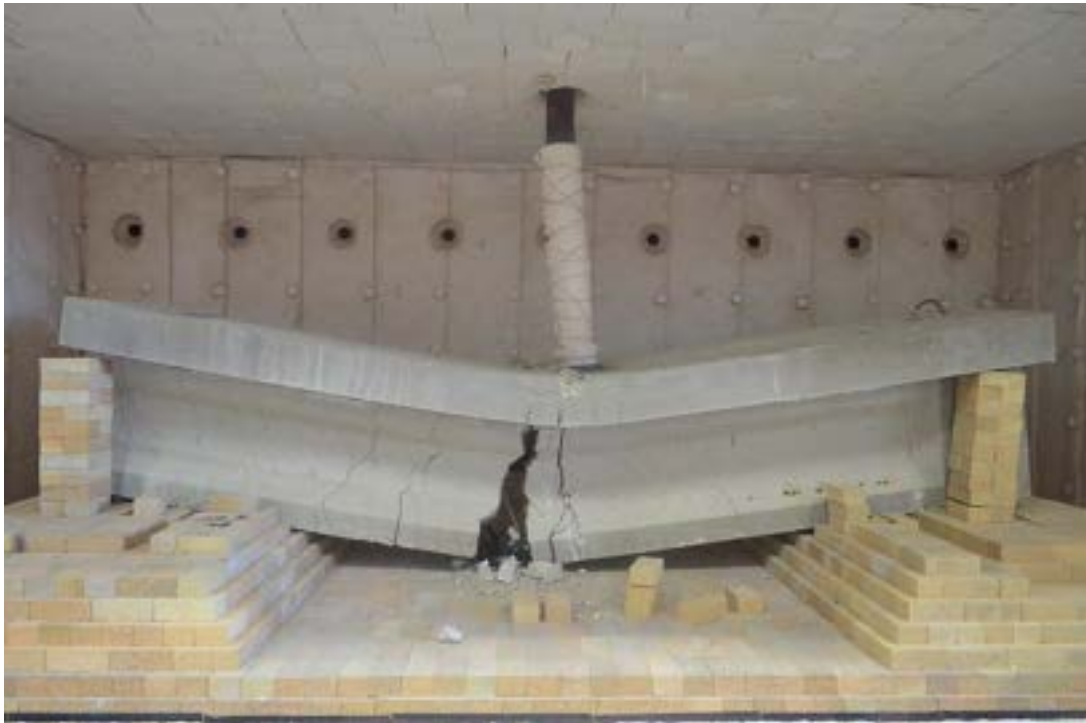
Figure 6.3-52 Beam I-0.6C after fire test
