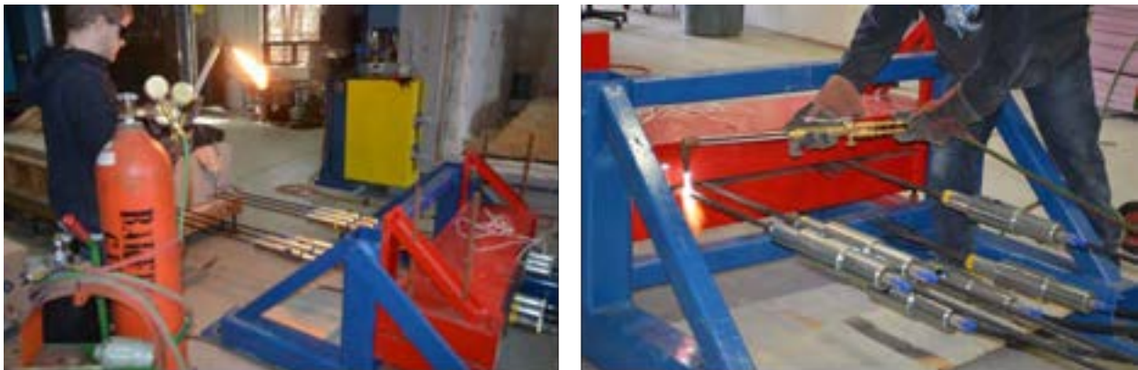
Figure 8.4-8 Prestress release by heating the steel strands using an acetylene/oxygen torch
