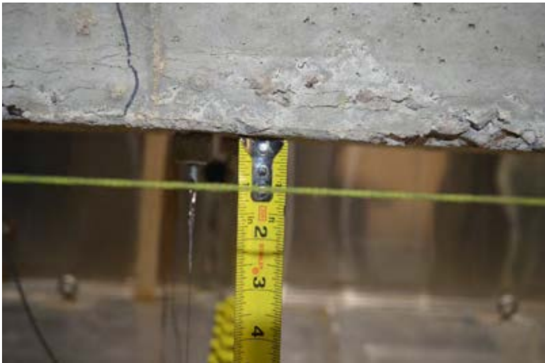
Figure 7.3-67 Midspan camber of 1.0 in. (25.4 mm) in Beam F2 before flexural testing
