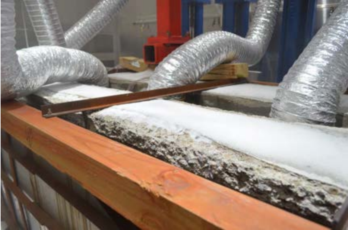
Figure 7.3-45 Deterioration of decked bulb T beams after exposure to 300 freeze-thaw cycles
