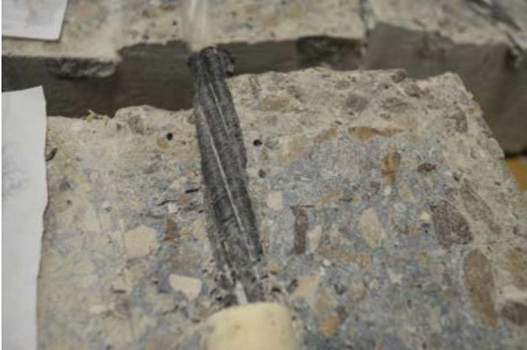
Figure 4.2-13 Exposing the bonded length of CFCC specimen in pullout specimen after testing
