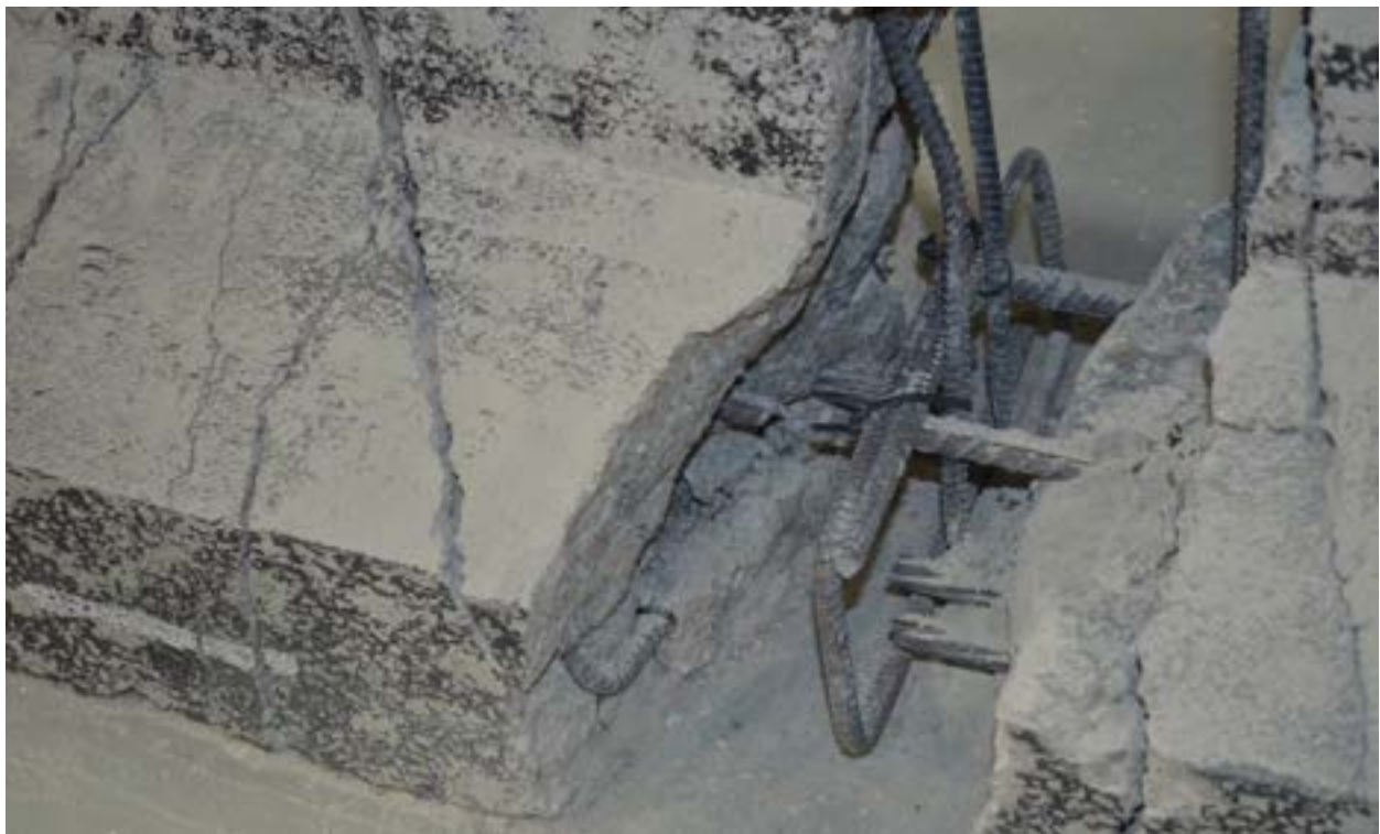
Figure 5.5-18 Rupture of steel prestressing strands during failure of Beam S0.6
