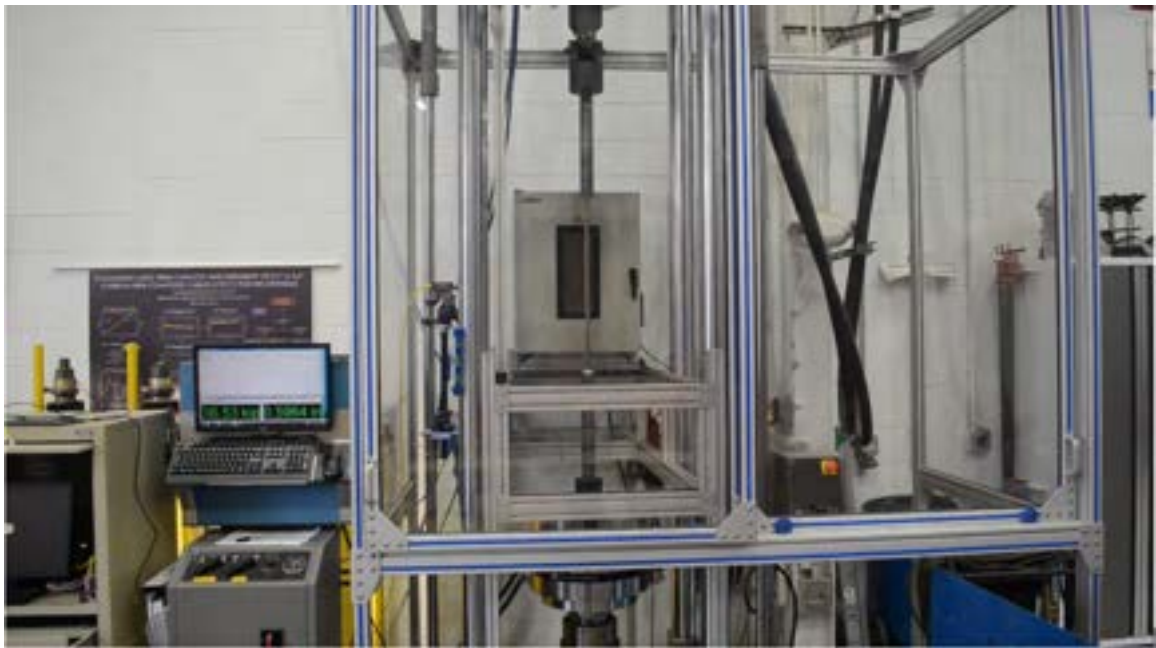
Figure 3.2-5 Creep rupture test setup for 0.7" CFCC specimens with stress levels higher than 95 % of the CFCC average tensile strength
