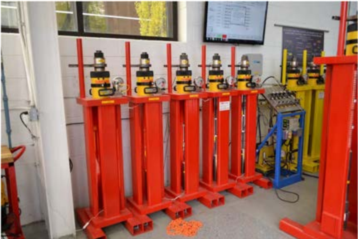
Figure 3.2-3 Creep test setup of 0.7" CFCC specimens with closed loop hydraulic system
