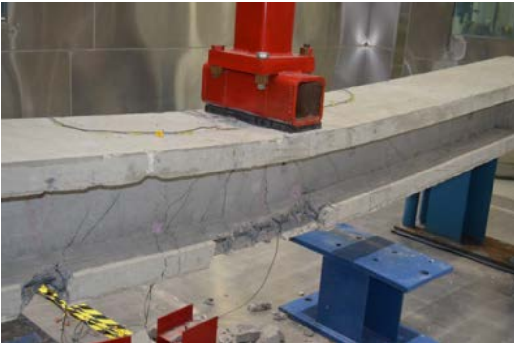
Figure 7.3-57 Failure of Beam C2 under three-point loading
