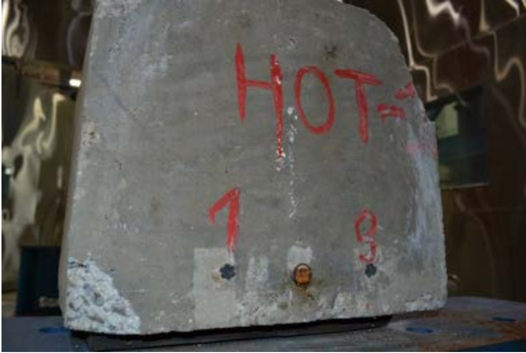
Figure 7.3-76 End view showing slippage of CFCC strands in Beam H1 after failure
