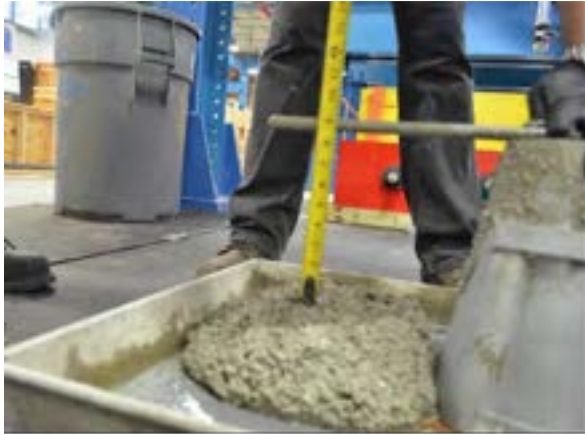
Figure 6.3-11 Slump test and casting of concrete cylinders
