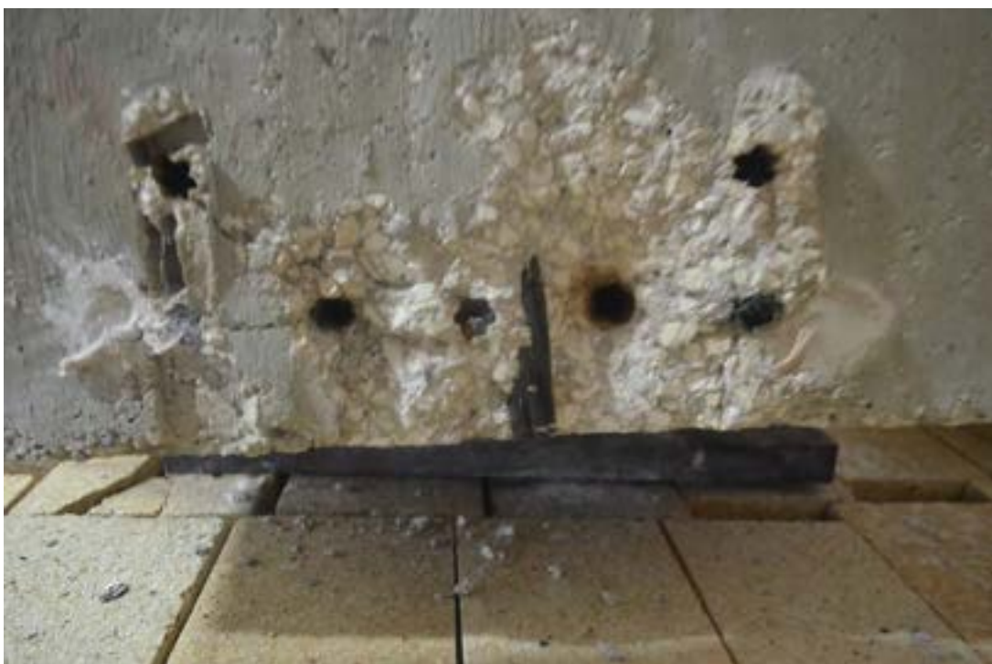
Figure 6.3-54 CFCC strands slippage from concrete at failure
