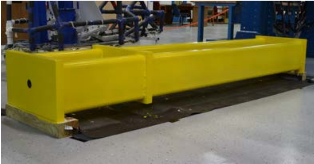
Figure 4.4-3 Development length frame for a single CFCC specimen
