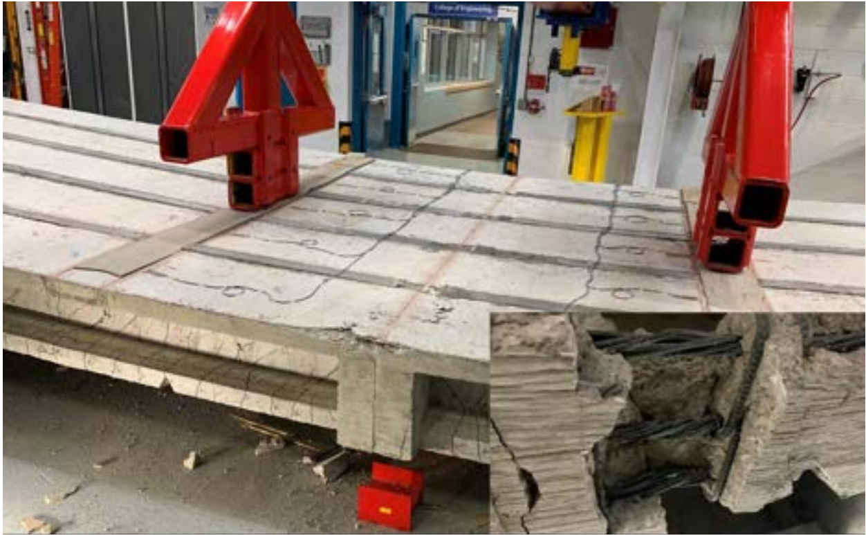
Figure 8.8-20 Rupture of CFCC strands accompanied by partial concrete crushing after failure
