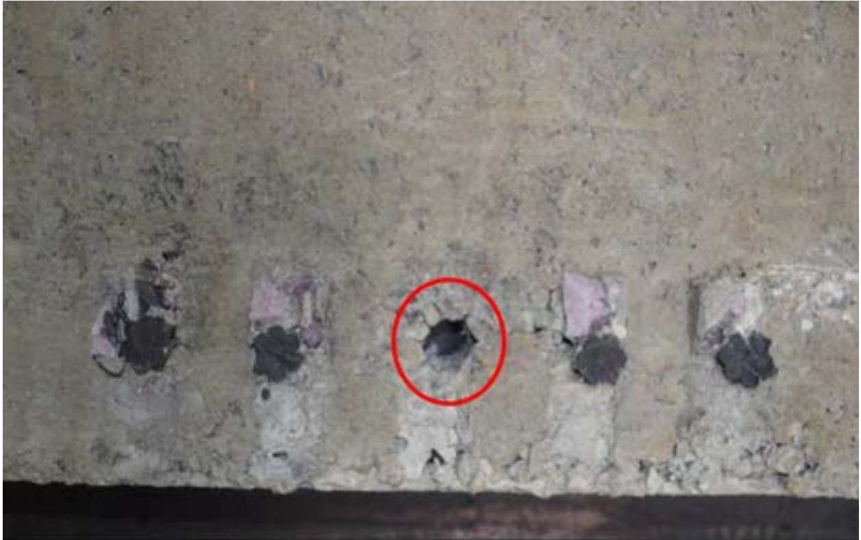
Figure 5.5-5 Slippage of partially debonded CFCC strands prior to failure of Beam C0.7
