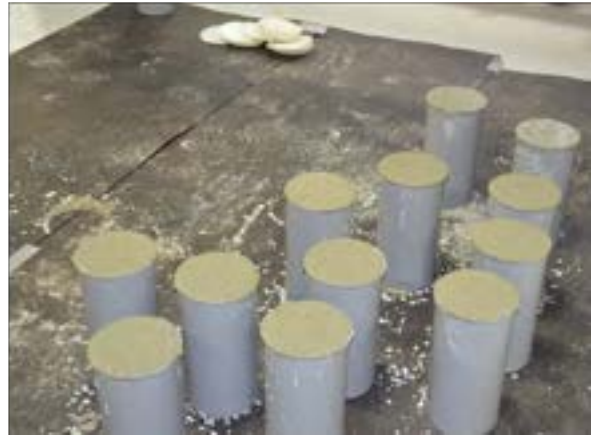
Figure 6.3-11 Slump test and casting of concrete cylinders
