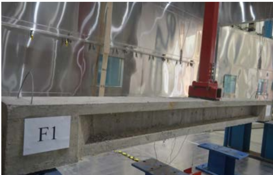
Figure 7.3-61 Three-point loading of Beam F1
