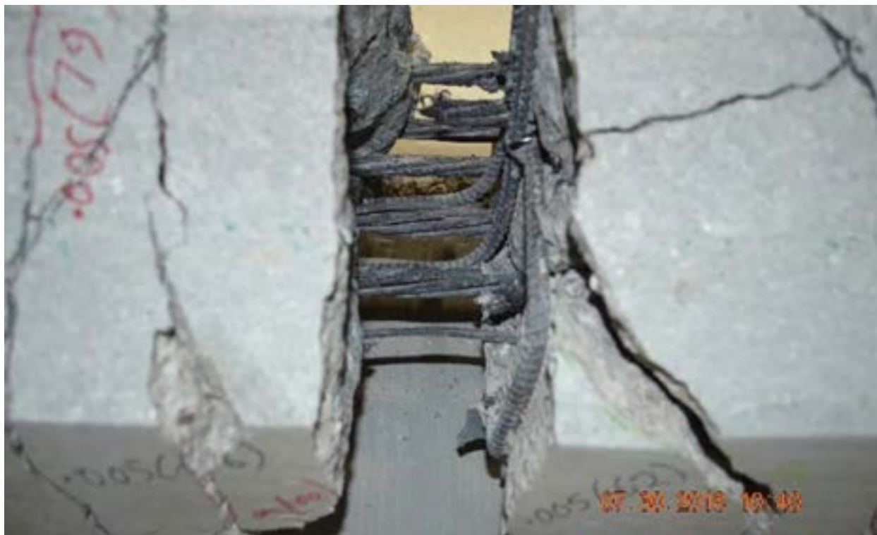
Figure 5.5-11 Rupture of CFCC prestressing strands at failure of Beam C0.6
