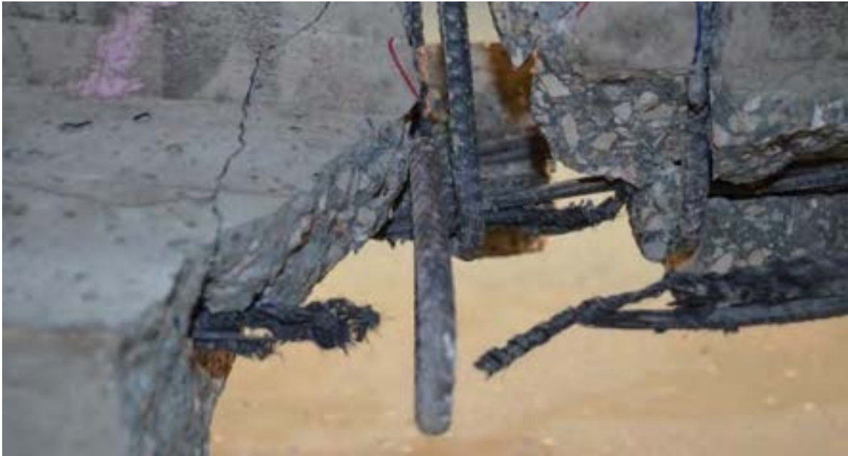
Figure 8.7-7 Spalling of concrete and rupture of CFCC strands after failure of control beam
