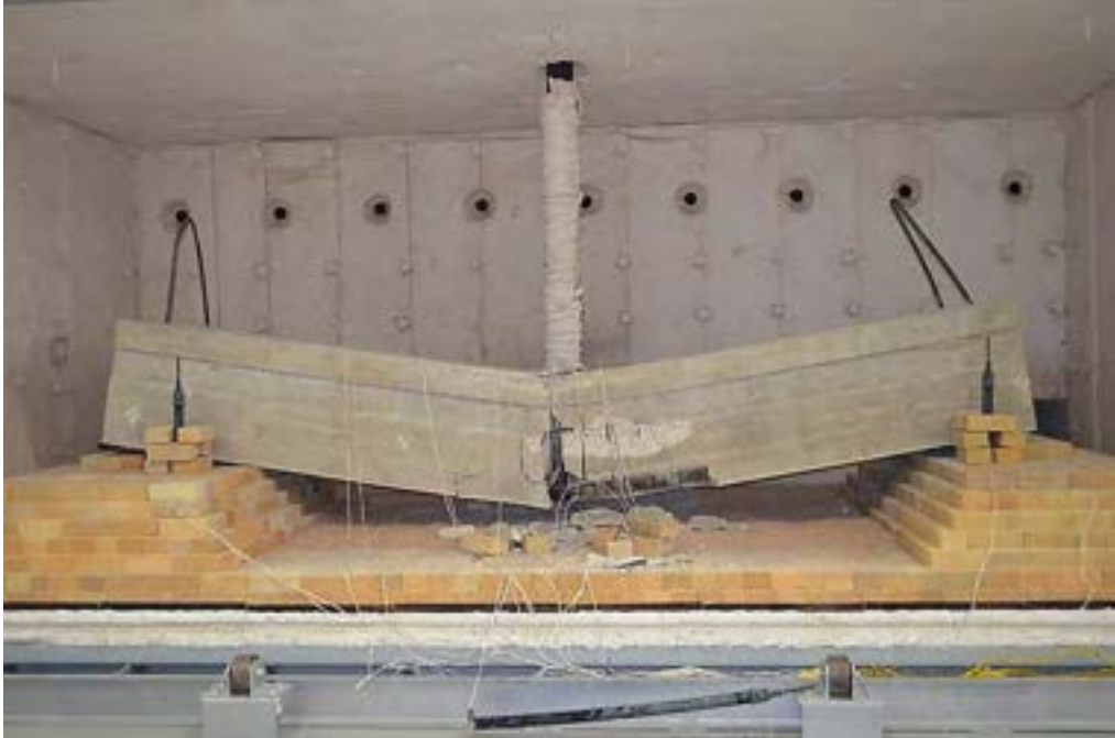
Figure 6.3-35 Beam B-0.7C after fire test
