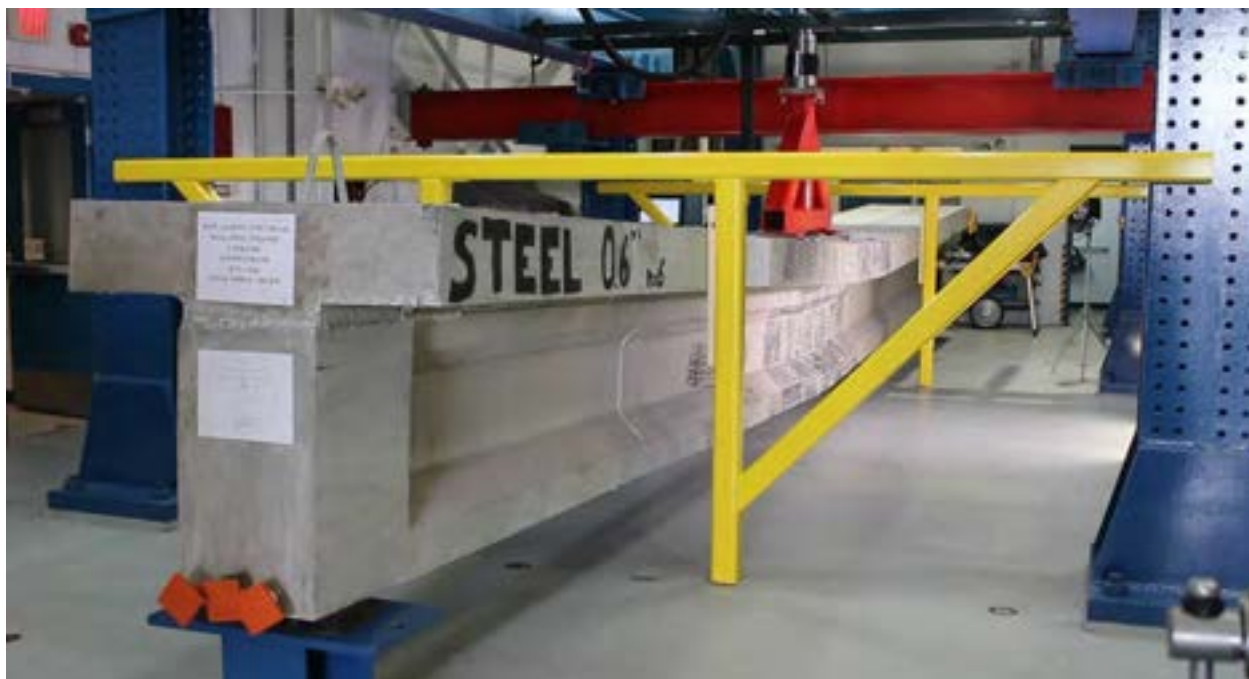
Figure 5.4-1 Test setup of full-scale AASHTO I-beams
