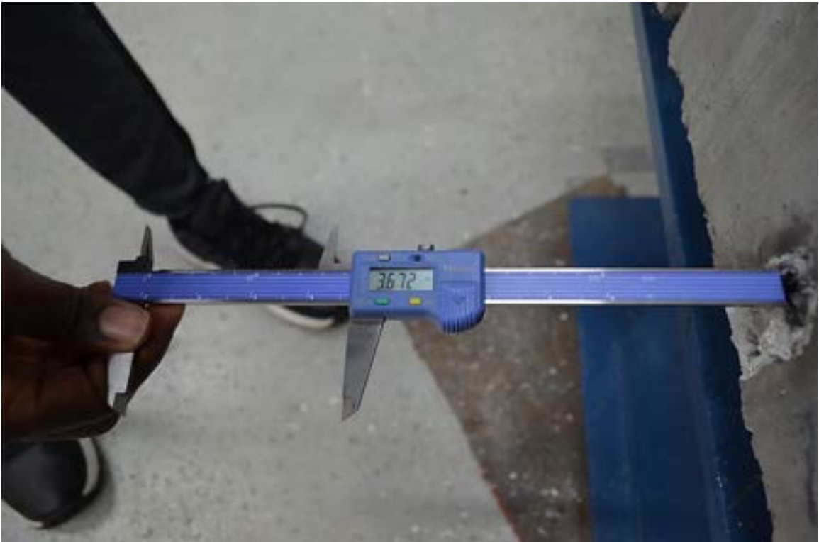
Figure 6.3-91 Measuring strand slip at the end of the beam
