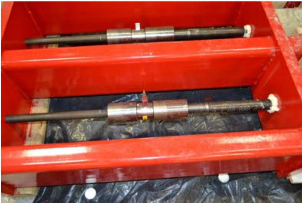
Figure 4.3-4 In-line load cell attached to the end of the CFCC strands
