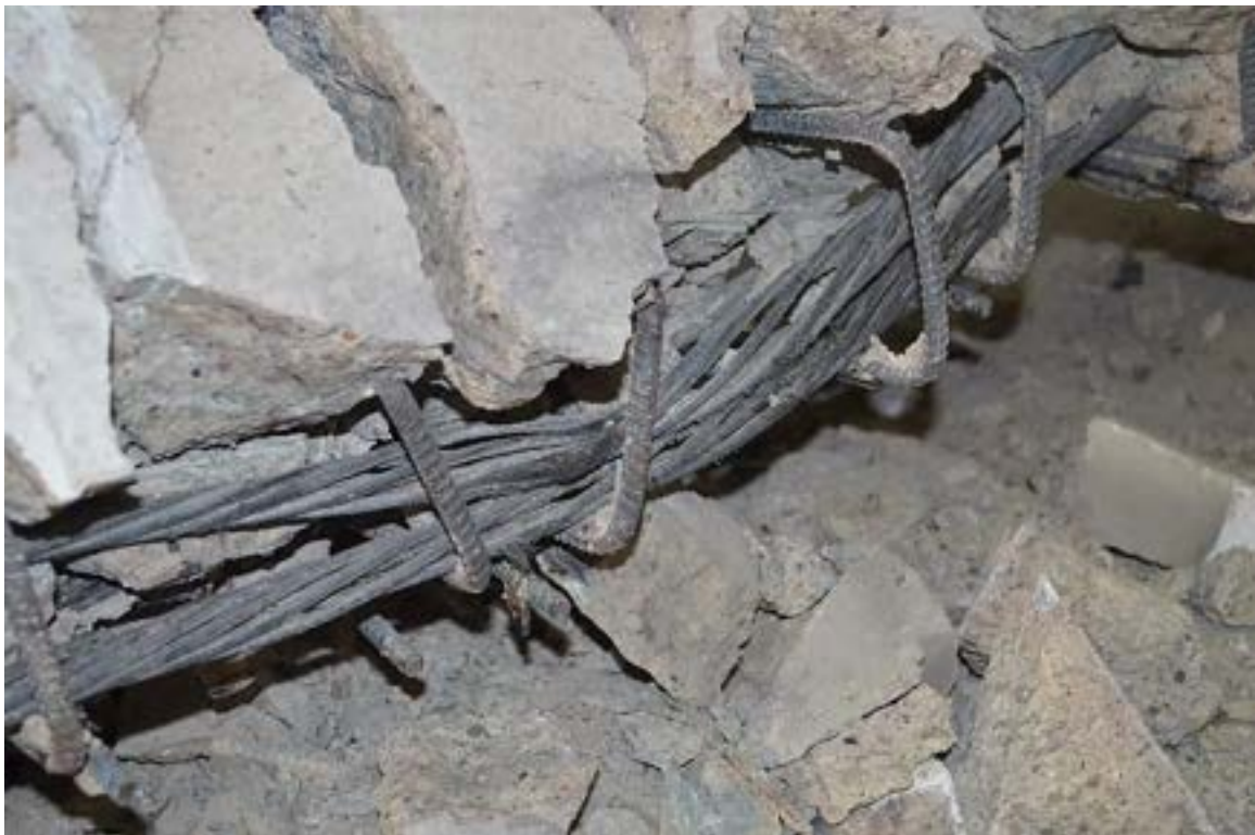
Figure 6.3-102 Rupture and slippage of CFCC strand at failure
