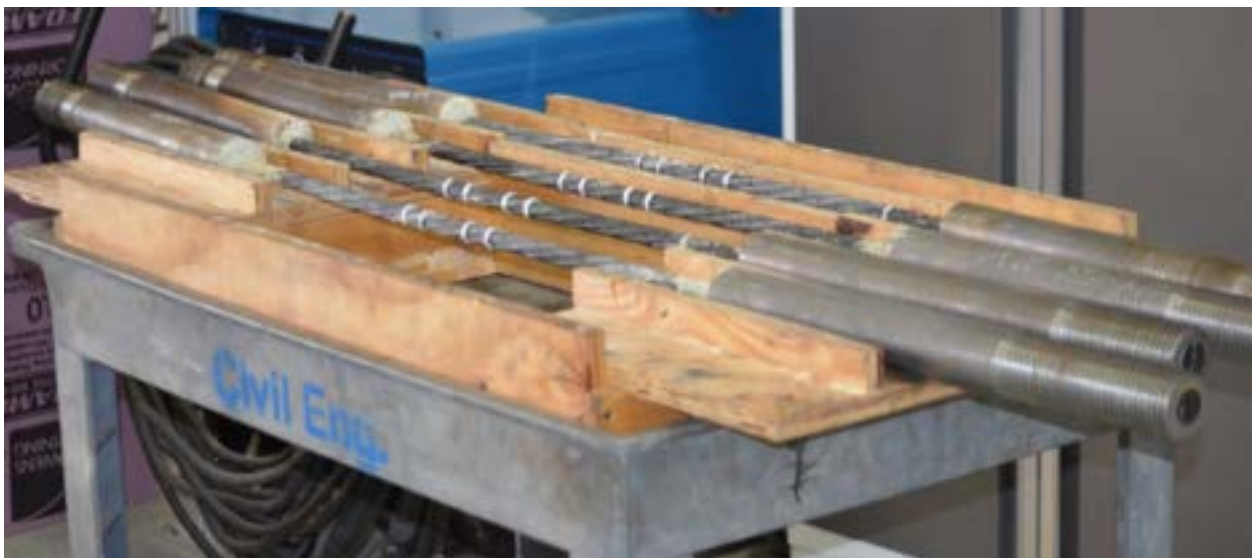
Figure 7.2-10 CFCC specimens after release from the stressing frames
