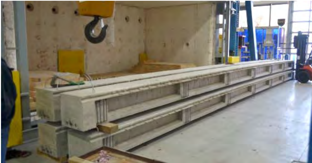
Figure 8.5-5 Individual beams of the bridge model after construction
