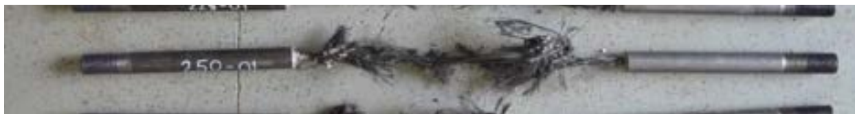
Figure 6.2-10 Failure of CFCC specimen at 482 °F (250 °C)
