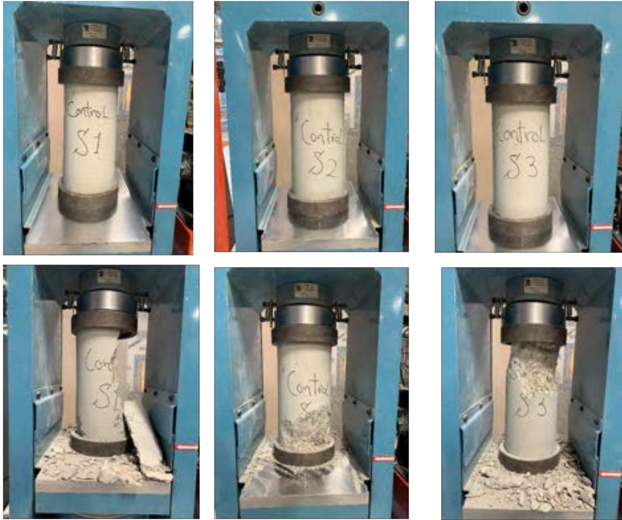
Figure 7.3-51 Testing and failure of control cylinders
