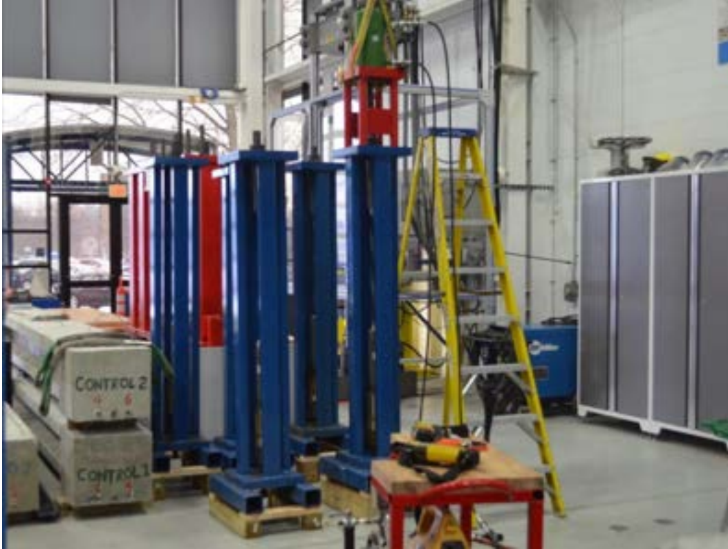
Figure 7.2-7 Stressing CFCC strands for 300 freeze-thaw cycles
