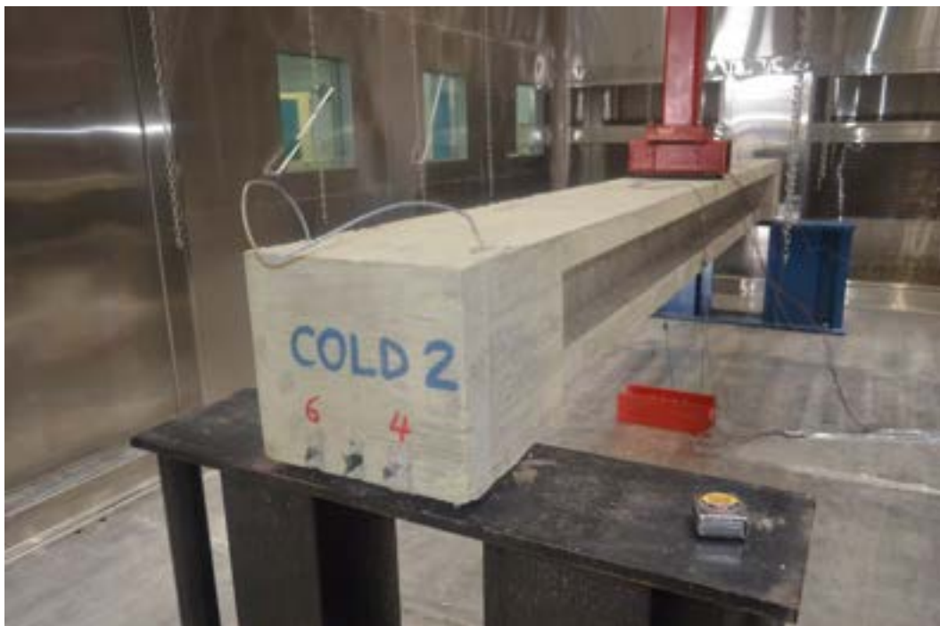
Figure 7.3-22 Beam F2 under three-point loading in the environmental chamber
