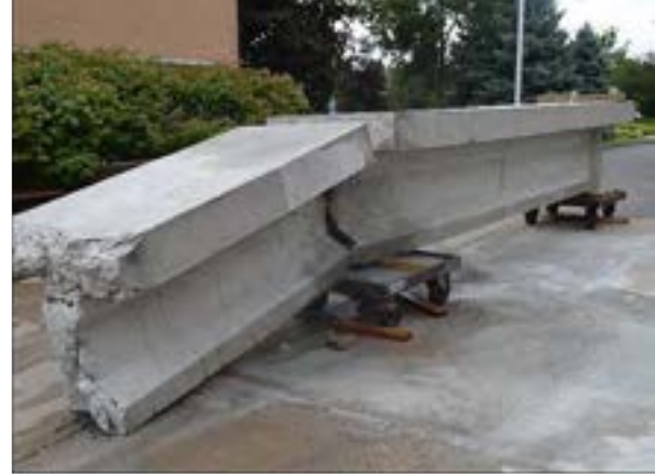
Figure 6.3-17 Cutting through the web with a circular concrete saw
