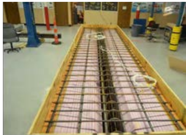
Figure 6.3-7 Assembling the reinforcement cage around the molded Styrofoam
