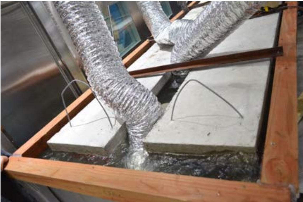
Figure 7.3-38 Decked bulb T beams during freezing and thawing cycles
