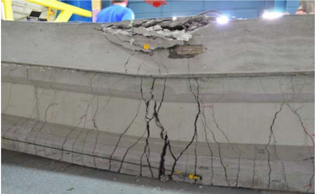
Figure 5.5-17 Failure of Beam S0.6
