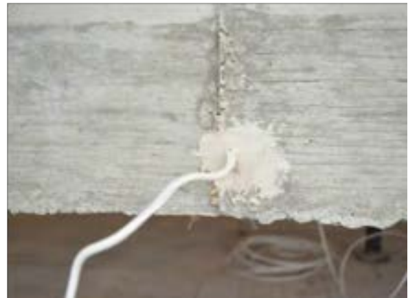
Figure 6.3-23 Installation of thermocouple into AASHTO I-beams
