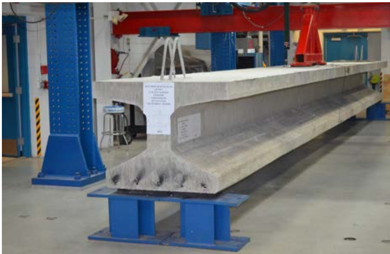
Figure 5.7-3 Flexural testing of full-scale bulb T beam under four-point-loading setup
