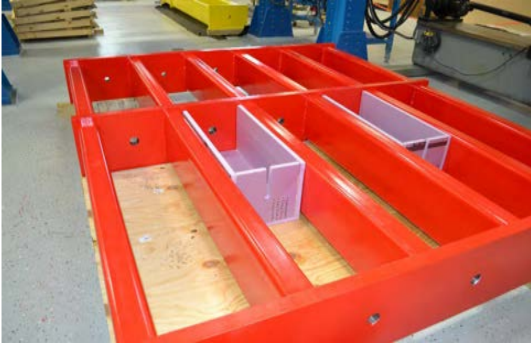
Figure 4.3-3 Transfer length frame hosting five specimens at one time
