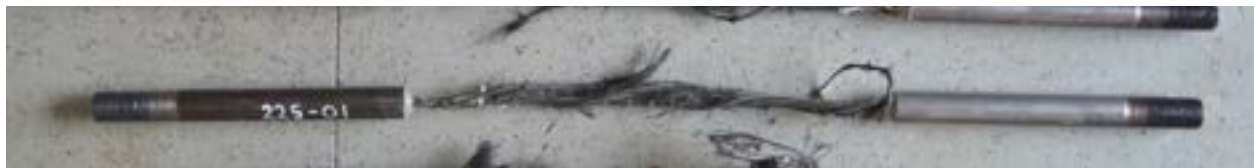
Figure 6.2-9 Failure of CFCC specimen at 437 °F (225 °C)
