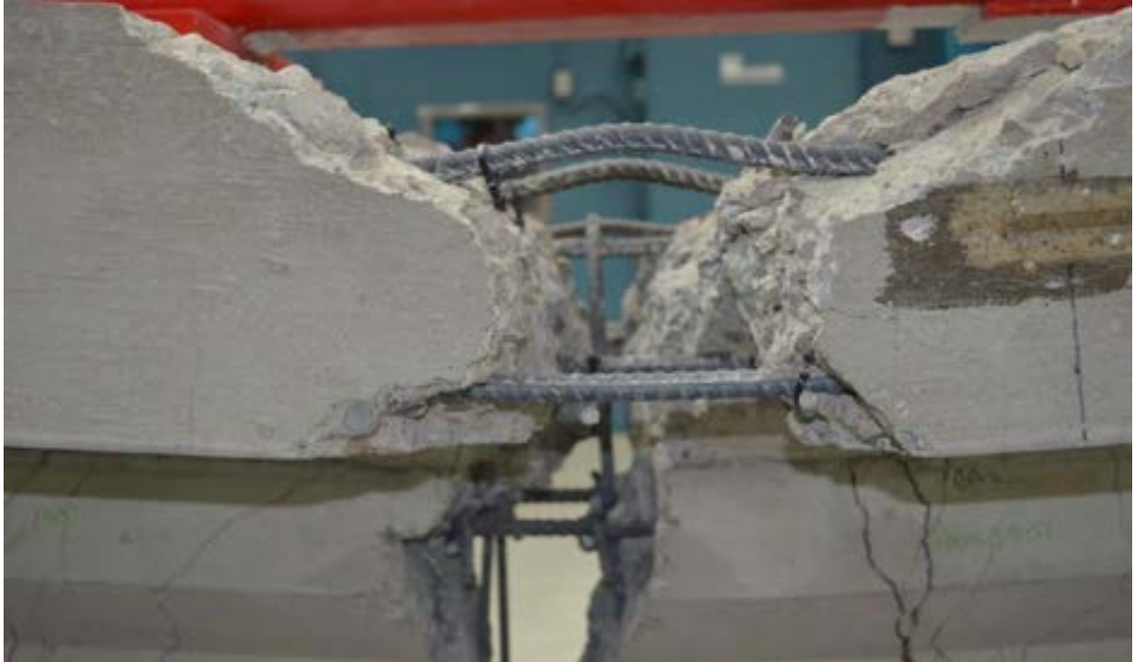
Figure 5.5-19 Buckling of top deck reinforcement at mid-span of Beam S0.6 at failure
