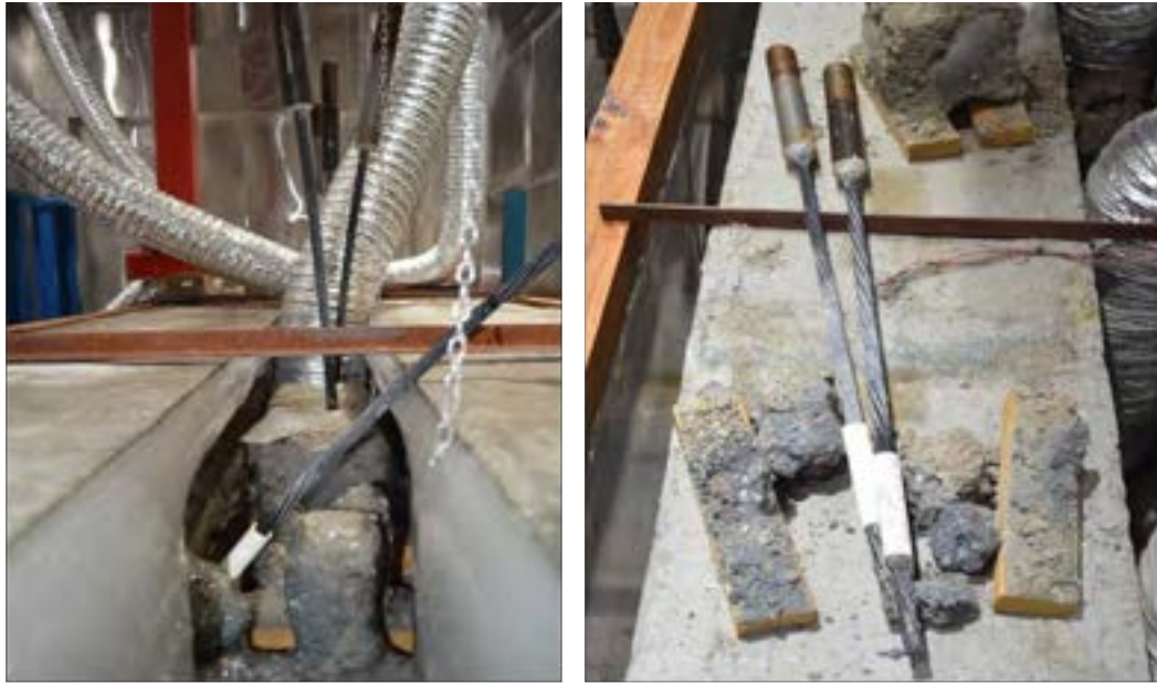
Figure 7.3-43 Deterioration of pullout specimens after exposure to 150 freeze-thaw cycles
