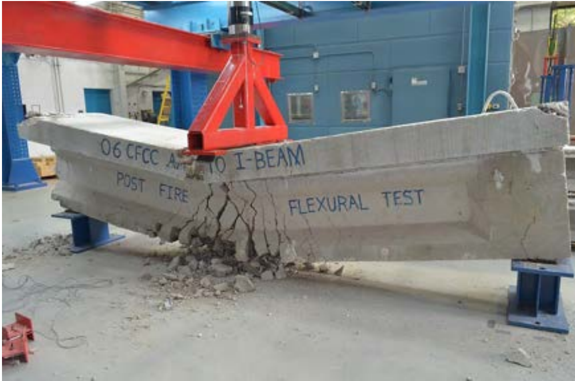
Figure 6.3-101 Failure of Beam RI-0.6C after flexural test
