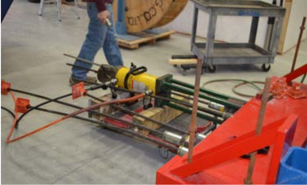
Figure 7.3-6 Prestressing the strands using a hydraulic pump and a jacking system
