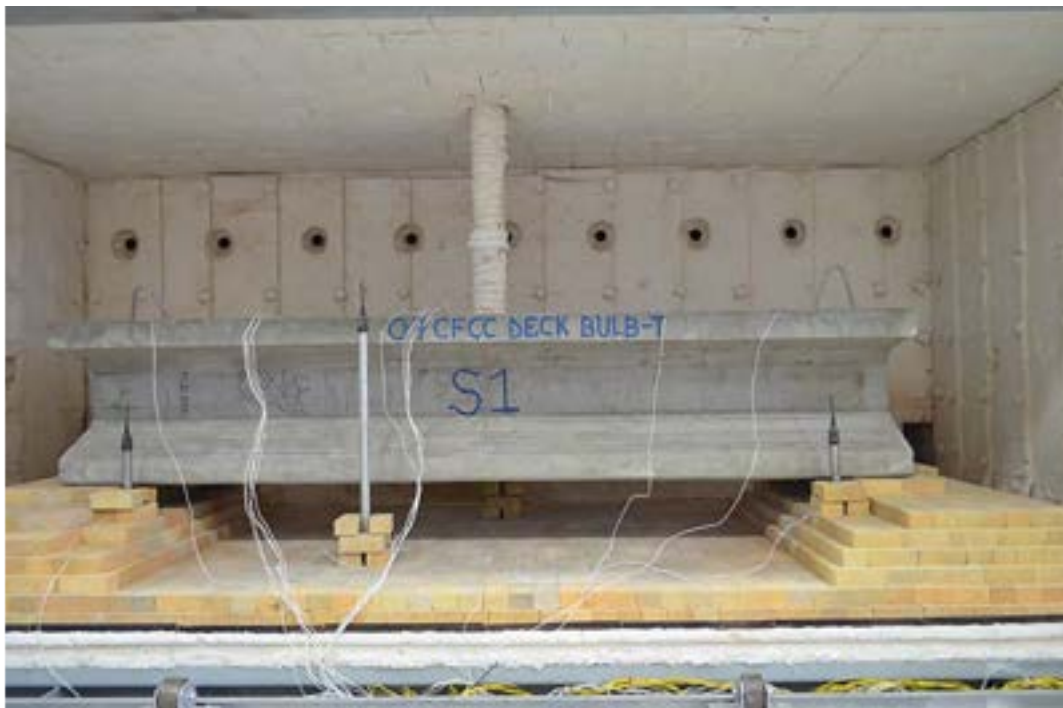
Figure 6.3-42 Beam T-0.7C before fire test
