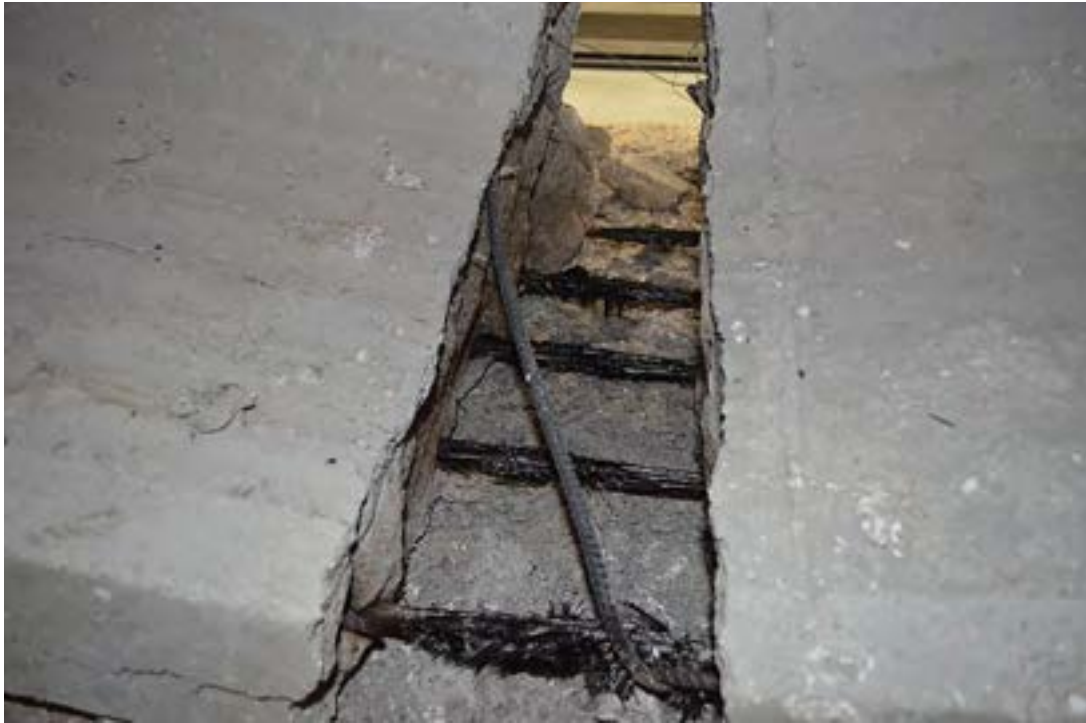
Figure 6.3-45 CFCC strands exposed at midspan at failure
