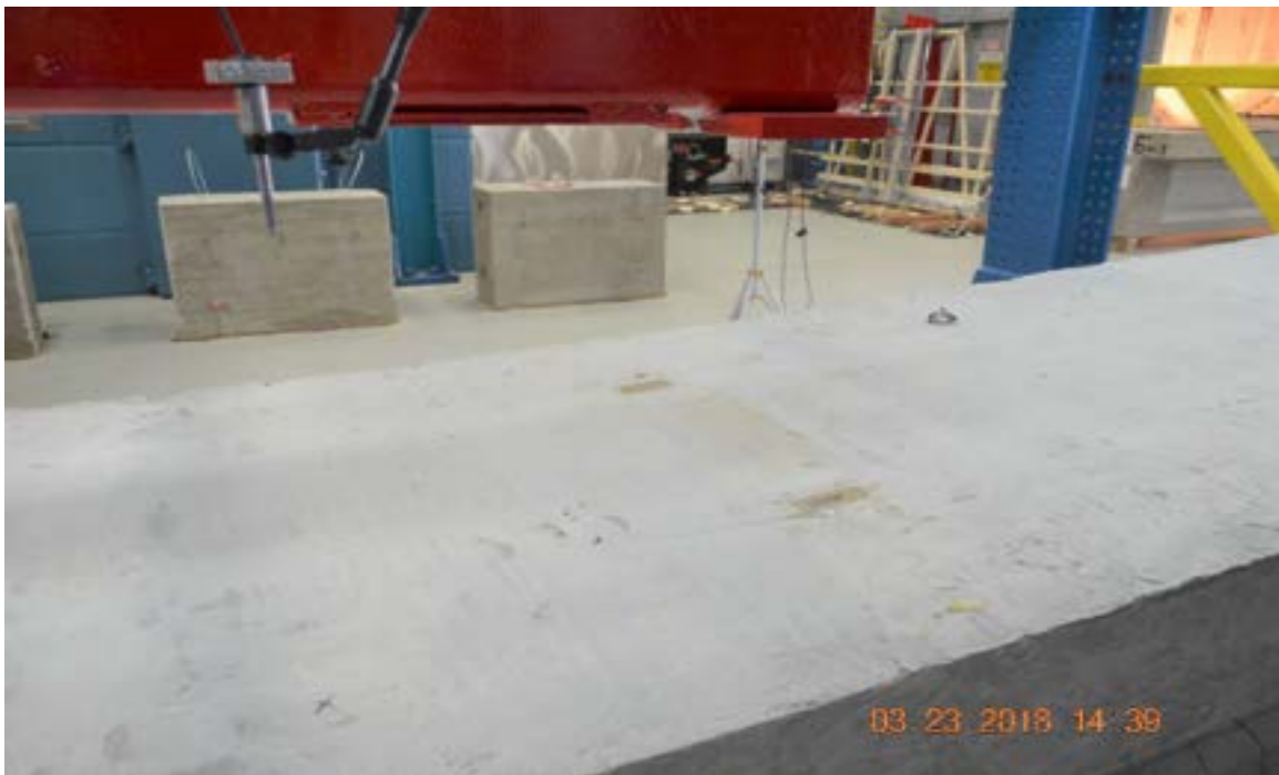
Figure 5.5-6 Deck surface of Beam C0.7 at failure with no concrete spalling
