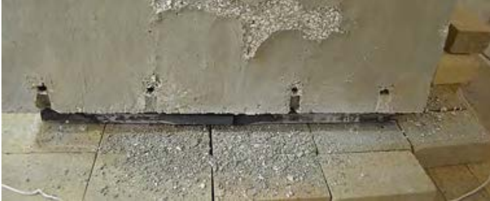
Figure 6.3-37 CFCC Strands debonded from concrete at failure
