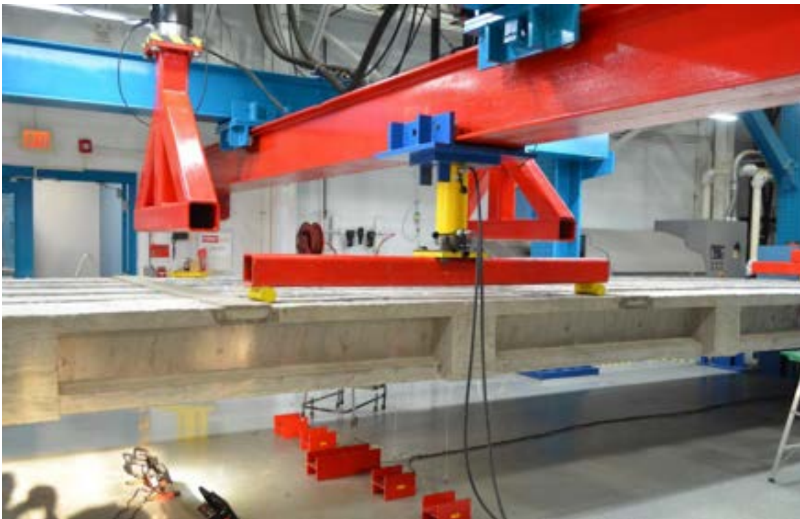
Figure 8.8-11 Test setup for evaluating the shear key joints of the bridge model
