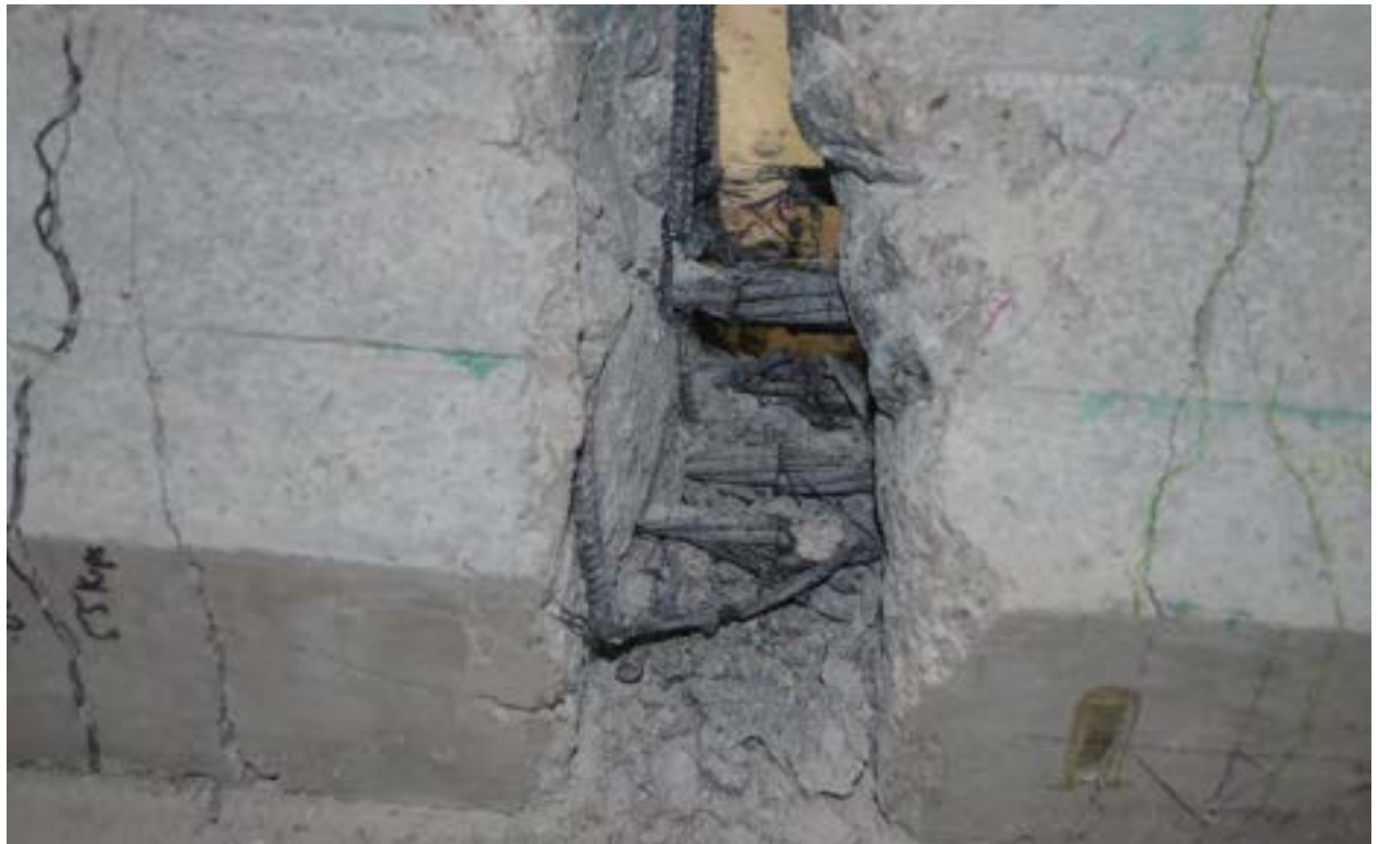
Figure 5.5-4 Rupture of CFCC strands at failure of Beam C0.7
