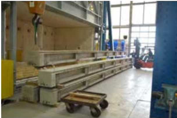
Figure 8.5-6 Lifting and placing the beams on steel supports with 3-in. (76-mm) gaps
