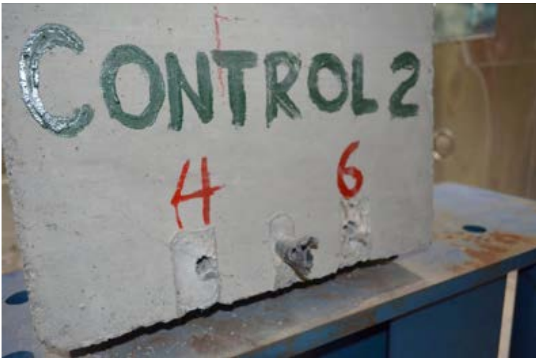
Figure 7.3-59 End view showing debonding of CFCC strands in Beam C2 after failure
