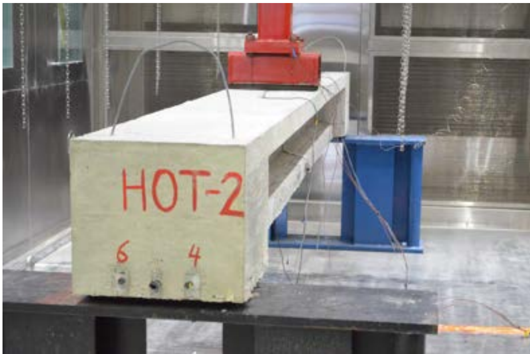
Figure 7.3-28 Beam H2 under three-point loading in the environmental chamber
