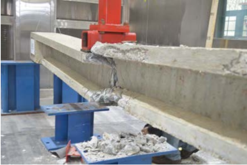
Figure 7.3-74 Failure of Beam H1 under three-point loading
