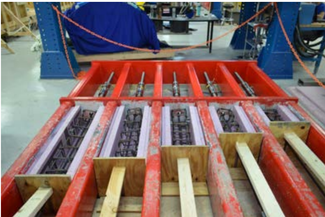
Figure 4.3-8 Second set of transfer length specimens prior to concrete pouring, measuring 8 in. \times 8 in. with lengths of 18, 24, 30, 36, and 42 in. (No. 3 steel stirrups every 6 in.)
