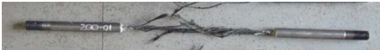
Figure 6.2-8 Failure of CFCC specimen at 392 °F (200 °C)
