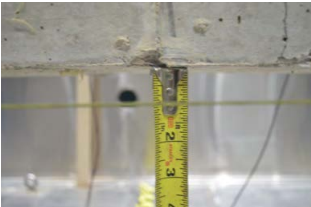
Figure 7.3-62 Midspan camber of 1.0 in. (25.4 mm) in Beam F1 before flexural testing
