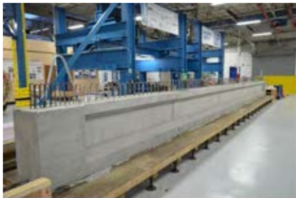
Figure 5.3-7 Completed Beam C0.6 after prestress transfer with minor cracks at the beam end
