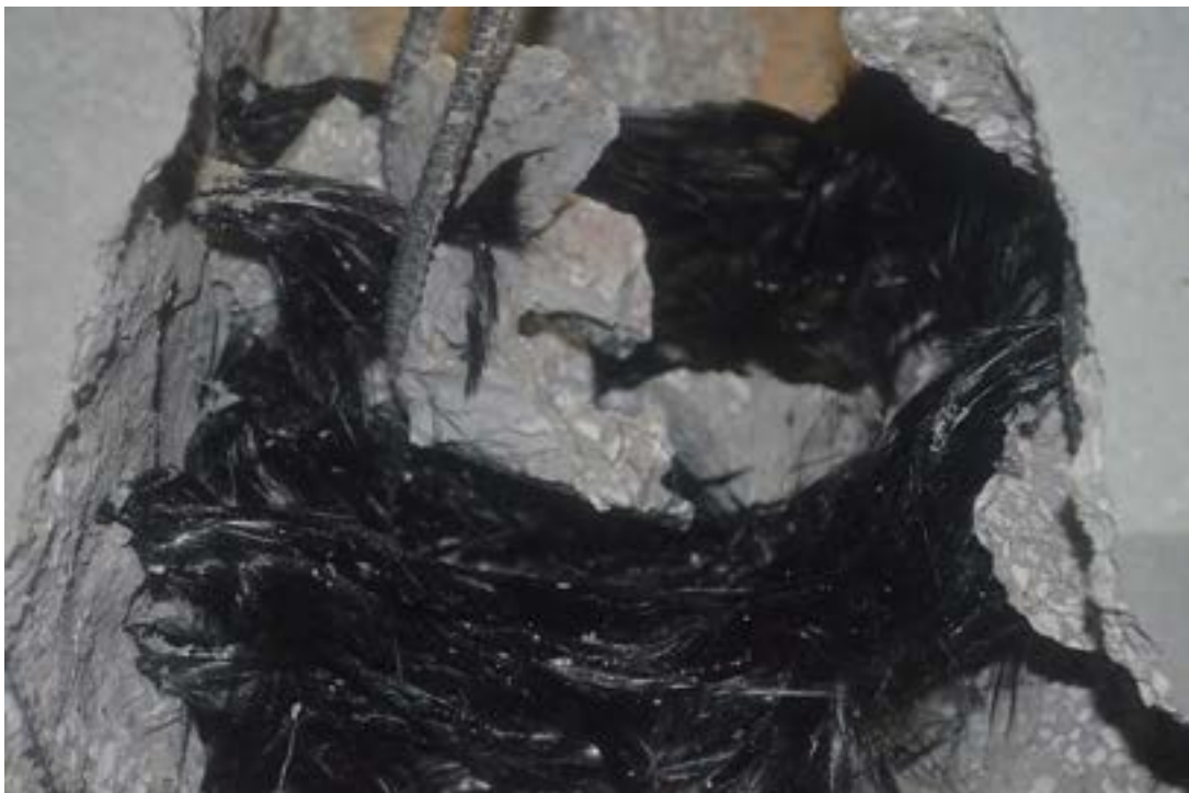
Figure 6.3-53 CFCC strands exposed at midspan at failure
