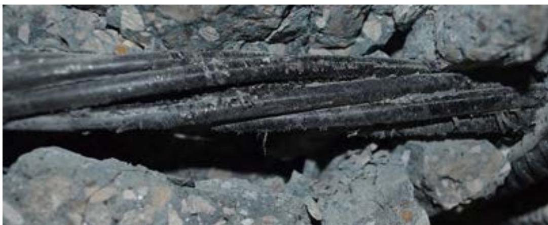
Figure 6.3-77 Close-up picture of CFCC strand after failure
