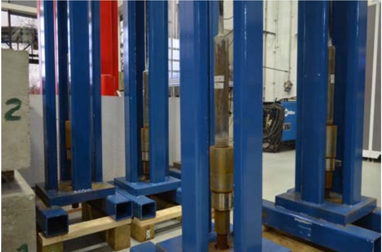
Figure 7.2-9 Unbonded CFCC specimens after exposure to 300 freeze-thaw cycles
