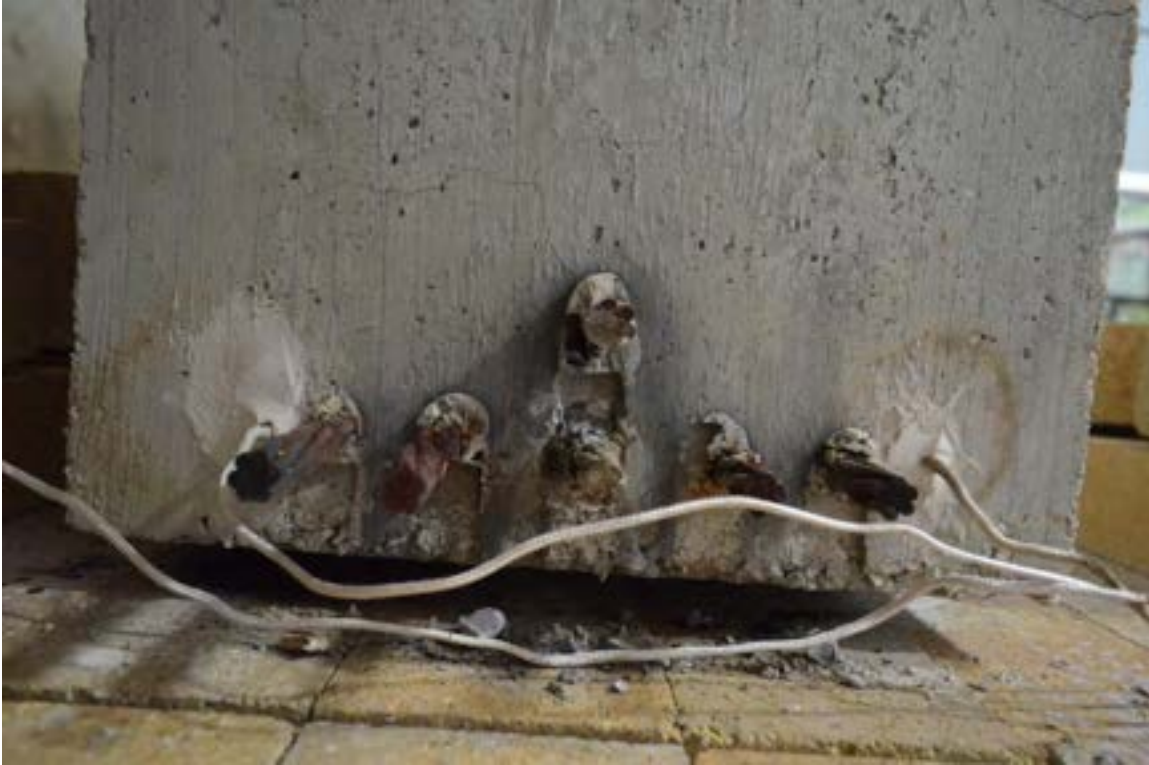
Figure 6.3-110 Prestressing strands remained bonded after fire test
