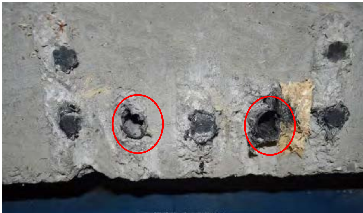
Figure 5.5-13 Slippage of partially debonded stands prior to failure of Beam C0.6
