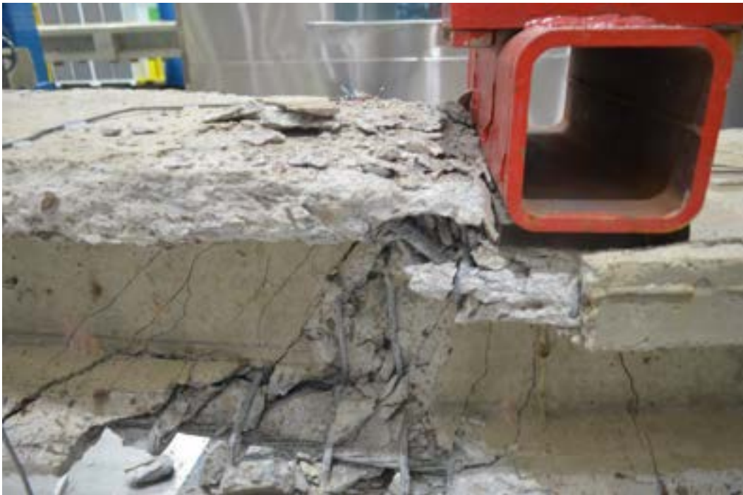
Figure 7.3-75 Debonding of CFCC strands and spalling of concrete at midspan of Beam H1
