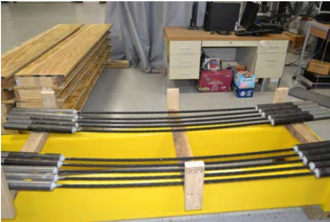
Figure 4.3-2 CFCC specimens prepared to evaluate the transfer length
