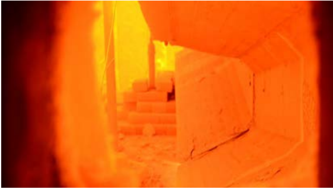
Figure 6.3-43 Beam T-0.7C during fire test
