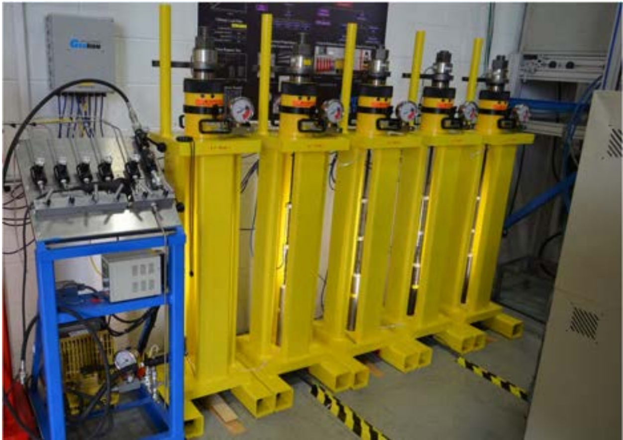
Figure 3.3-1 Test setup for evaluating relaxation of CFCC strands
