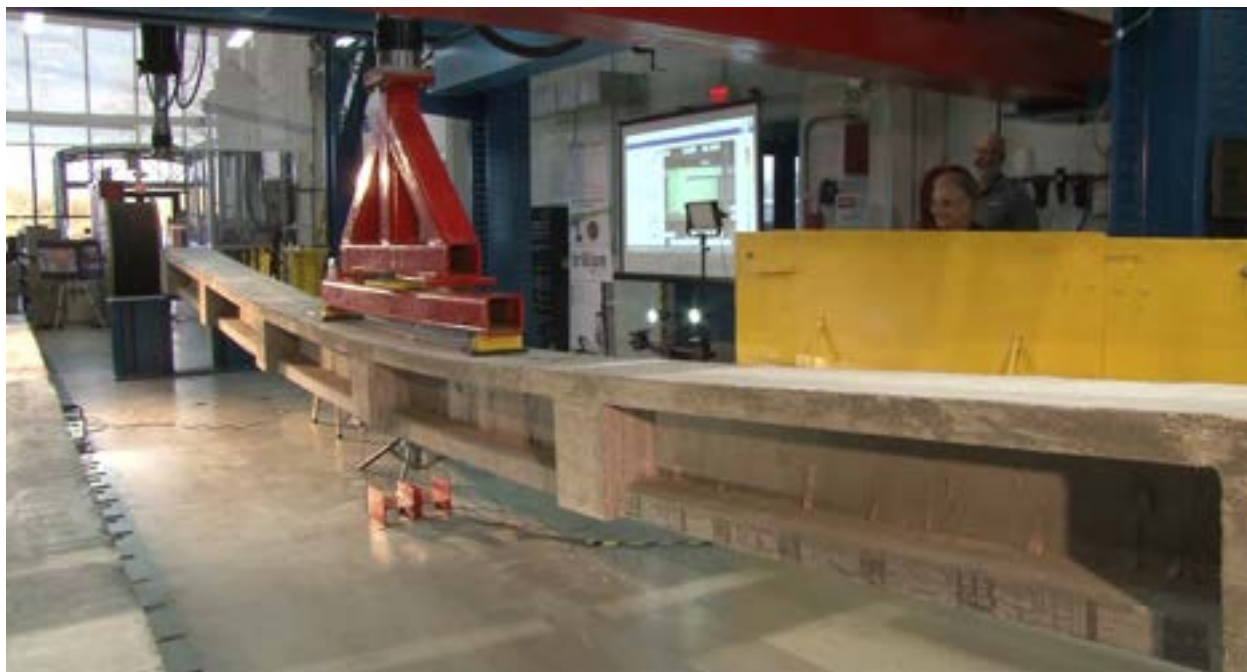
Figure 8.7-4 Deflection of control beam during 24-kip (107-kN) load cycle
