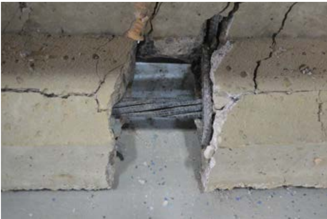
Figure 7.3-69 Debonding of CFCC strands and spalling of concrete at midspan of Beam F2
