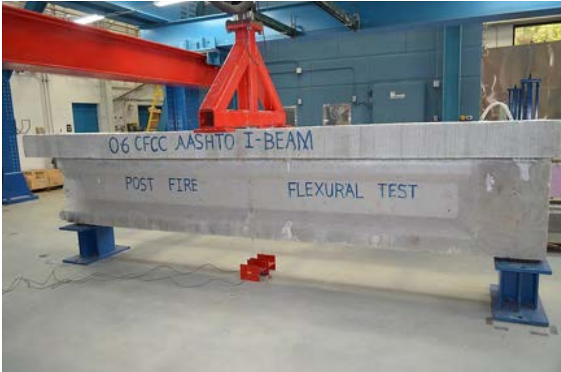
Figure 6.3-100 Flexural test setup for Beam RI-0.6C after fire test
