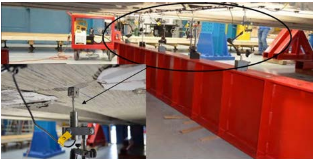
Figure 8.6-4 Attaching Linear Variable Inductive Transducers (LVITs) at the soffit of the bridge
