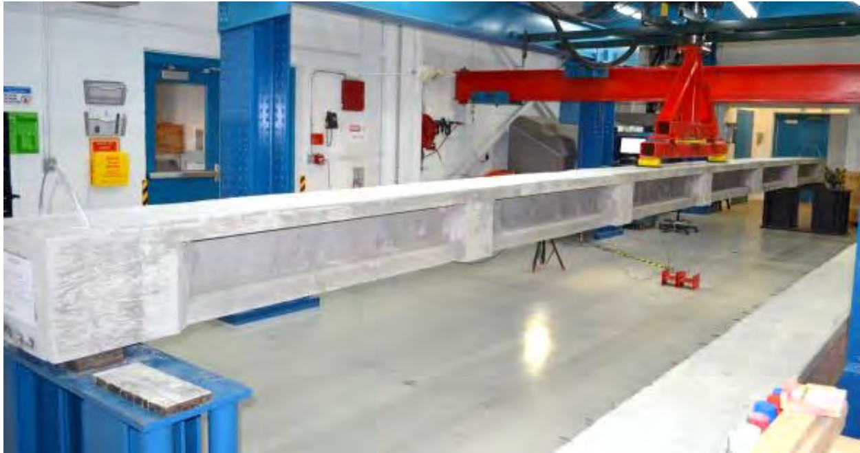
Figure 8.7-1 Flexural test setup of the control beam
