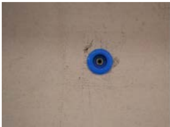
Figure 6.3-20 Installation of the sleeve and the RH Probe sensor
