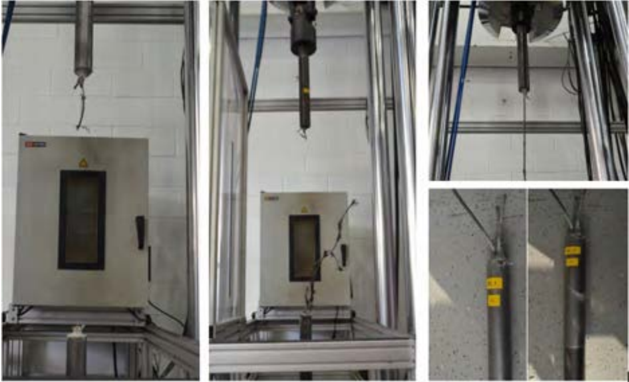
Figure 2.4-7 Typical failure mode of CFCC specimens with sleeve type anchorage
