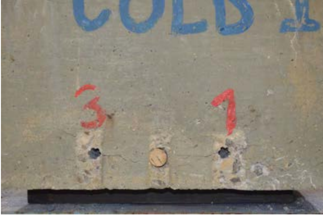
Figure 7.3-64 End view showing slippage of CFCC strands in Beam F1 at maximum load
