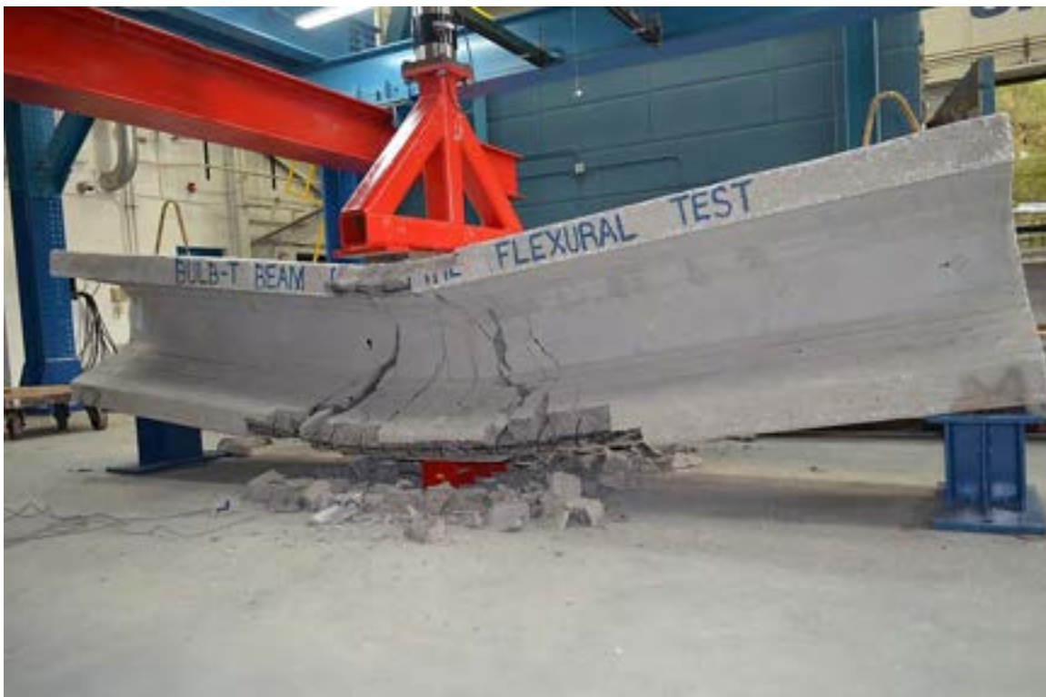
Figure 6.3-89 Failure of Beam RT-0.7C after flexural test
