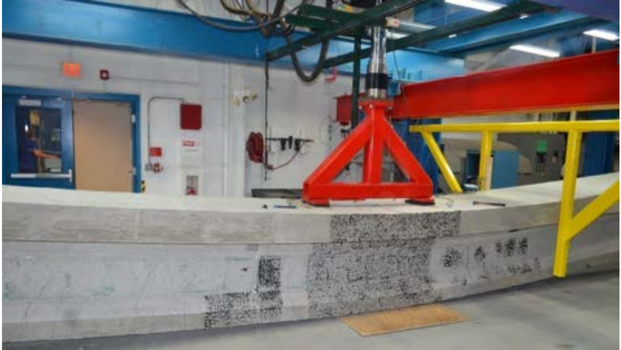
Figure 5.5-3 Tension failure of Beam C0.7
