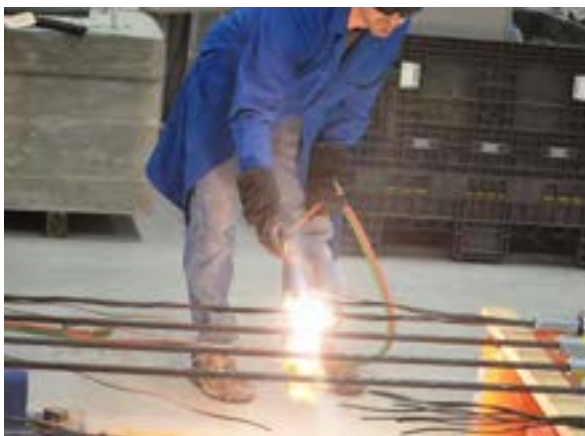
Figure 6.3-13 Transfer of prestressing force into concrete
