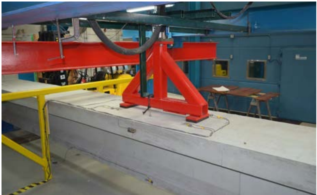
Figure 5.4-3 Close up view showing the instrumentation for testing of AASHTO I-beams
