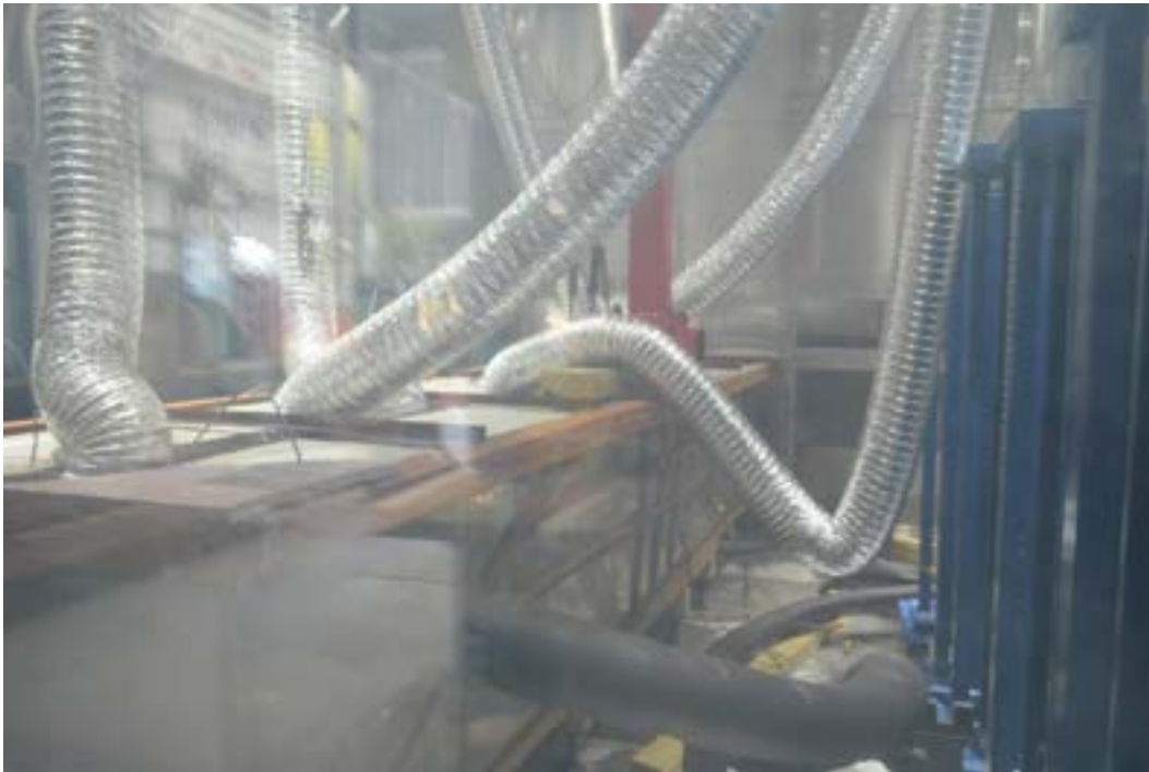
Figure 7.3-36 Decked bulb T beam placed in the tank for freeze-thaw testing
