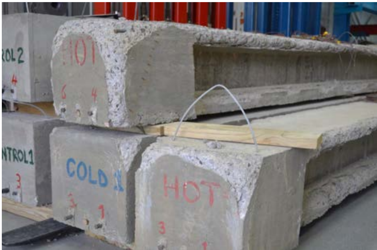
Figure 7.3-48 Decked bulb T beams after exposure to 300 freeze-thaw cycles
