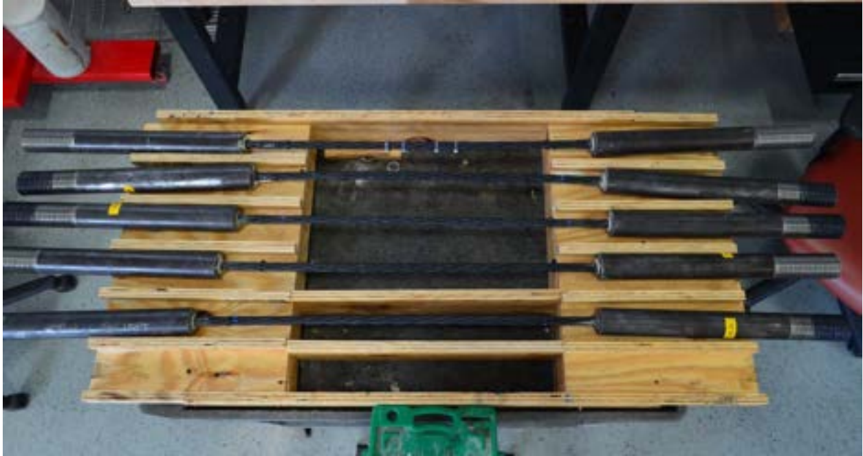
Figure 2.4-5 CFCC specimens with sleeve anchorage device after curing
