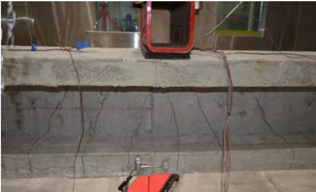
Figure 7.3-20 Development of flexural cracks in Beam F1 after load cycles
