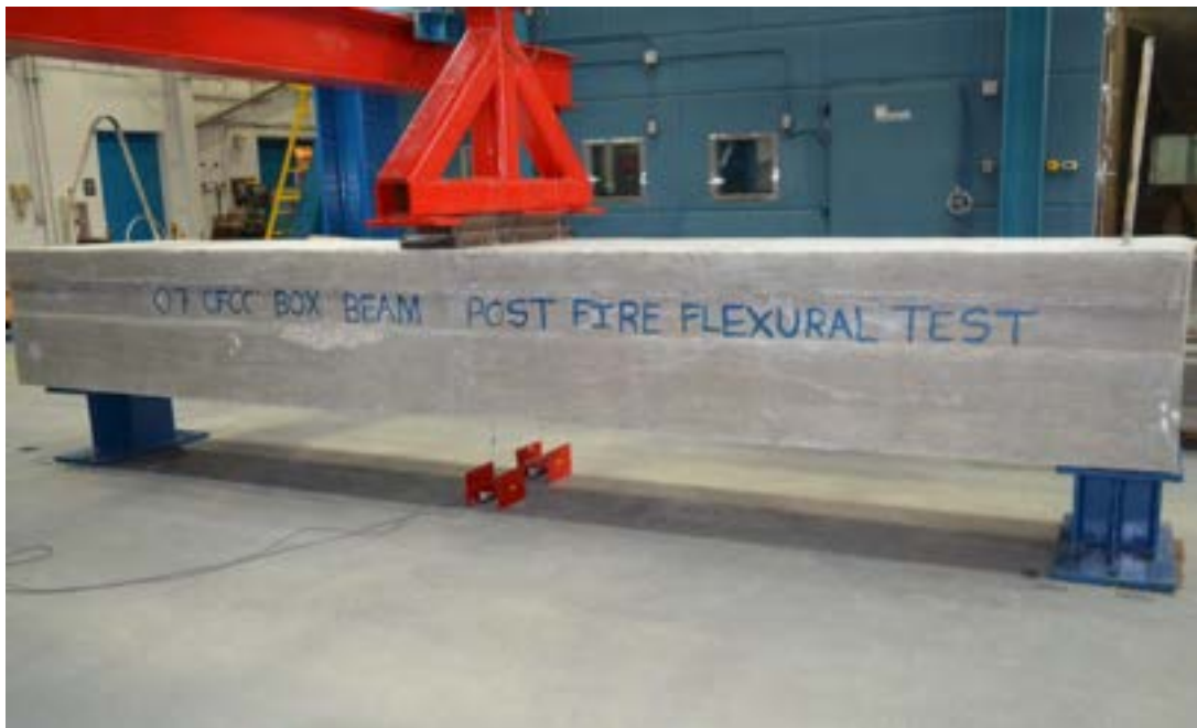
Figure 6.3-75 Test setup of Beam RB-0.7C after fire/loading event
