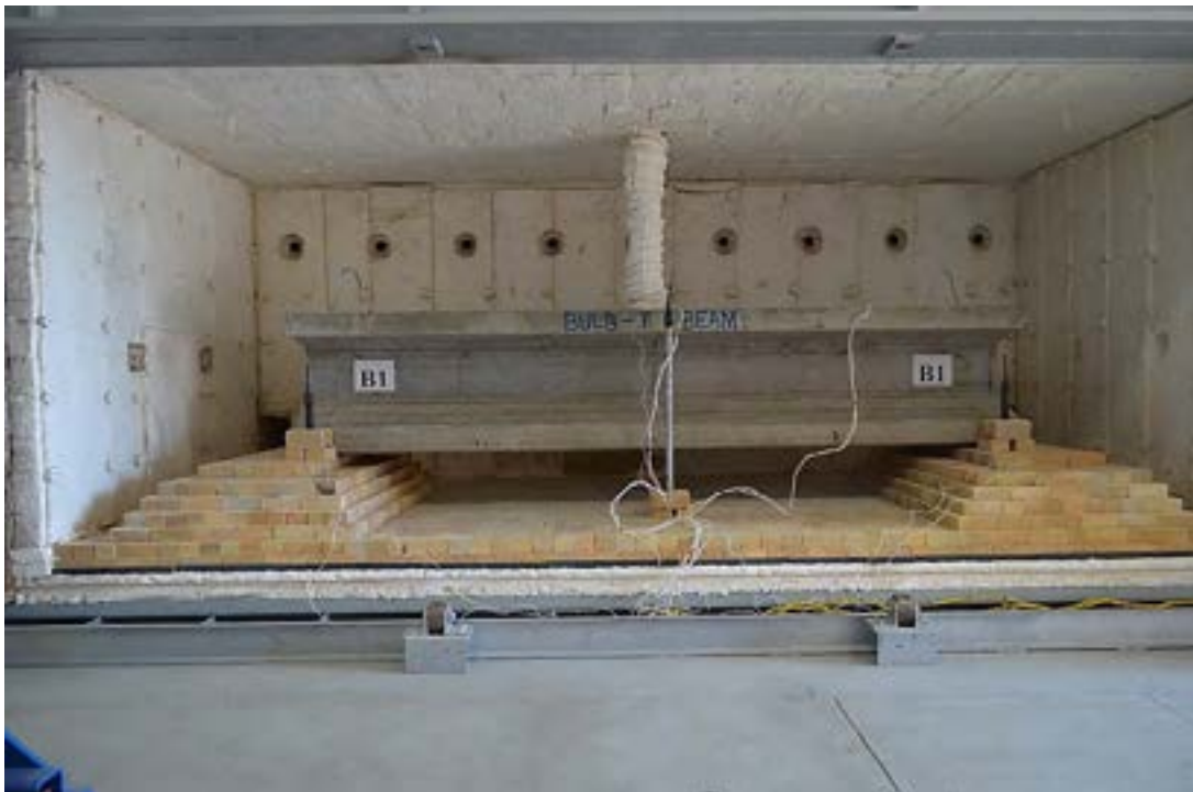
Figure 6.3-83 Beam RT-0.7C before one-hour fire test
