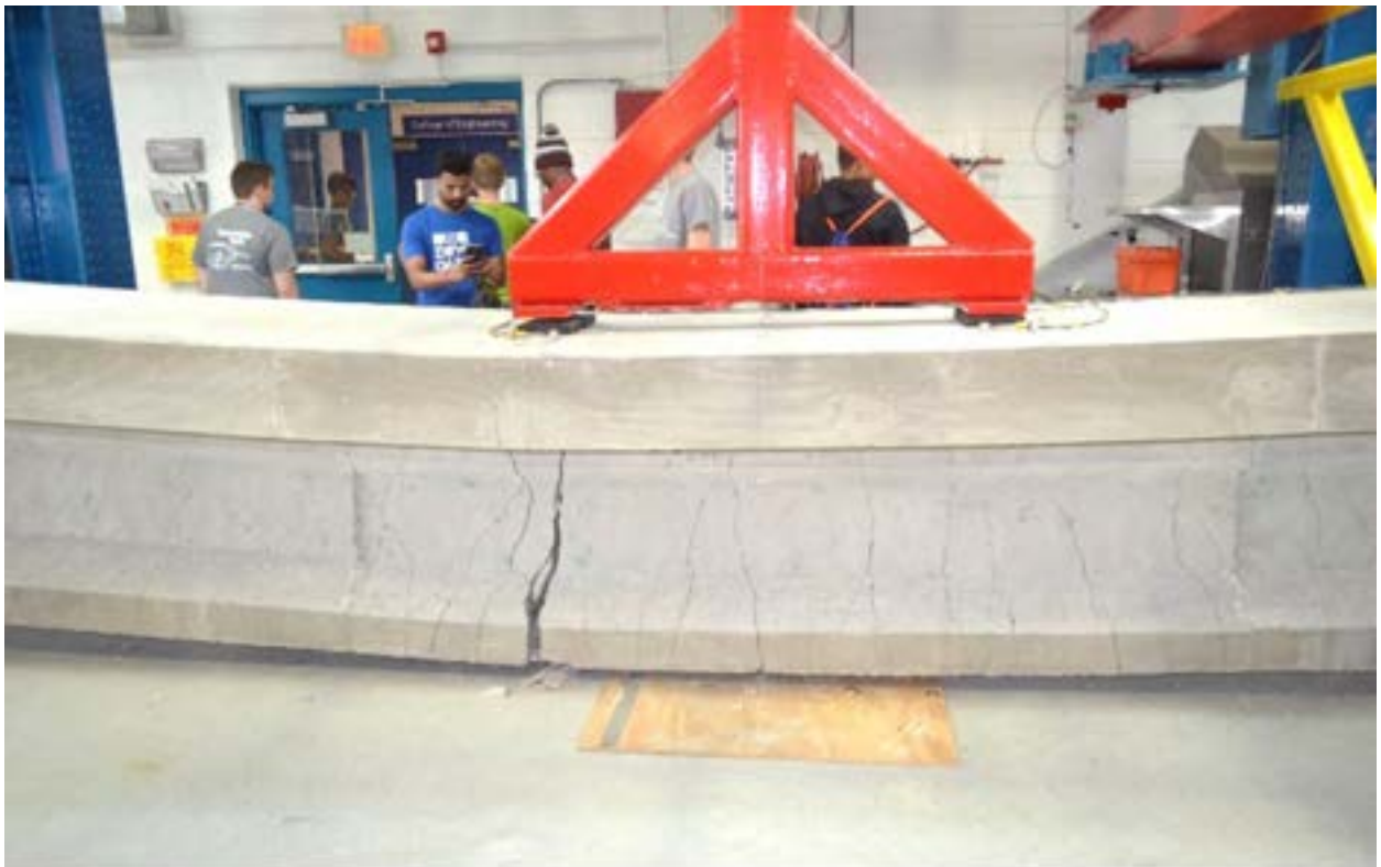
Figure 5.5-10 Tension failure of Beam C0.6
