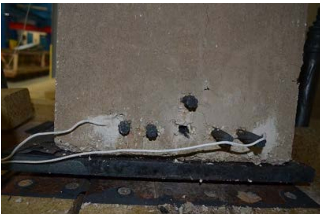
Figure 6.3-64 Steel strands remained bonded to concrete after testing of I-0.6S
