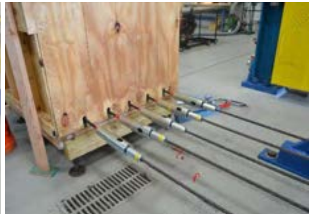
(b) Pulling 0.7 in. (17.3 mm) CFCC strands
