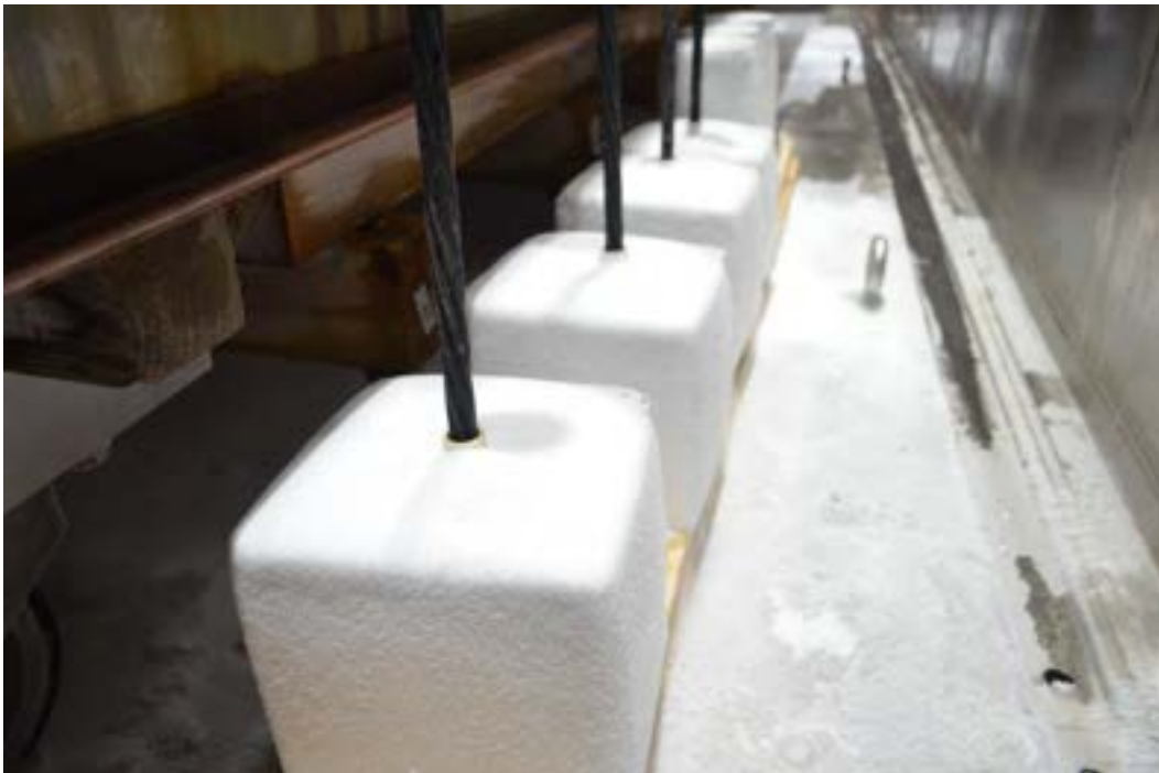
Figure 4.2-20 Pullout test specimens with 0.7" CFCC strands under freeze-thaw cycles
