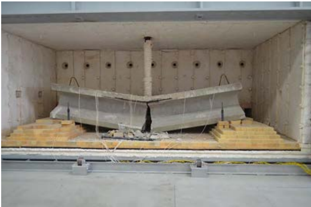
Figure 6.3-44 Beam T-0.7C after fire test
