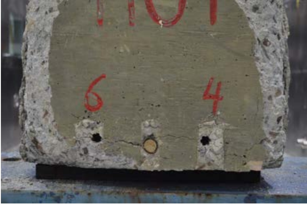
Figure 7.3-82 End view showing slippage of CFCC strands in Beam H2 after failure
