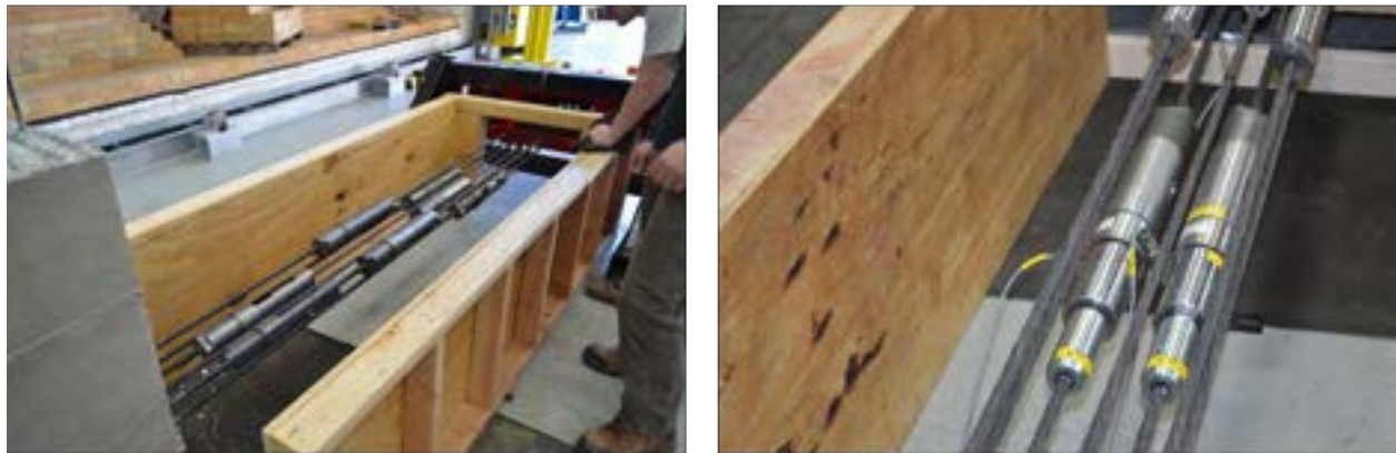
Figure 5.3-2 Live and dead-end anchorage set-up with load cells attached to the dead end
