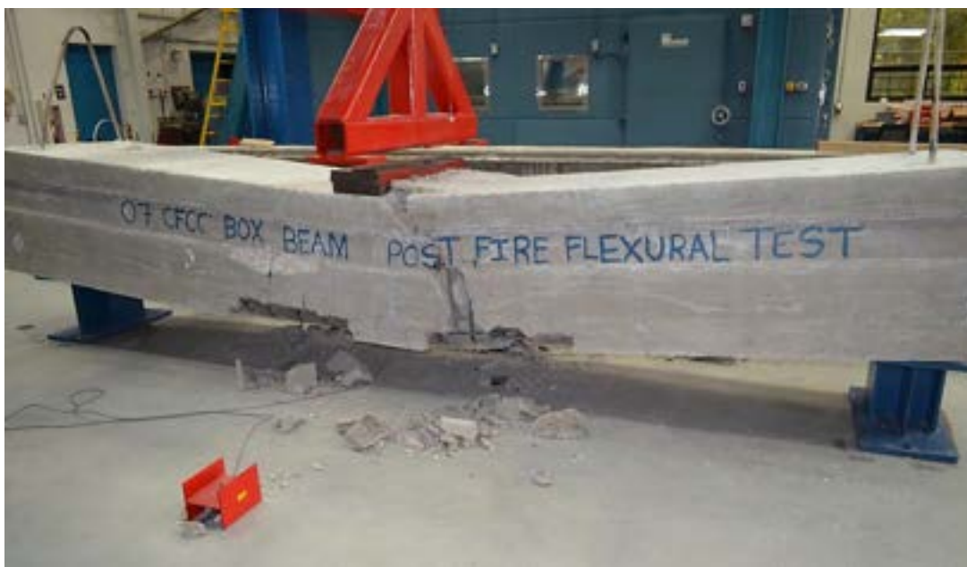
Figure 6.3-76 Failure of Beam RB-0.7C
