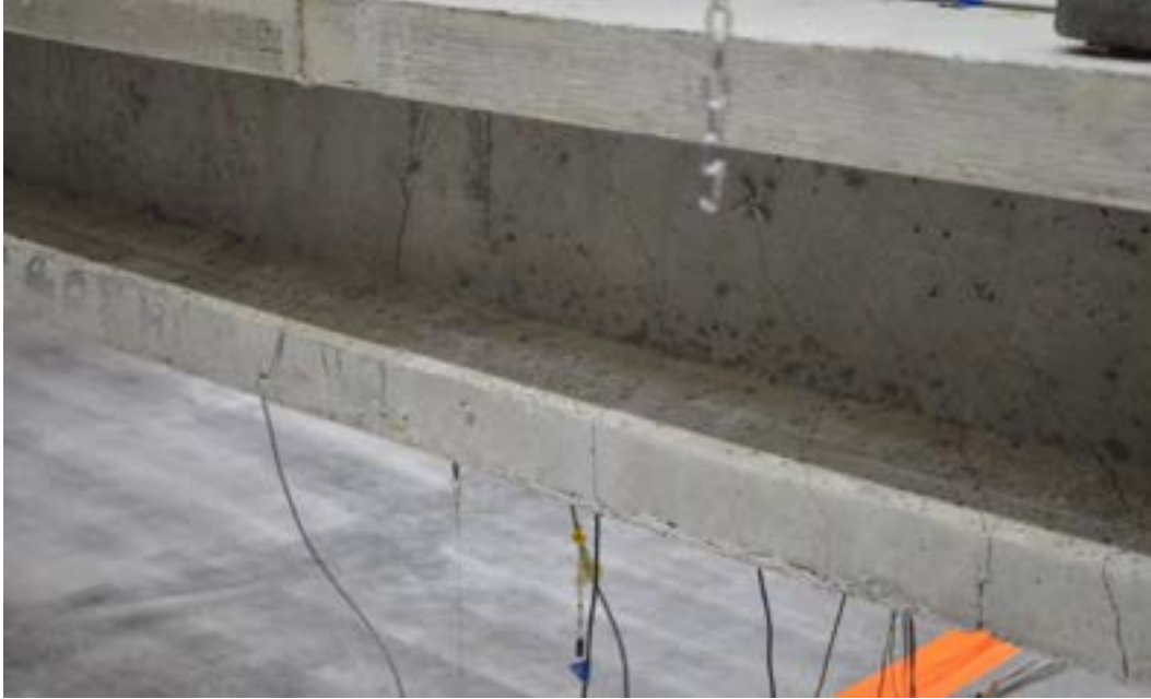
Figure 7.3-29 Development of flexural cracks in Beam H2 after load cycles
