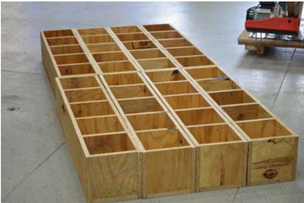
Figure 4.2-2 Preparing the formwork for the test specimens
