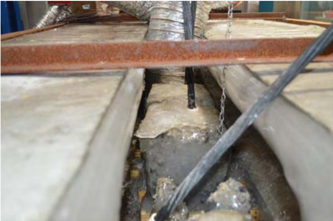
Figure 7.3-42 Freeze-thaw cycles caused deterioration of the concrete cylinders and pullout specimens (picture taken after 150 cycles)
