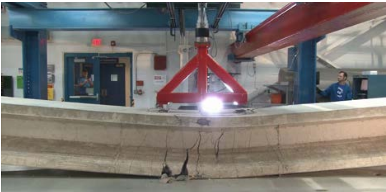
Figure 5.7-5 Failure of bulb T beam due to rupture of CFCC prestressing strands
