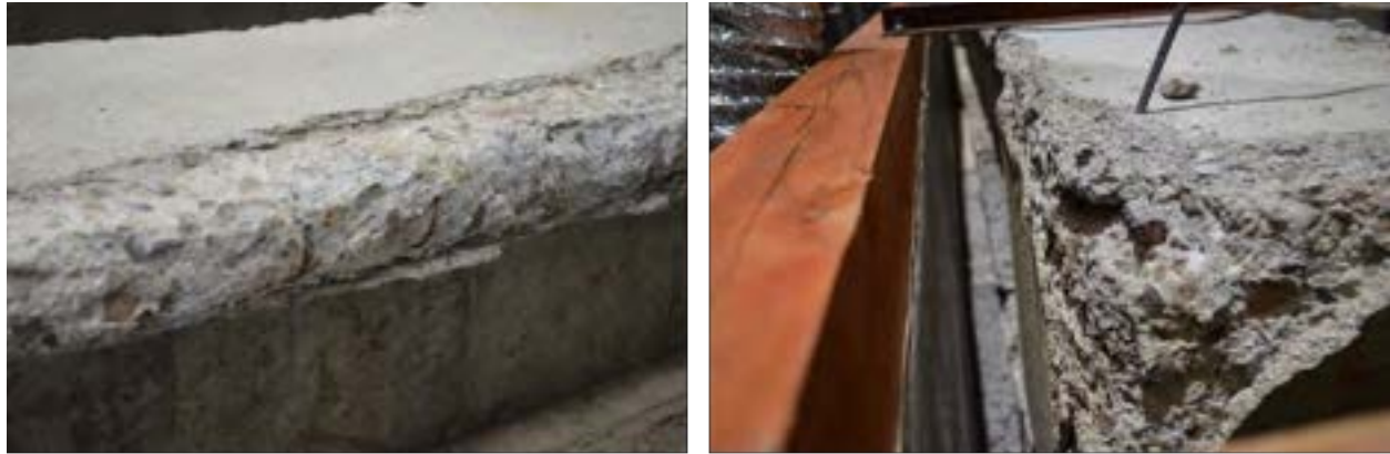
Figure 7.3-47 Deterioration of beam edges due to 300 freeze-thaw cycles
