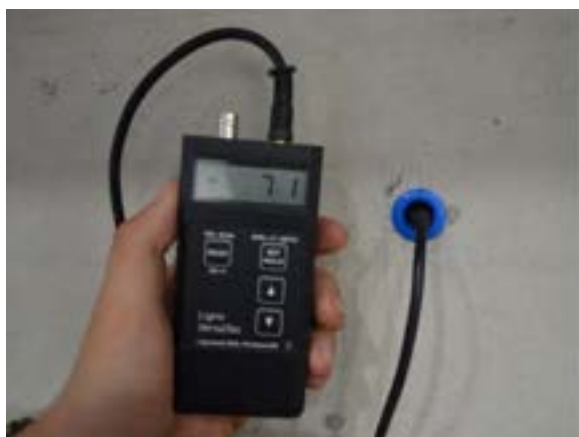
Figure 6.3-21 Obtaining humidity and temperature readings with the moisture meter
