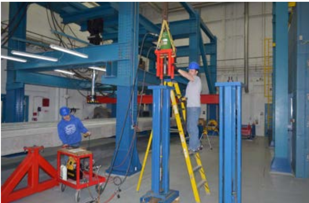
Figure 7.3-32 Stressing CFCC strands for high temperature evaluation
