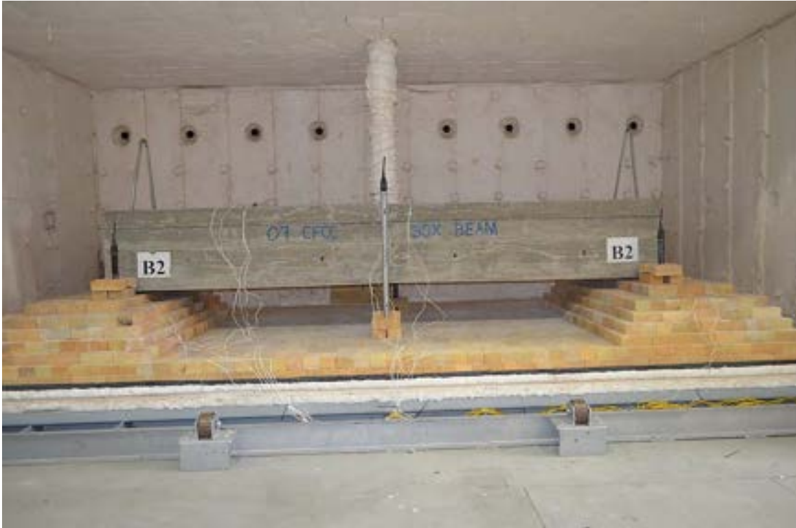
Figure 6.3-71 Beam RB-0.7C before fire test
