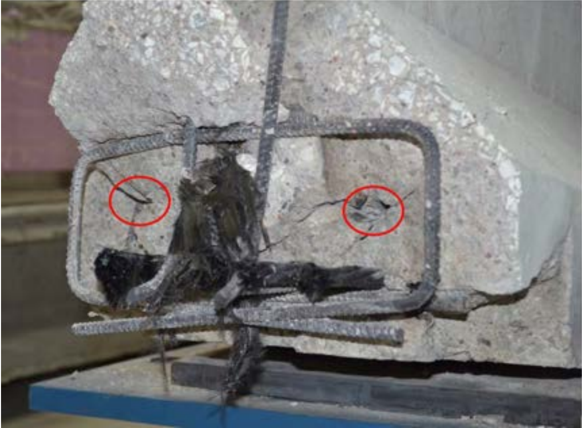
Figure 6.3-103 Rupture and slippage of CFCC strand at failure
