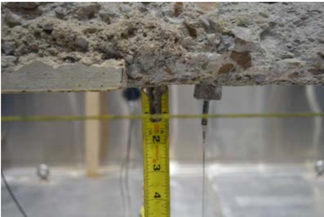
Figure 7.3-79 Midspan camber of 1.0 in. (25.4 mm) in Beam H2 before flexural testing
