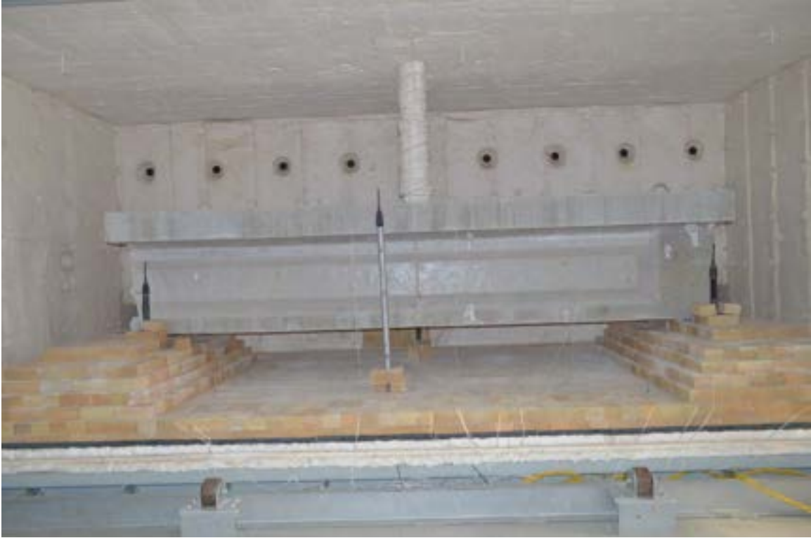
Figure 6.3-97 Beam RI-0.6C after one-hour fire test
