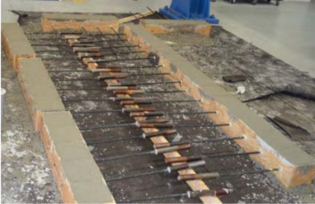
Figure 4.2-5 Pullout specimens ready for curing
