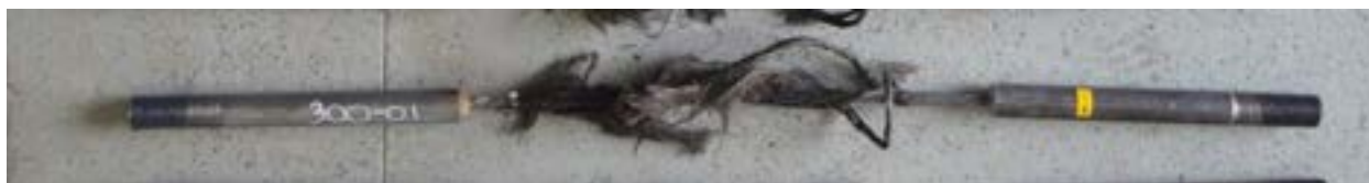
Figure 6.2-12 Failure of CFCC specimen at 572 °F (300 °C)
