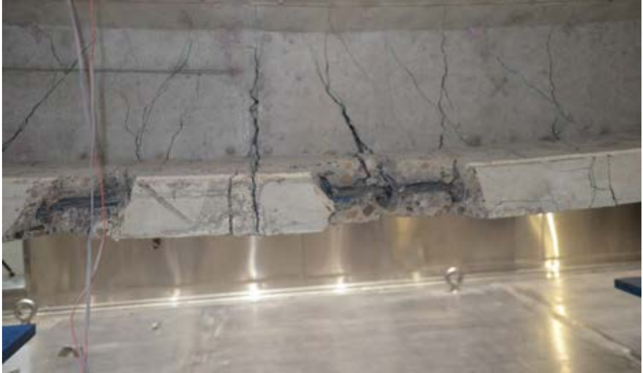
Figure 7.3-54 Debonding of CFCC strands in Beam C1
