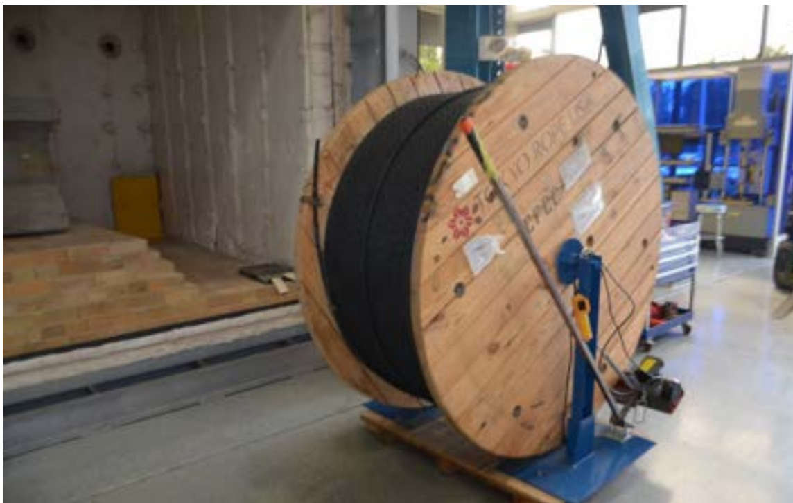
Figure 2.2-1 Spool of CFCC strands with a diameter of 0.7" (17.3 mm)
