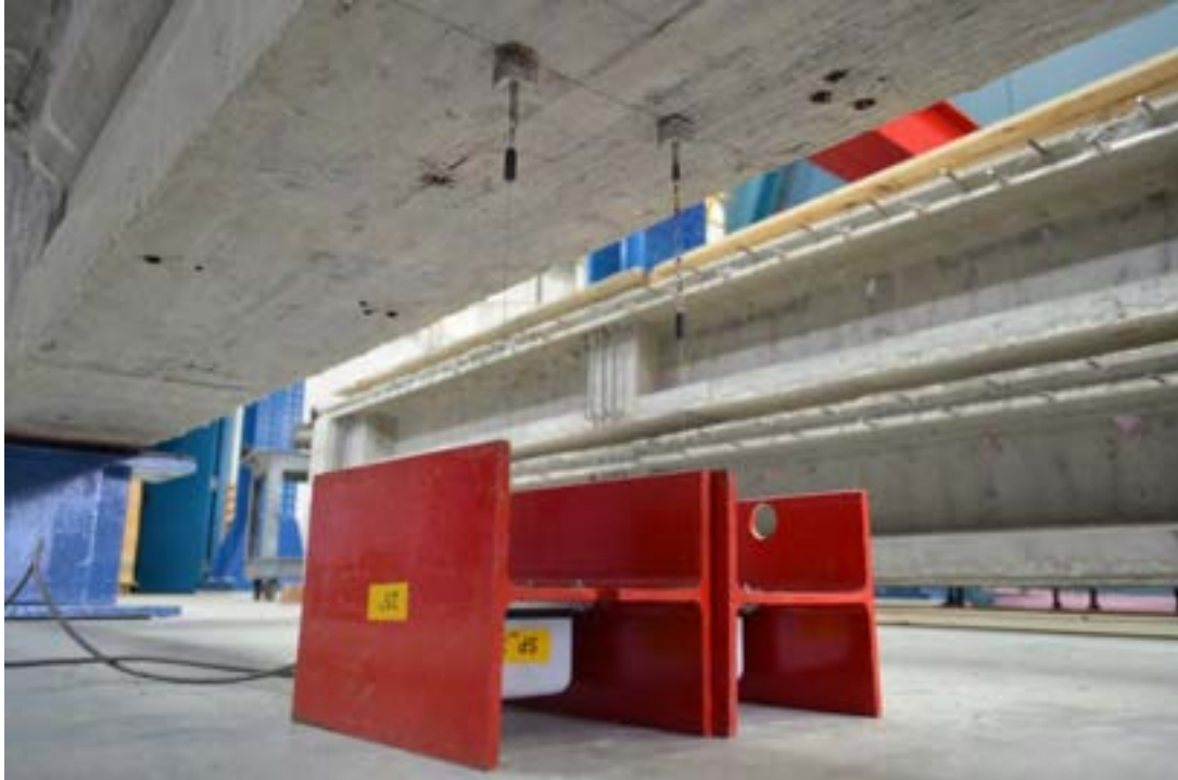
Figure 6.3-66 Installation of String Pot. at the soffit of the beam
