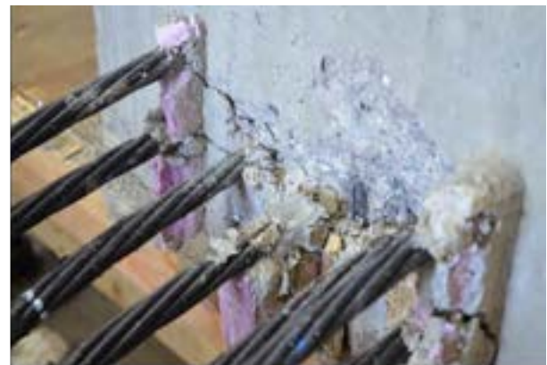
Figure 5.3-7 Completed Beam C0.6 after prestress transfer with minor cracks at the beam end
