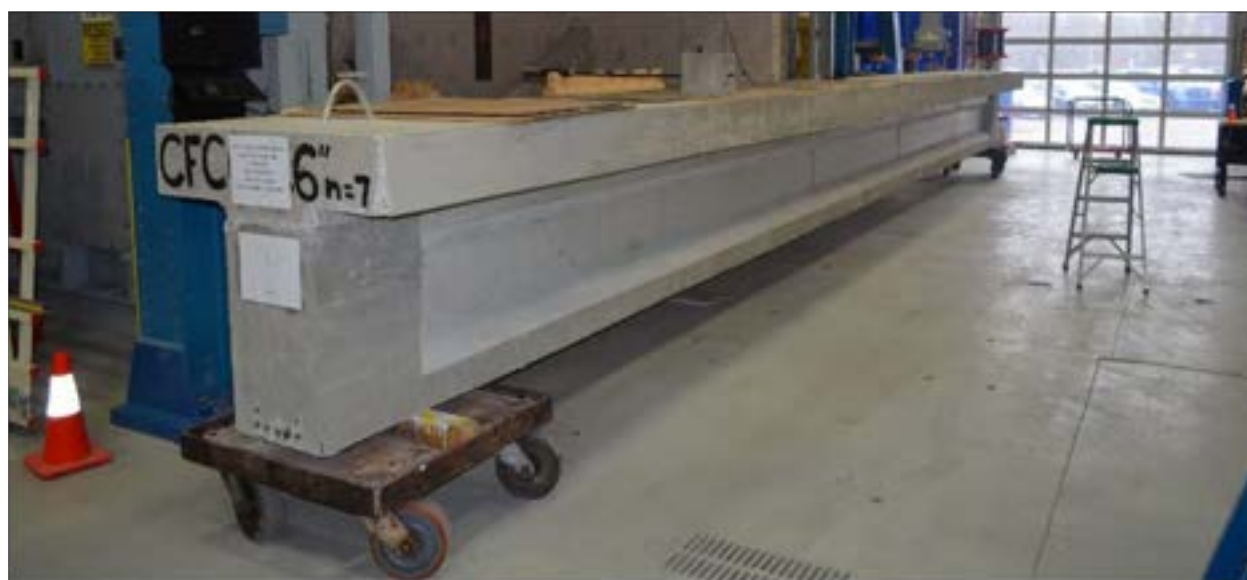
Figure 5.3-11 AASHTO I-Beam C0.6 with a cast-in-place slab after construction
