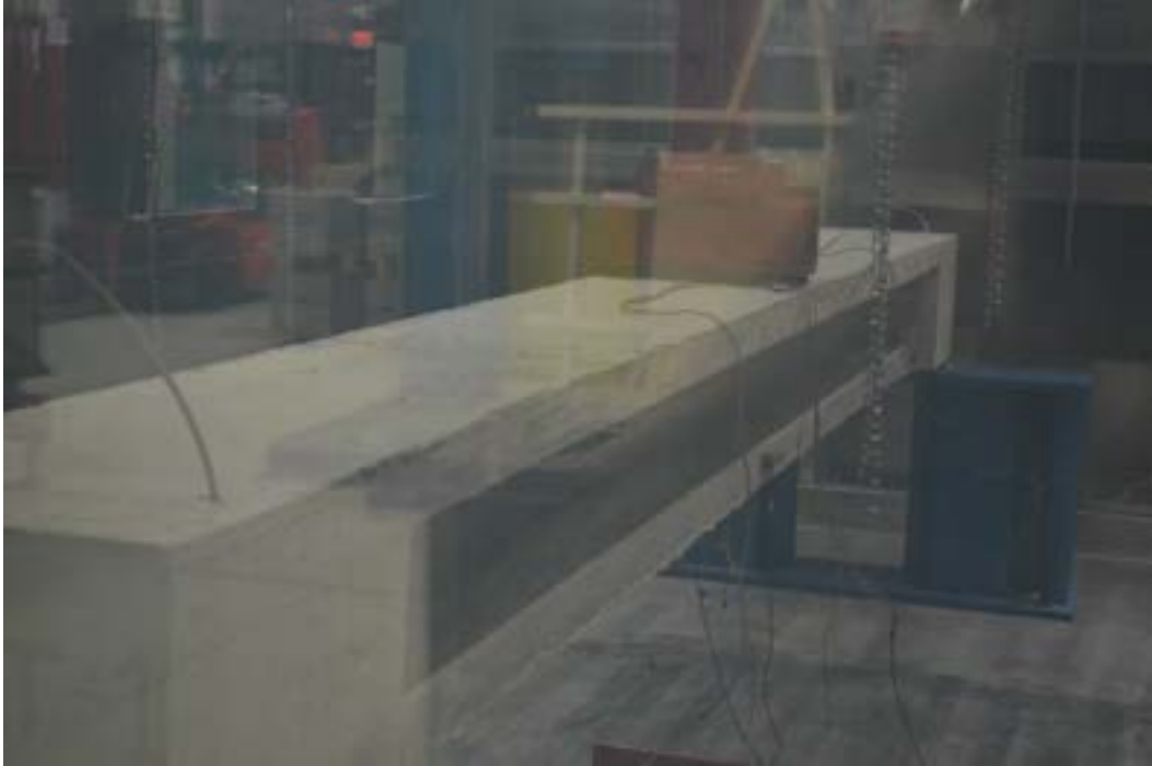
Figure 7.3-25 Beam H1 under three-point loading in the environmental chamber
