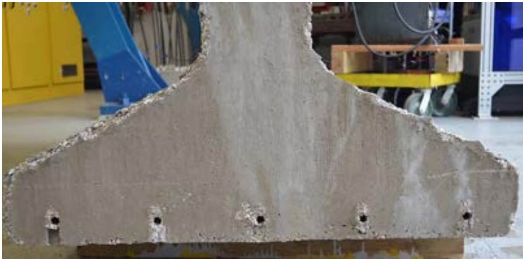
Figure 6.3-46 Slipped CFCC strands from concrete at failure
