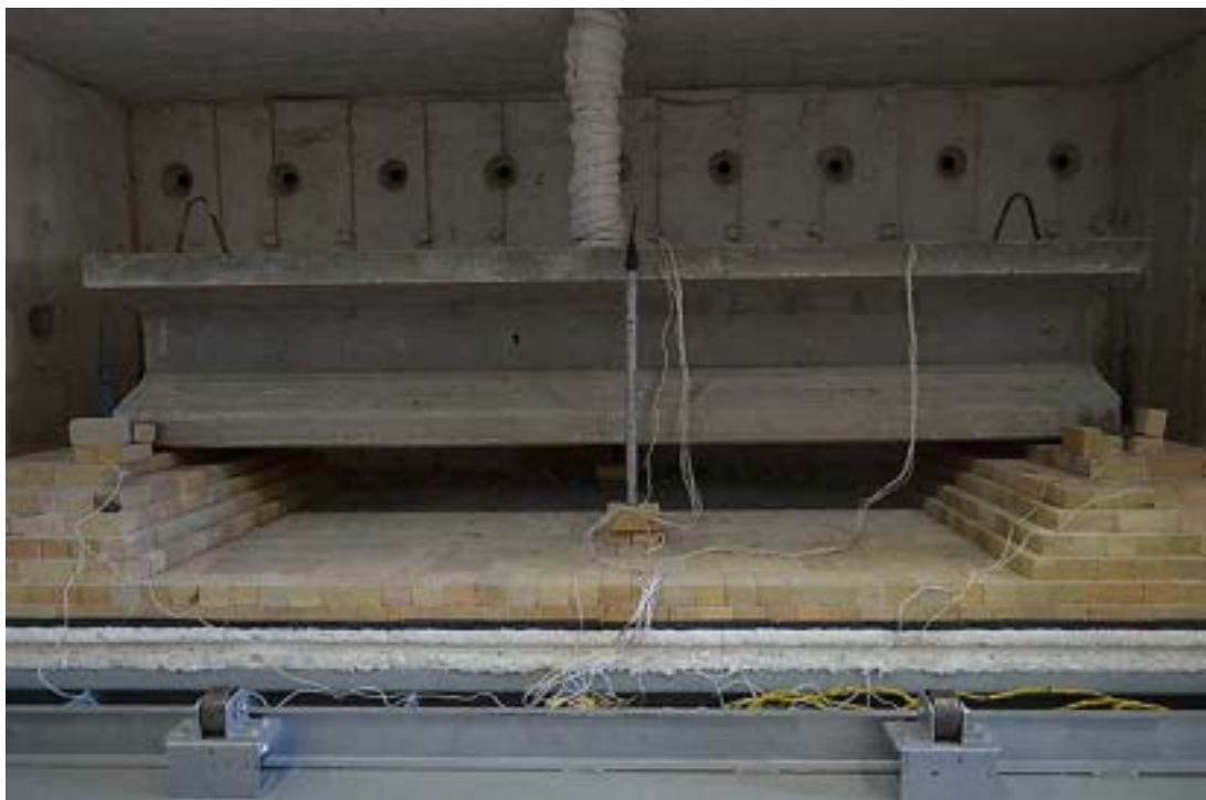
Figure 6.3-85 Beam RT-0.7C after one-hour fire test
