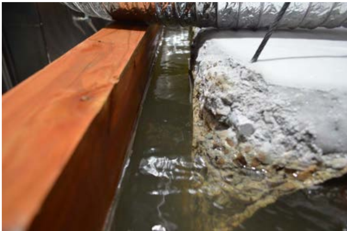
Figure 7.3-46 Concrete corners after exposure to 300 freeze-thaw cycles
