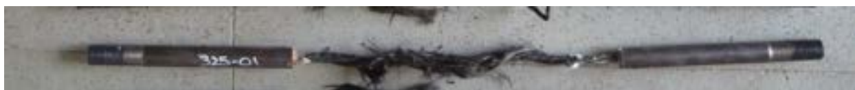
Figure 6.2-13 Failure of CFCC specimen at 617 °F (325 °C)
