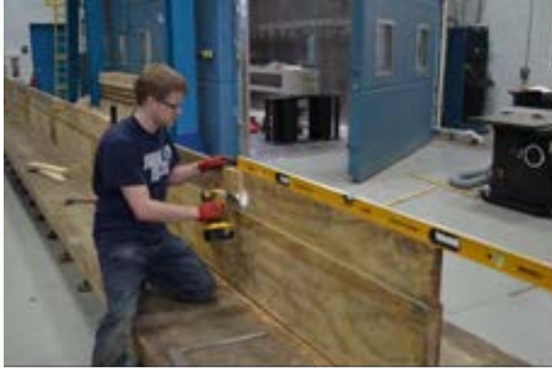
Figure 8.4-1 Setting up the wooden center walls and attaching the Styrofoam to center walls
