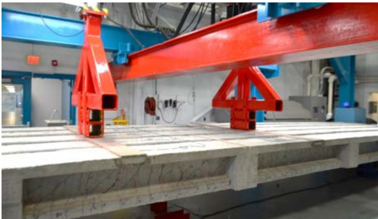
Figure 8.8-17 Four-point loading of the intermediate beam during the strength limit state test
