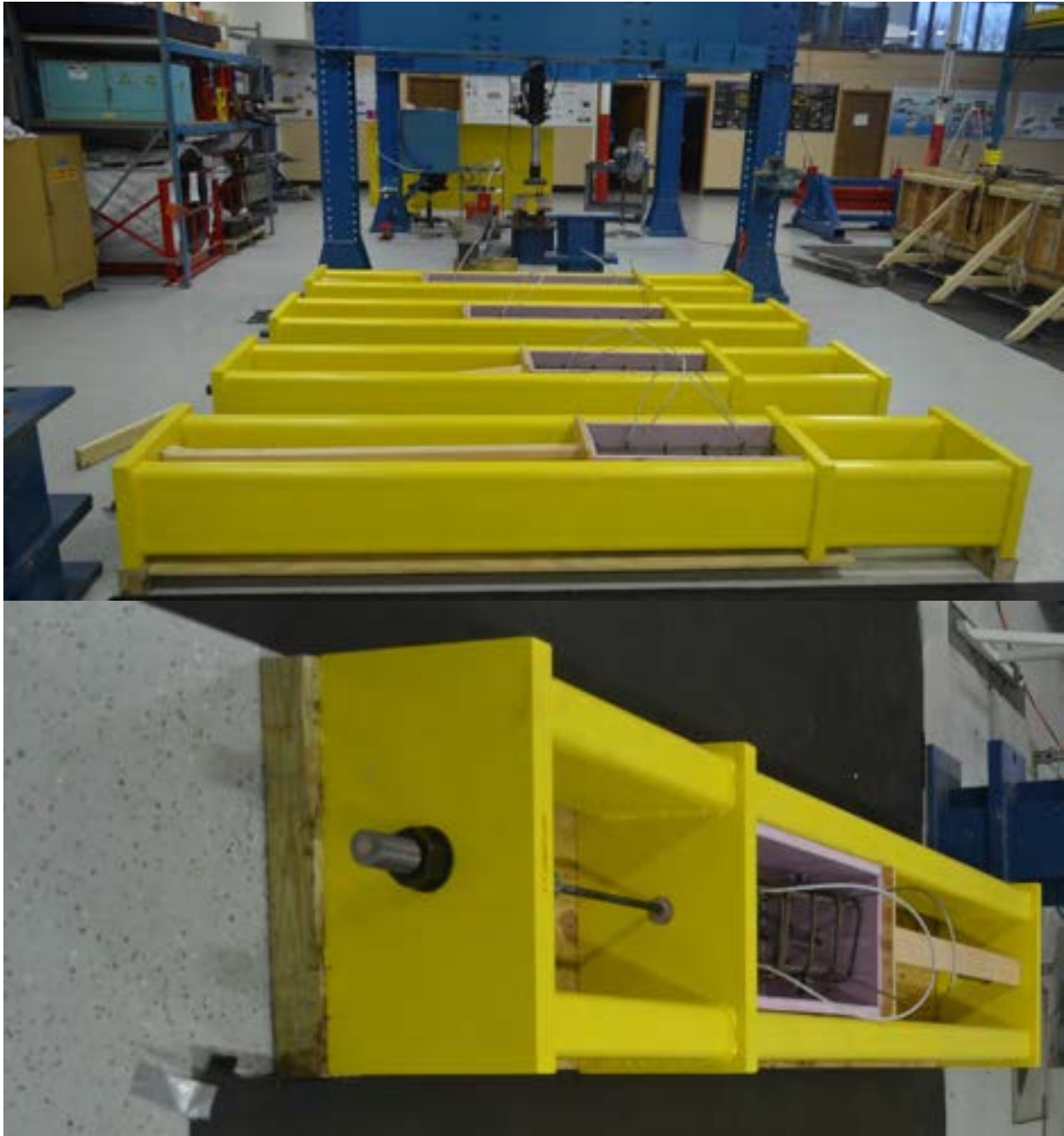
Figure 4.4-5 First set of development length specimens, measuring 12 in. \times 12 in. with lengths of 18, 24, 36, 48, and 60 in. (No. 3 steel stirrups every 6 in.), prior to pouring concrete
