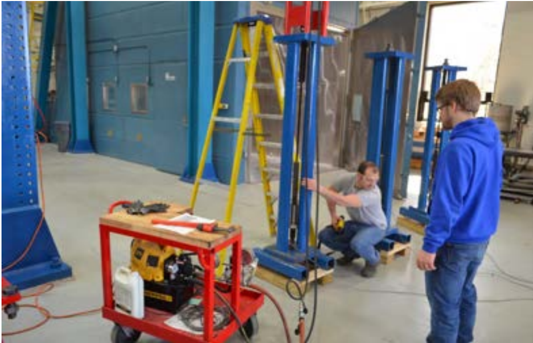
Figure 7.3-31 Preparing unbonded CFCC strands for high temperature evaluation
