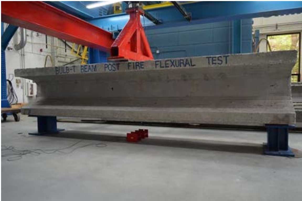
Figure 6.3-88 Test setup for Beam RT-0.7C after fire test
