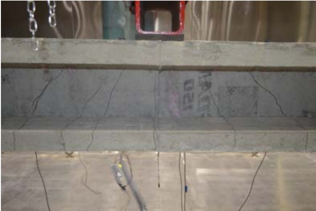
Figure 7.3-23 Development of flexural cracks in Beam F2 after load cycles
