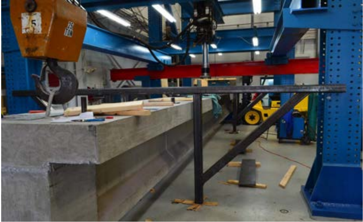
Figure 5.4-2 Construction of lateral steel bracing system
