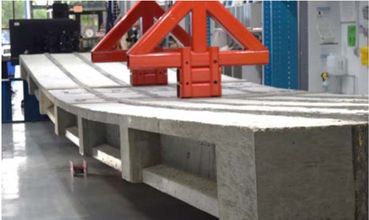
Figure 8.8-18 Deflection of bridge model during strength limit state testing
