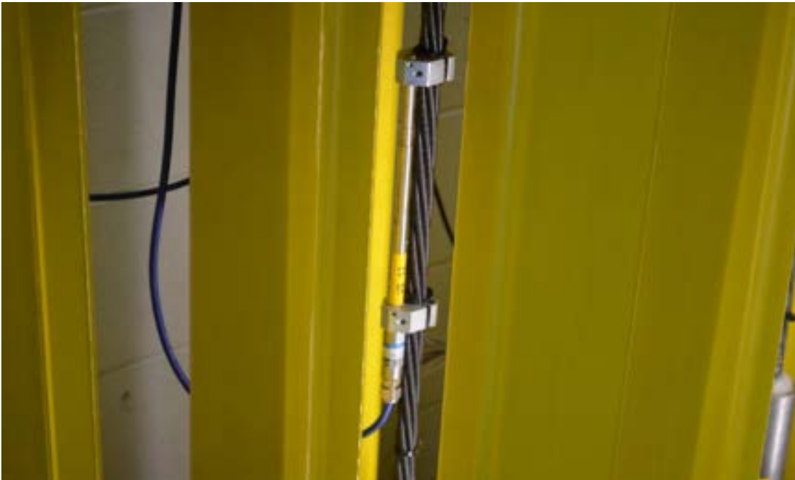
Figure 3.3-3 Strand meters to evaluate the strain in CFCC relaxation specimens
