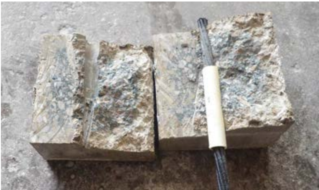
Figure 4.2-14 CFCC strand leaving impression of strand twist on concrete
