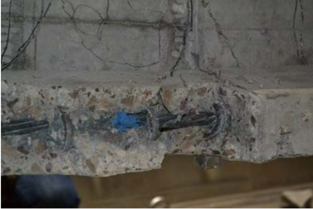
Figure 7.3-58 Debonding of CFCC strands and spalling of concrete at midspan of Beam C2
