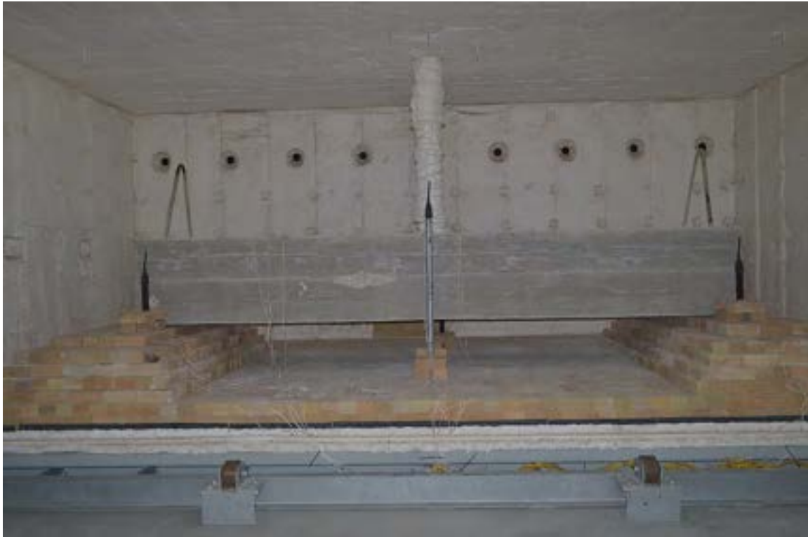
Figure 6.3-73 Beam RB-0.7C after one-hour fire test
