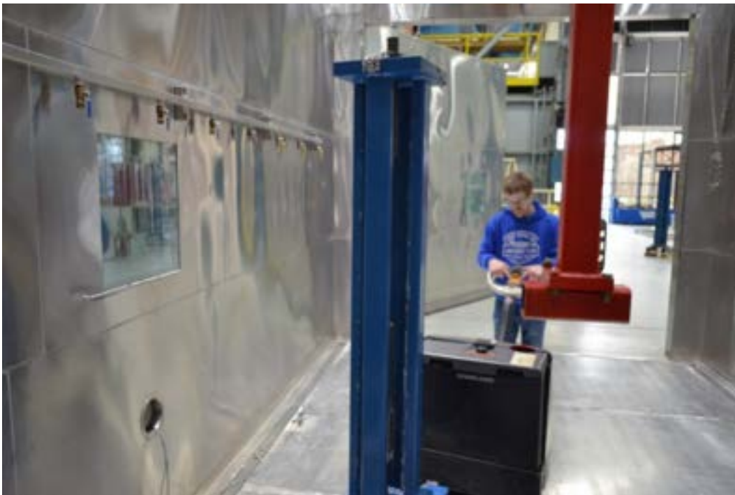
Figure 7.2-8 Placing the stressed CFCC strands in the environmental chamber
