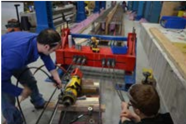
Figure 8.4-5 Prestressing CFCC strands by pulling coupled steel strands using hydraulic pump
