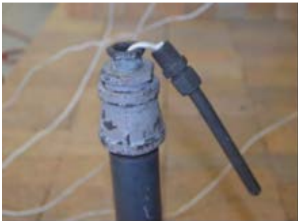
Figure 6.3-24 Measuring air temperature around the beam specimens
