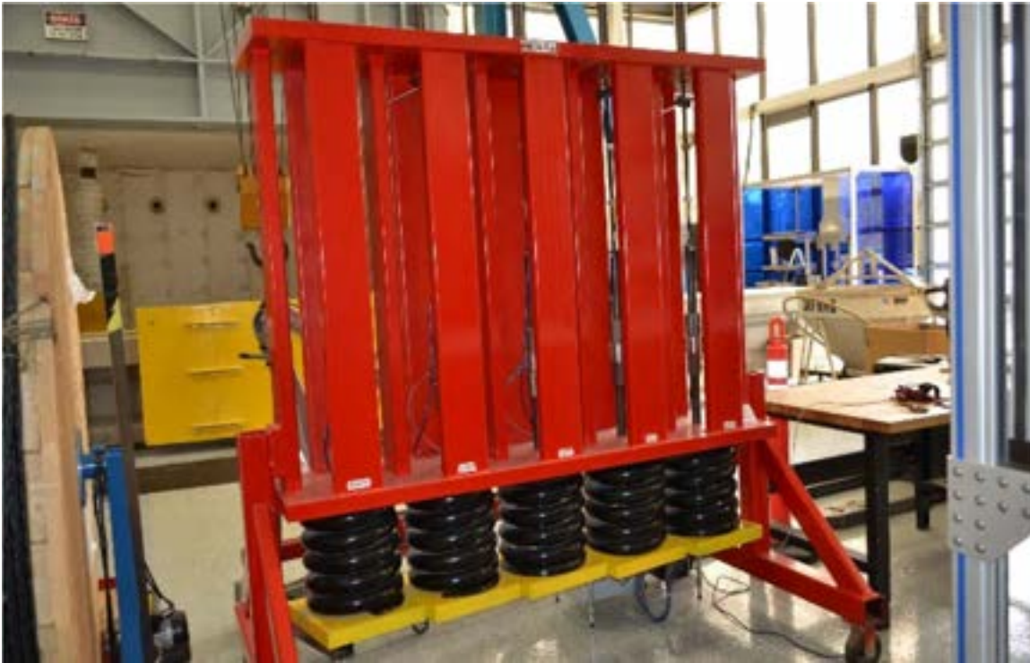
Figure 3.2-1 Creep test setup of 0.6" CFCC specimens with steel springs
