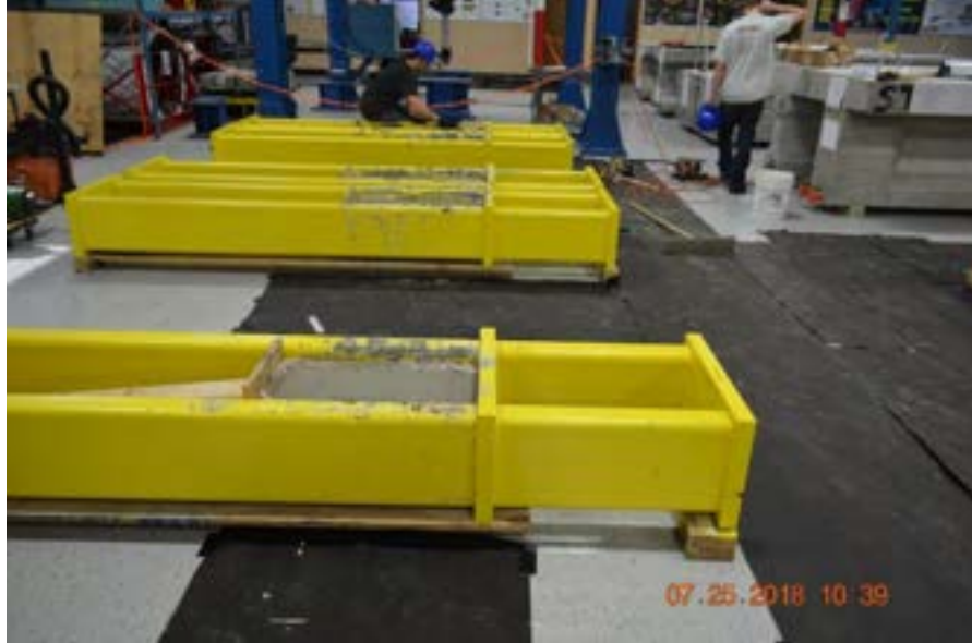
Figure 4.4-7 Third set of development length specimens, measuring 8 in. \times 8 in. with lengths of 24, 30, 36, 42, and 48 in. (no steel stirrups and after pouring concrete)
