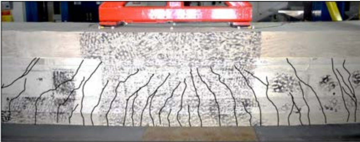
Figure 5.5-1 Development of flexural cracks during flexural loading of Beam C0.7
