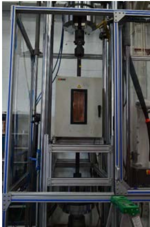
Figure 6.2-3 CFCC strand passing through a central opening in the environmental chamber
