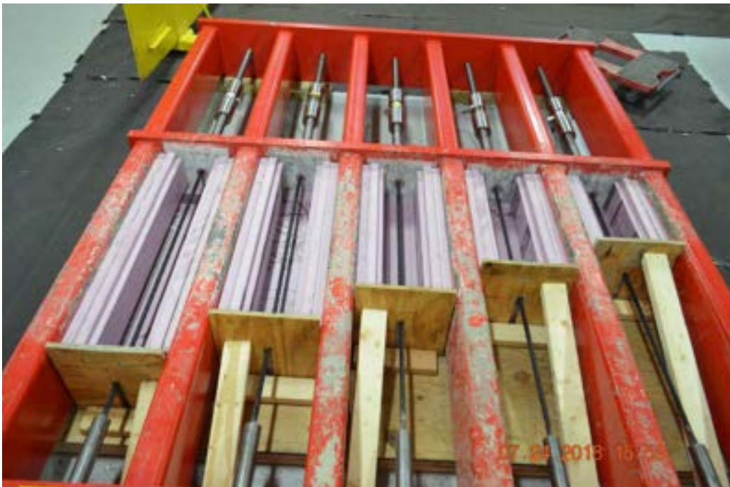
Figure 4.3-10 Third set of transfer length specimens prior to concrete pouring, measuring 6 in. \times 6 in. with lengths of 18, 24, 30, 36, and 42 in. (no steel stirrups)
