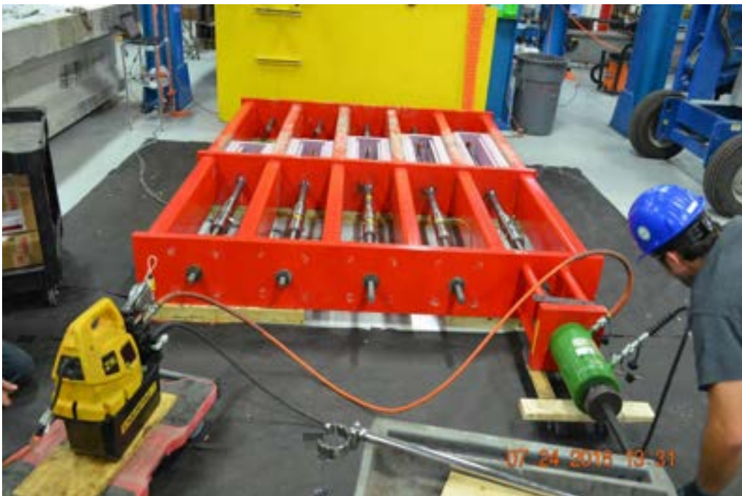
Figure 4.3-6 Stressing CFCC specimens before pouring the concrete
