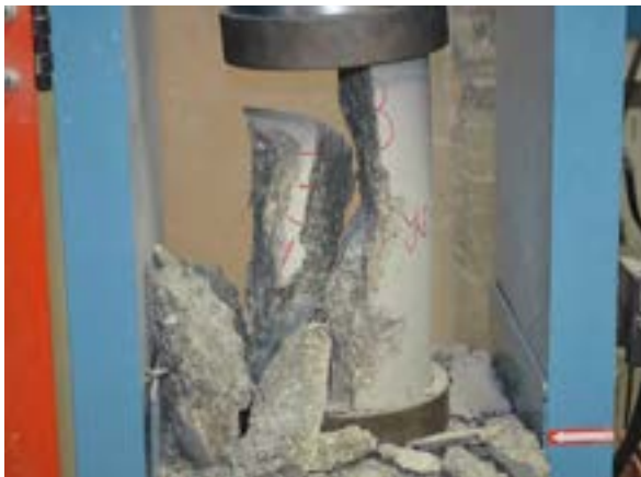
Figure 6.3-12 Uniaxial compressive strength test for concrete
