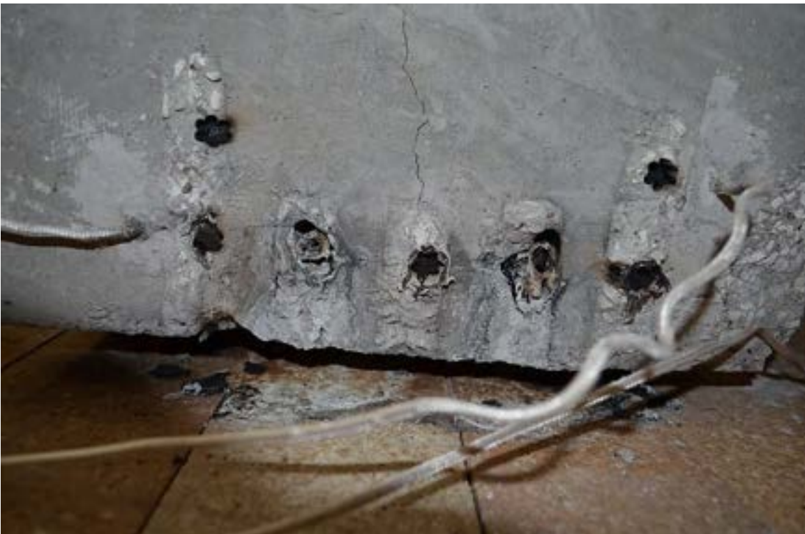
Figure 6.3-98 Close-up look at the end of the beam after fire test
