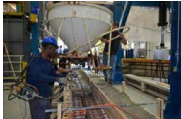
Figure 8.4-6 Placing concrete into the formwork and compacting using electric pencil vibrators
