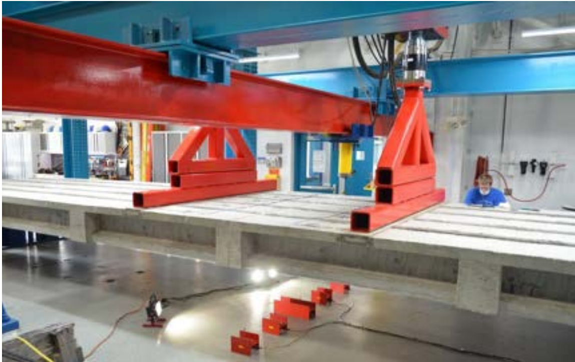
Figure 8.8-7 Four-point loading of bridge model for inducing flexural cracks
