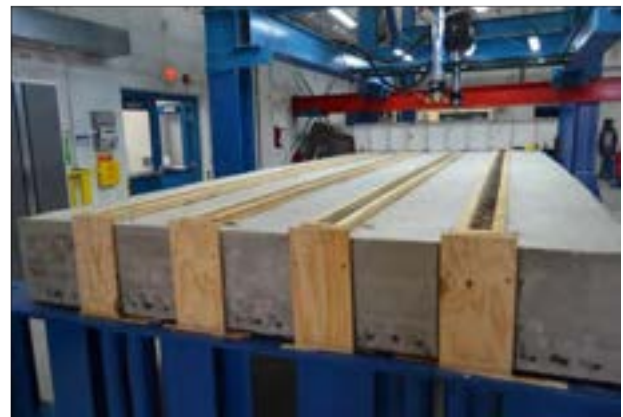
Figure 8.5-7 Beam leveling and wooden end plates at the beam ends
