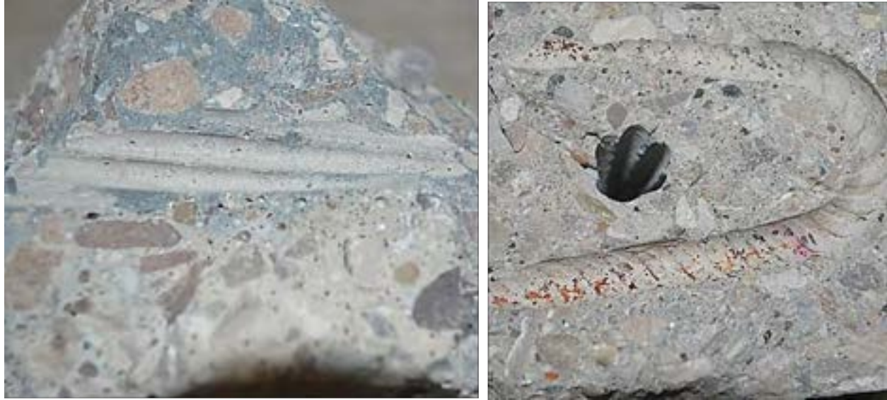
Figure 6.3-92 Strand pattern in concrete
