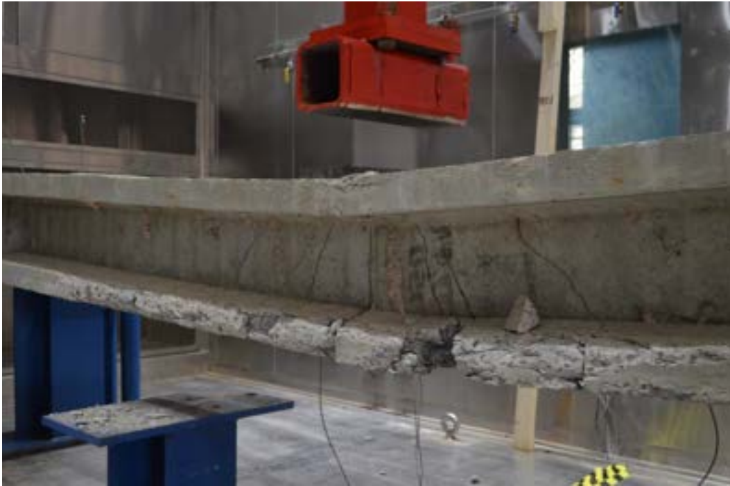
Figure 7.3-68 Failure of Beam F2 under three-point loading
