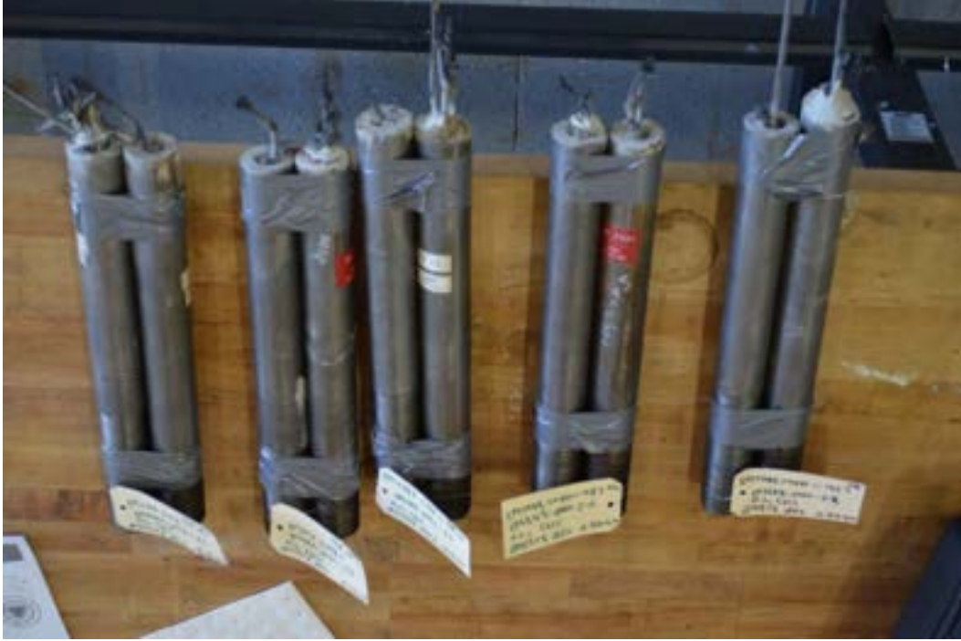
Figure 7.2-13 Failure of CFCC strands under uniaxial tension test
