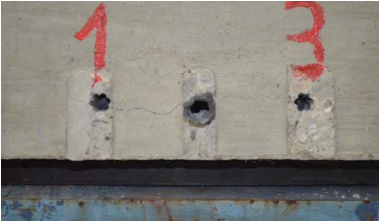
Figure 7.3-55 End view showing the slippage of CFCC strands in Beam C1 at maximum load
