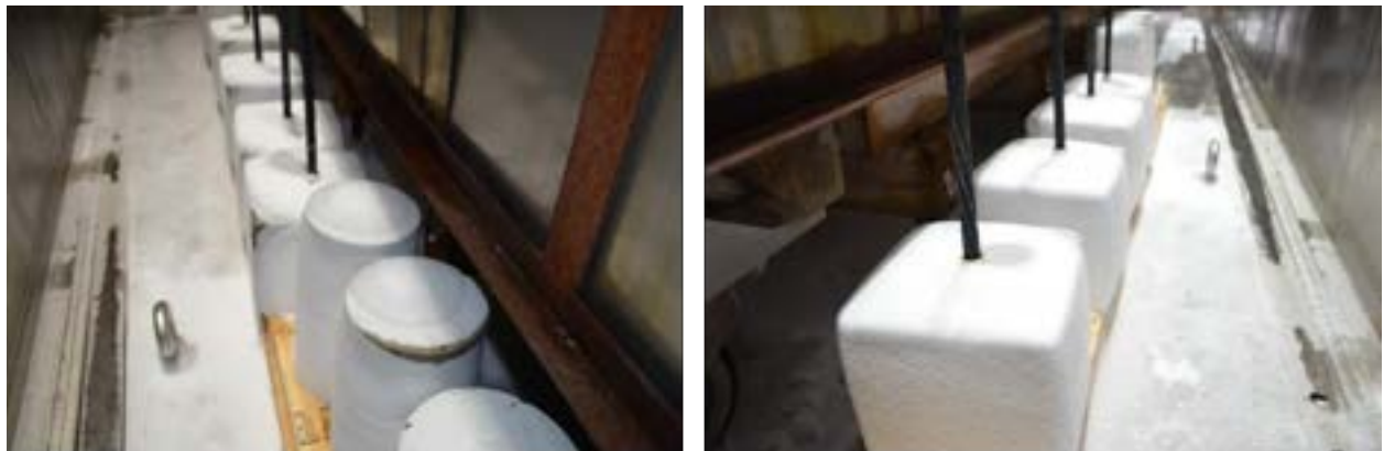
Figure 7.3-44 New cylinders and pullout specimens placed outside the tank after 150 freeze-thaw cycles
