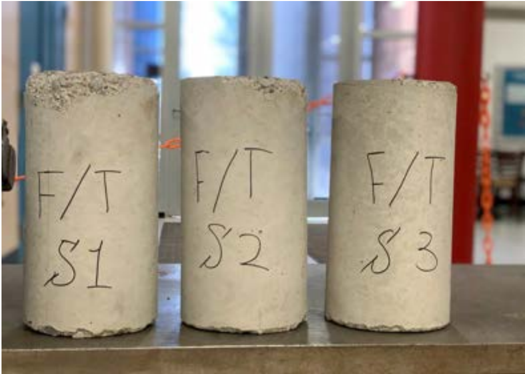
Figure 7.3-49 Concrete cylinders after exposure to 150 freeze-thaw cycles (outside the tank)
