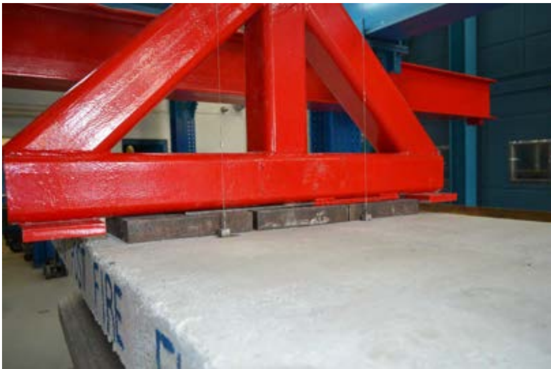
Figure 6.3-67 Installation of String Pot. at the top of the beam
