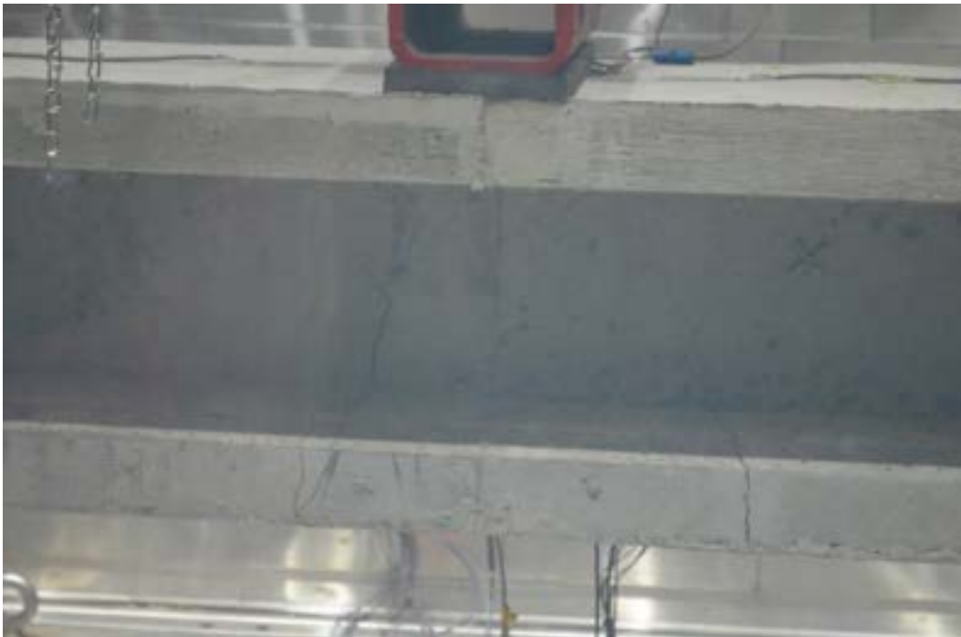
Figure 7.3-26 Flexural cracks during loading Beam H1 at 176 °F (80 °C) after 35-kip (156-kN) load cycle
