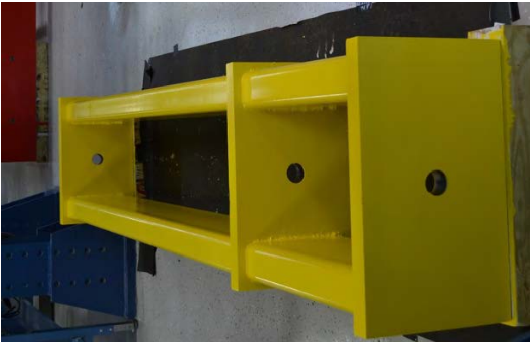
Figure 4.4-4 Development length frame showing access holes for the CFCC strand
