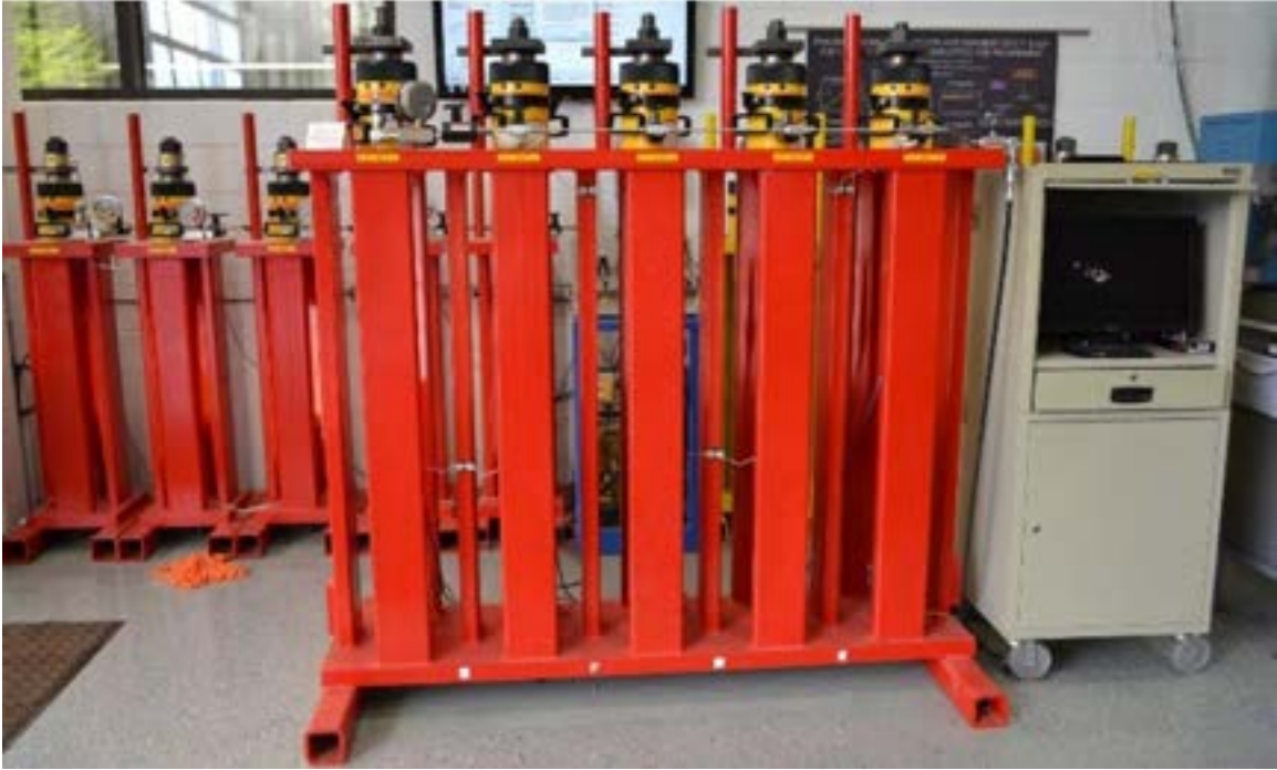
Figure 3.2-2 Creep test setup of 0.6" CFCC specimens with closed loop hydraulic system
