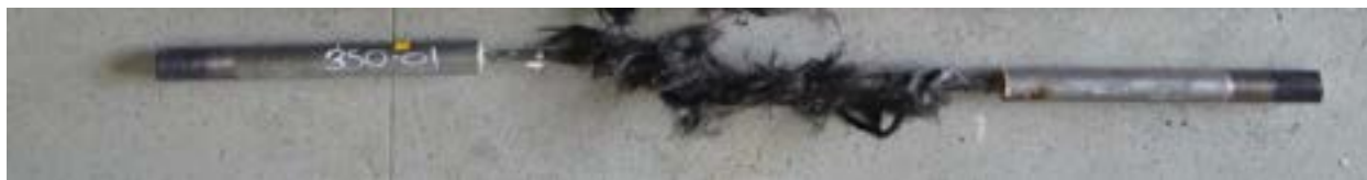
Figure 6.2-14 Failure of CFCC specimen at 662 °F (350 °C)
