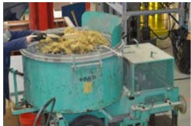
Figure 8.5-10 Mixing UHPC using centrifugal concrete mixer
