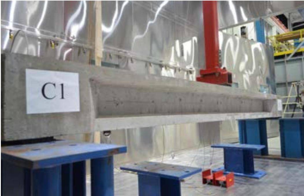
Figure 7.3-52 Three-point loading of Beam C1 (midspan camber of 0.75 in.)
