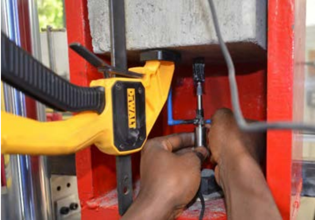
Figure 4.2-6 Attaching LVDT to monitor the slippage of strands
