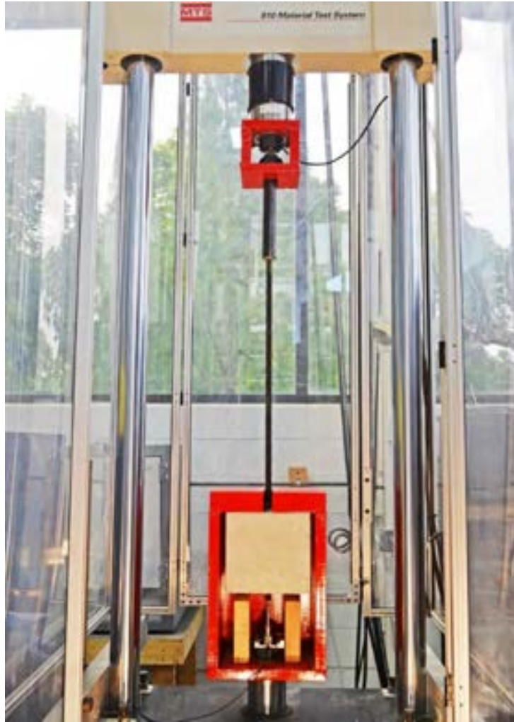
Figure 4.2-8 Test setup for pullout specimens
