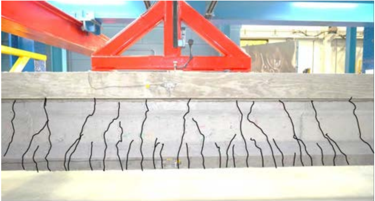
Figure 5.5-9 Development of flexural cracks during flexural loading of Beam C0.6 before failure
