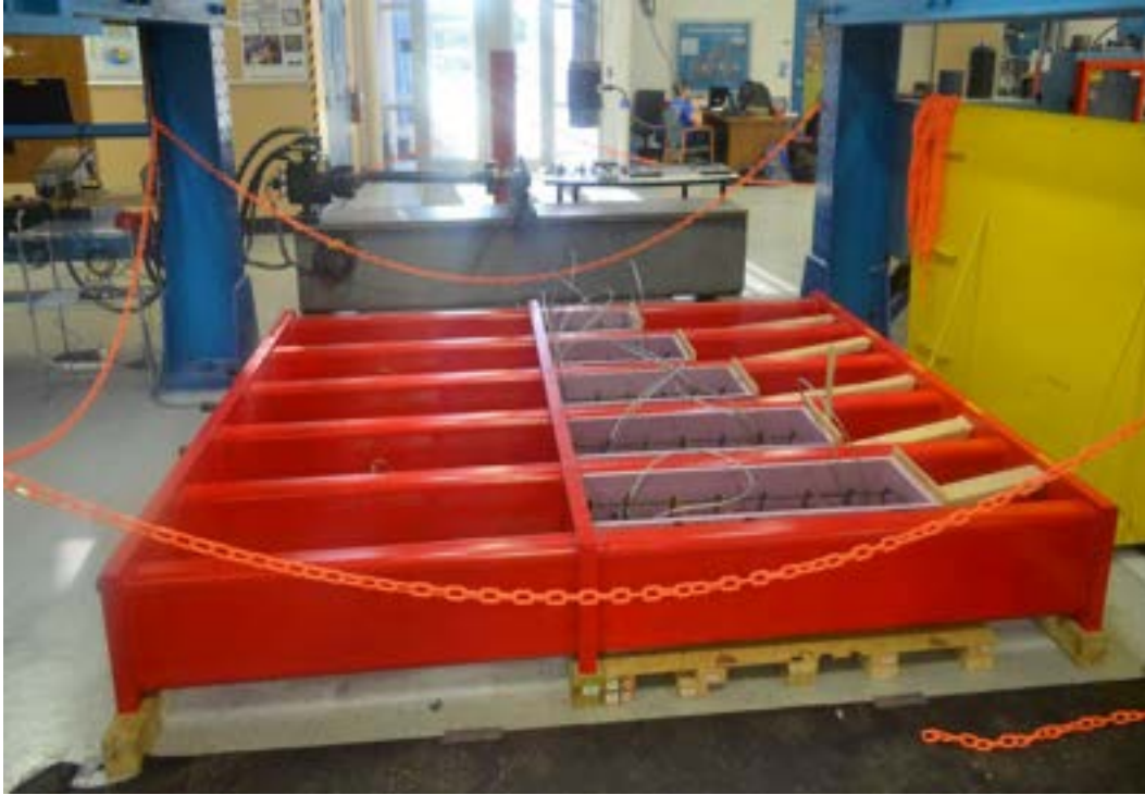
Figure 4.3-5 First set of transfer length specimens prior to concrete pouring, measuring 12 in. \times 12 in. with lengths of 18, 24, 30, 36, and 42 in. (No. 3 steel stirrups every 6 in.)
