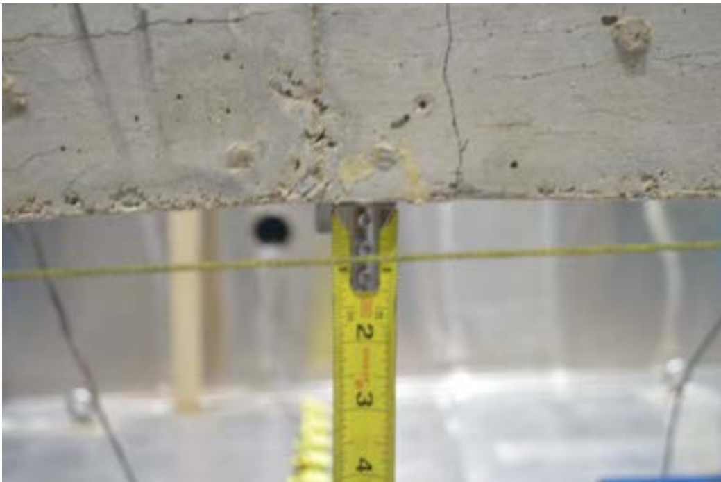
Figure 7.3-73 Midspan camber of 0.75 in. (19 mm) in Beam H1 before flexural testing
