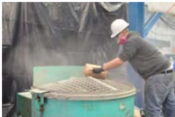
Figure 8.5-10 Mixing UHPC using centrifugal concrete mixer
