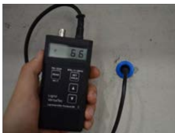
Figure 6.3-21 Obtaining humidity and temperature readings with the moisture meter
