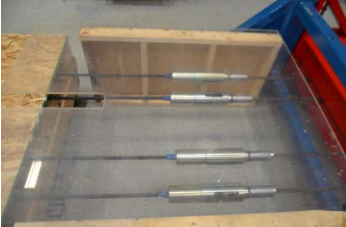
Figure 2.3-7 Coupling CFCC strands with steel strands at the live end
