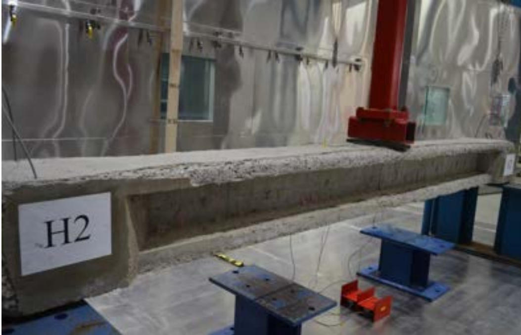
Figure 7.3-78 Three-point loading of Beam H2
