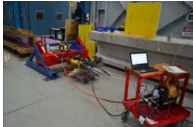
Figure 8.4-5 Prestressing CFCC strands by pulling coupled steel strands using hydraulic pump
