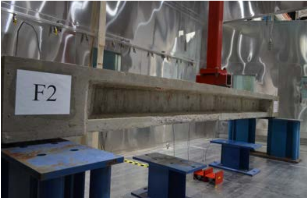
Figure 7.3-66 Three-point loading of Beam F2
