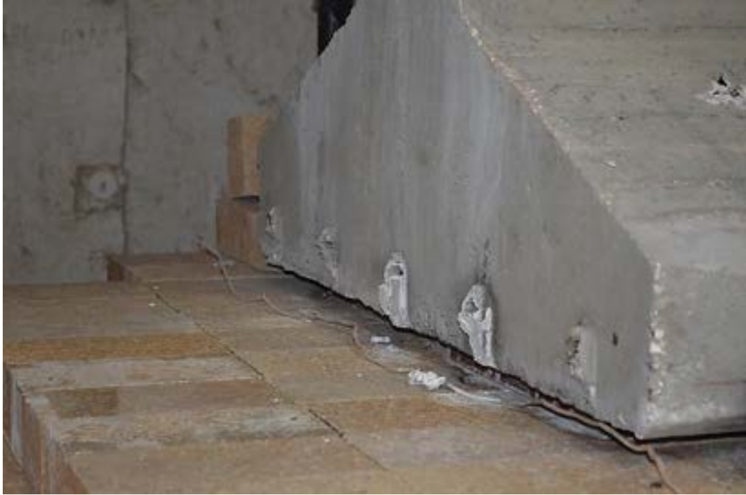
Figure 6.3-86 Close-up view at end of beam after fire test showing slippage of the strands
