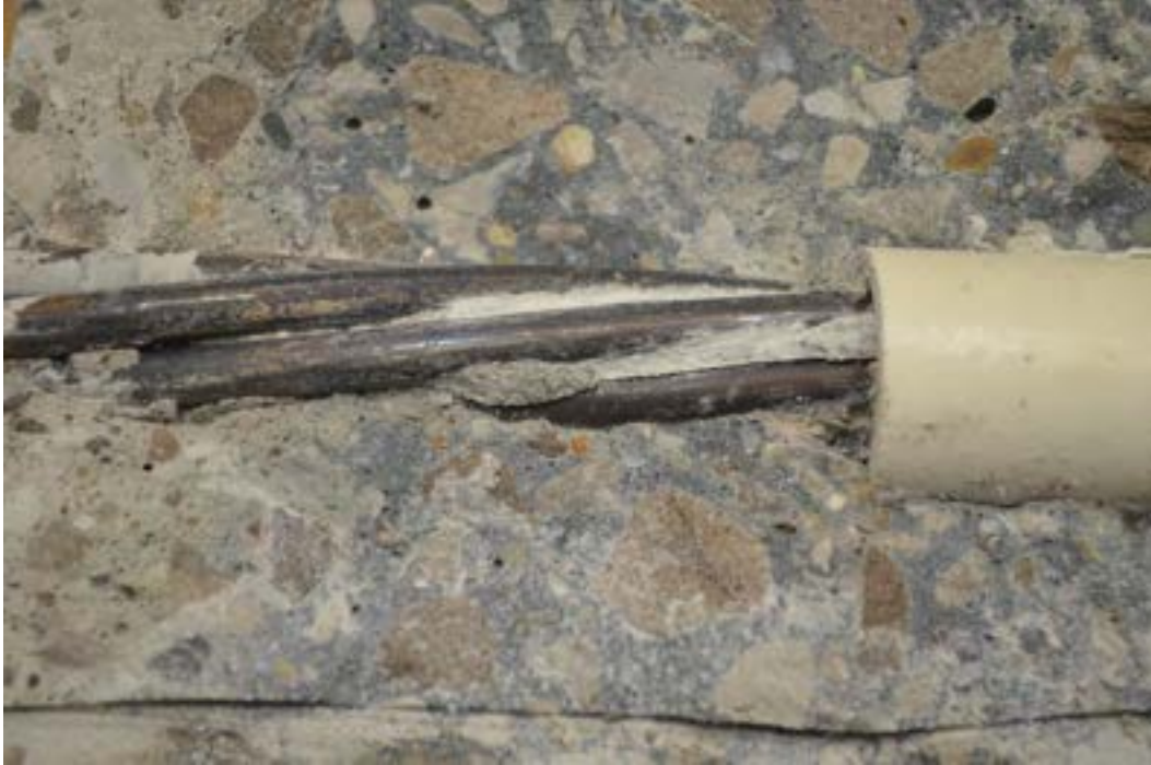
Figure 4.2-15 Development of shear interlock between the concrete paste and steel strands
