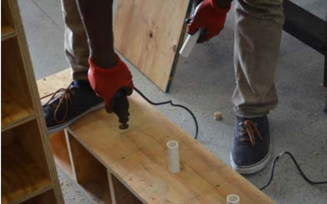
Figure 4.2-3 Inserting debonding PVC tubes to control the bond length
