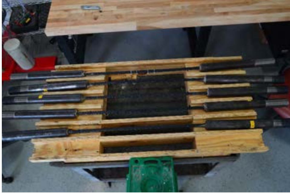
Figure 6.2-2 Completed test specimens with two anchor devices
