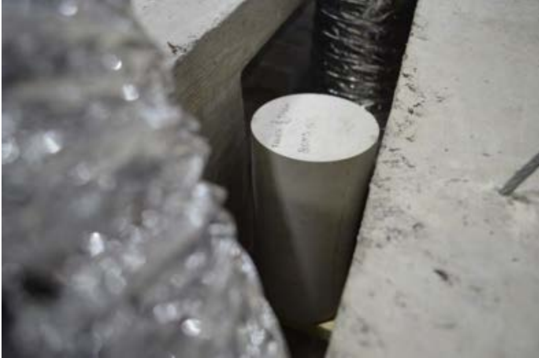
Figure 7.3-37 Concrete cylinders from the same batch as the beams placed with the beams and exposed to freeze-thaw cycles
