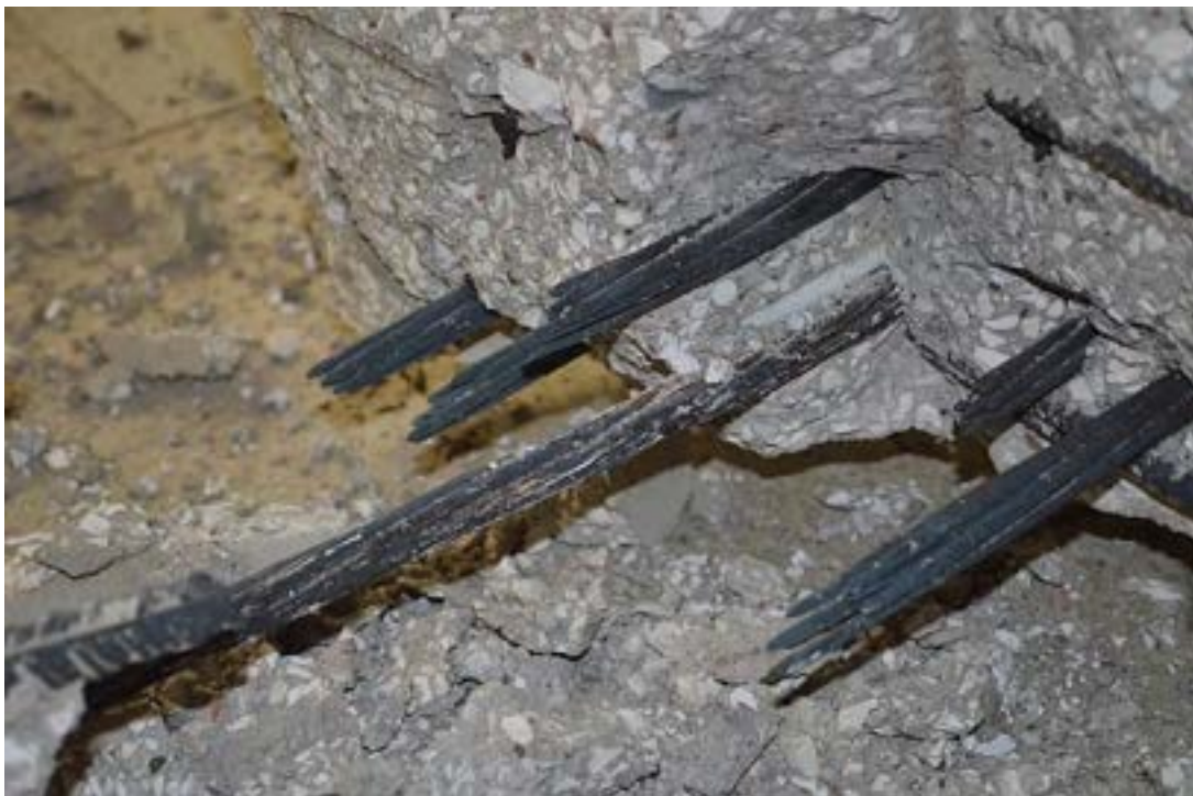
Figure 6.3-63 Rupture of steel strands at midspan
