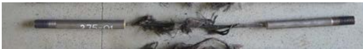
Figure 6.2-11 Failure of CFCC specimen at 527 °F (275 °C)
