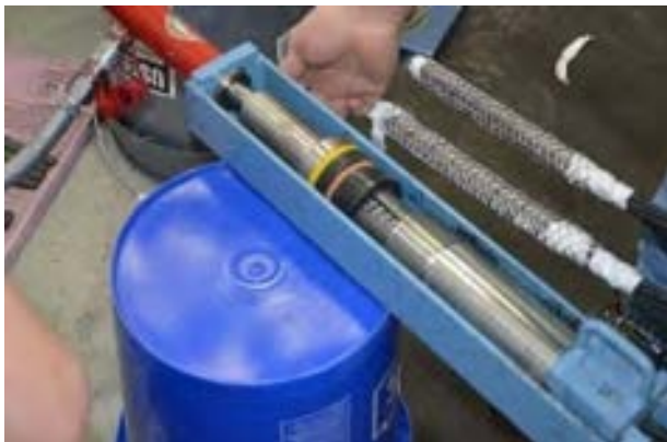
(e) Sliding steel wedges using hand pump
