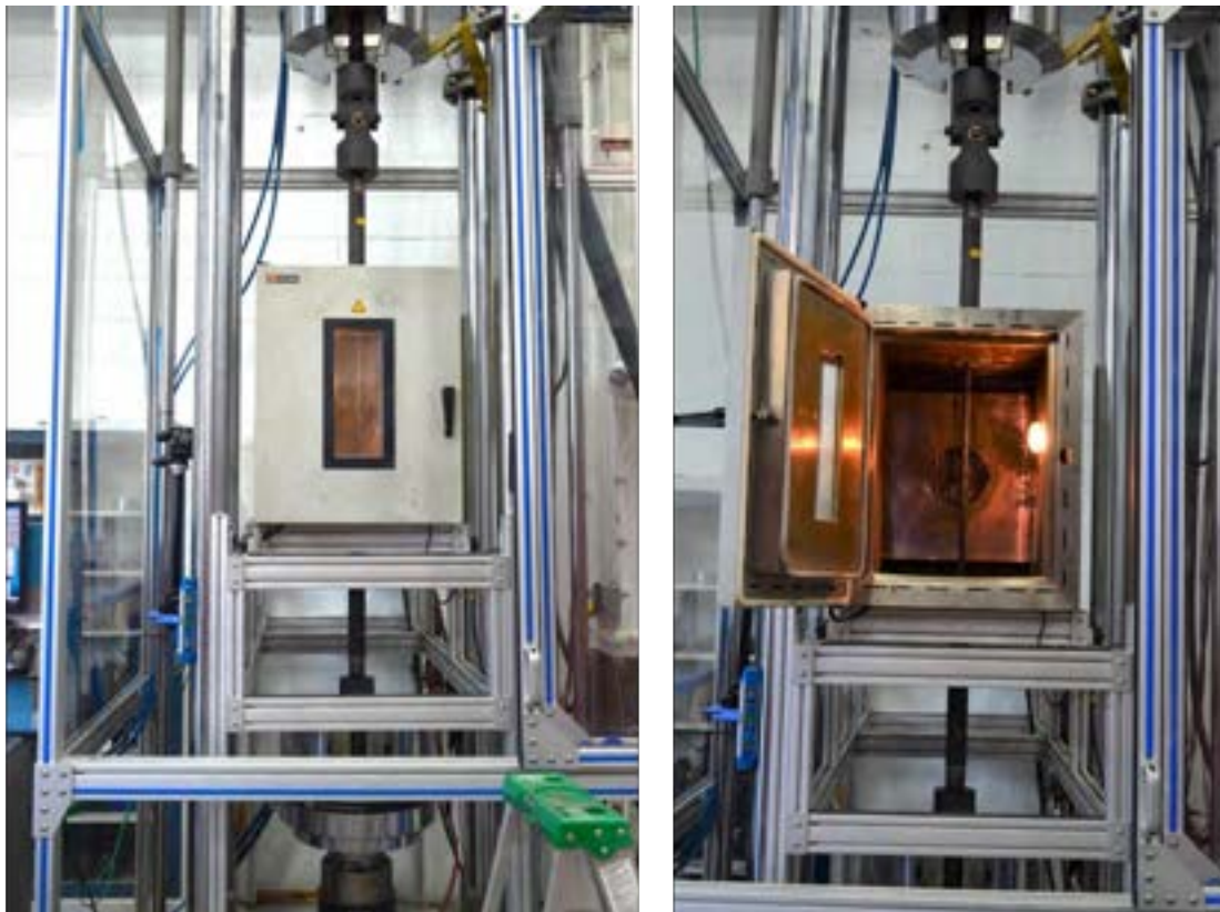
Figure 3.3-13 Heat relaxation test setup
