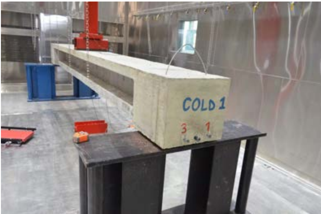
Figure 7.3-19 Beam F1 under three-point loading in the environmental chamber
