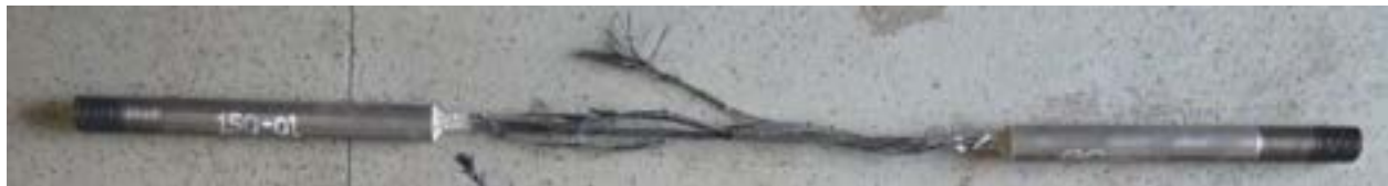
Figure 6.2-6 Failure of CFCC specimen at 302 °F (150 °C)
