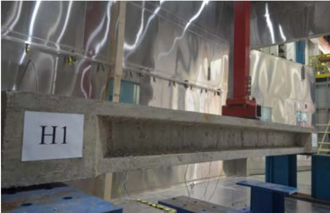
Figure 7.3-72 Three-point loading of Beam H1
