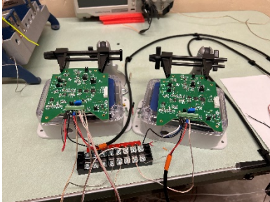
a) Separate battery power supply for 2 boards
