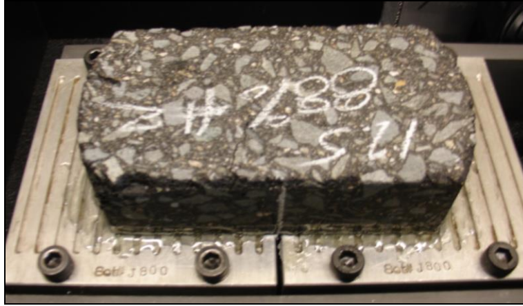
Figure 6. Typical Overlay Test Setup
