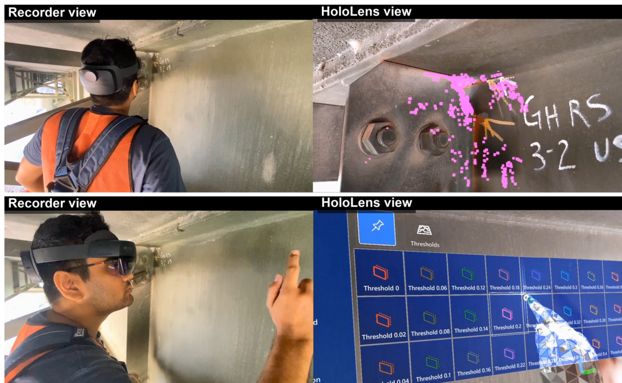
Figure 1. Human-centered fatigue crack inspection tool developed under NCHRP IDEA 223
