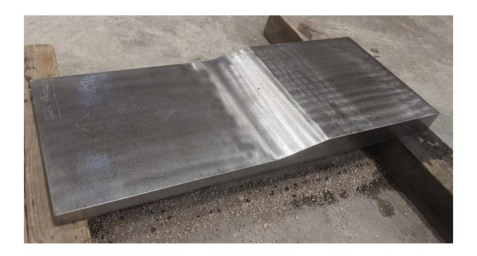
Photograph of typical plate for performance testing of UT inspectors examining CJP welds in T1 steels
