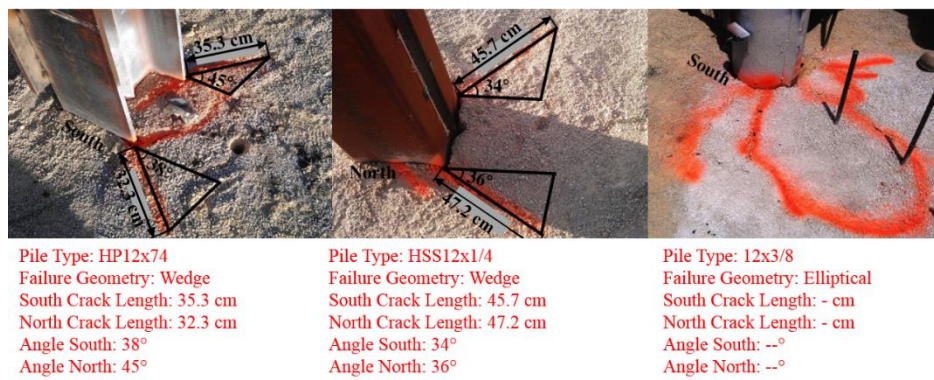
Figure 3-4: Shear planes adjacent to each pile shape at end of lateral loading.
