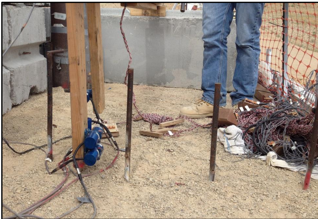
Figure 4-2: Horizontal ground displacement setup.
