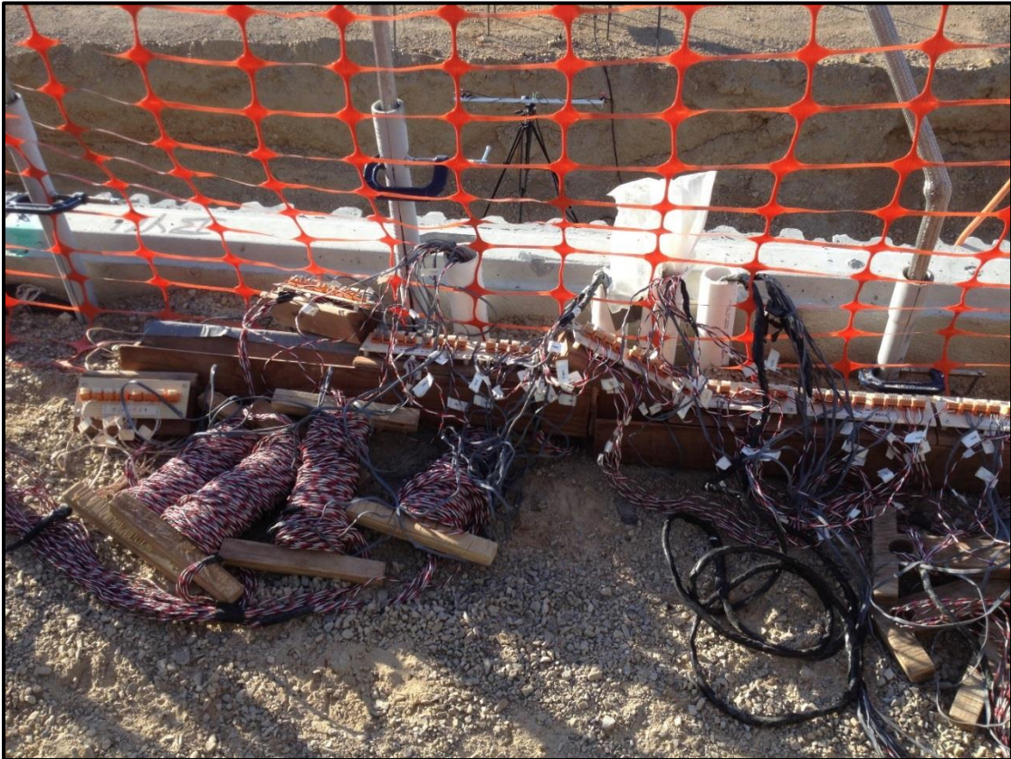
Figure 4-4: Strain gauge connections to terminal strips.
