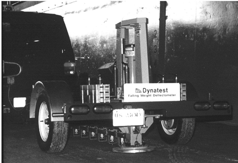
Figure 2.5.6.1: CRREL Falling Weight Deflectometer.
