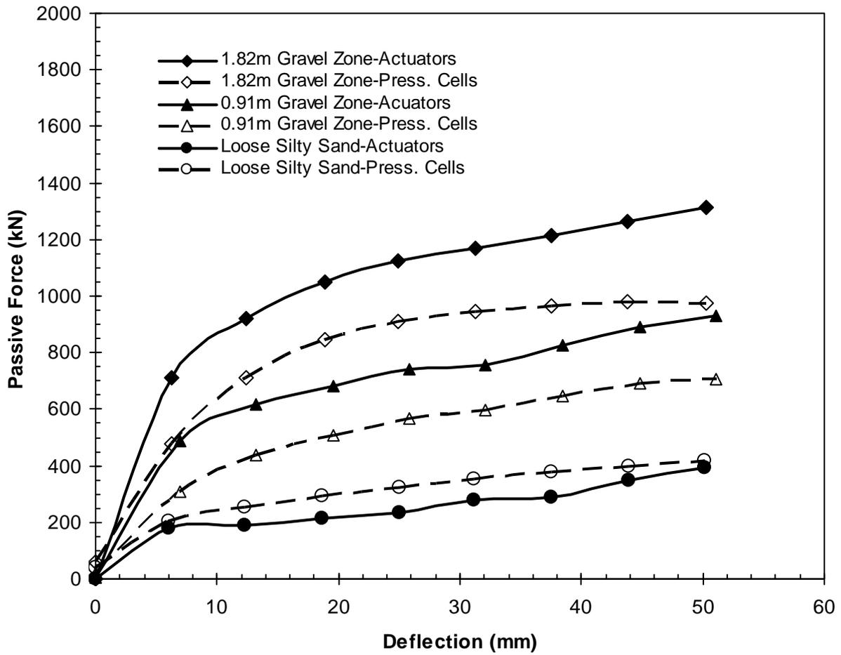
**Fig. 5. Comparison of passive force vs. deflection curves obtained from hydraulic actuators and earth pressure cells for lateral pile cap tests.**
