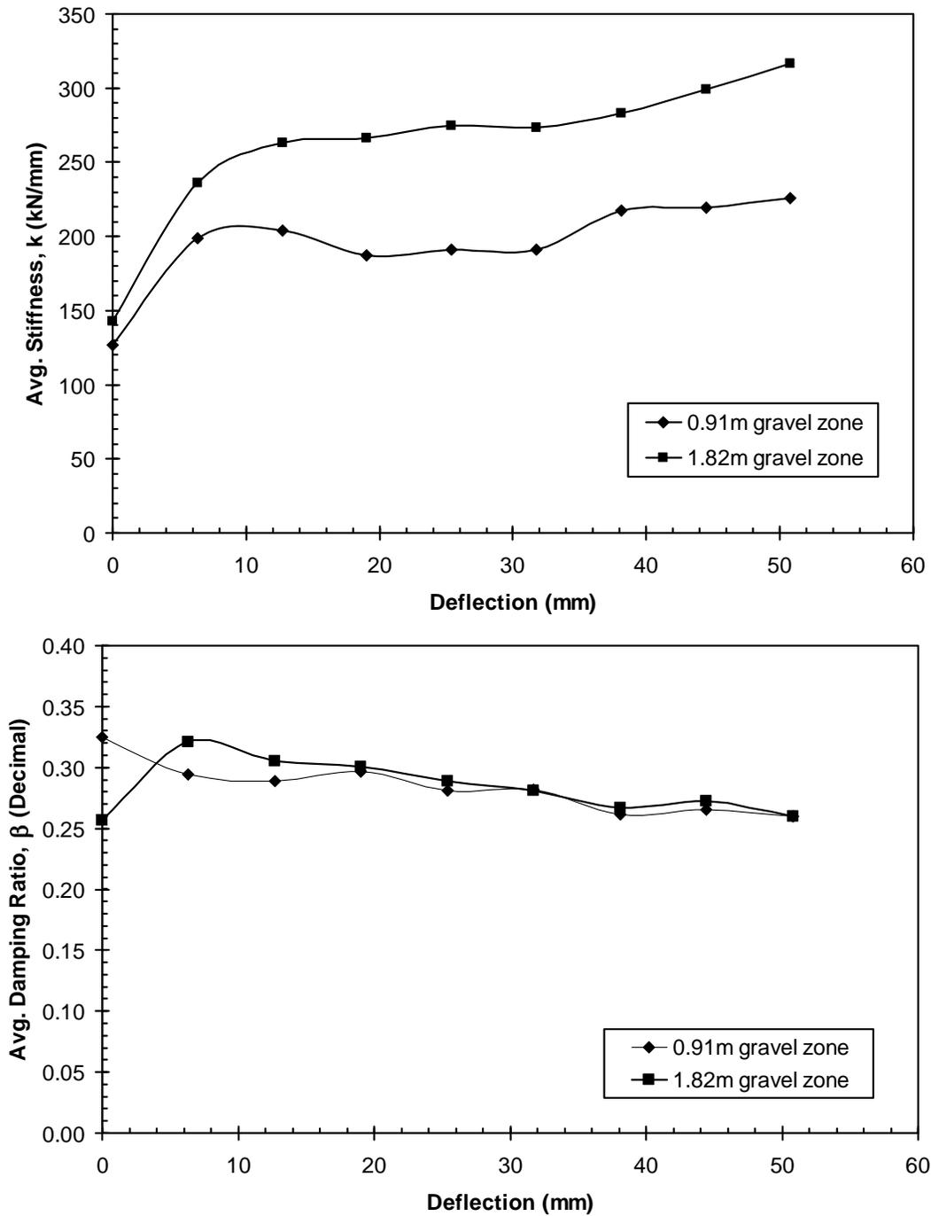
**Fig. 10. Plots of (a) average dynamic stiffness and (b) average damping ratio as a function of deflection level for the backfill tests involving 0.91- and 1.82-m wide dense gravel zones.**
