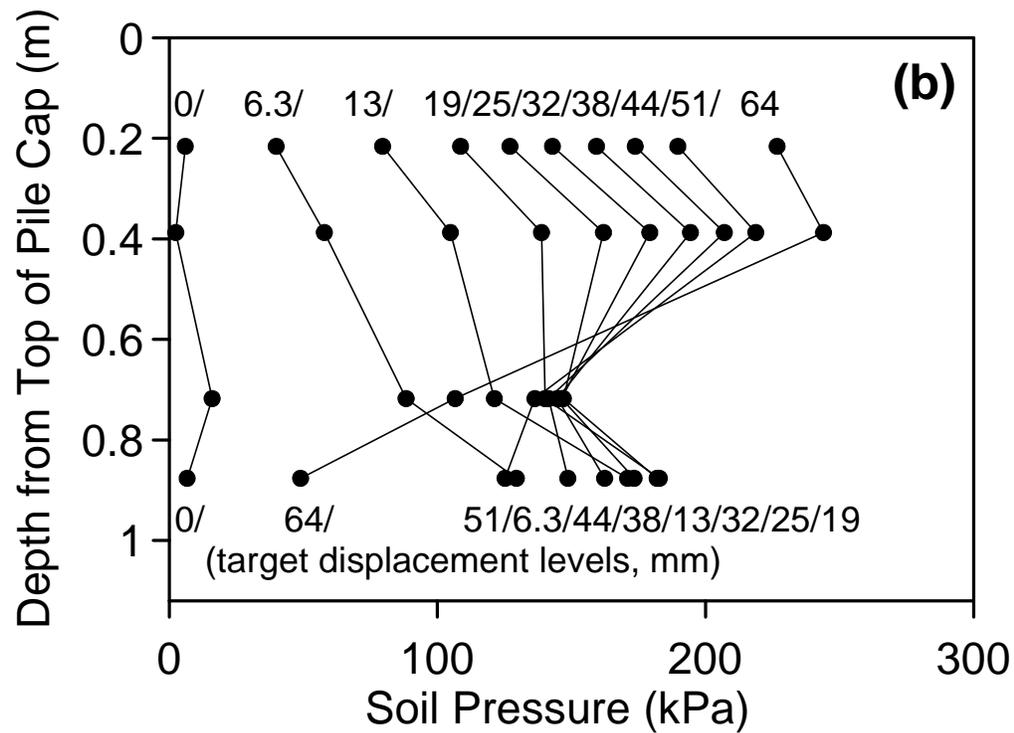
Fig. 4. Pressure vs. depth curves at various deflection increments for the backfill with (a) the 0.91-m wide gravel zone and (b) the 1.82-m wide gravel zone.
