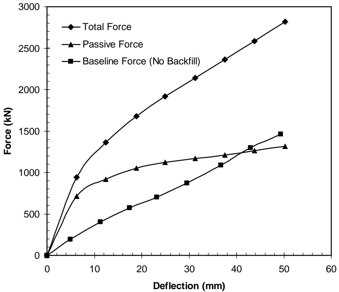
**Fig. 2. Plots of total force, baseline force, and passive force vs. deflection for the pile cap with backfill consisting of a 1.82-m wide zone of dense sand in front of loose silty sand.**
