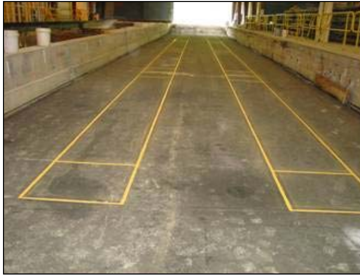
Figure 3. Paved test sections showing test windows (outlined in yellow) to which traffic was applied, including the short transition sections. Traffic was applied in a direction away from the viewer of this image.
