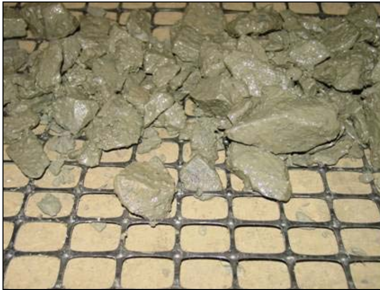
Figure 25. Close-up of geogrid and base aggregate particles.
