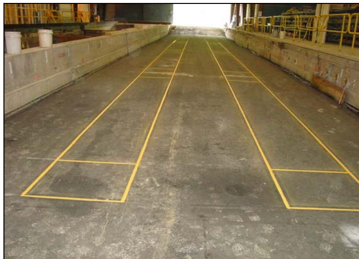
Figure 29. Paved test sections and marked test windows. The traffic was applied in the direction away from the viewer; the loading transition zone is in the foreground.
