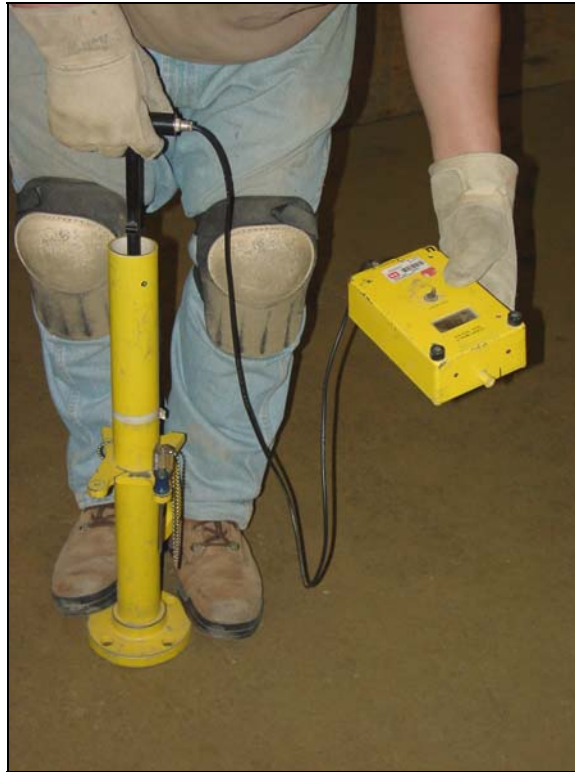
Figure 17. Clegg impact hammer.
