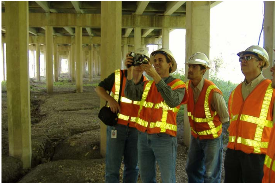
Figure 4. Photograph of field testing of the IR cameras in Texas.
