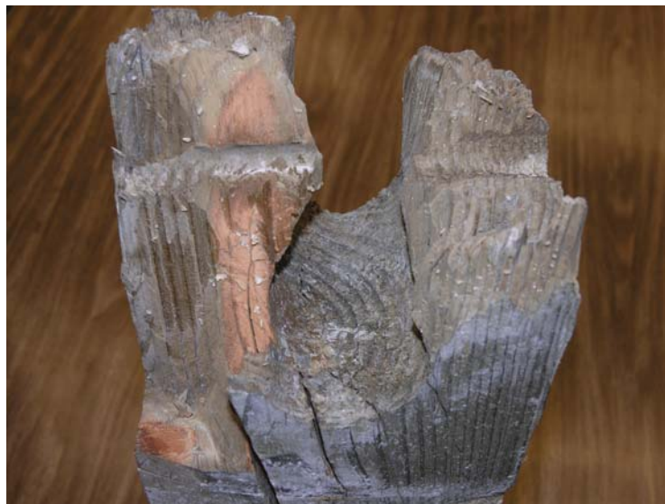
Figure 7. Damaged BCT Wood Post - Test MWTSP-1
