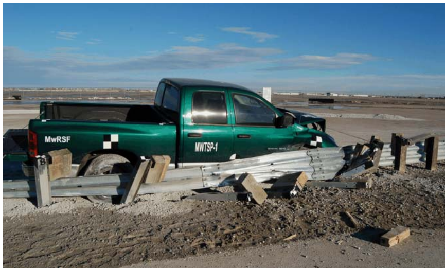
Figure 6. Damage to Approach Guardrail Transition - Test MWTSP-1
