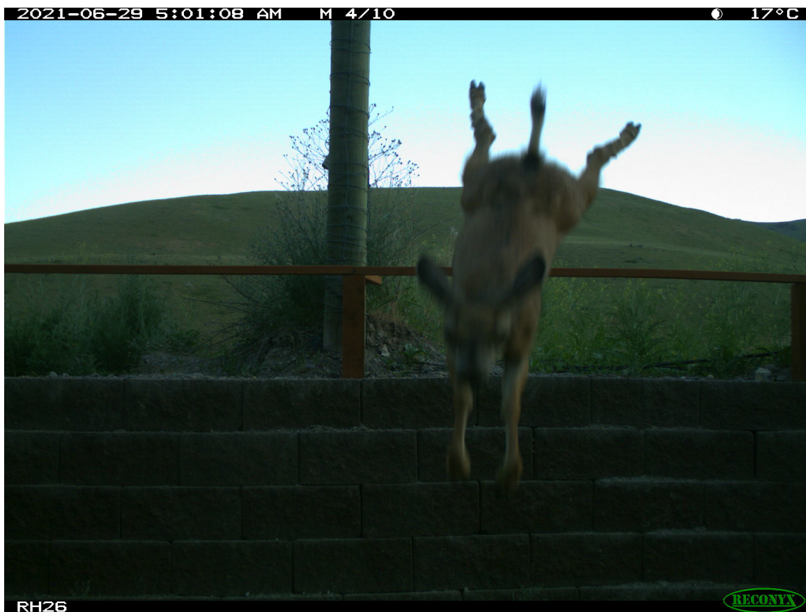
Figure 12: A mule deer jumps down the jump-out with the prototype (height 18 inches, setback 4 inches). The animal starts the jump from behind the bar and does not step over the bar first before jumping down.
