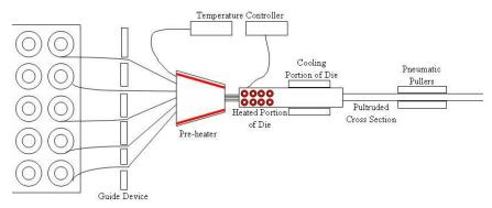
Figure 2: Schema of how pultrusion members are formed (Kamble, 2008).
