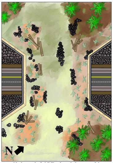
Figure 35: Planting strategy with clear path of visibility through the center of the structure.
