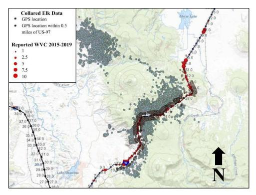
Figure 25: Collared elk GPS locations and WVC density along the US-97 mitigation area 2015-2019.
