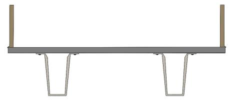
Figure 43: Cross section of CT girder pedestrian bridge design.
