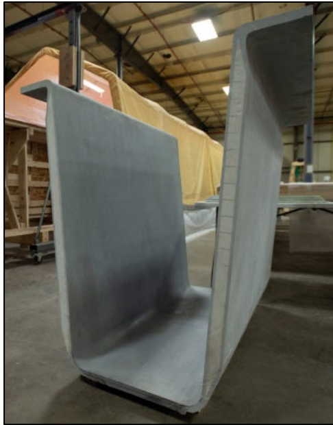
Figure 16. A photo and the dimensions in centimeters (cm) of the FRP or composite tub girder used to form the structure for the design of the wildlife overpass structure on US-97 in Siskiyou County, California.
