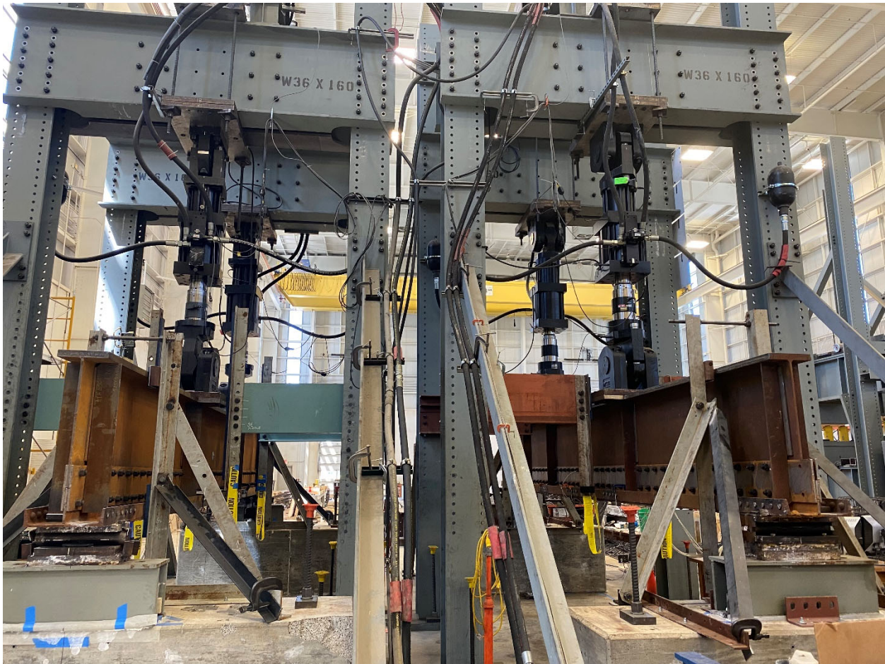
Figure 1 – Photographs of fatigue testing set-up of large-scale girders with real pack-out corrosion.
