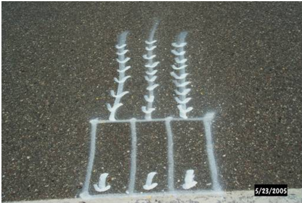
Figure C-1. Core and beam layout prior to cutting
