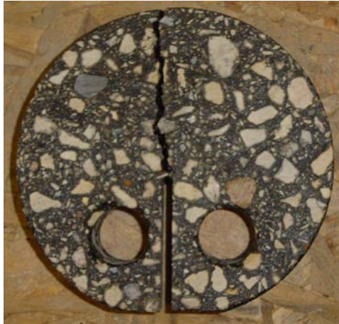
Figure 6.3. DC(T) specimen after testing
