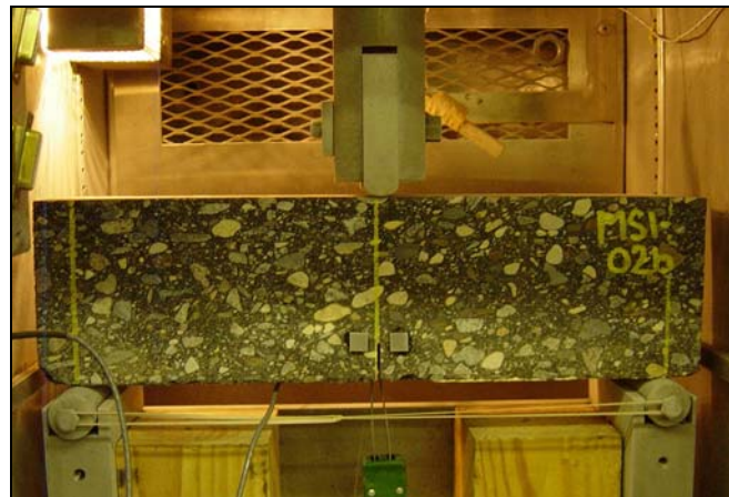
Figure 6.14. Test configuration of the SE(B)
