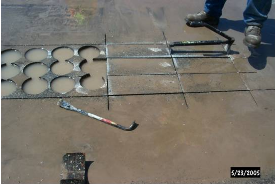
Figure C-5. Sample area and tools for removing beams
