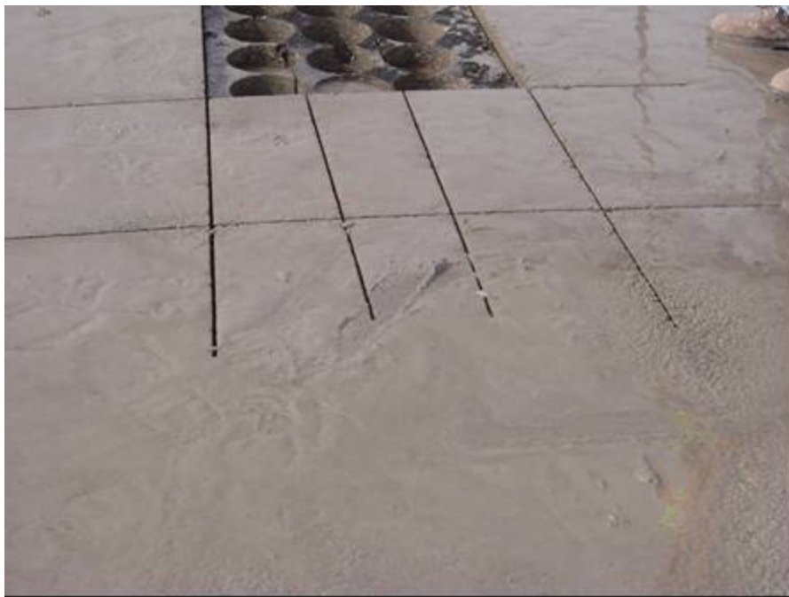
Figure D-5. Cut beams in road
