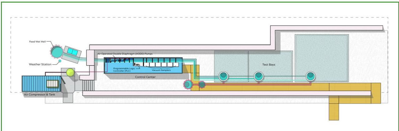
Figure 2. Plan view of major physical components for the Stormwater Technology Testing Center
