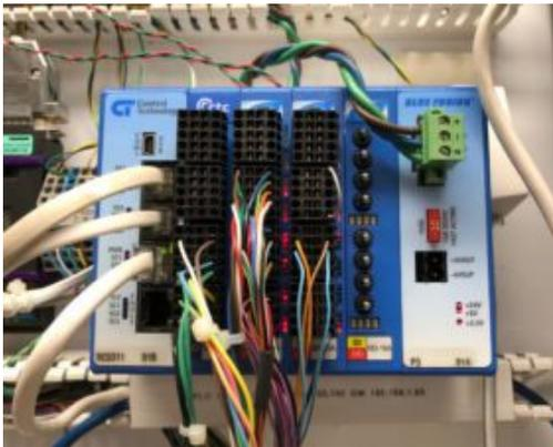
**Figure 5. Programmable Logic Controller**
