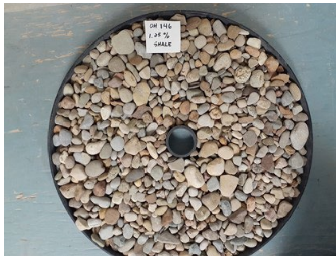
Figure 5.7: Blended Shale (1.25%) in OH146 Sample Tray
