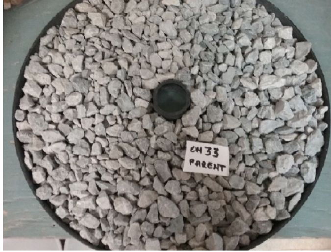
Figure 2.4: Ohio Coarse Aggregate in SLT Sample Tray
