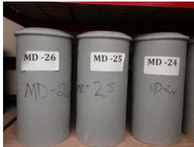
Figure 1.4: Sample Cylinders from MDSHA
