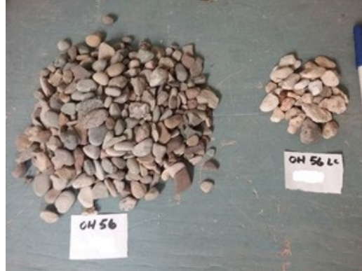
Figure 5.1: OH56 Parent Gravel and Light Chert Sample
