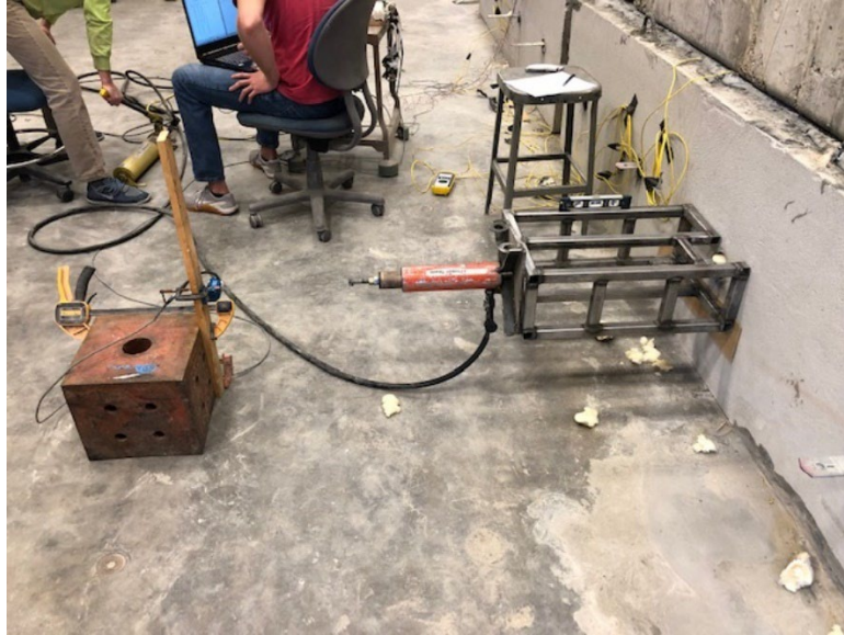
Figure 6. Photograph of the center-pull hydraulic jack used to apply the pull-out force to the ribbed-strip reinforcement along with string potentiometer attached to an independent reference point to monitor lateral displacement of the reinforcement.
