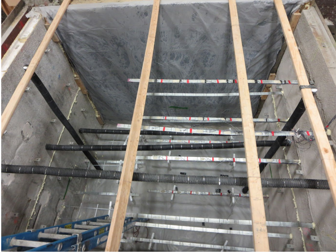
Figure 3. Reinforcements in concrete test box 6 prior to pouring the first lift.
