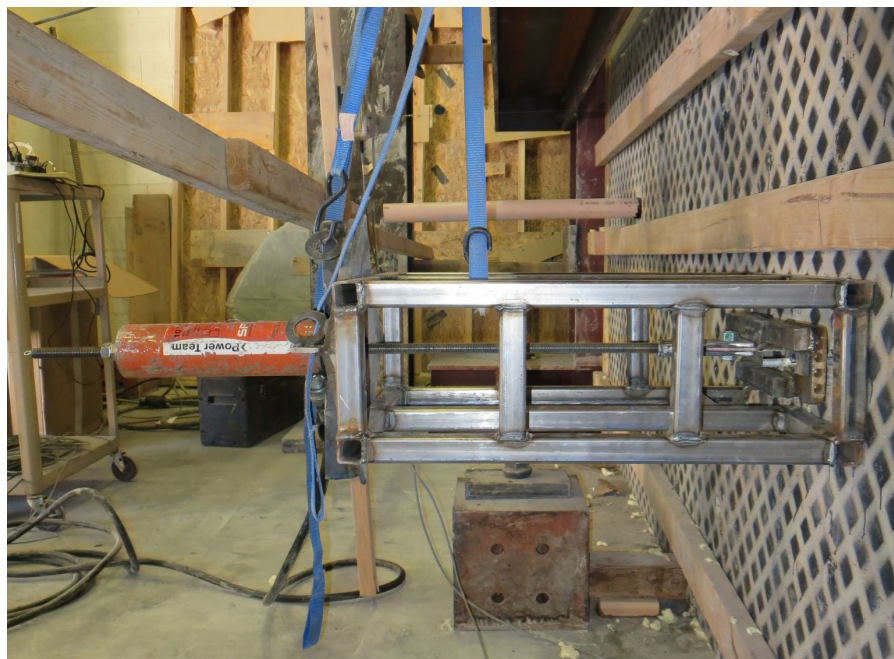
Figure 9. Photograph of the center-pull hydraulic jack used to apply the pull-out force to the welded-wire reinforcement.
