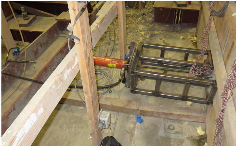
Figure 4. Photograph of the center-pull hydraulic jack used to apply the pull-out force to the ribbed-strip reinforcement along with string potentiometer attached to an independent reference point to monitor horizontal displacement of the reinforcement.
