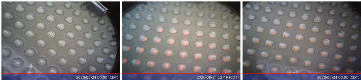
Figure 21: Lawrence field test data during the coldest days in winter 2019-2020 and hottest days in summer 2020 showing the performance of the red, yellow, and green signal lights under different weather conditions. Test results were collected at the intersection of County Rd 458 (or 1200 Rd) /US-59, where the selected signals are on the side of the road shoulder, facing north.
