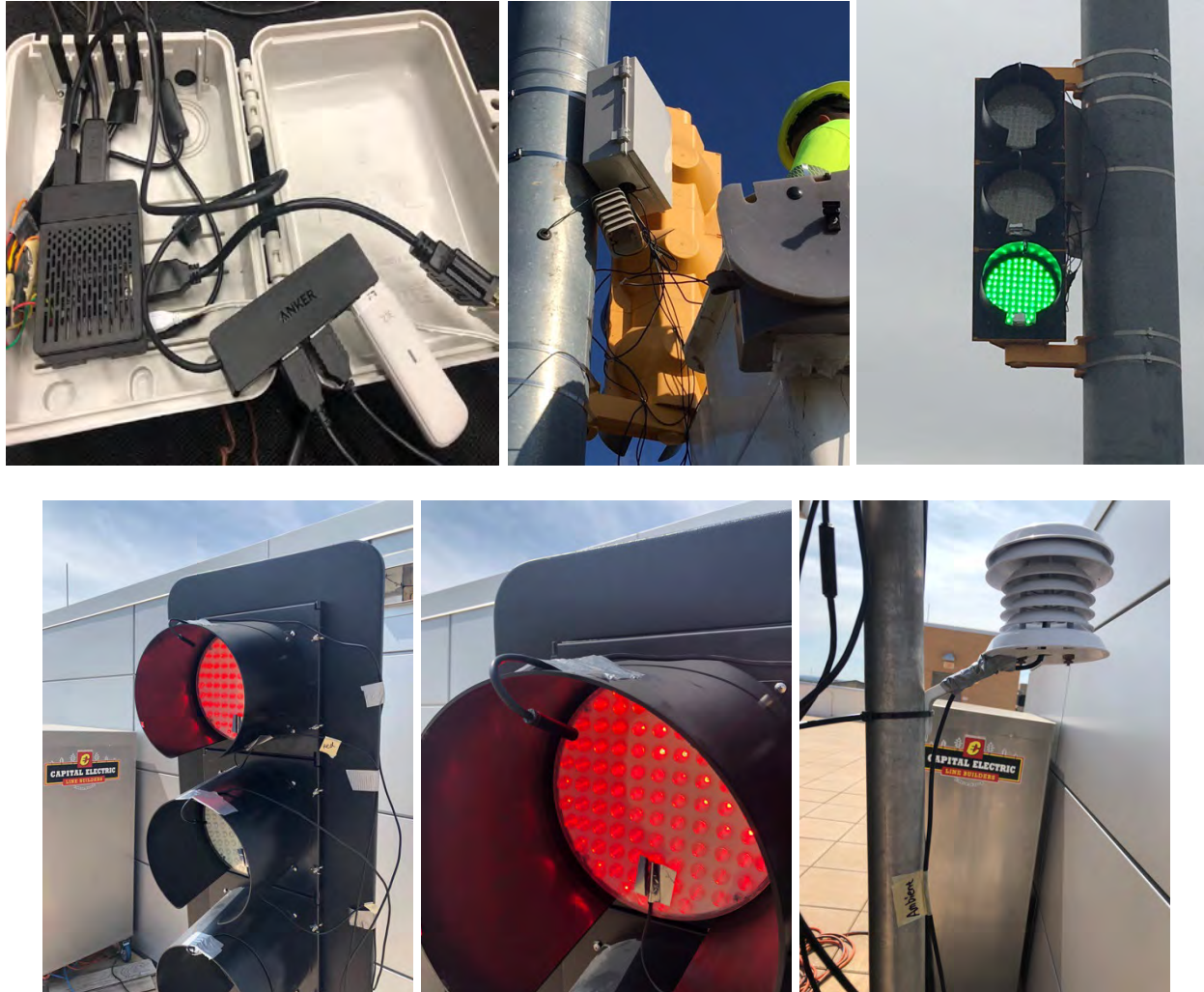
Figure 16: A remote field performance monitoring system, controlled by a Raspberry PI computer with a USB driver for recording data, which consists of three cable cameras used to monitor the lens of the three signal lights (Red, Yellow, Green), four temperature sensors used to record the lens' surface temperature of signal lights and the ambient air temperature, LTE mobile communication device with a monthly data plan, power supplies, and mounting accessories.
