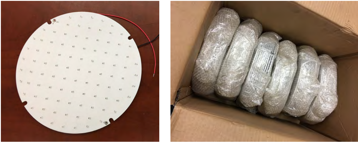
Figure 4: Sixty pieces of self-designed LED light engines, which were custom made with the aid of the industrial partner, including 20 pieces in each color (R, G, Y).
