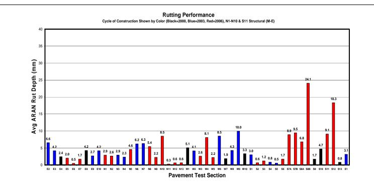
Figure 2 Rutting Performance of Test Sections at the End of Reporting Period
