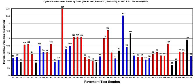
Roughness Performance Cycle of Construction Shown by Color (Black=2000, Blue=2003, Red=2006), N1-N10 & S11 Structural (M-E)
