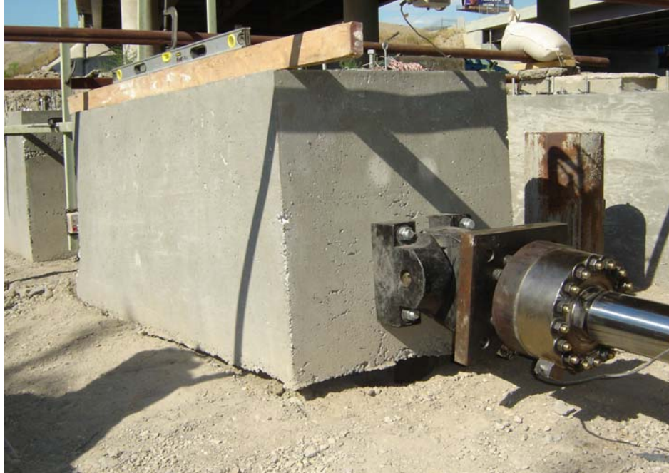
Figure 6 Uplift and rotation of Test Cap 1 at failure.
