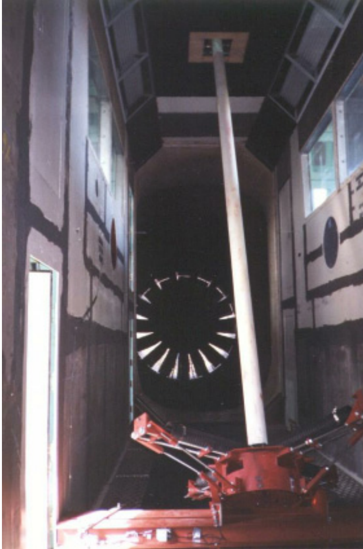
Figure 48: Cable set up in wind tunnel for testing.
