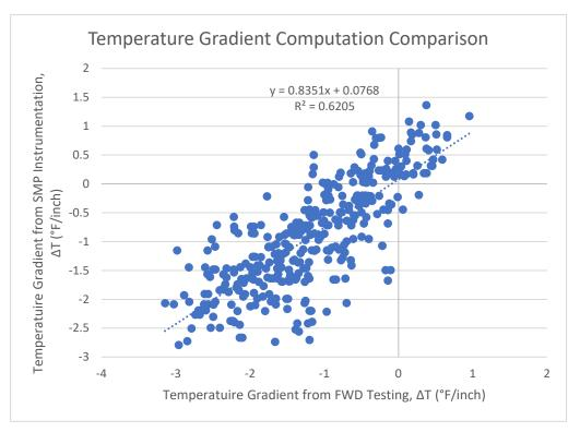
*Figure 10. Comparison of Temperature Gradient Calculated from SMP Instrumentation and FWD Testing for Arizona 0215.*
