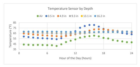
*Figure 3. Air and Pavement Subsurface Temperature for Arizona 0215 on 12/05/1995.*
