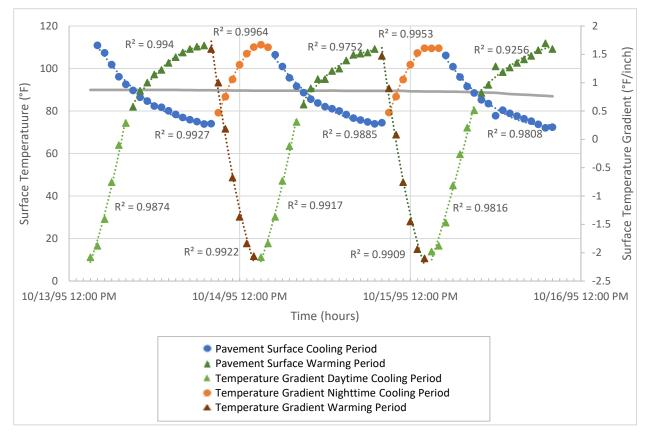
*Figure 8. Impact of Pavement Surface Temperature on Temperature Gradient for Arizona 040215.*
