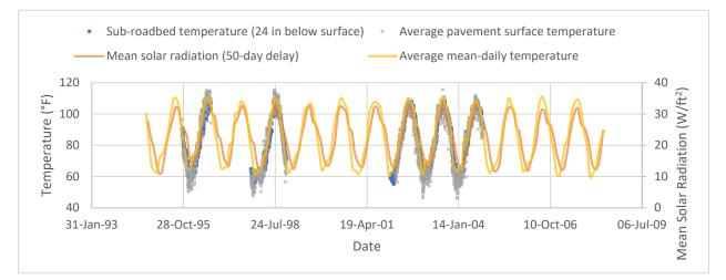
*Figure 4. Comparison of Temperature at 24-inches below the Surface to the Mean Solar Radiation at Arizona 0215*
