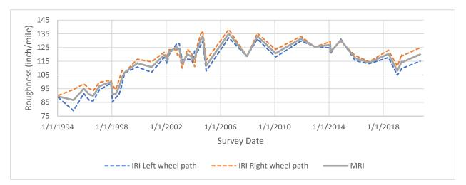
Figure 2. Section-Wide Roughness Measurements for Arizona 040215
