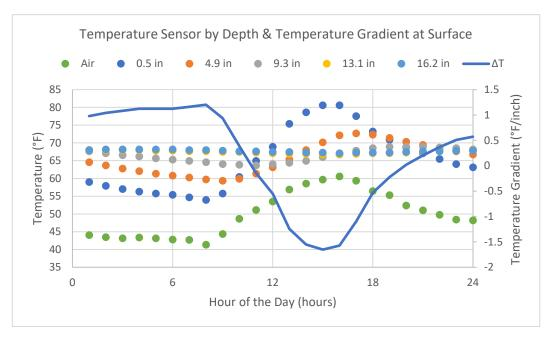
Figure 7. Temperature Gradient for Arizona 040215 on 12/05/1995.
