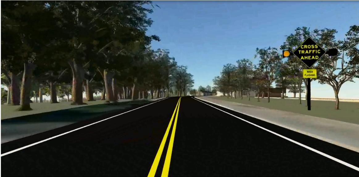
**Figure 3. Screenshot. Blank-out sign with “WHEN FLASHING” placard along two-lane approach to a stop-controlled cross street.**
