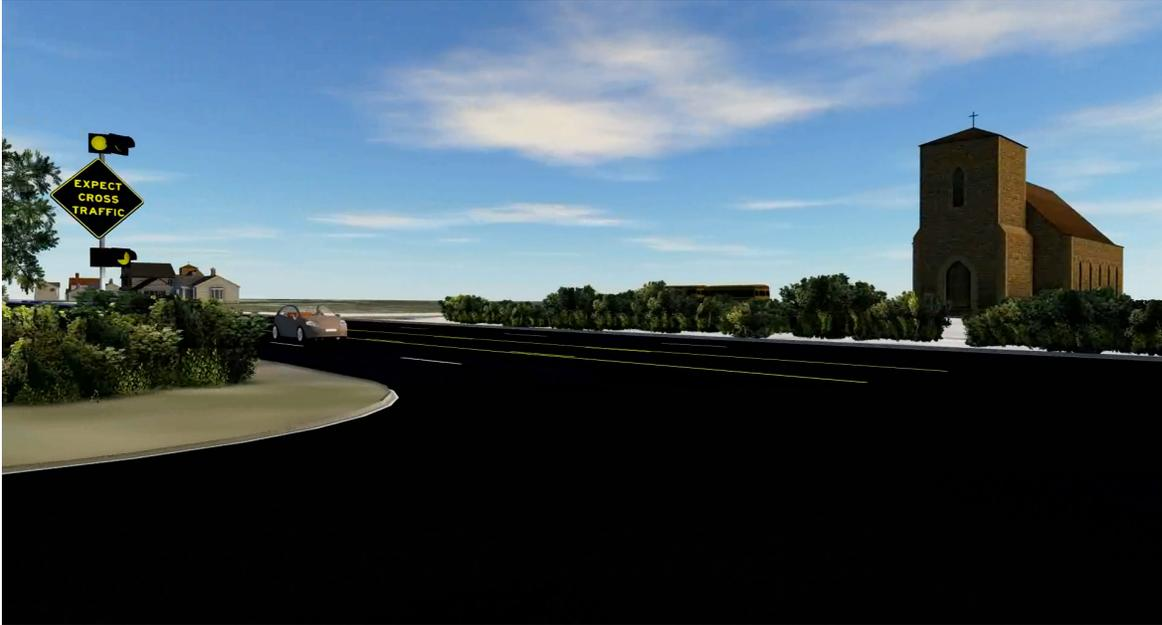
**Figure 7. Screenshot. ICWS warning at stop-controlled intersection with four-lane undivided highway.**
