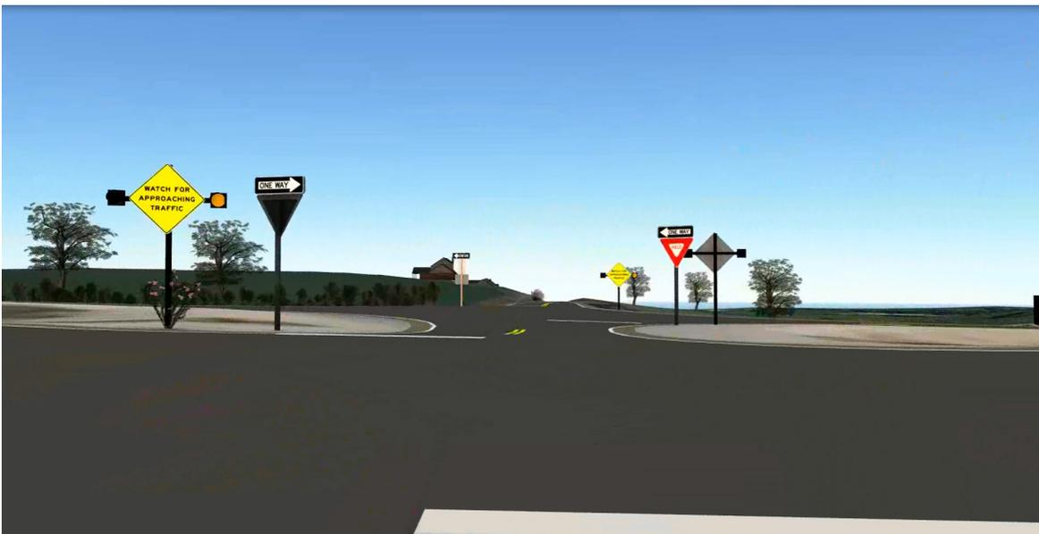
**Figure 8. Screenshot. ICWS at stop-controlled approach to four-lane divided highway.**
