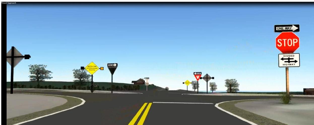
**Figure 22. Screenshot. Exemplar from video showing the ICWS sign placement across from the stop and yield lines.**
