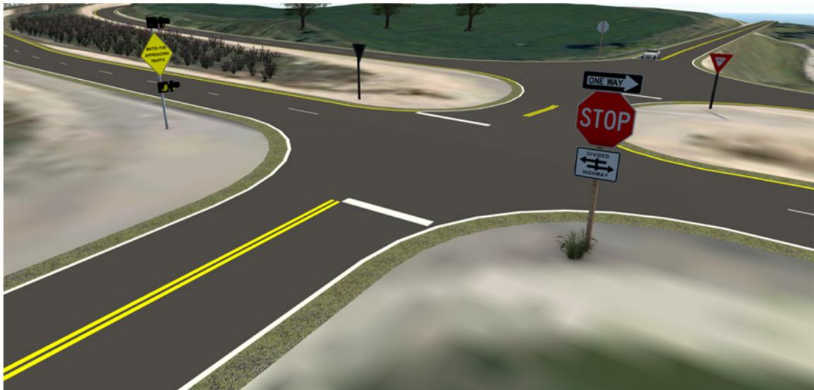
**Figure 2. Illustration. ICWS warning installation at stop sign at intersection with four-lane divided highway.**
