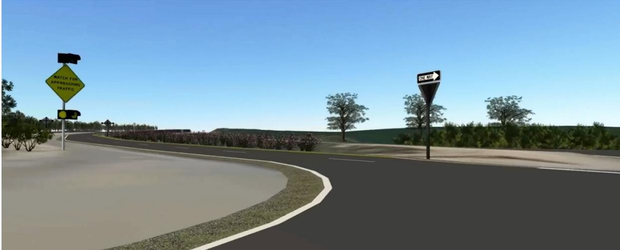
**Figure 23. Screenshot. Exemplar from video showing the ICWS sign placements up stream on the cross road.**
