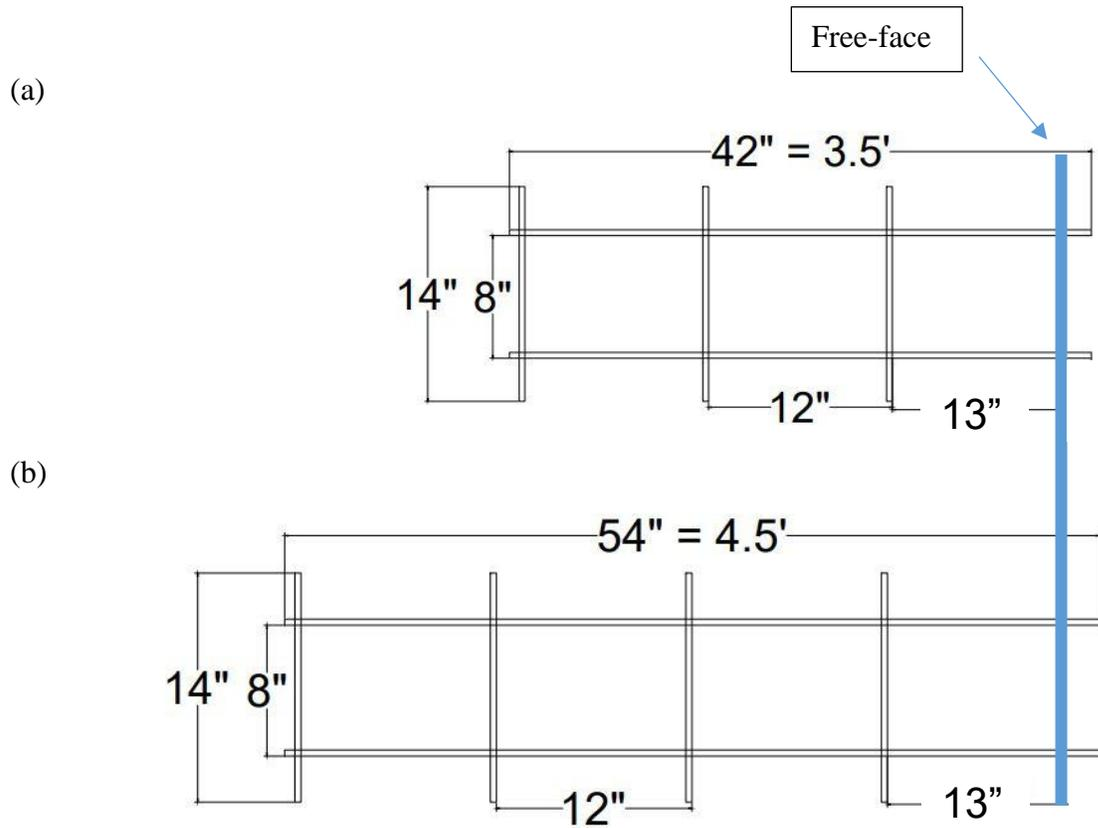
**Figure 3: Auto CAD drawings showing: (a) plan view of 3.5-foot reinforcements and (b) 4.5-foot reinforcements on free face wall.**
