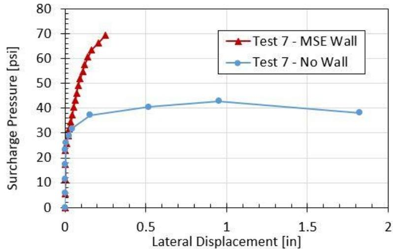
**Figure 8: Applied surcharge pressure vs. lateral wall displacement in the LCC for tests with and without MSE wall for reinforced LLC test 7.**
