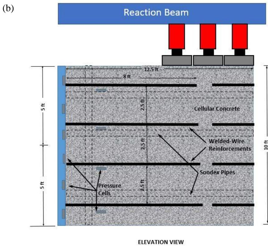
**Figure 5: Schematic drawings illustrating the surcharge load application for (a) the MSE wall test and (b) the free face wall test.**
