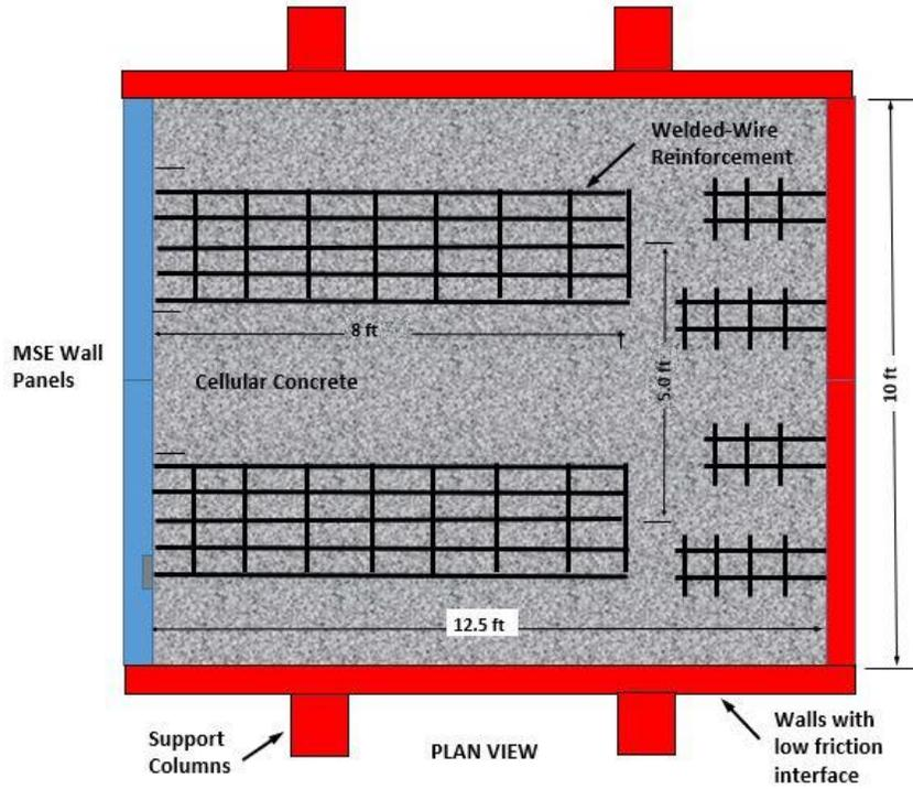
Figure 1: Profile drawings of the test with reinforced LCC behind two 5 feet x 10 feet MSE wall panels (a) Elevation view and (b) Plan view.
