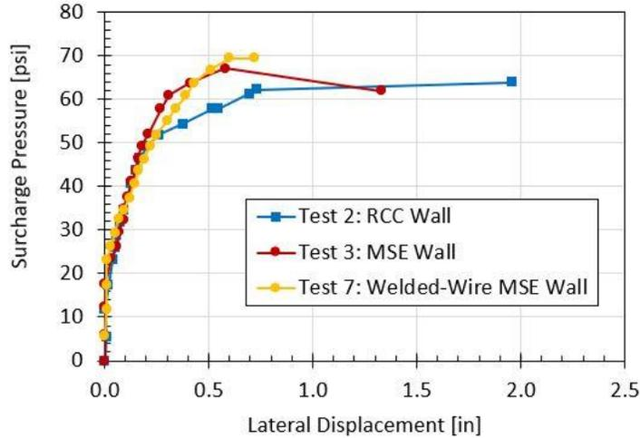
**Figure 9: Applied surcharge pressure vs. lateral wall displacement with MSE retaining wall for reinforced LCC tests 2, 3, and 7.**
