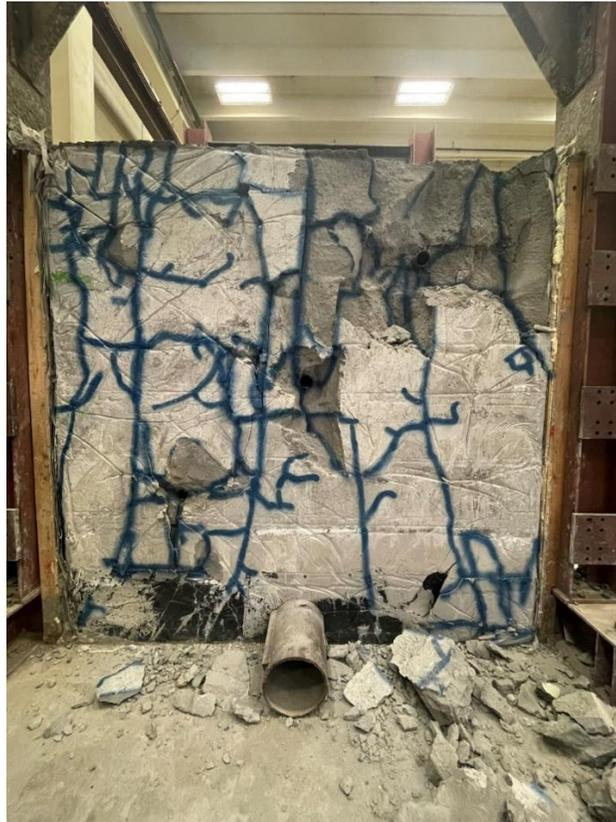
**Figure 14: Photograph of the crack pattern in the LCC on the free face opposite to the MSE retaining wall side.**
