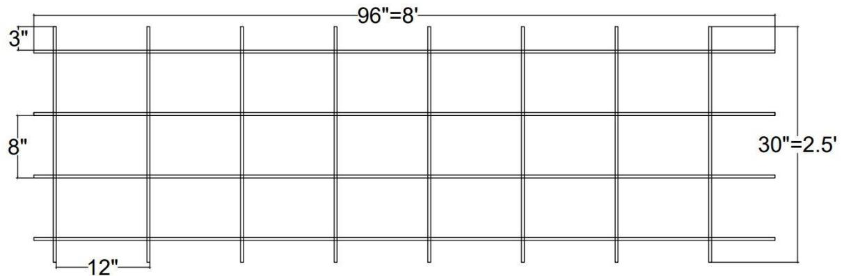
Figure 2: Auto CAD drawings showing: (a) front view of the welded wire grid dimensions and (b) plan view of the welded wire grid dimensions.
