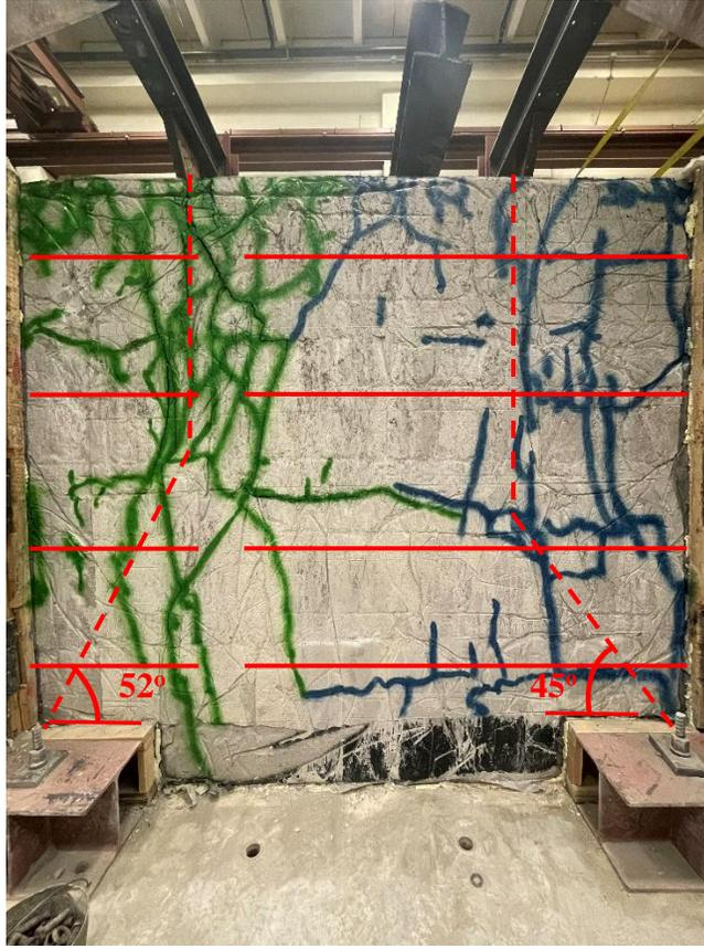
**Figure 13: Photo showing the blue crack patterns adjacent to the MSE wall with the six-foot wide surcharge load at the surface. Green crack patterns are for a second test with four-foot wide surcharge adjacent to free-face without MSE wall. Reinforcement locations are shown by horizontal black lines.**
