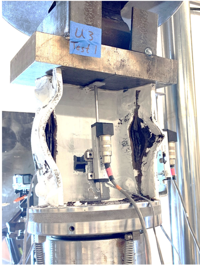
Figure 1 – Photograph of typical compression test on stub-column section. Note light shining through the areas where the corrosion has completely eaten away the cover plate and presence of loose pack-out corrosion product.
