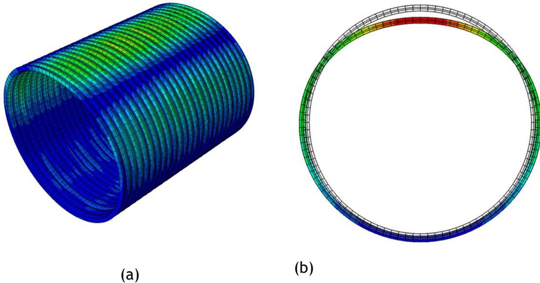
Figure 10-31. (a) Development of plastic strain and (b) Deformation pattern for 2- in. thick polymeric SAPL.
