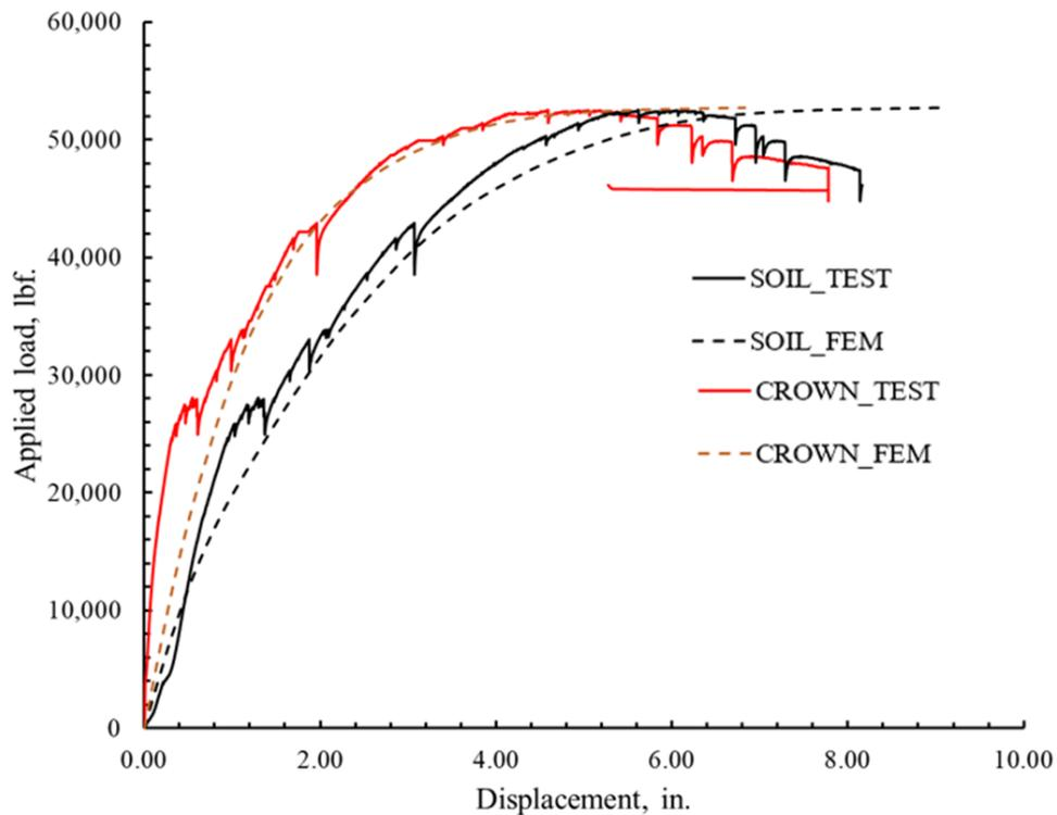
Figure 10B- 2. Comparison of load-displacement plot for the 0.5 in. thick polymeric circular liner.
