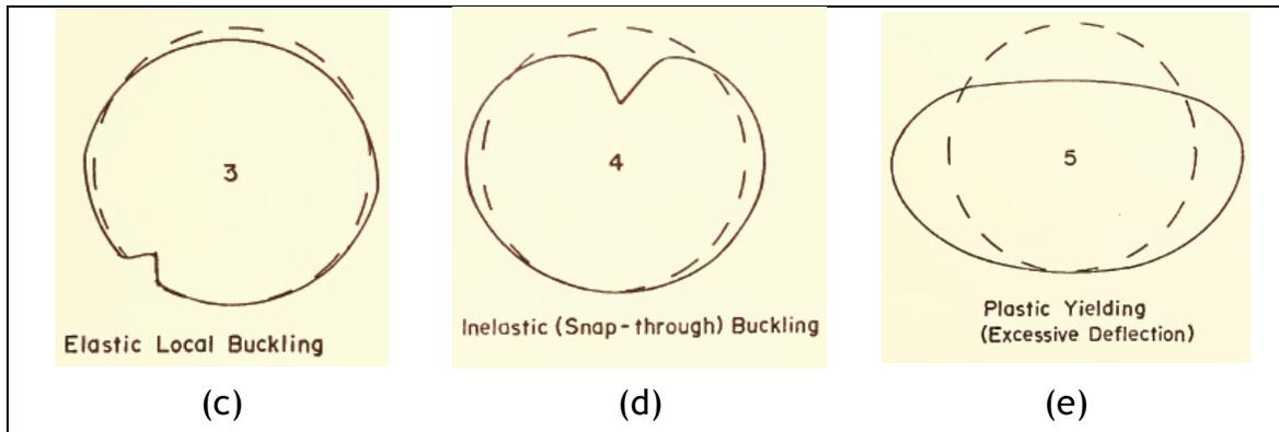
Figure 2-8. Failure modes of flexible conduits: (a) wall crushing, (b) seam separation, (c) elastic local buckling, (d) inelastic (snap-through) buckling, and (e) plastic yielding (excessive deflection) (Leonards and Stetkar 1978).
