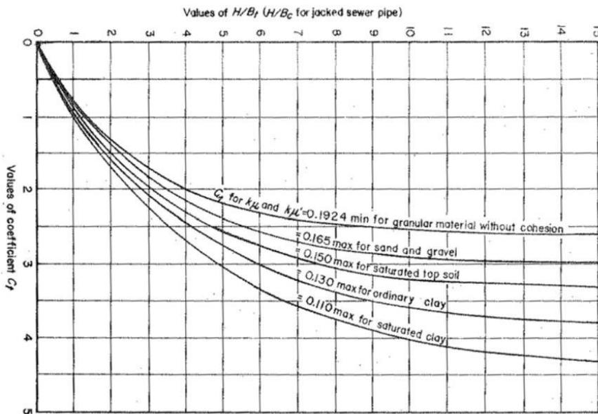
Figure 8-1 Diagram for coefficient  $C_t$  (Figure 9-13 in ASCE MOP 60).
