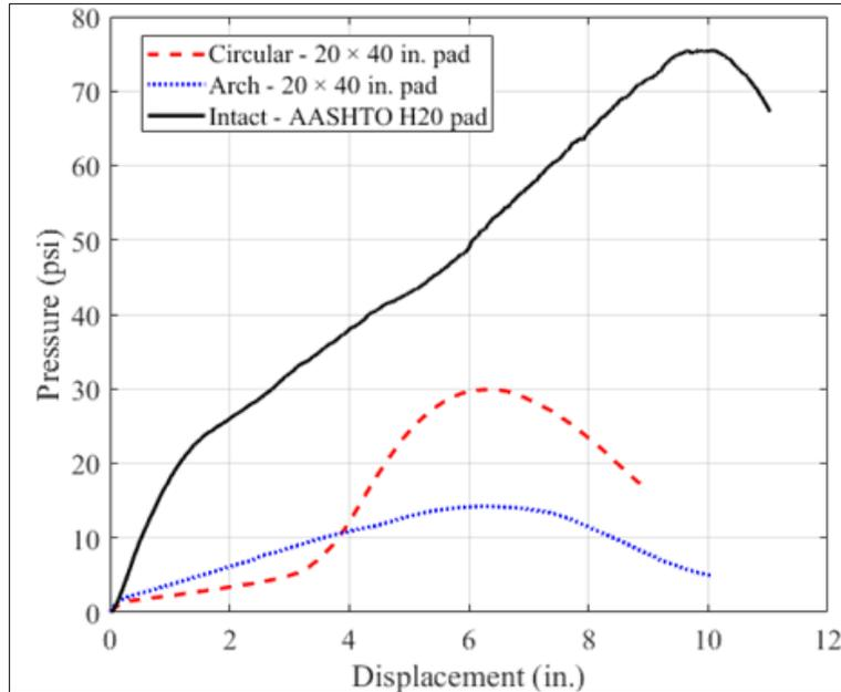
Figure 11-44. Control test: pressure on top of the CMP samples vs. soil settlement.
