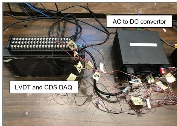
Figure 11-24. LVDT and CDS DAQ, and alternating current (AC) to direct current (DC) convertor (from left to right).
