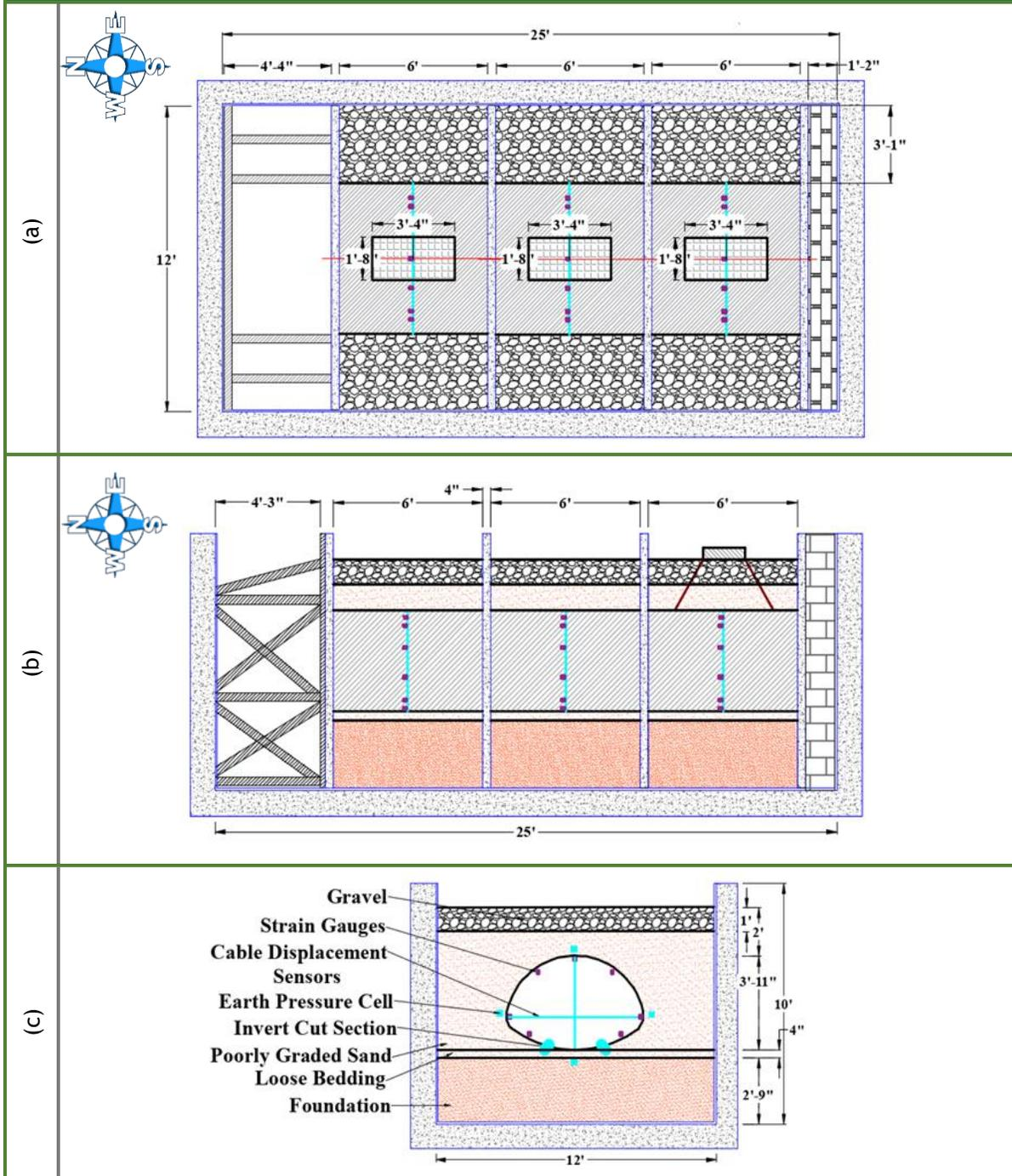
Figure 11-10. The CMP arch samples' burial configuration (SAPL renewed testing): (a) plan view, (b) profile view of the aligned CMP arch samples in the soil-box, and (c) cross sectional view of the CMP arch.
