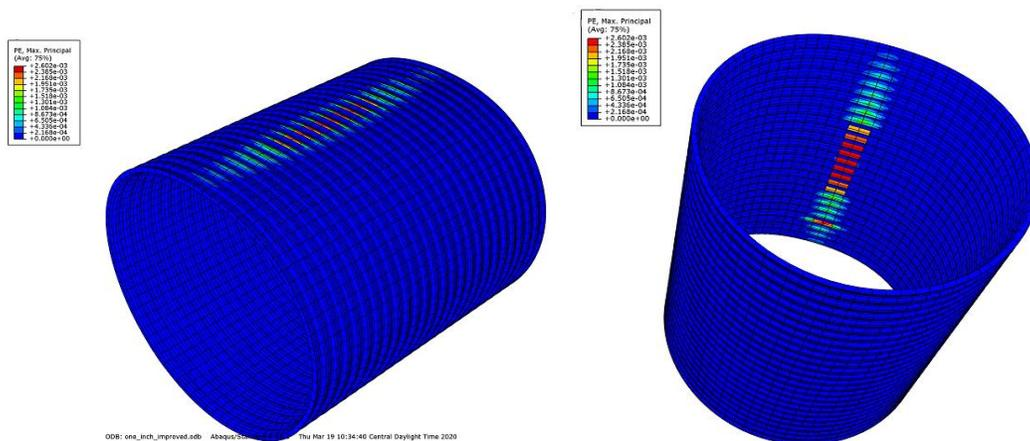
Figure 10-29. Plastic strain in the inside and outside the liner for 1 in. thick polymeric SAPL.
