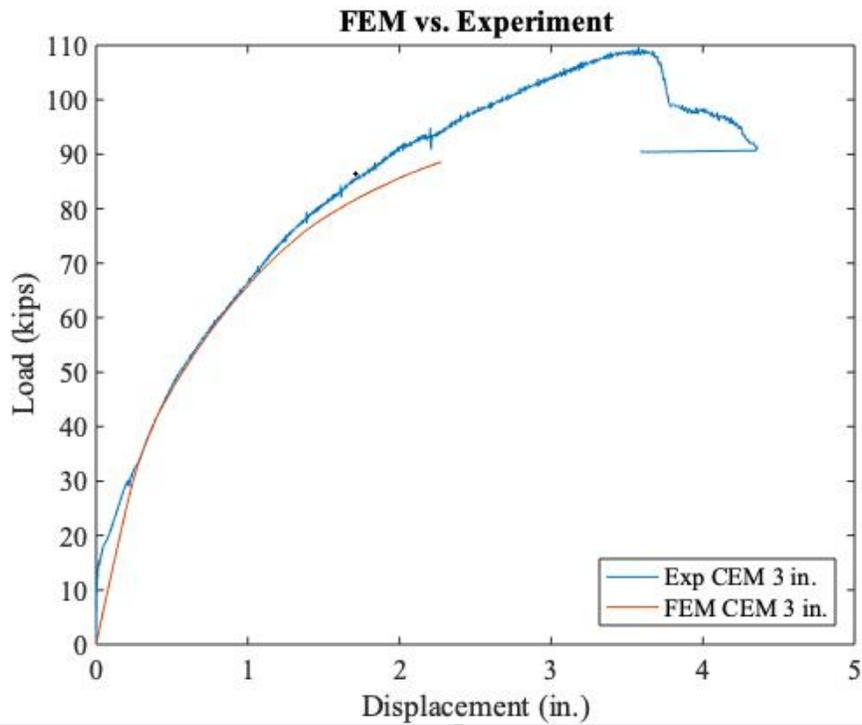
Figure 10F-7. Load displacement plot for 3-in. thick cementitious liner.
