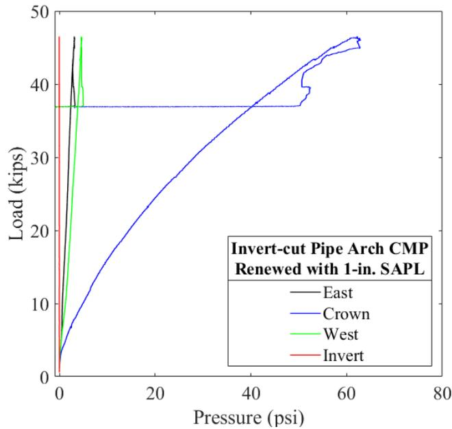
Figure 11-102. Load vs. pressure for the 1-in. thick SAPL renewed invert-cut CMP arch.
