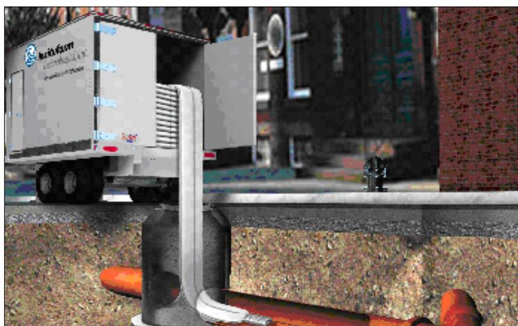
Figure 2-16. CIPP method installation process (Source: Insituform Technologies).
