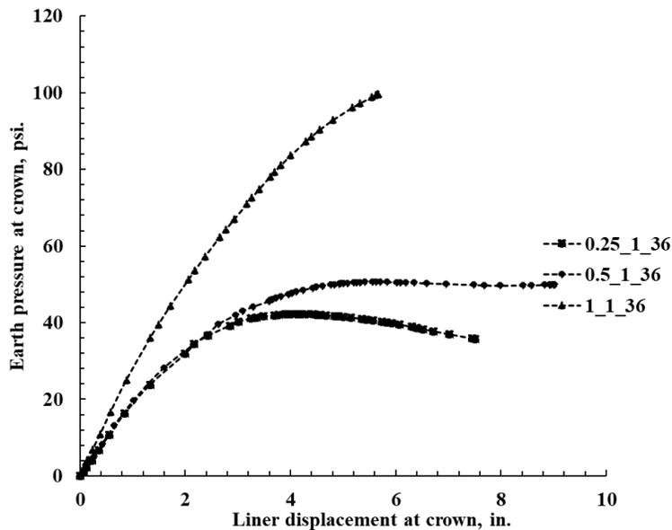
Figure 10E-24. Earth pressure 4 in. above the crown vs. crown displacement for invert-cut circular 36 in. CMPs with 1 ft cover and 0.25, 0.5, and 1 in. thick polymeric liner.
