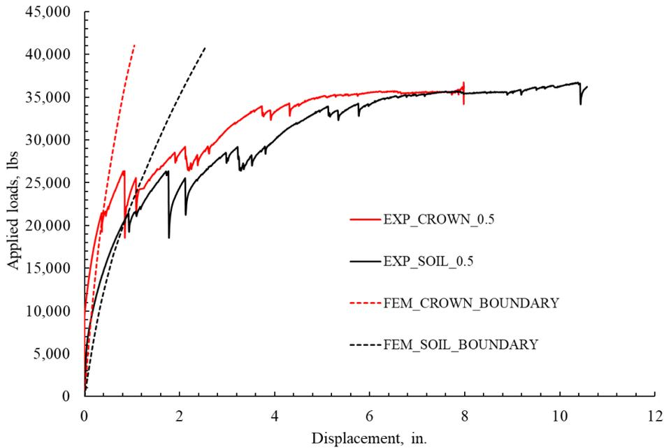
Figure 10-52. Load displacement curve comparison between FEM and Experiment for 0.5-in. thick polymeric SAPL with the boundary conditions at the end.
