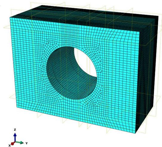
Figure 10-2. Soil model in FE with 2.4 in. mesh size.
