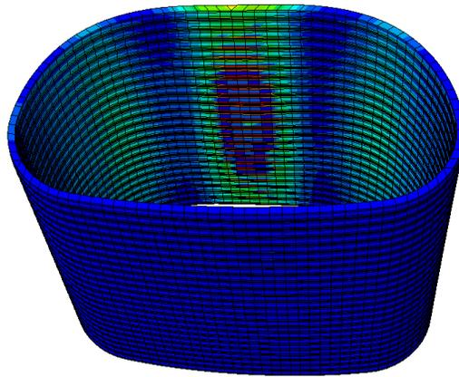
Figure 10E-6. Ultimate Von Mises stress around the liner at the ultimate load conditions for 1 in. thick arch polymeric liner.
