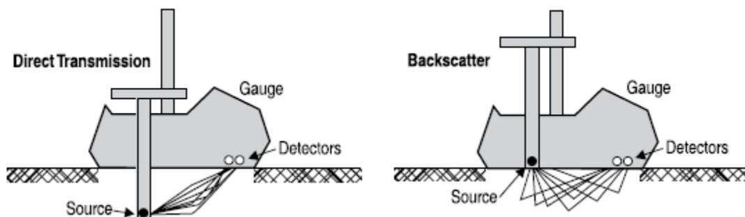
Figure 11-13. Modes of operation of nuclear density gauge (MULTIQUIP, 2018).
