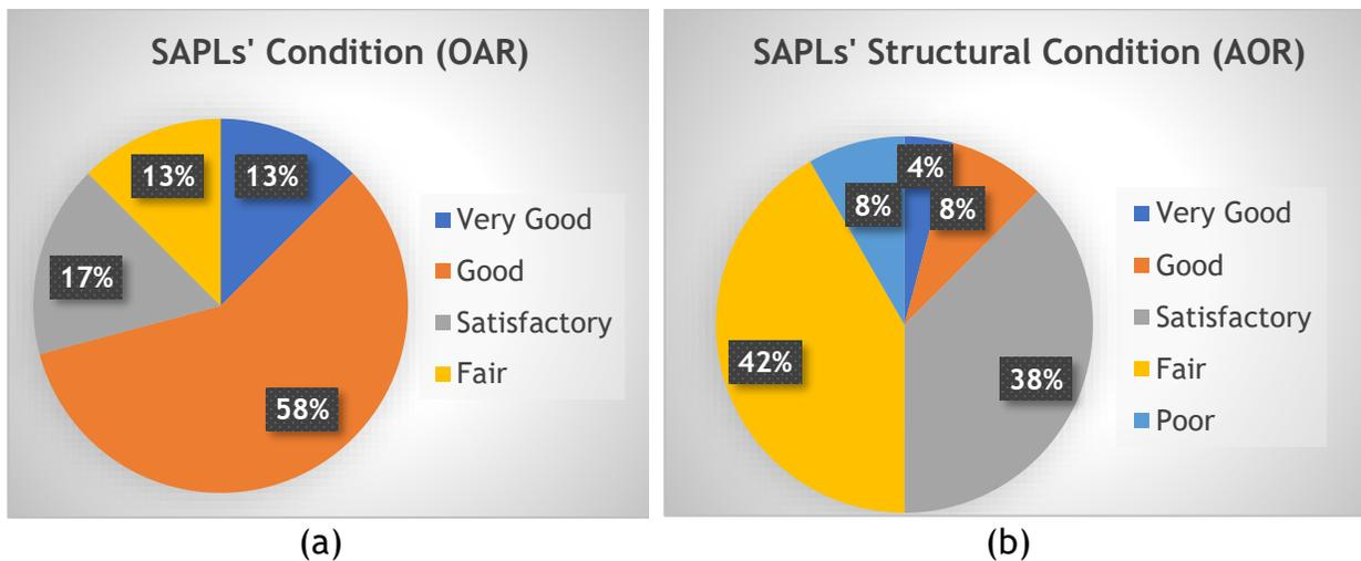
Figure 7-5. Condition assessment of SAPLs, (a) SAPL original condition given as percent of liner condition, (b) SAPLs structural condition given as percent of liner structural condition.
