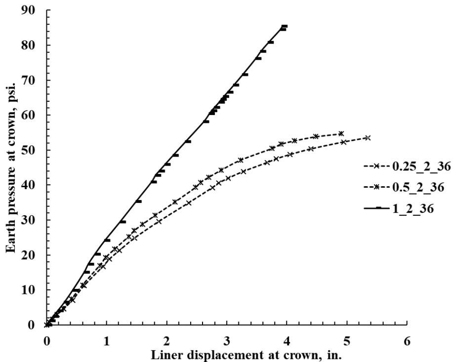
Figure 10E-22 Earth pressure at 4 in. above the crown vs. crown displacement for invert-cut circular 36 in. CMPs with 2 ft cover and 0.25, 0.5, and 1 in. thick polymeric liner.
