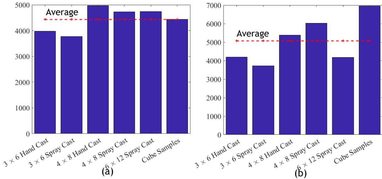
Figure 11-144. Bar chart results for: (a) 7 days, and (b) 28 days samples.
