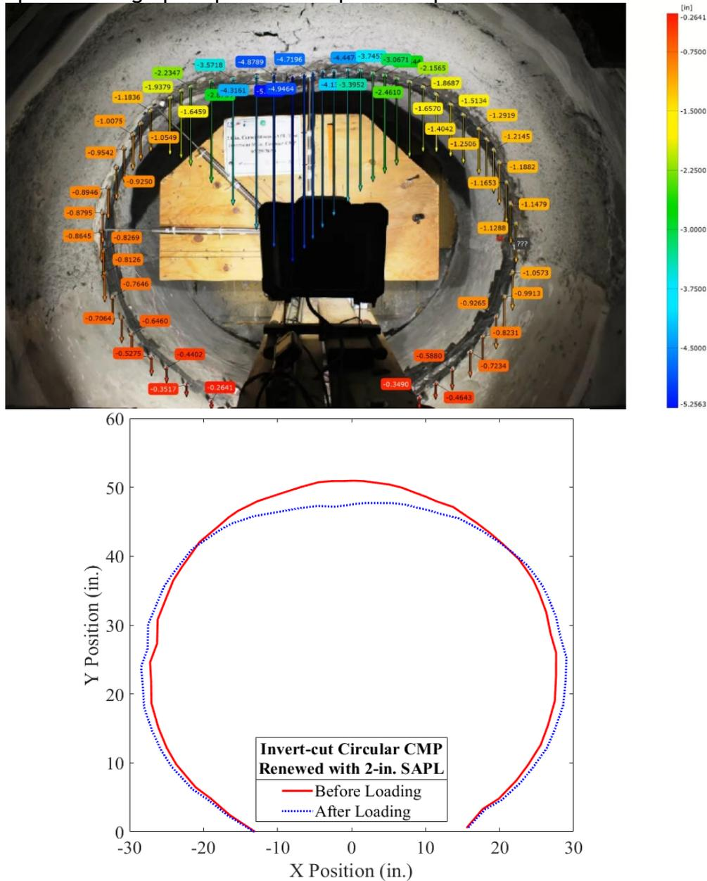
Figure 11-123. Pipe profiling using DIC for the 2-in. thick SAPL renewed invert-cut circular CMP.
