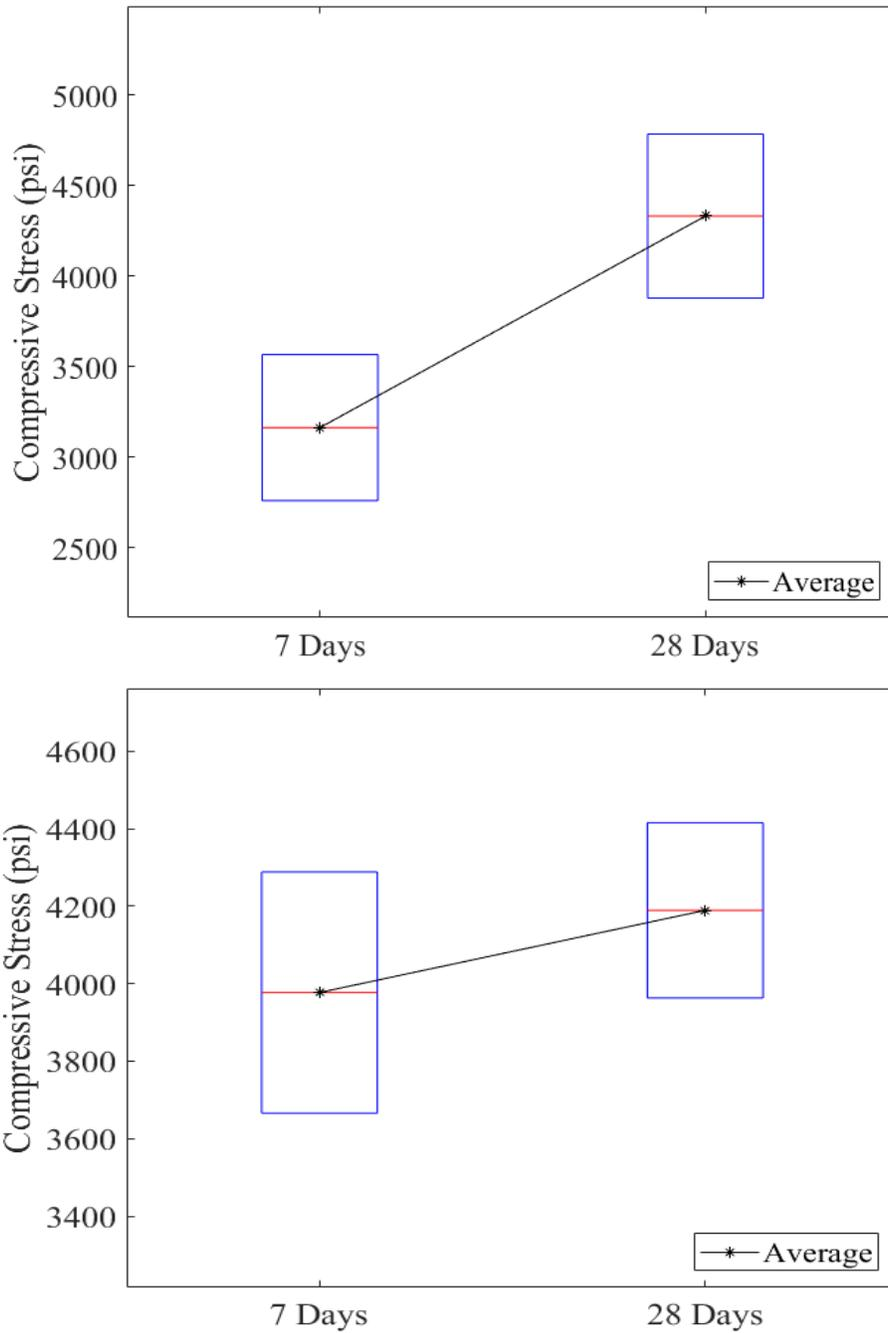
Figure 11-141. Box plot for the 3 × 6-cylinder samples taken from SAPL batch sprayed on circular CMPs: (top) spray cast, (bottom) hand cast.
