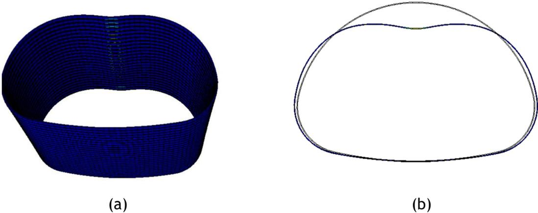
Figure 10-42. Deformation of the CMP at ultimate load condition for 0.25-in thick polymeric SAPL.
