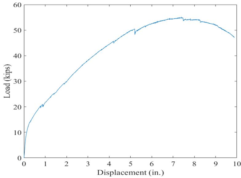
Figure 11-87. Invert-cut CMP arch renewed with 2-in. thick cementitious SAPL subjected to static live load: (top) load-time and (bottom) load-soil displacement graphs.
