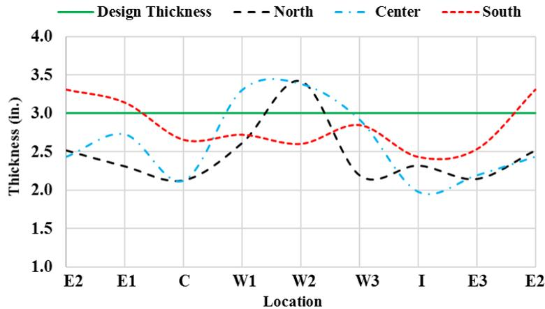
Figure 11-85. Thickness measurement for the 3-in. thick cementitious SAPL renewed CMP arch.
