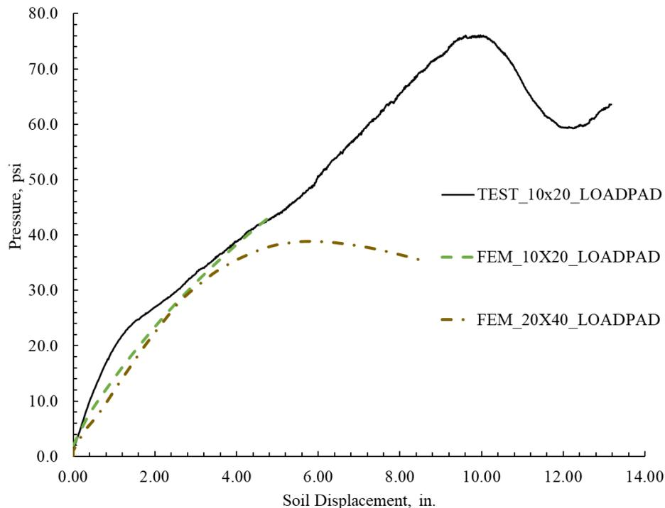
Figure 10-18. Earth pressure comparison for the bigger and smaller load pad conditions.
