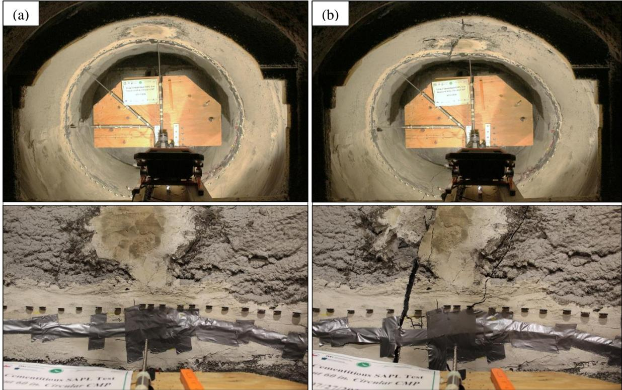
Figure 11-109. Invert-cut circular CMP renewed with 3 in. cementitious SAPL:
