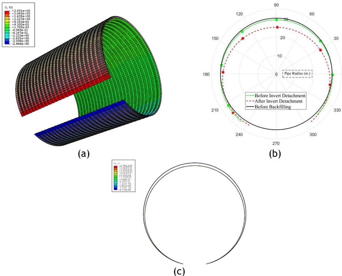
Figure 10-19. (a) Reduction in the invert gap from FEM (b) Experimental recording of the reduction in invert gap by Digital Image Processing (Darabnoush Tehrani, et al., 2020) (c) Vertical diameter change from FEM after invert removal.
