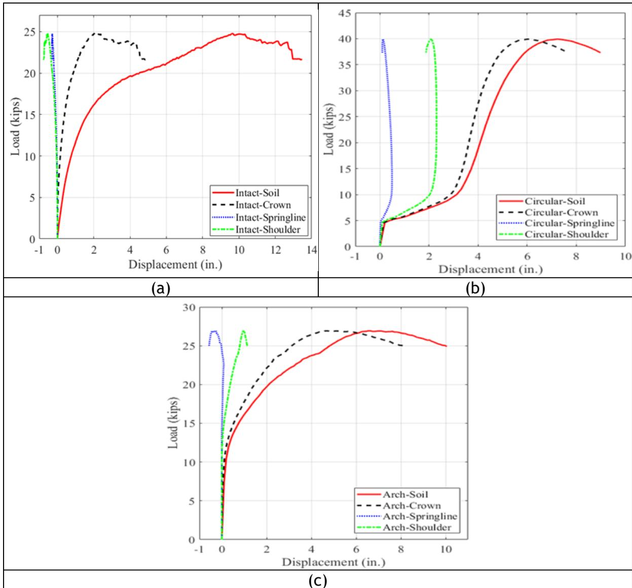
Figure 11-52. Load versus displacement of CMPs at different locations for the control test: (a) intact 60 in. circular CMP under a 10×20 in. steel load pad, (b) invert-cut 60 in. circular CMP under a 20×40 in. steel load pad, and (c) invert-cut 47×71 in. arch CMP under a 20×40 in. steel load pad.
