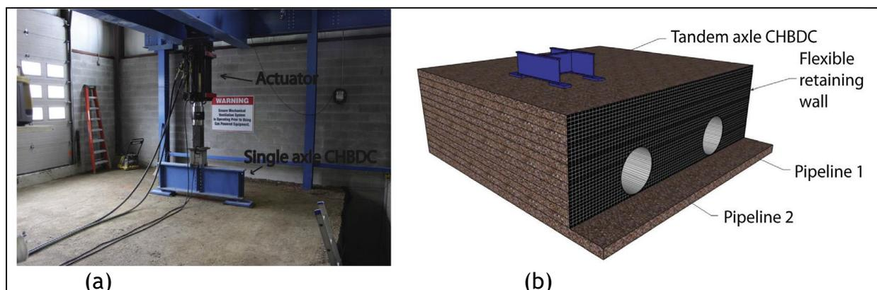
Figure 2-28. Soil box laboratory testing of corrugated metal pipes: (a) single axle loading configuration, and (b) schematic tandem axle loading configuration (Garcia and Moore 2015).
