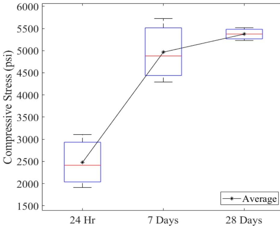
Figure 11-142. Box plot for the 4 × 8-cylinder samples taken from SAPL batch sprayed on circular CMPs: (top) spray cast, (bottom) hand cast.
