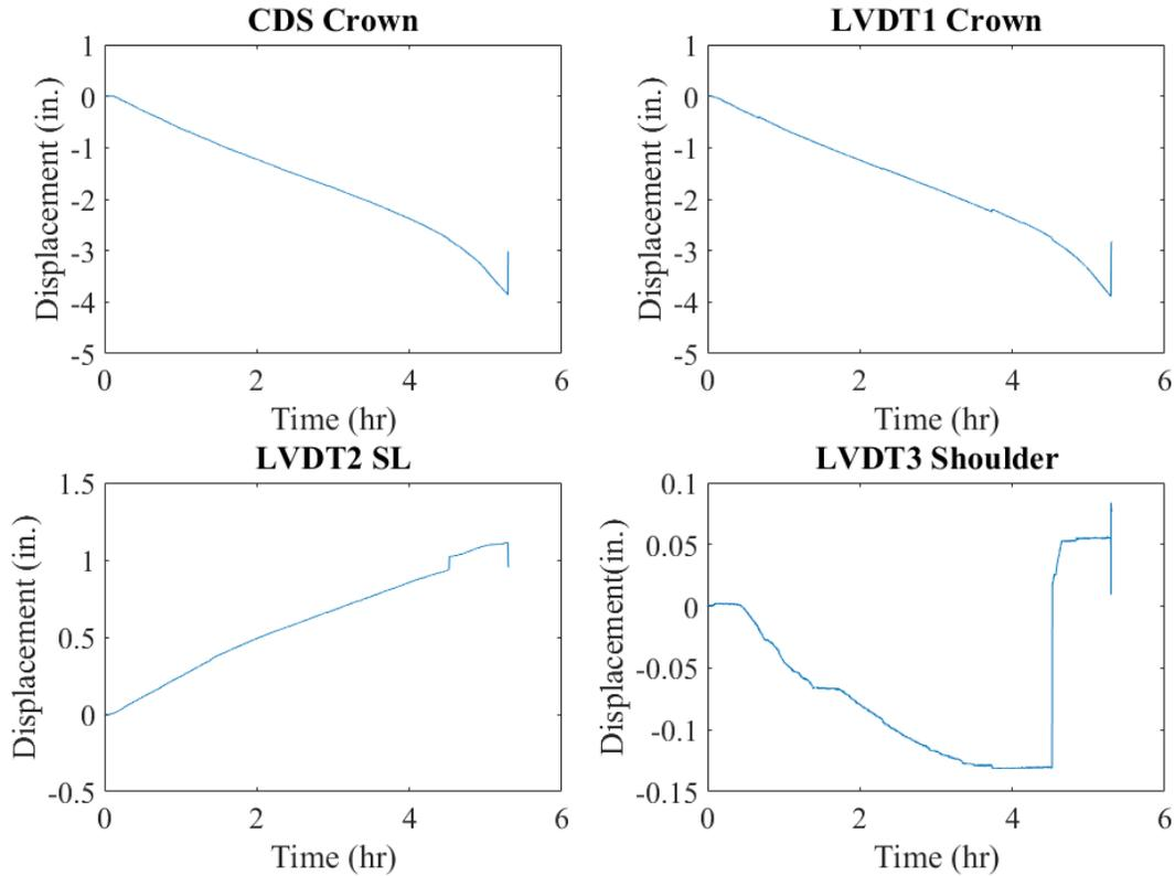
Figure 11-130. Mechanical sensors result for 1-in. thick SAPL renewed invert-cut circular CMP.
