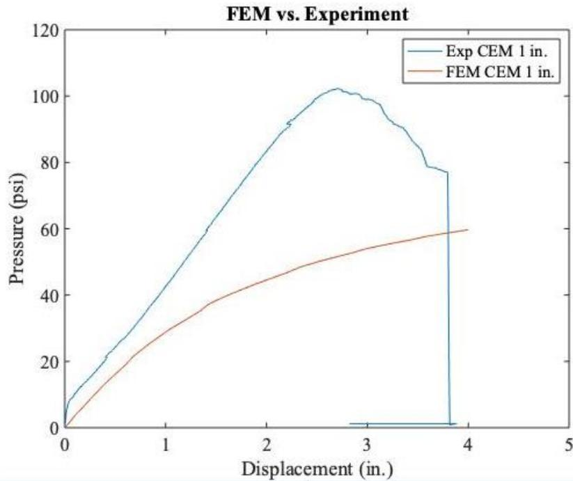
Figure 10F-2. Earth pressure at 4 in. above the crown vs. crown displacement for 1-in. thick cementitious liner.
