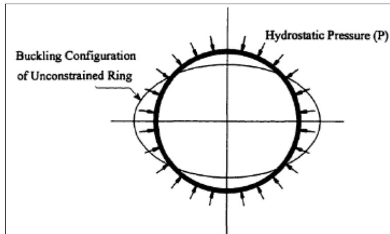
Figure 2-10. Bresse Model for calculating the critical buckling pressure of a thin unconstrained circular ring under external hydrostatic pressure.
