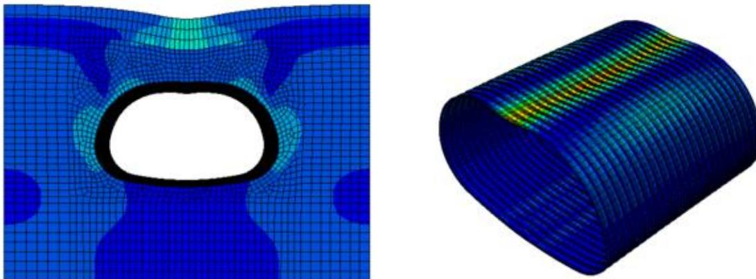
Figure 8. Finite element modeling of the soil box testing.
