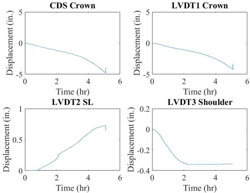
Figure 11-80. Mechanical sensors result for 3-in. thick SAPL renewed invert-cut CMP arch.
