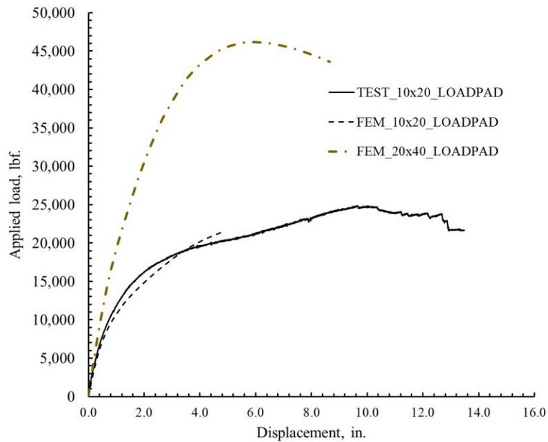
Figure 10-17. Effect of load pad size on the load- soil settlement under the load.
