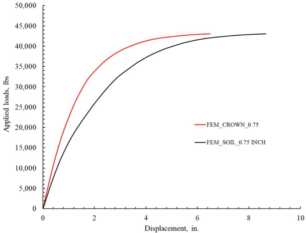
Figure 10E-10. Load displacement plot of crown displacement and soil settlement from FE analysis for 0.75-in. thick arch polymeric liner.
