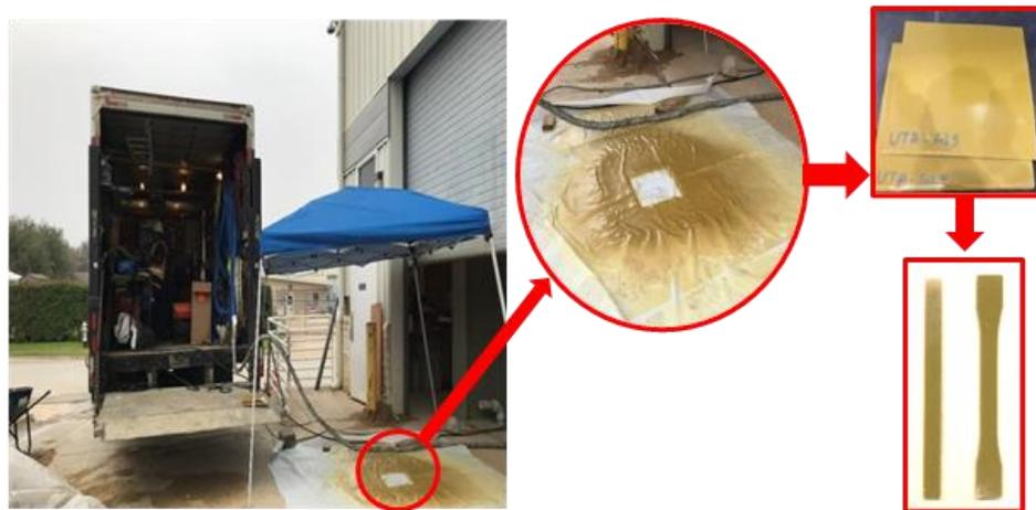
Figure 11-34. Plate sampling from the SAPL batch to provide material test samples for CMP arch test setup.
