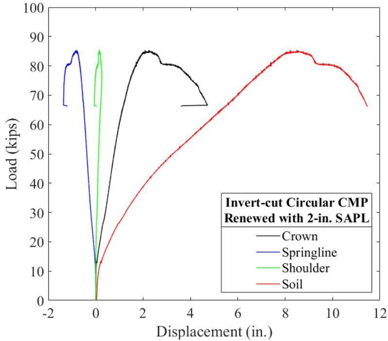
Figure 11-124. Load vs. displacement of the soil surface, crown, springline, and shoulder of the 2-in. thick SAPL renewed invert-cut circular CMP due to the applied static load.
