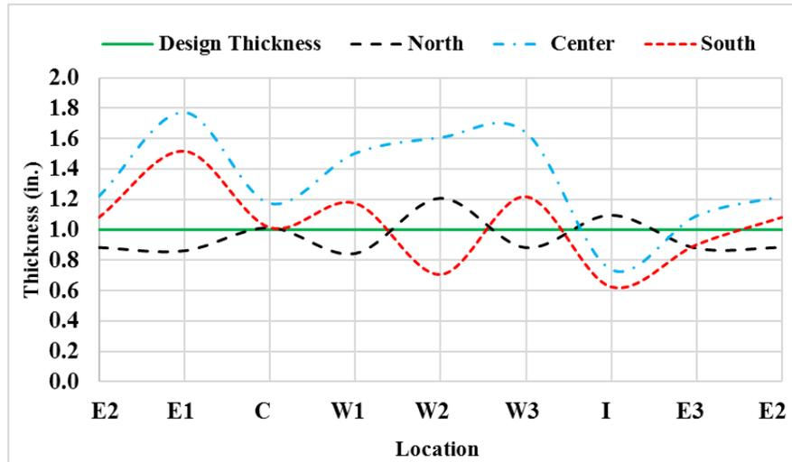
Figure 11-103. Thickness measurement for the 1-in. thick cementitious SAPL renewed CMP arch.
