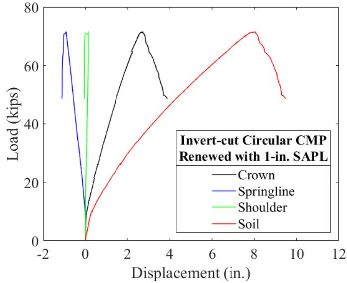
Figure 11-133. Load vs. displacement of the soil surface, crown, springline, and shoulder of the 1-in. thick SAPL renewed invert-cut circular CMP due to the applied static load.
