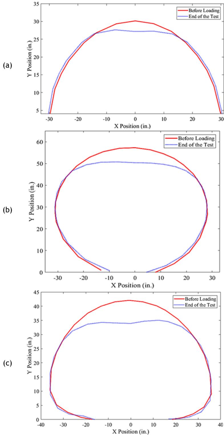
Figure 11-56. Pipe profiling using DIC results before loading and after loading at the ultimate load carrying capacity of the samples: (a) intact CMP, (b) invert-cut circular CMP, and (c) invert-cut CMP arch.
