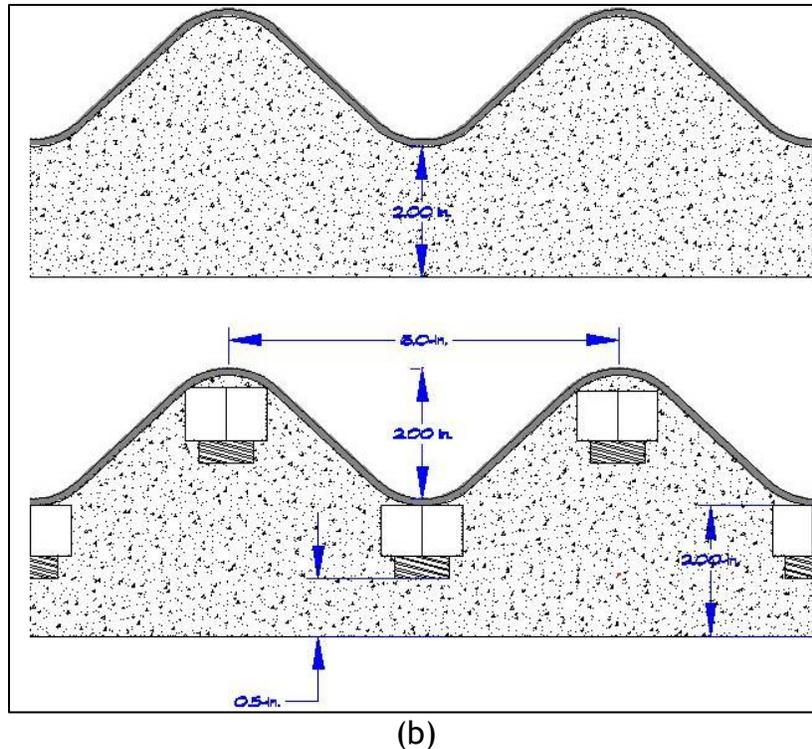
Figure 4-5. Linings in a 6×2-in. corrugation profile CMP: (a) not filling the corrugations and (b) filling the corrugations.
