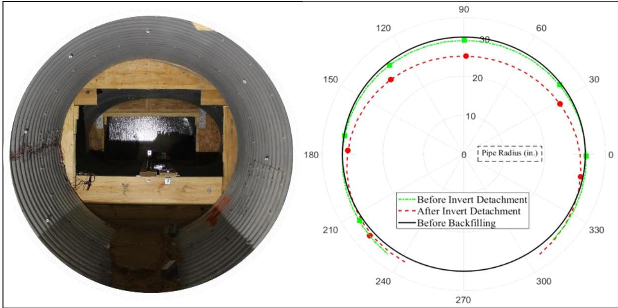
Figure 11-41. 60-in. invert-cut circular bare CMP, pipe profiling using DIC technique.
