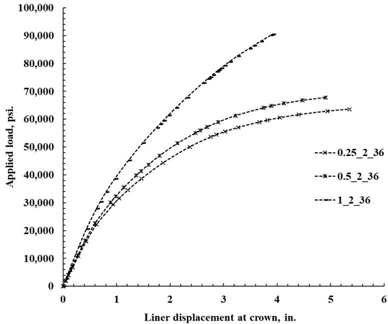
Figure 10E-21. Load displacement plot for invert-cut circular 36 in. CMPs with 2 ft cover and 0.25, 0.5, and 1 in. thick polymeric liner.
