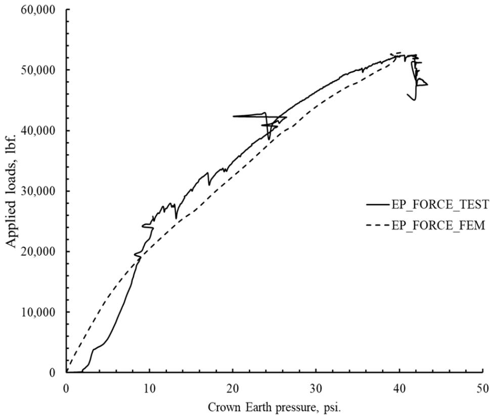
Figure 10B- 4. Comparison of the earth pressure with the applied load for 0.5 in. thick polymeric circular liner.
