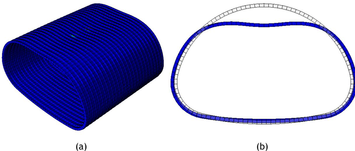
Figure 10-55. (a) Development of plastic strain in the inside liner for 1.5 in. thick arch SAPL, and (b) Deformation pattern for 1.5-in. thick arch polymeric liner.
