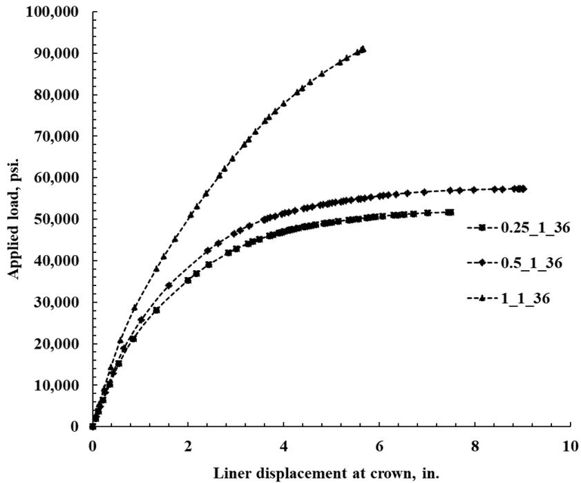
Figure 10E-23. Load displacement plot for invert-cut circular 36 in. CMPs with 1 ft cover and 0.25, 0.5, and 1 in. thick polymeric liner.
