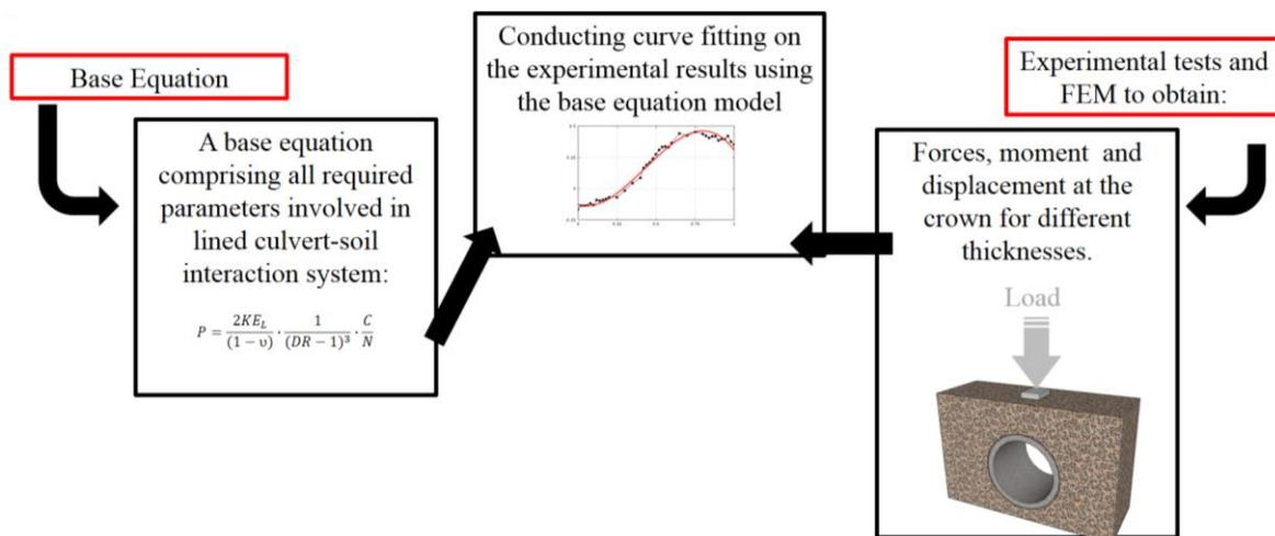
Figure 7. Design equation development methodology.
