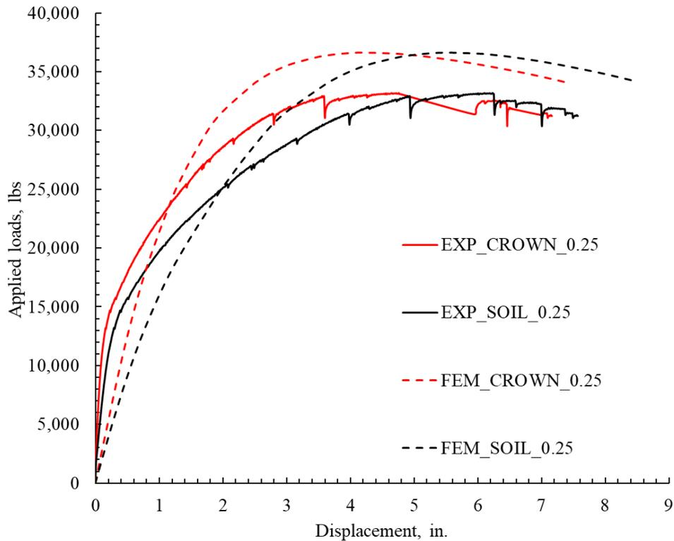
Figure 10-53. Load displacement curve comparison between FEM and Experiment for 0.5-in. thick polymeric SAPL with the boundary conditions at the end.
