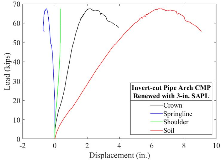
Figure 11-83. Load vs. displacement of the soil surface, crown, springline, and shoulder of the 3-in. thick SAPL renewed invert-cut CMP arch due to the applied static load.
