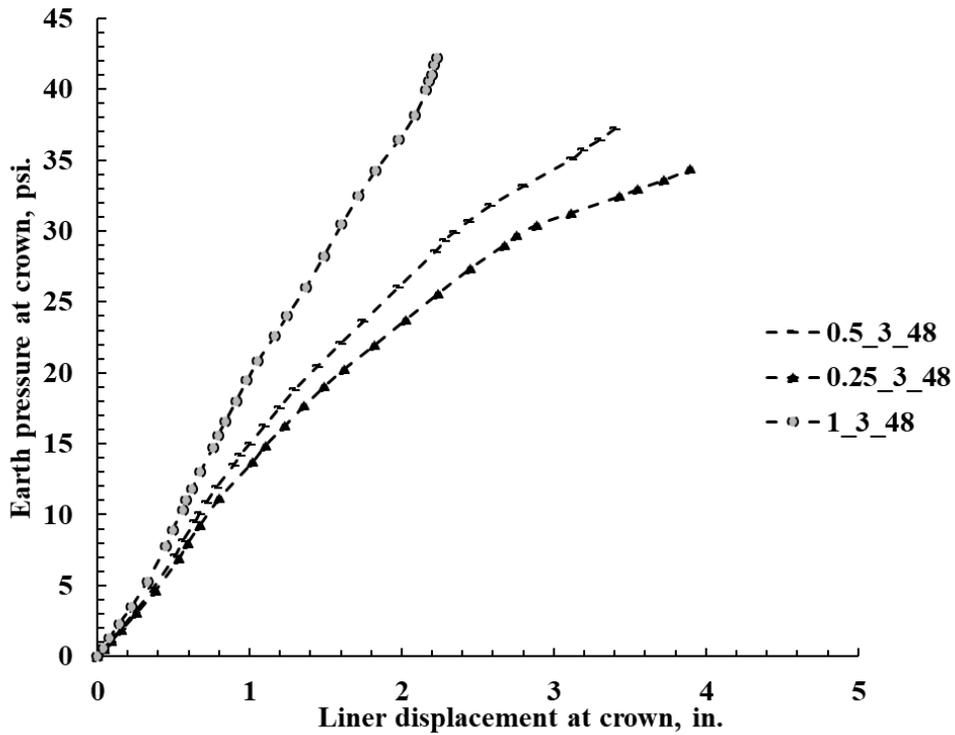
Figure 10E-14. Earth pressure at 4 in. above the crown vs. crown displacement for 48 in. invert-cut circular CMPs with 3 ft cover and 0.25, 0.5, and 1 in. thick polymeric liner.
