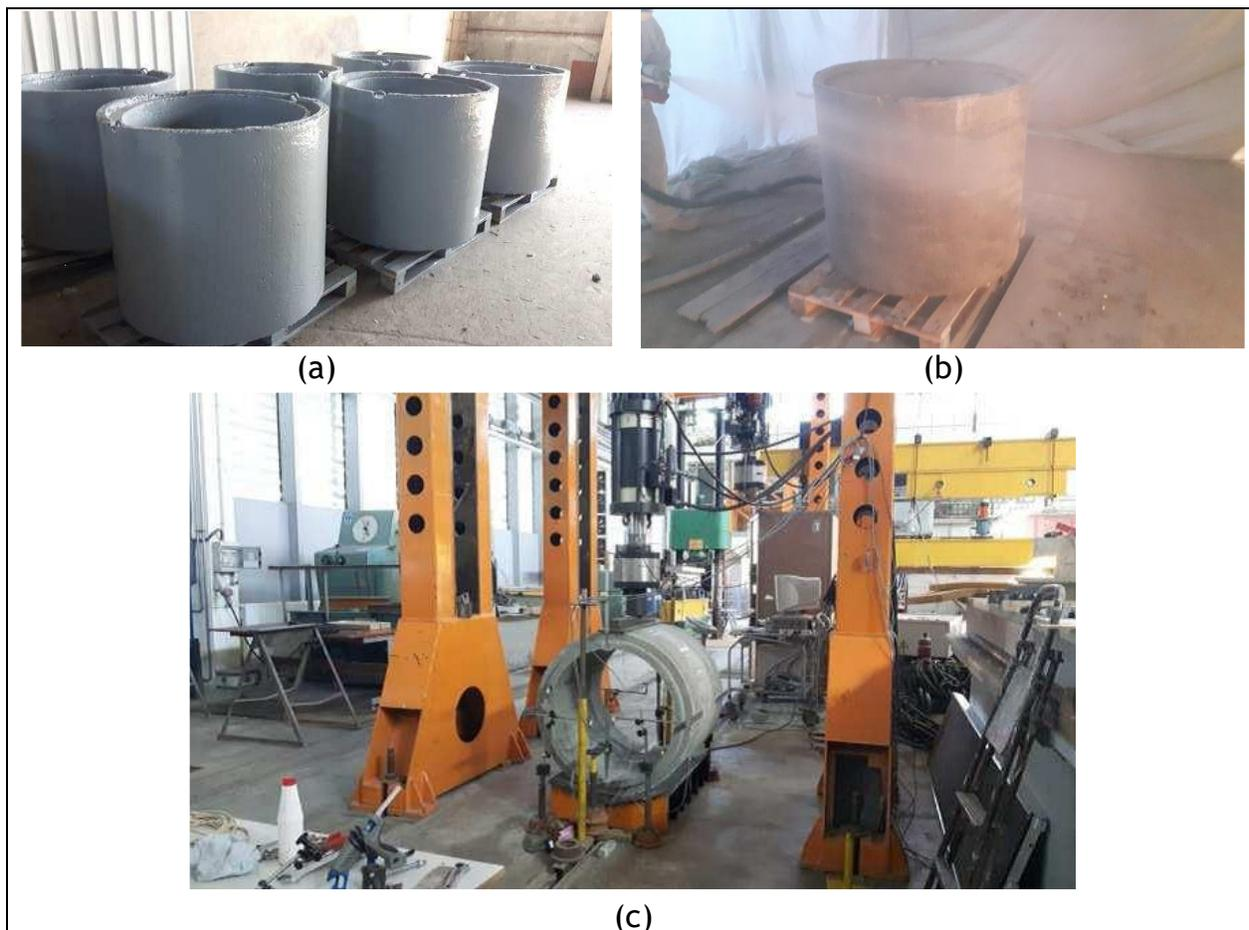
Figure 2-25. Dead-load testing of reinforced concrete pipes (RCPs) renewed with polymeric SAPLs: (a) tested concrete rings covered by polyurea coating, (b) spraying polyurea coating system on concrete ring, and (c) D-load testing frame (Szafran and Matusiak 2017).
