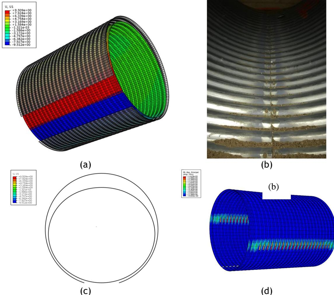
Figure 10-20. Complete closure of the invert after loading (a), (c) from FEM (b) closure of invert seen in the Experiment (d) plastic strain at the spring line area.
