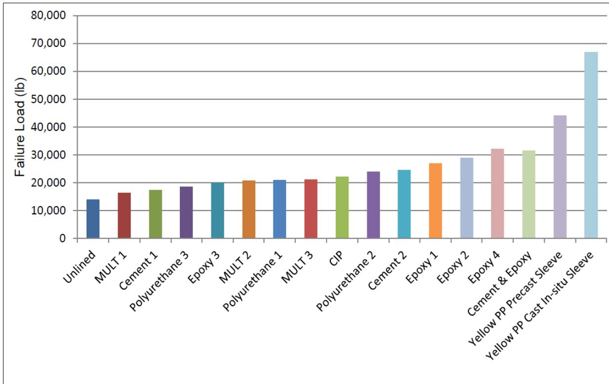
Figure 2-21. Significant increase in renewed CRP structural capacity (Entezarmahdi, 2015).
