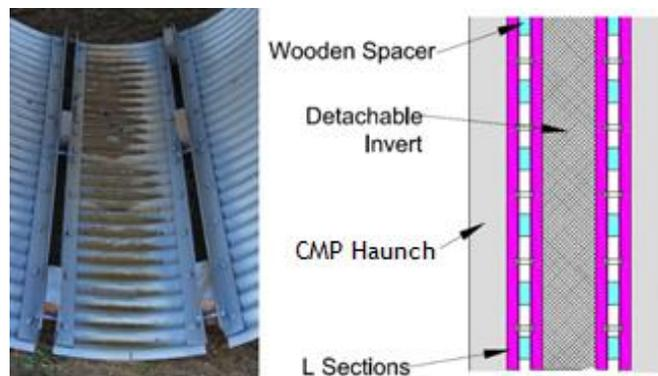
Figure 11-16. Detachable invert section for control test.
