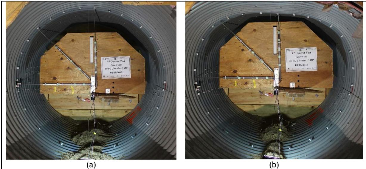
Figure 11-47. 60-in. Invert-cut circular CMP soil box testing: (a) before loading and (b) after loading.
