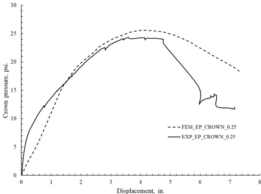
Figure 10-45. Comparison of the earth pressure at crown plotted against the soil displacement for 0.25-in. thick arch polymeric SAPL.
