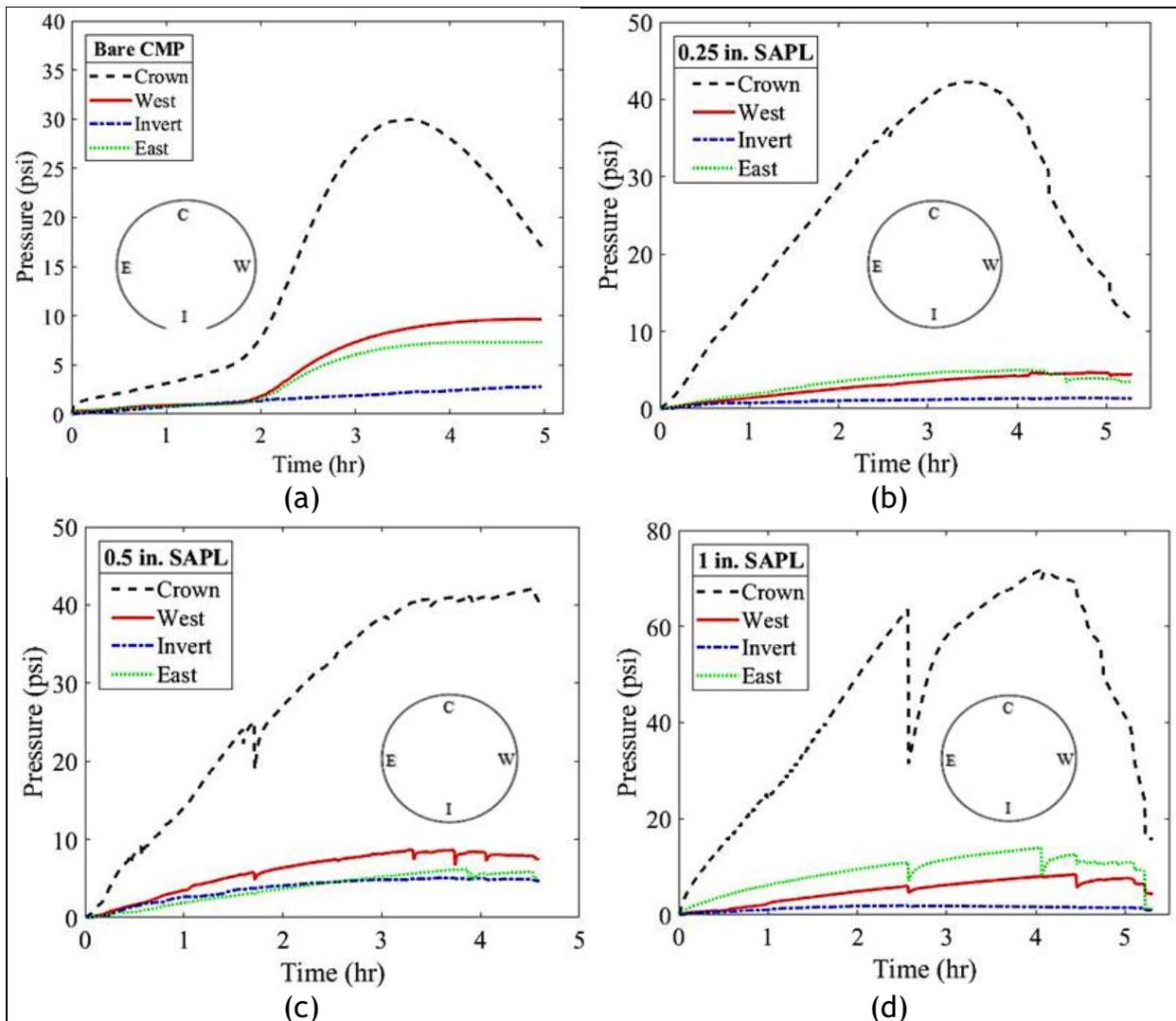
Figure 11-62. Earth pressure cells' results: (a) bare circular CMP, (b) 0.25 in. SAPL renewed circular CMP (c) 0.5 in. SAPL renewed circular CMP and (d) 1 in. SAPL renewed circular CMP.
