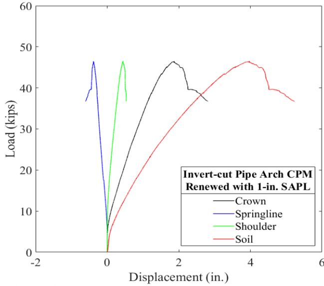
Figure 11-101. Load vs. displacement of the soil surface, crown, springline, and shoulder of the 1-in. thick SAPL renewed invert-cut CMP arch due to the applied static load.
