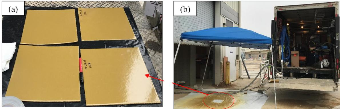
Figure 11-33. SAPL sampling for circular CMPs test setup: (a) sample plates prior to the cut into required shape for flexural and tensile test, and (b) the sampling site with Sprayroq installation truck.
