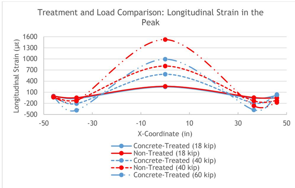
Figure 2-29. Comparison of longitudinal strain at peak of corrugation before and after paving (Sargand et al. 2015).
