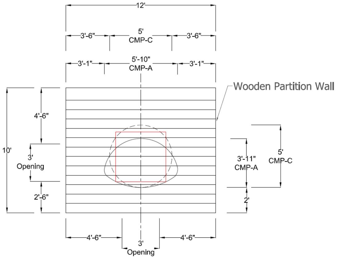
Figure 11-4. Initial schematic design of the wooden partition wall.
