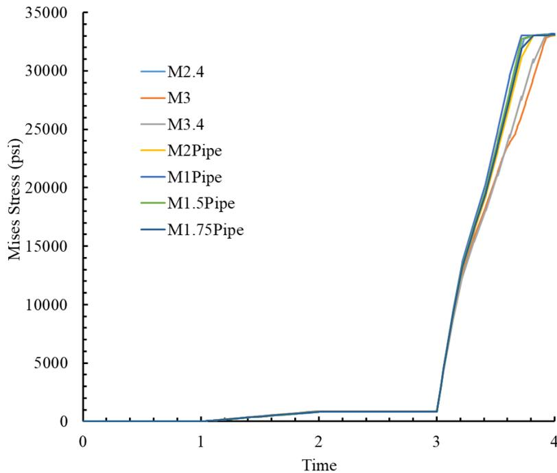
Figure 10-8. Von Mises Stress in the pipe.
