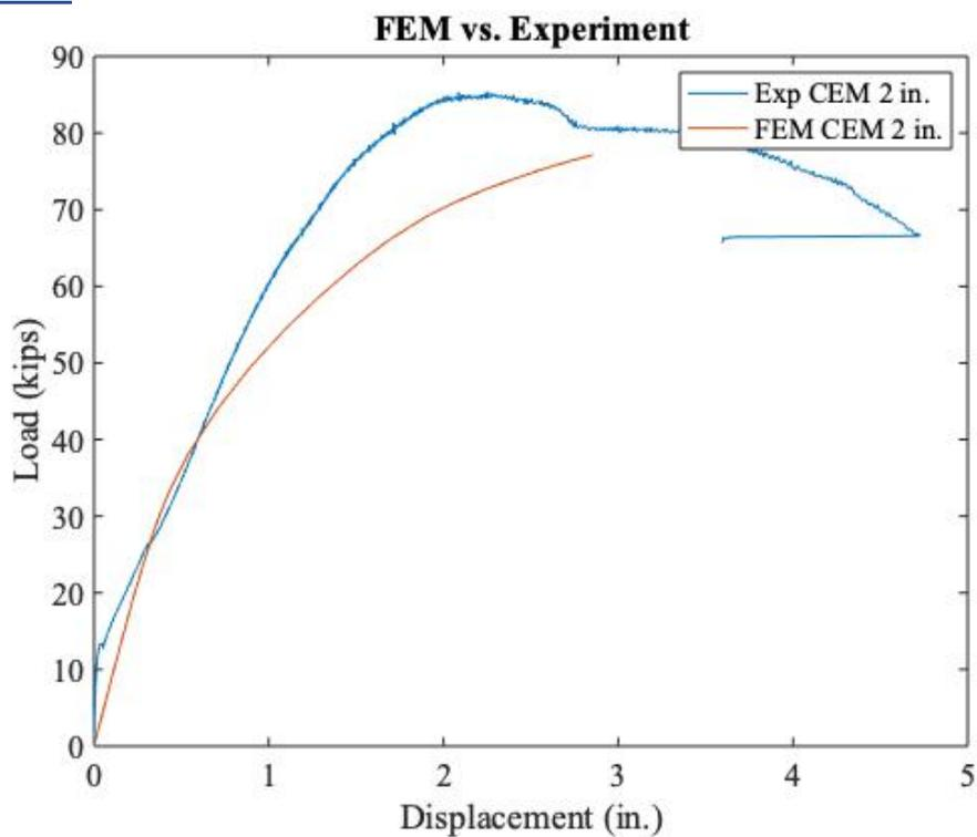
Figure 10F-4. Load displacement plot for 2-in. thick cementitious liner.
