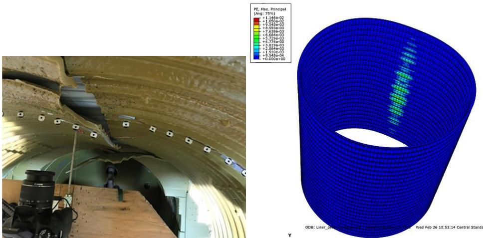
Figure 10-28. Crack in the CMP (Left) Plastic strain in the crown from FE model (Right) of the CMP at the ultimate load conditions for 0.5 in. thick polymeric SAPL.
