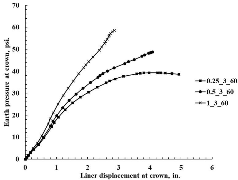
Figure 10D-2. Earth pressure at 4 in. above the crown vs. crown displacement for 60-in. invert-cut circular CMP with 3-ft cover and 0.25-, 0.5-, and 1-in. polymeric circular thick liner.
