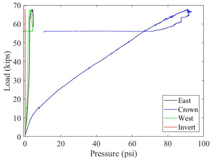
Figure 11-84. Load vs. pressure for the 3-in. thick SAPL renewed invert-cut CMP arch.
