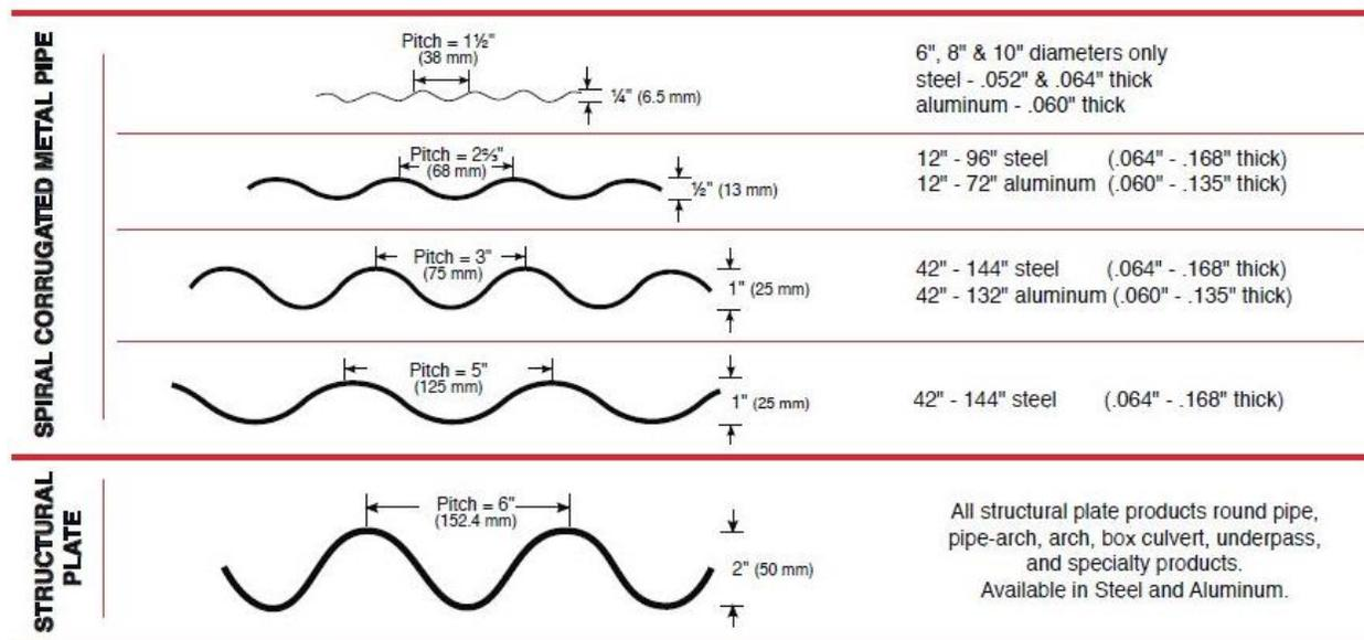
Figure 4-2. CMP profiles in North America, (Source: PCPIPE, Website: <http://www.pcpipe.com>).
