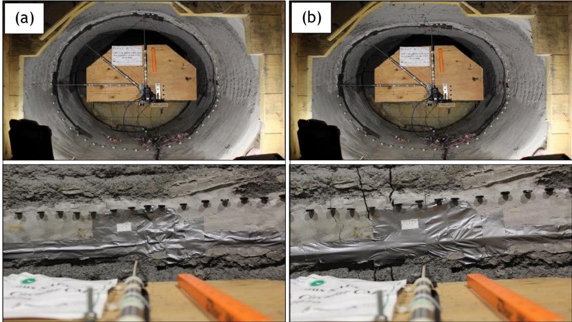
Figure 11-127. Invert-cut circular CMP renewed with 1 in. cementitious SAPL:
