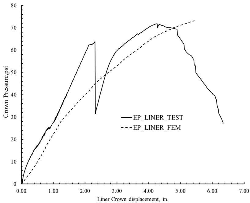
Figure 10B- 8. Comparison of the earth pressure with liner's crown disp., for 1-in. thick polymeric circular liner.
