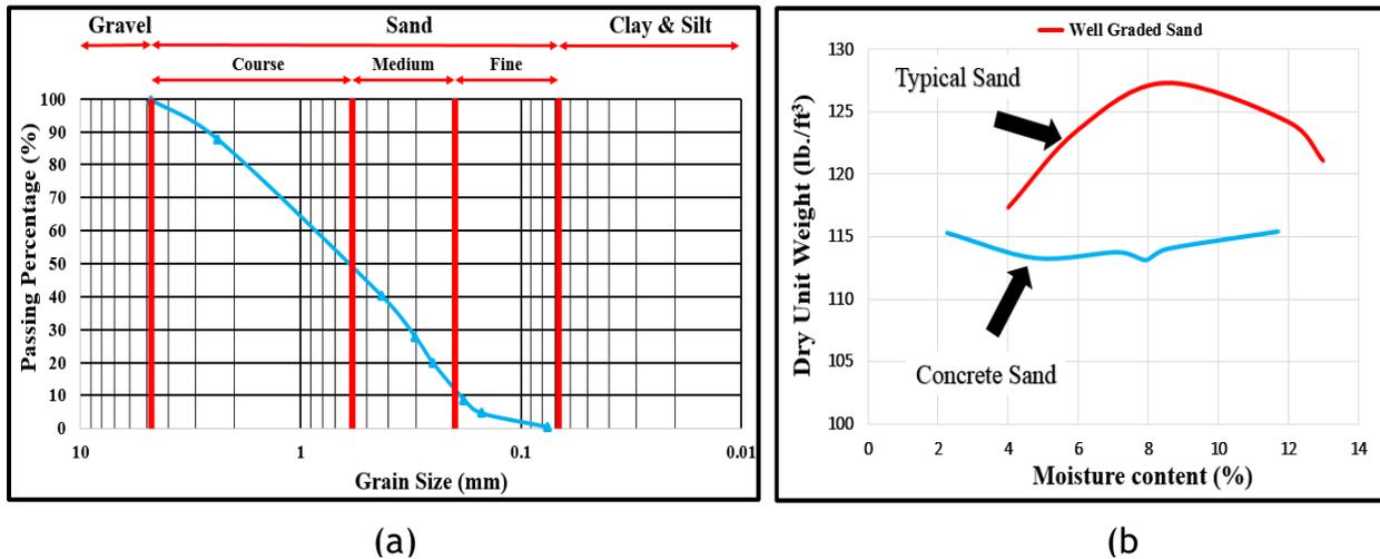
Figure 11-7. Embedment soil characteristics: a) soil sieve analysis, and b) standard Proctor test.
