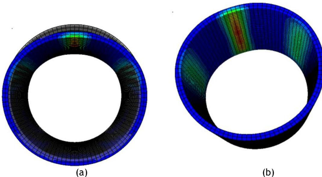
Figure 10F-6. (a) Deformation of 2 in. thick cementitious liner under ultimate load, and (b) crack location in 2-in. thick cementitious liner.
