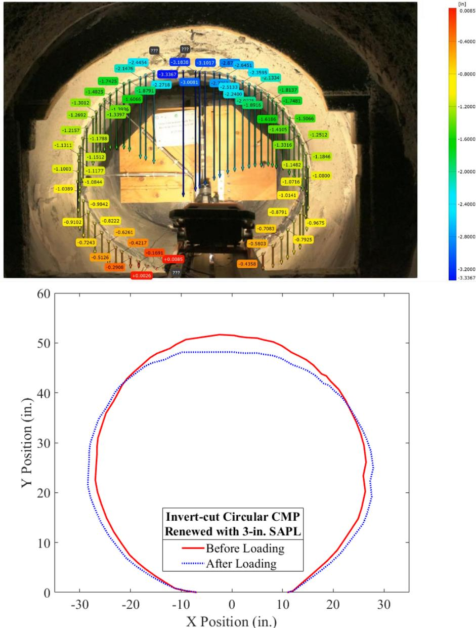
Figure 11-114. Pipe profiling using DIC for the 3-in. thick SAPL renewed invert-cut circular CMP.
