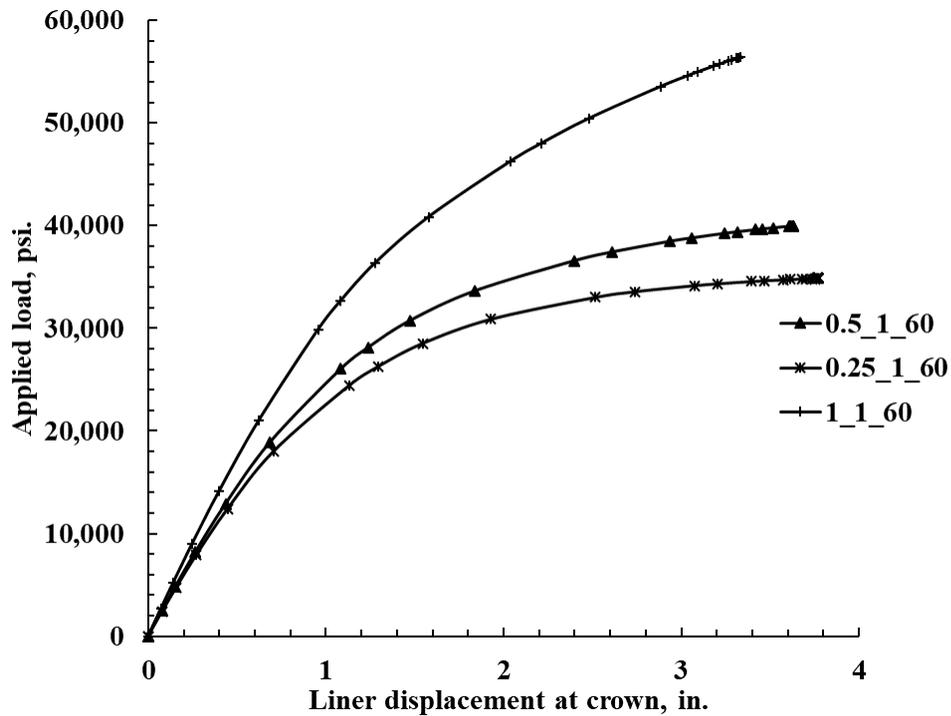
Figure 10D-3. Load displacement plot for 60-in. invert-cut circular CMP with 1-ft cover and 0.25-, 0.5-, and 1-in. thick polymeric circular liner.
