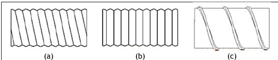
Figure 2-12. Types of corrugated metal pipes (CMPs): (a) helical, (b) annular and (c) spiral rib CMPs.
