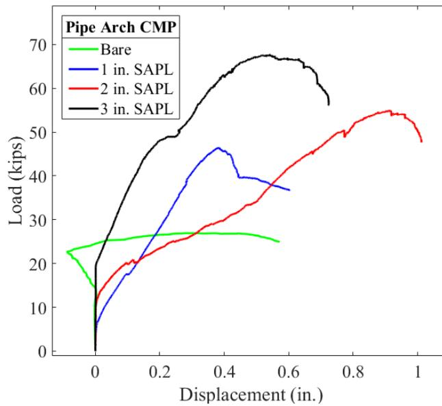
Figure 11-106. Load vs. springline displacement comparison graph.
