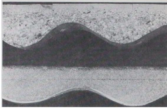
Figure 4-1. The Upper section of the concrete lining was made by spinning the pipe, the lower section was made with the pipe stationary, (Source: Construction Products Division of Armco, Inc.).
