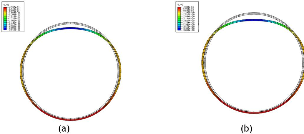
Figure 10B- 5. Deformation of the liner at (a) 1<sup>st</sup> plastic strain (b) at ultimate load conditions for 1-in. thick polymeric circular liner.
