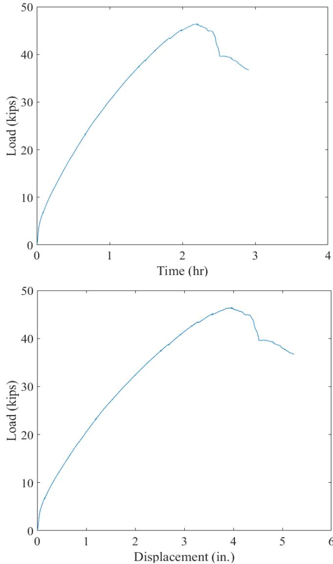
Figure 11-96. Invert-cut CMP arch renewed with 1-in. thick cementitious SAPL subjected to static live load: (top) load-time, and (bottom) load-soil displacement graphs.
