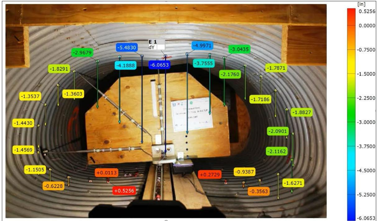
Figure 11-51. Result of DIC measurement at the end of the test (47×71 in. invert-cut arch CMP).
