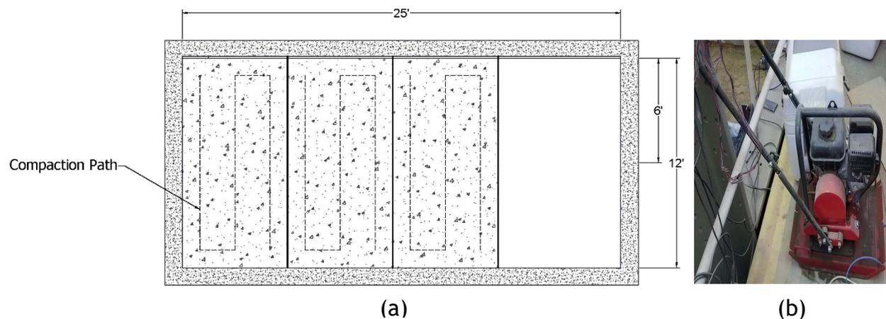
Figure 11-6. Foundation compaction: (a) schematic illustration of soil compaction, (b) soil compaction using a 4,496 lbs vibratory plate compactor.
