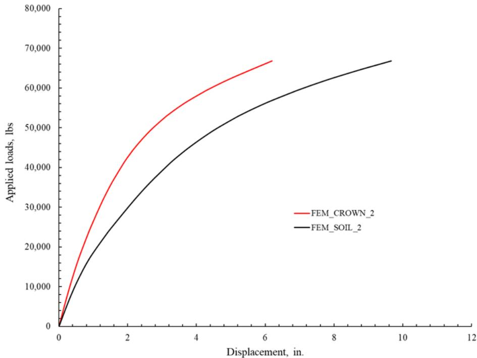
Figure 10E-12. Load displacement plot of crown displacement and soil settlement from FE analysis for 2.0-in. thick arch polymeric liner.
