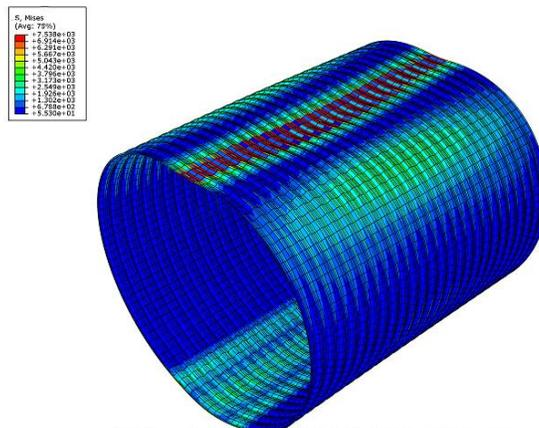
Figure 10-24. Stress distribution in the pipe at the ultimate load conditions for 0.25-in. thick polymeric SAPL.
