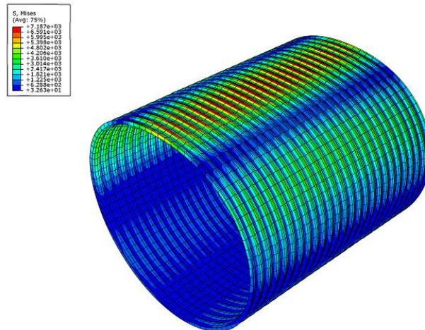
Figure 10B- 6. Von Mises stress around the liner at the ultimate load conditions for 1 in. thick polymeric circular liner.
