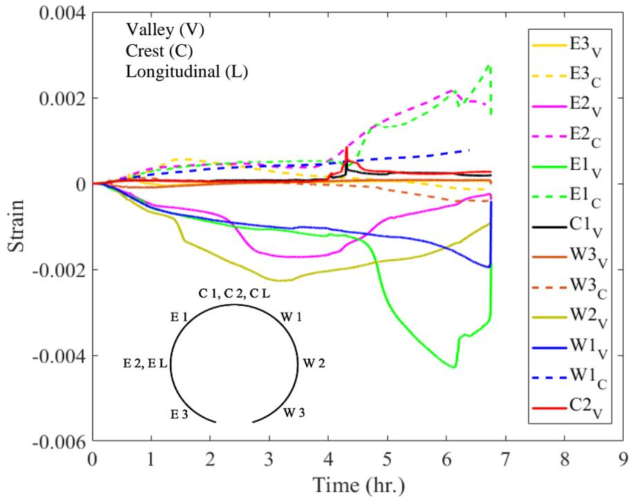
Figure 11-113. Strain gauge result for 3-in. thick SAPL renewed invert-cut circular CMP.
