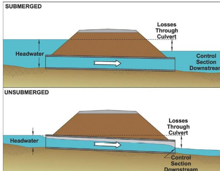
Figure 2-6. Typical “outlet control” flow in both full flow (submerged) and partly full flow (unsubmerged) conditions (FHWA 2012).
