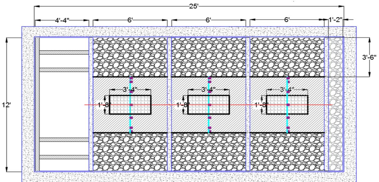
Figure 11-3. Soil box configuration for three CMP samples divided by wooden partition walls.
