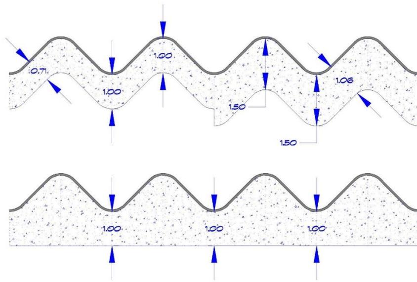
Figure 4-4. 3x1-in. CMP profile lined with SAPL.
