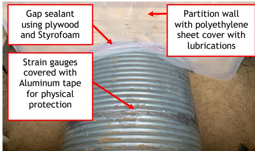
Figure 11-18. Pipe installation and preparation before backfilling.
