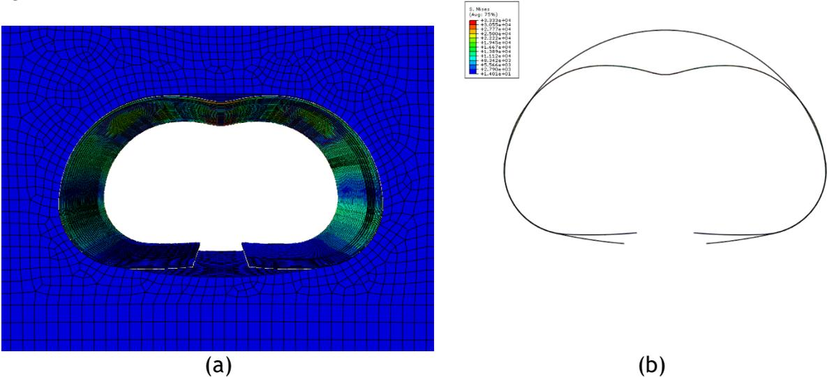
Figure 10-37. (a) Bending of the arch CMP along the crown after complete loading (b) Vertical diameter change from FEM after complete loading.
