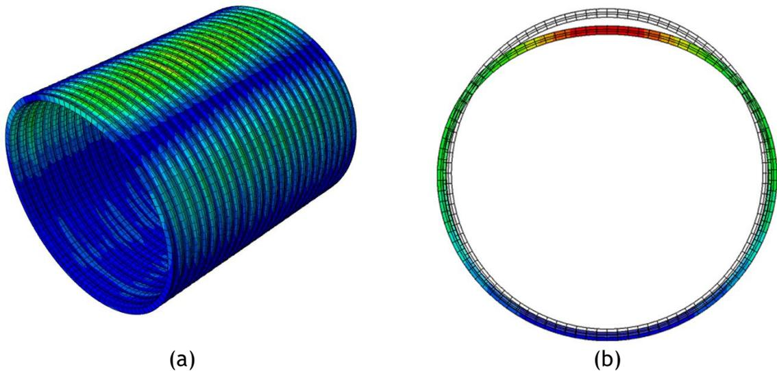
Figure 10-31. (a) Ultimate von Mises stress distribution around the liner and (b) Deformation pattern for 1.5- in. thick polymeric SAPL.
