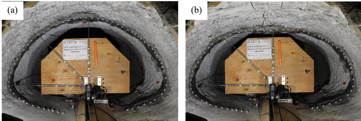
Figure 11-86. Invert-cut CMP arch renewed with 2 in. cementitious SAPL: (a) before loading, and (b) after loading.
