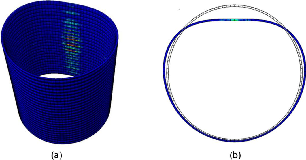
Figure 10-30. (a) Development of plastic strain in the inside polymeric liner for 0.75 in. thickness, and (b) Deformation pattern of the polymeric liner.
