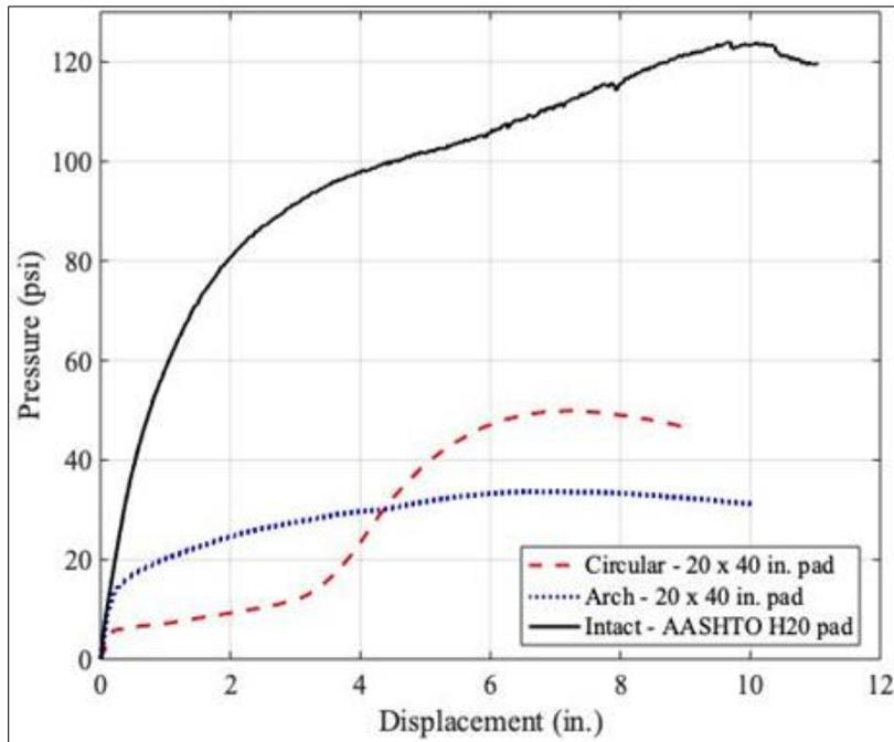
Figure 11-43. Control test: pressure on the soil surface under the load pad vs. soil settlement.
