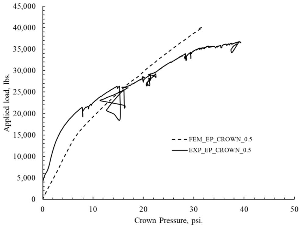
Figure 10E-4. Comparison of the earth pressure with the applied load for 0.5-in. thick arch polymeric liner.
