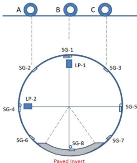
Figure 2-31. Culvert loading positions in the field (Masada et al. 2017).
