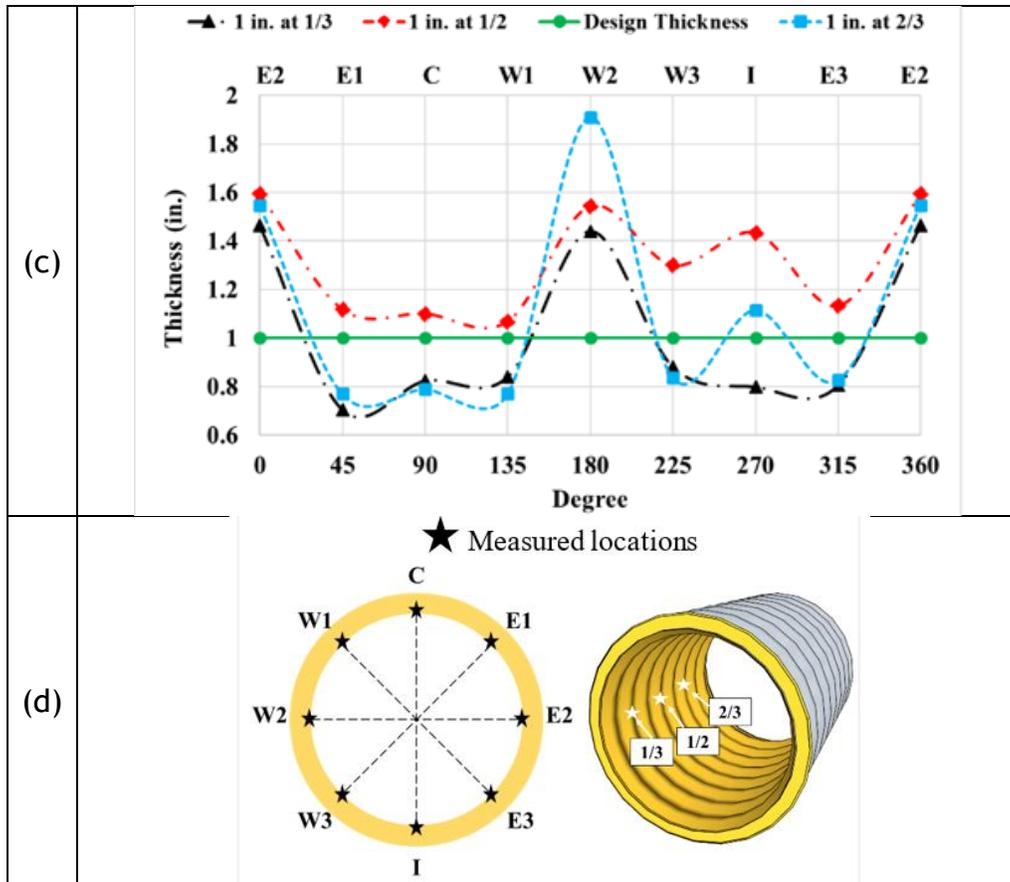
Figure 11-58. Thickness measurement results of polymeric SAPL renewed circular CMPs: (a) 0.25 in. thick SAPL, (b) 0.5 in. thick SAPL, (c) 1 in. thick SAPL, and (d) measured locations in circumferential and longitudinal direction.
