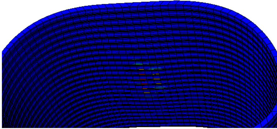
Figure 10-49. Development of the plastic strain in 1-in. thick arch polymeric SAPL along the crown.
