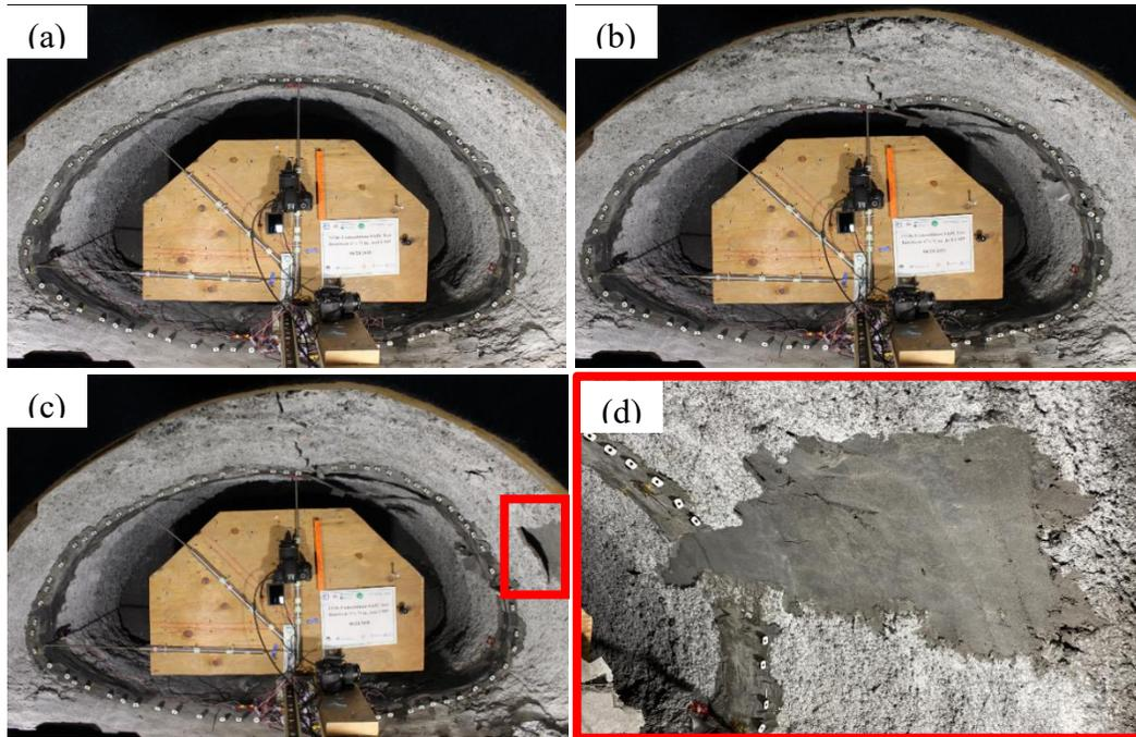
Figure 11-77. Invert-cut CMP arch renewed with 3 in. cementitious SAPL: (a) before loading, (b) after loading, (c) after unloading, and (d) delamination in the West springline.
