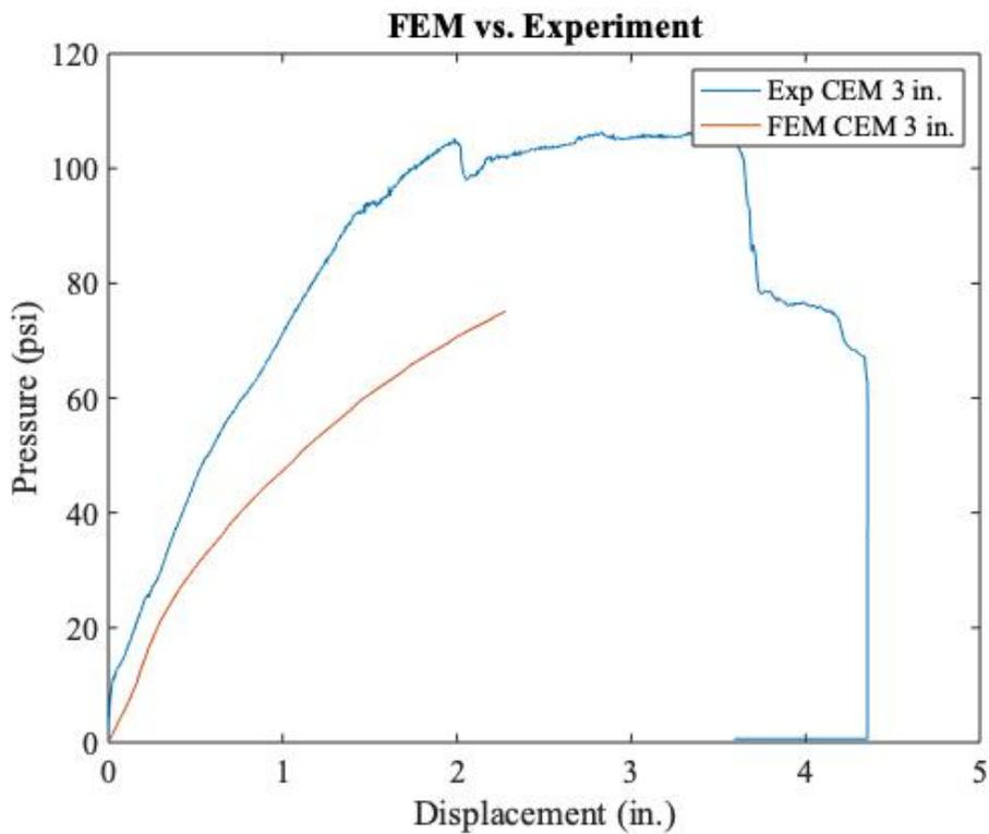
Figure 10F-8. Deformation of 3-in. thick cementitious liner under ultimate load.
