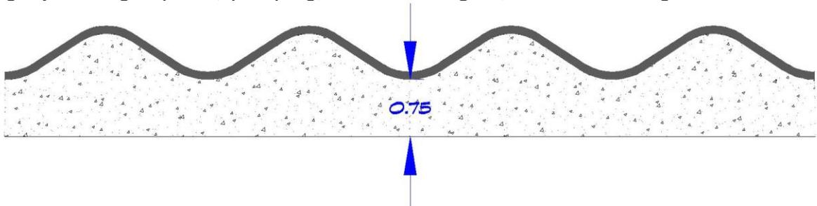
Figure 4-3 shows a  $\frac{3}{4}$  in. thick liner in this profile to graphically illustrate this to the reader.
