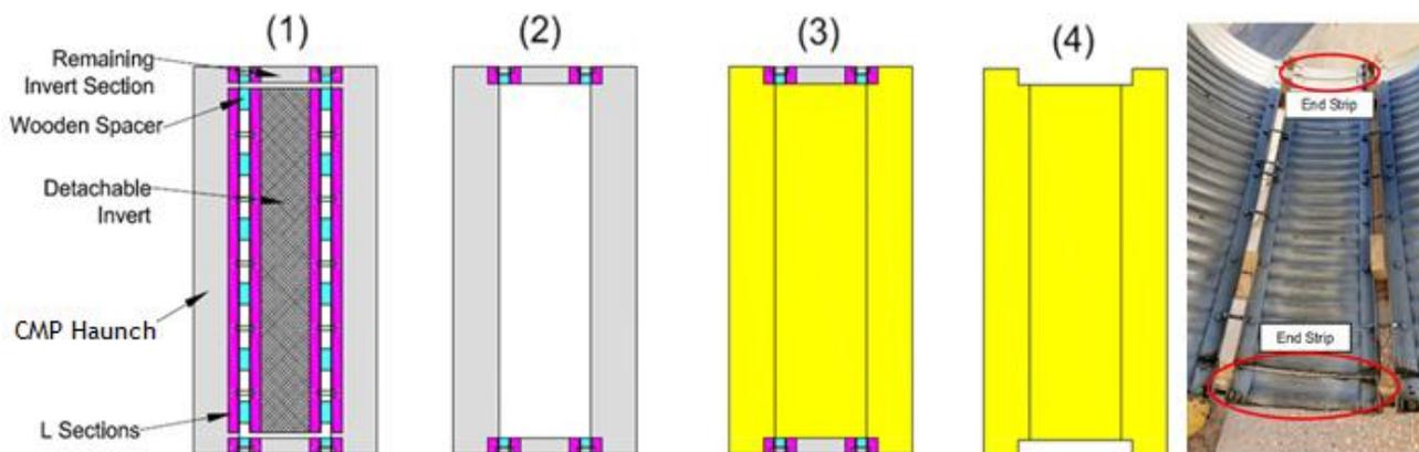
Figure 11-17. Detachable invert mechanism (in four stages) for SAPL renewed CMP samples before and during the SAPL installation.
