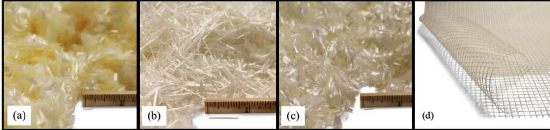
Figure 4. Micro-fibers used in concrete linings: (a) acrylic fiber, (b) alkali resistant (AR) glass fiber, (c) PVA fiber, and (d) alkali resistant glass scrim.
