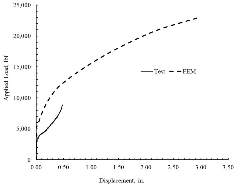
Figure 10A- 3. Movement of the spring line for FEM and TEST just before the meeting of the invert edges.
