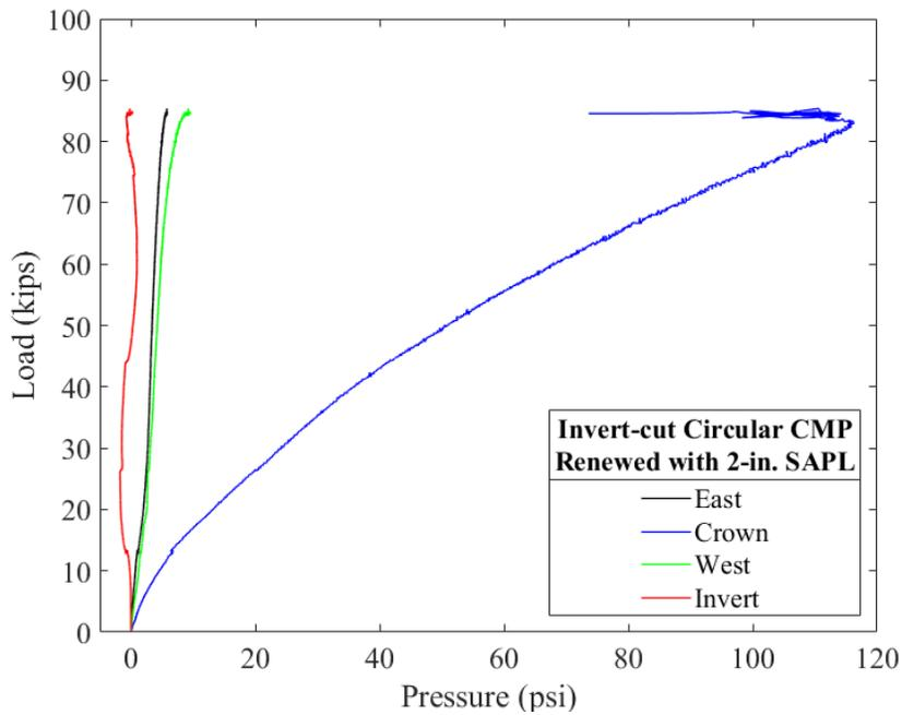
Figure 11-125. Load vs. pressure for the 2-in. thick SAPL renewed invert-cut circular CMP.
