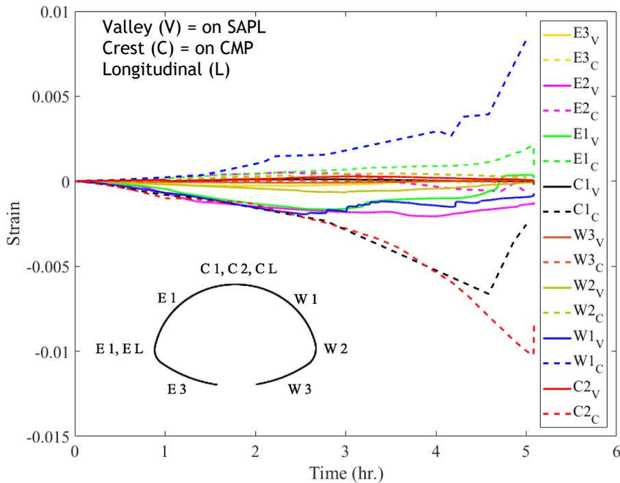
Figure 11-81. Strain gauges reading for the 3-in. thick SAPL renewed invert-cut CMP arch.
