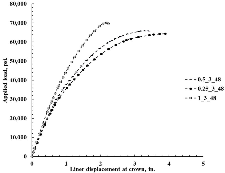
Figure 10E-13. Load displacement plot for 48 in. invert-cut circular CMPs with 3 ft cover and 0.25, 0.5, and 1 in. thick polymeric liner.
