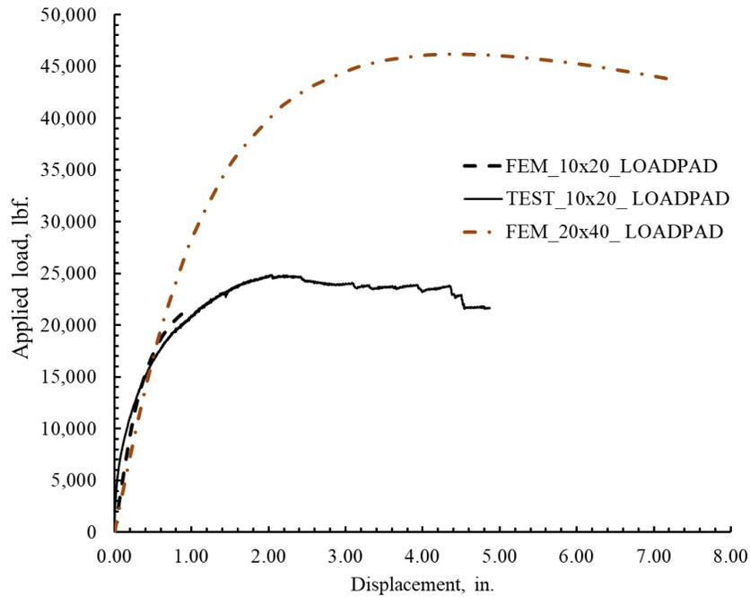
Figure 10-16. Effect of load pad size on the load-displacement at the crown.
