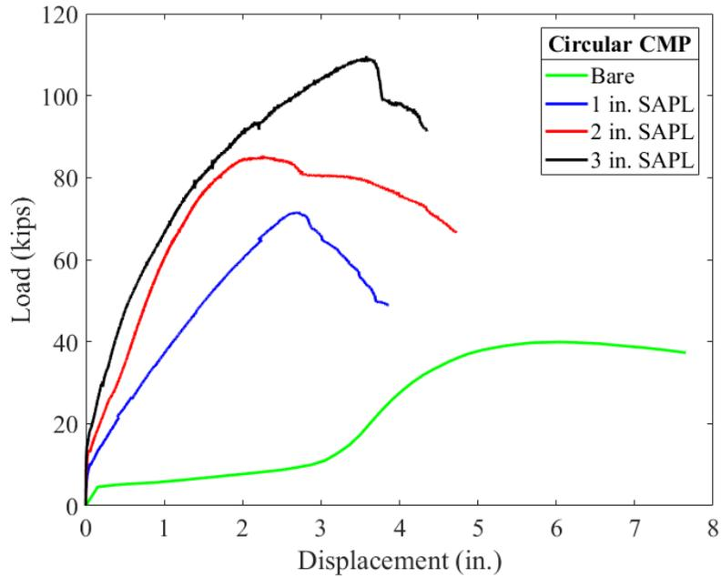
Figure 11-136. Load vs. crown displacement comparison graph.
