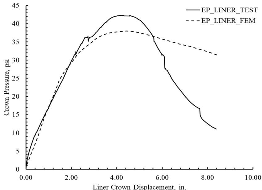
Figure 10-26. Comparison of the earth pressure at crown plotted against the liner displacement for 0.25 in thick polymeric SAPL
