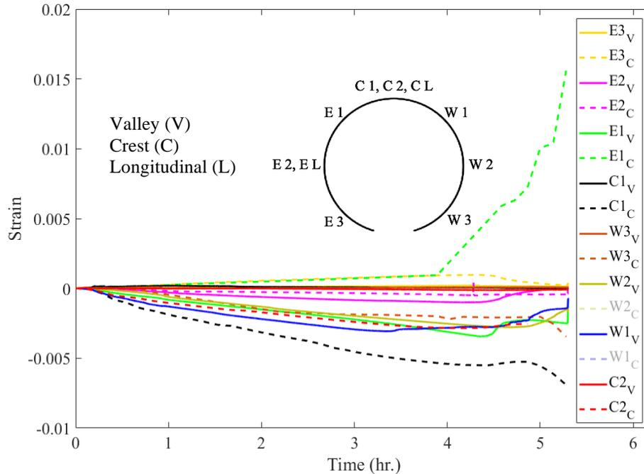
Figure 11-131. Strain gauges result for 1-in. thick SAPL renewed invert-cut circular CMP.
