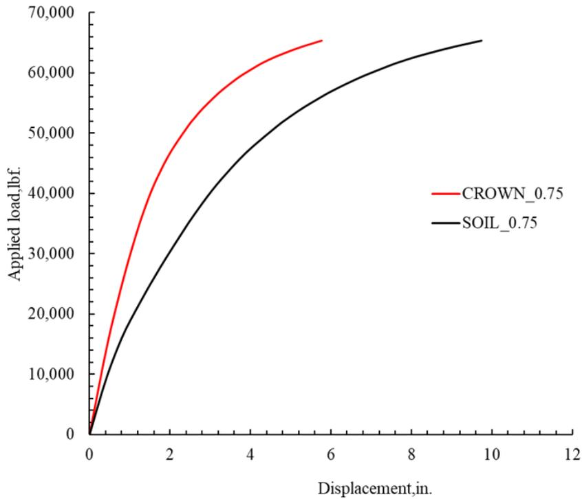
Figure 10B- 11. Load displacement plot from FE analysis for 0.75-in. thick polymeric circular liner.
