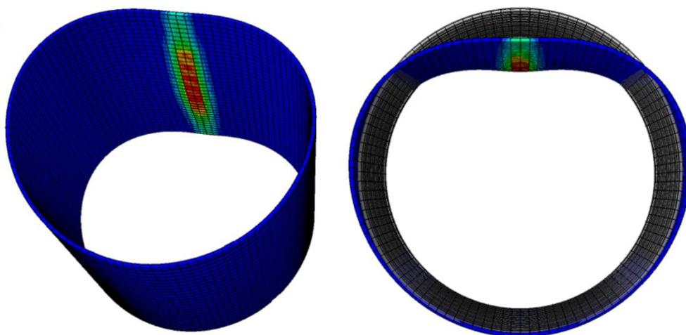
Figure 10-33. (a) Development of plastic strain (b) Deformation pattern for 0.25-in thick polymeric SAPL with filled corrugation.
