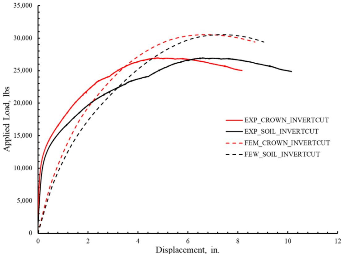
Figure 10C- 1. Load displacement plot for the movement of arch CMP's crown and settlement below load pad for invert cut arch CMP.
