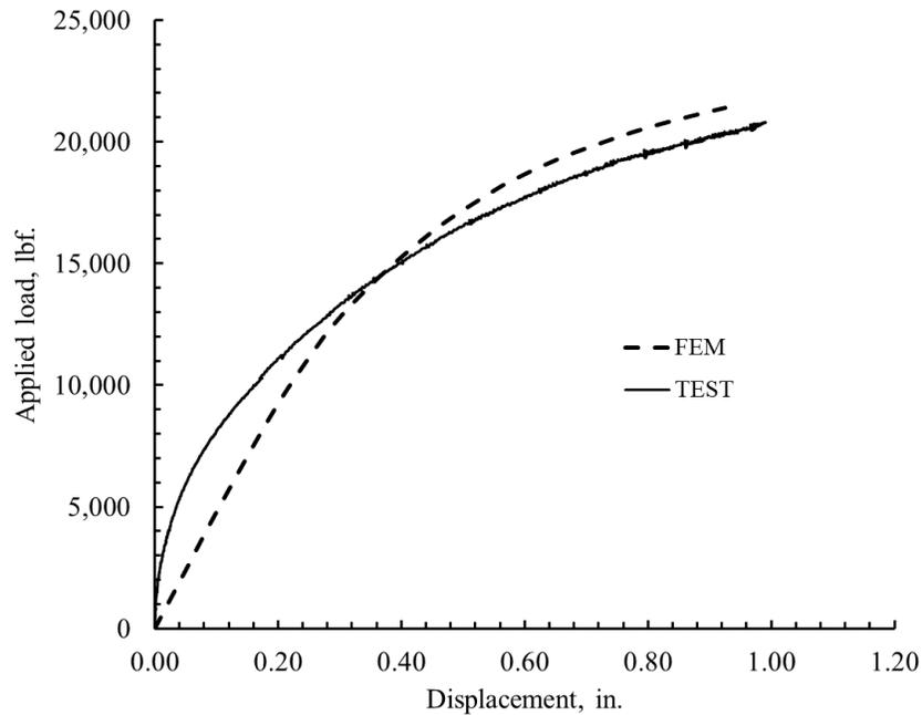
Figure 10-13. Load displacement curve for the crown at 5-in. displacement of the soil of intact CMP.
