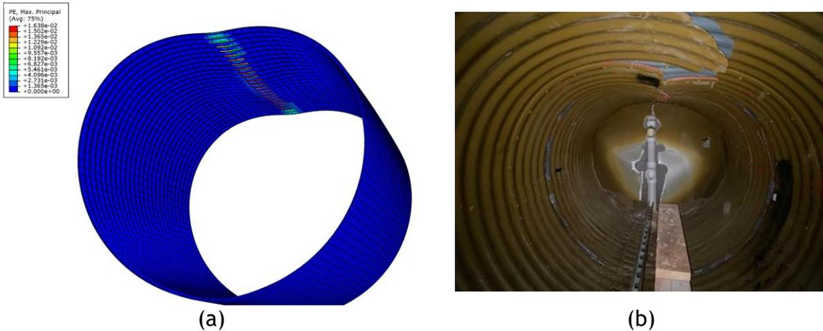
Figure 10-22. (a) Plastic strain at the ultimate load in the FE model (b) Crack in the model at the end of the test for 0.25 in. thick polymeric SAPL
