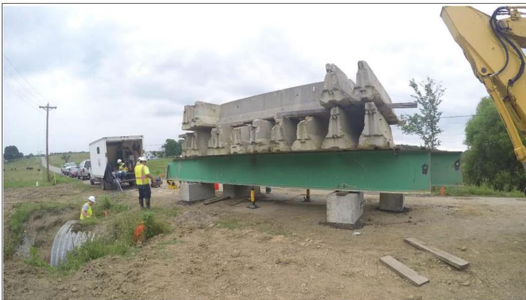
Figure 2-32. Field testing of a shallow cover severely deteriorated arch CMP (Sargand et al. 2018).
