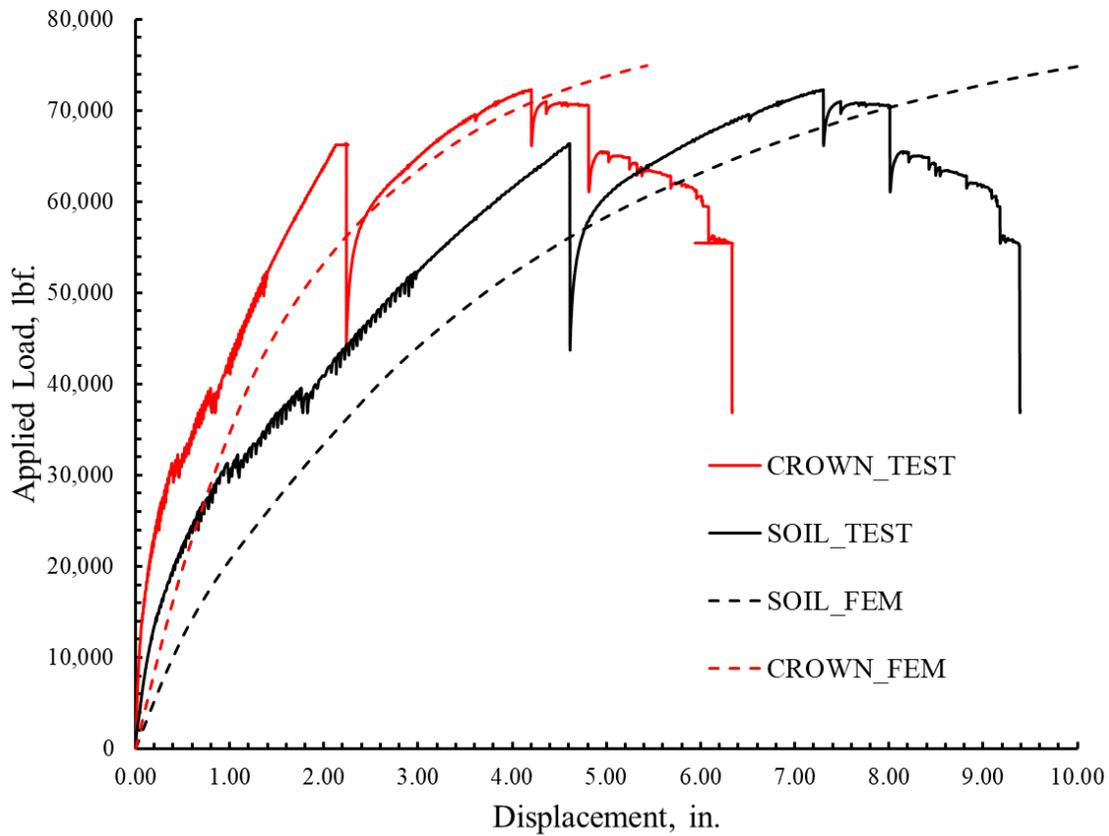
Figure 10B- 7. Load displacement comparison for FE and test results for 1-in. thick polymeric circular liner.
