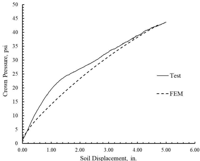
Figure 10-14 Earth pressure distribution just above the crown of the pipe of the intact pipe.
