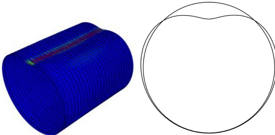
Figure 10-15. Plastic strain and the deformation of the pipe loaded under the 20x40 in.<sup>2</sup> load pad.
