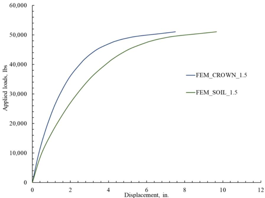
Figure 10E-11. Load displacement plot of crown displacement and soil settlement from FE analysis for 1.5-in. thick arch polymeric liner.
