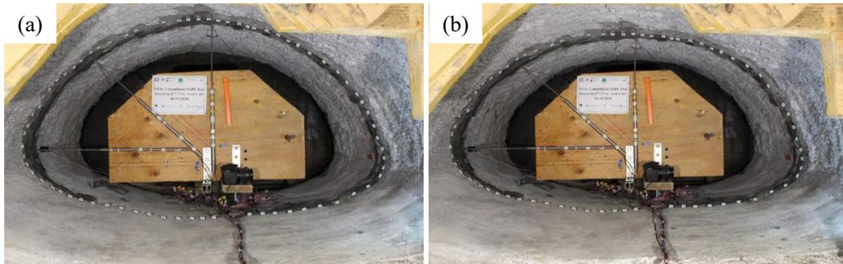
Figure 11-95. Invert-cut CMP arch renewed with 1 in. cementitious SAPL: (a) before loading, where the East haunch had a shrinkage crack and (b) after loading, where the shrinkage crack is closed.
