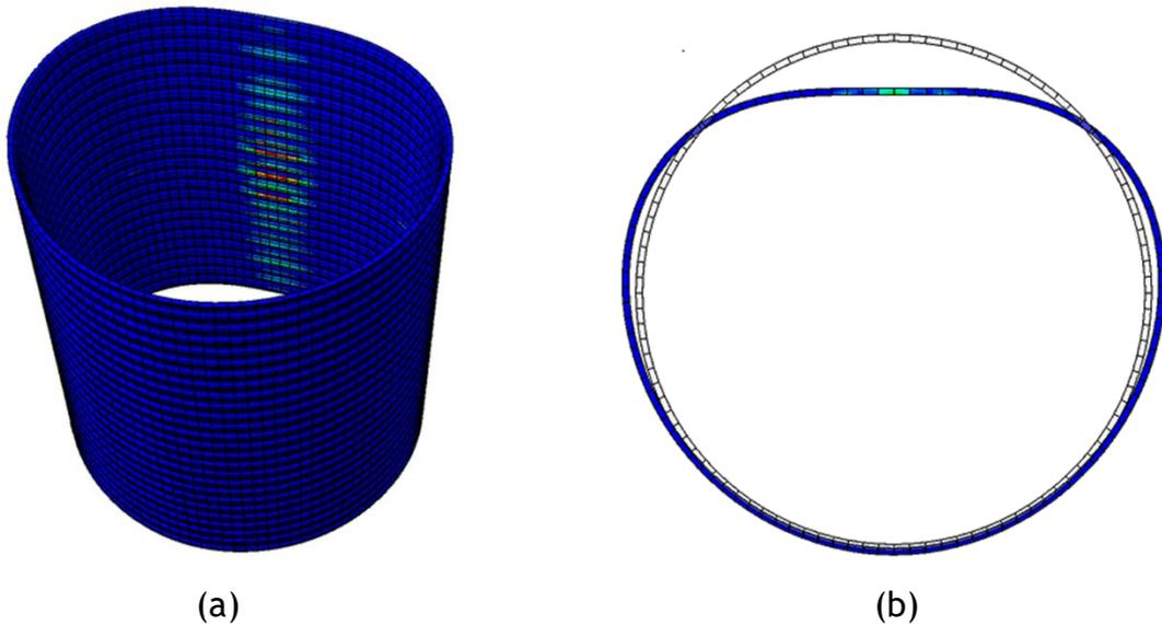
Figure 10B- 10. (a) Development of plastic strain in the inside liner for 0.75-in. thickness polymeric circular liner and (b) Deformation pattern of the polymeric circular liner.
