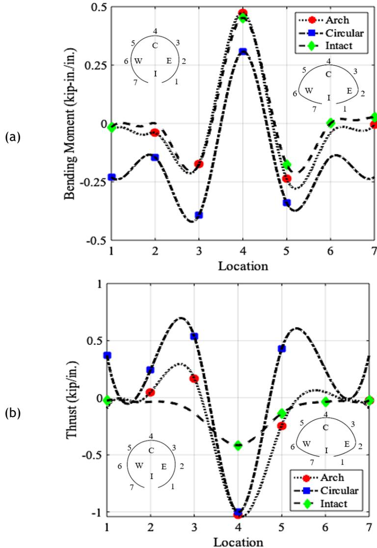
Figure 11-55. Internal forces on intact, invert-cut circular and invert-cut CMP arch samples: (a) bending moment, and (b) thrust forces for the invert-cut arch, invert-cut circular and circular intact CMPs.
