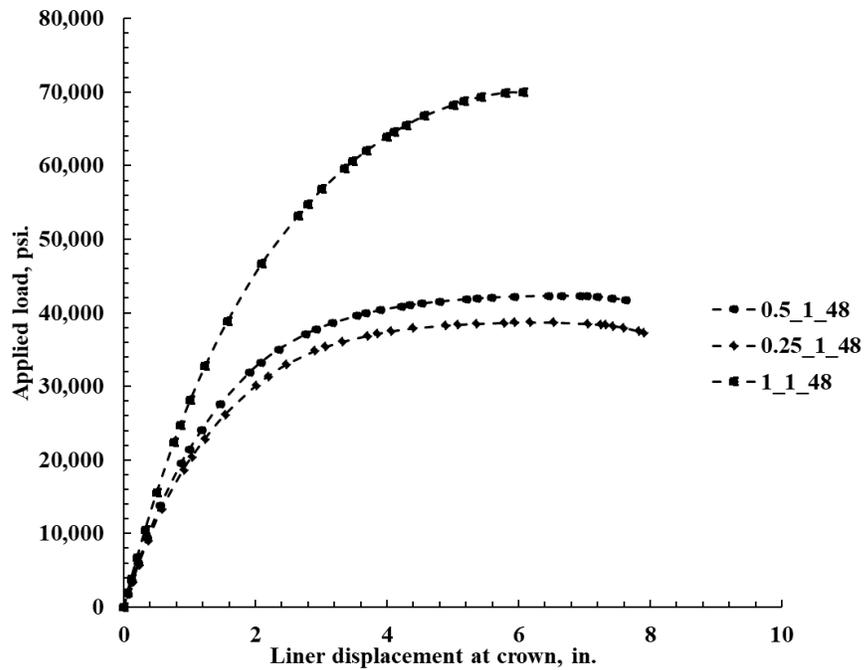
Figure 10E-17. Load displacement plot for Invert-cut circular 48 in. CMPs with 1 ft cover and 0.25, 0.5, and 1 in. thick polymeric liner.
