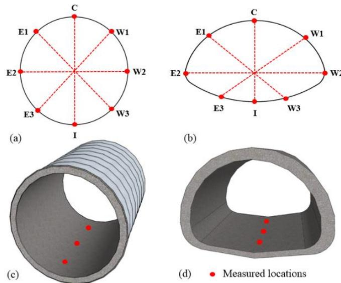
Figure 11-39. SAPL thickness measurement: (a) measurements in circumferential direction on circular and, (b) pipe arch SAPL samples, (c) measurements in longitudinal direction on circular and, (d) pipe arch SAPL samples.
