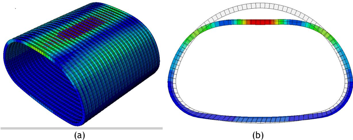
Figure 10-56. (a) Development of mises stress, and (b) Deformation pattern for 2- in. thick arch polymeric SAPL.
