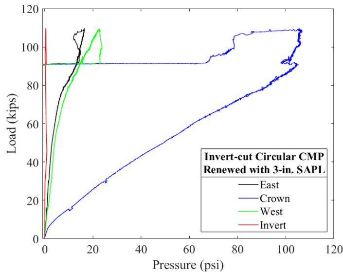
Figure 11-116. Load vs. pressure for the 3-in. thick SAPL renewed invert-cut circular CMP.
