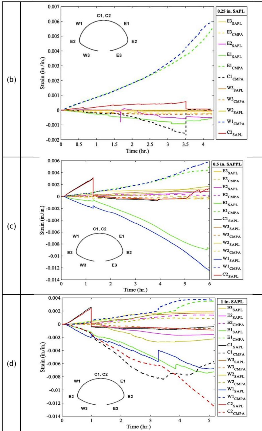
Figure 11-73. Strain gauge results: (a) invert-cut bare CMP arch, (b) 0.25 in. SAPL renewed CMP arch, (c) 0.5 in. SAPL renewed CMP arch, and (d) 1 in. SAPL renewed CMP arch.
