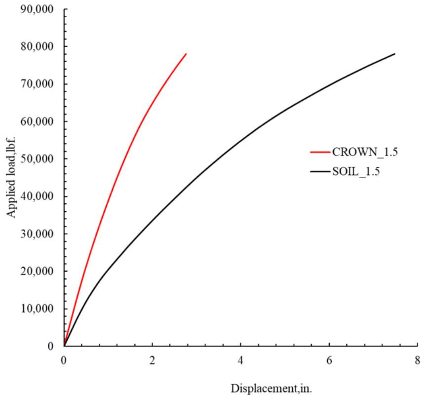
Figure 10B- 12. Load displacement curve for 1.5-in. thick polymeric circular liner.
