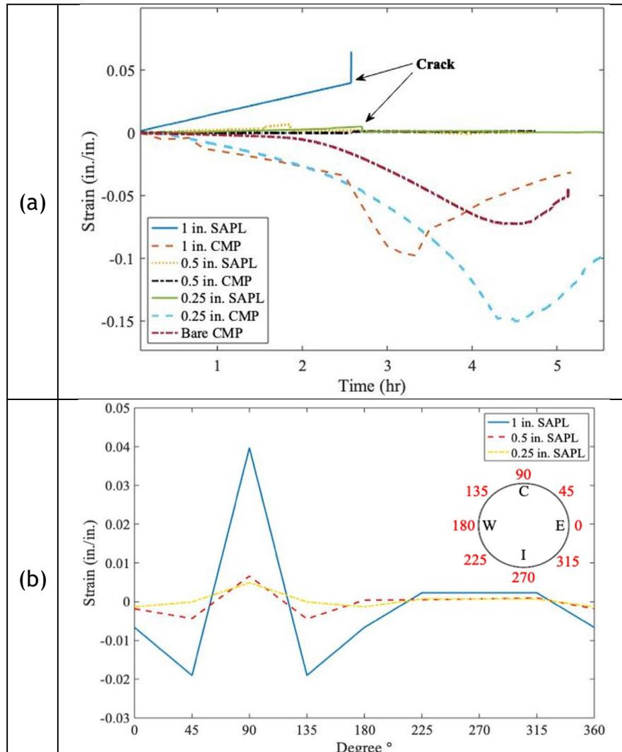
Figure 11-63. Strain gauge results for SAPL renewed circular CMP: (a) at the crown and (b) around the SAPL at the time of first structural crack.
