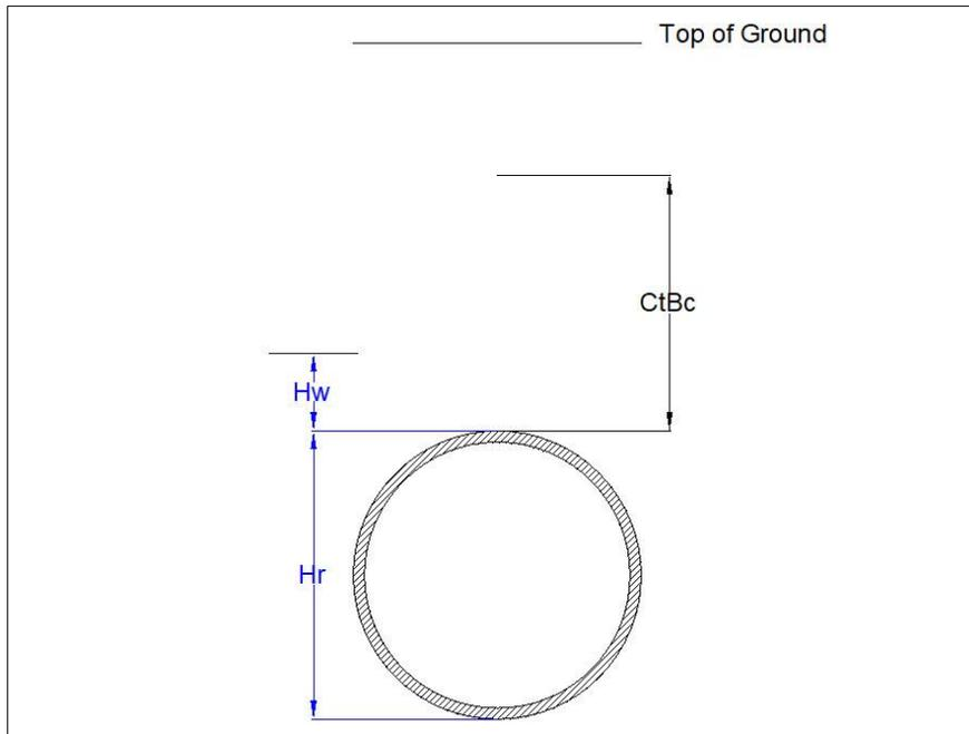
Figure 8-2 Dead loads acting on pipe.
