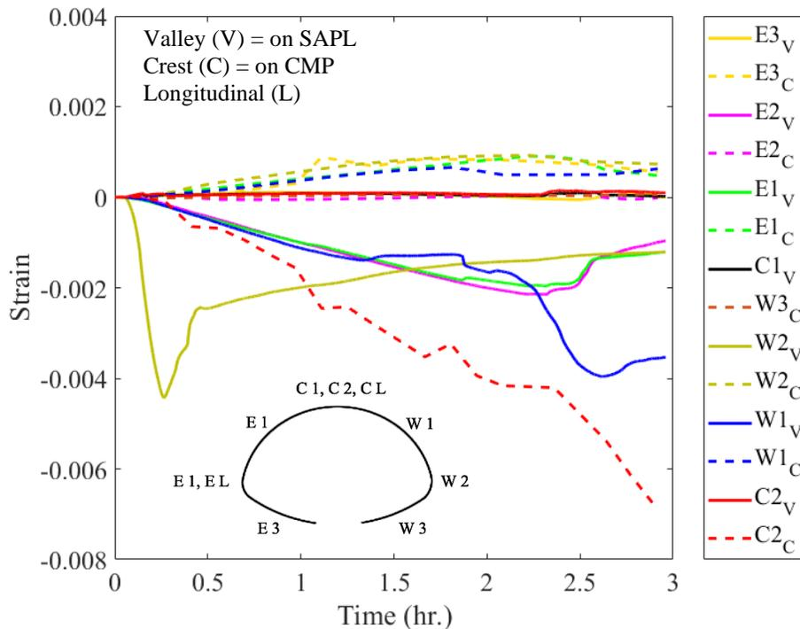
Figure 11-99. Strain gauges reading for 1-in. thick SAPL renewed invert-cut CMP arch.
