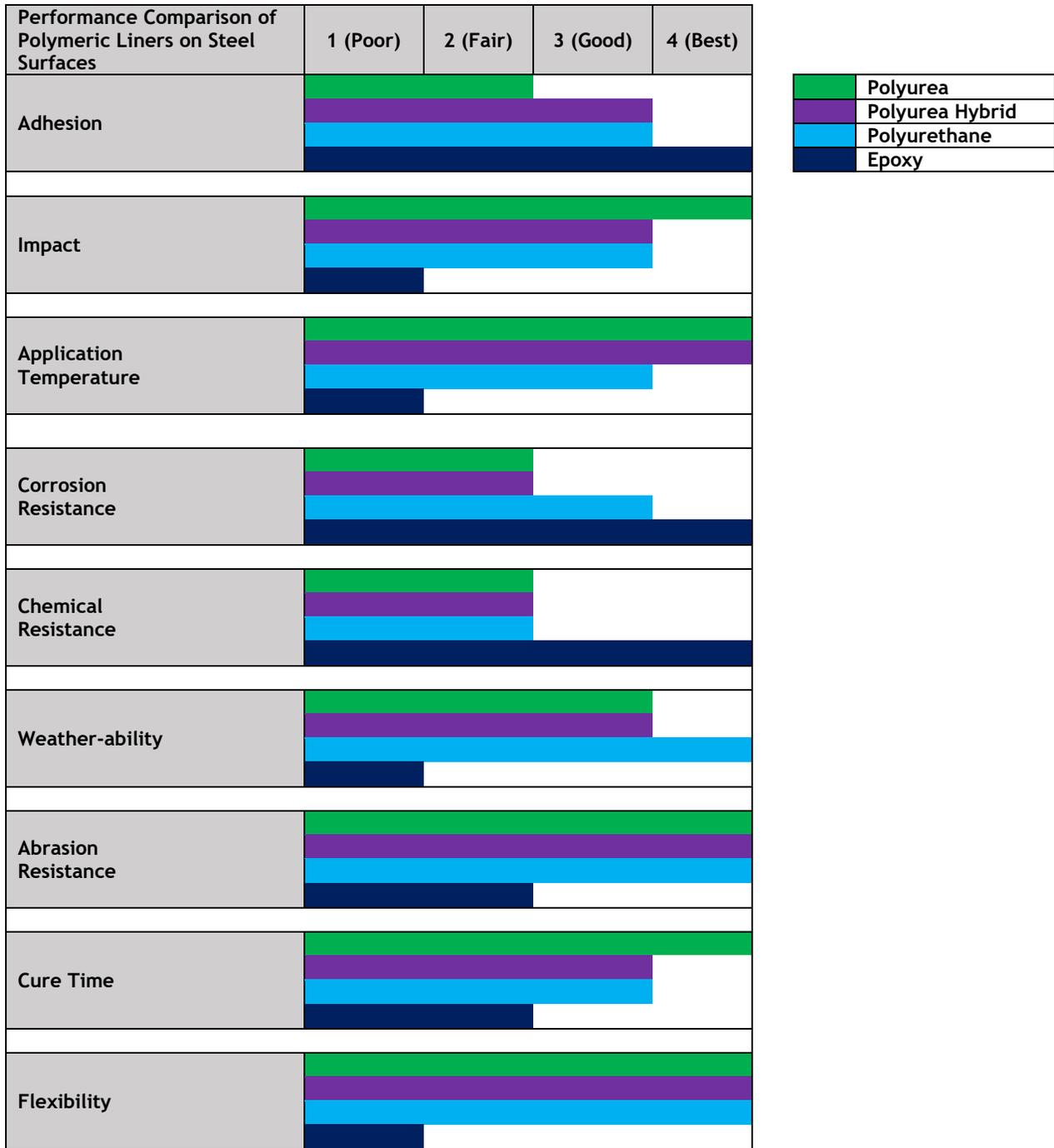
Figure 2-22. Performance comparison of polyurea, polyurea hybrid, polyurethane and epoxy coatings applied on steel substrate (Adapted from Cain 2016).
