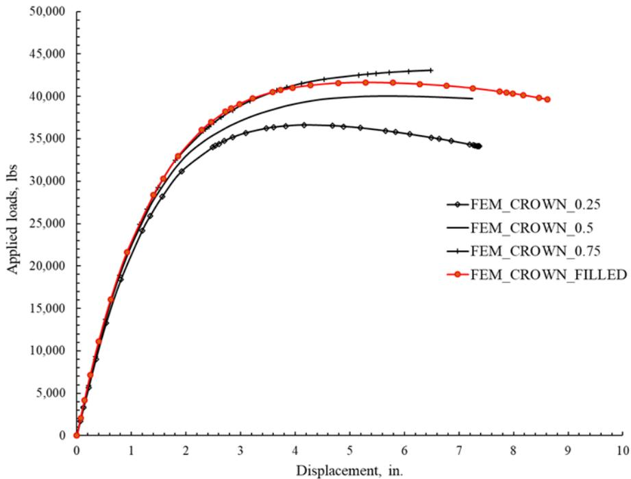
Figure 10-58. Comparison of the performance of 0.25-in. thick filled corrugated polymeric SAPL for arch with liner thickness following the corrugation.
