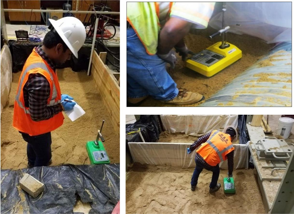
Figure 11-11. Nuclear density measurement.
