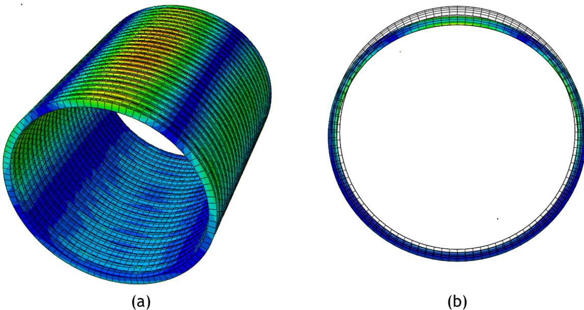
Figure 10-32. (a) Development of plastic strain and (b) Deformation pattern for 2- in. thick polymeric SAPL.
