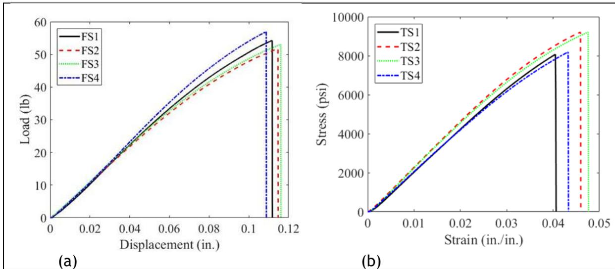
Figure 11-57. Polymeric SAPL material property test results: (a) flexural test (ASTM D790), and (b) tensile test (ASTM D638).
