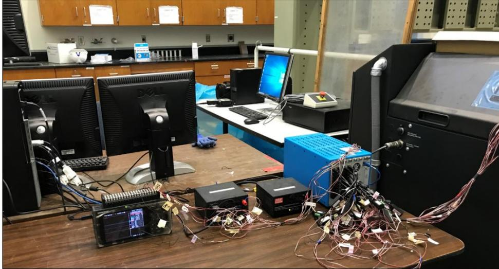
Figure 11-21. Strain gauges connected to a data acquisition system (DAQ).
