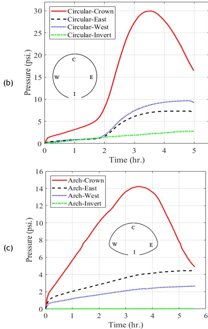
Figure 11-53. Results of earth pressure cells for the CMP control test: (a) intact circular CMP, (b) invert-cut circular CMP, and (c) invert-cut CMP arch.
