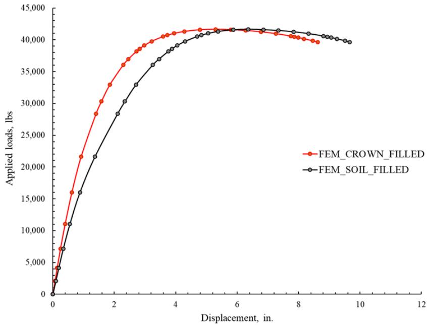
Figure 10-57. Load displacement curve for 0.25-in. thick polymeric SAPL (filled corrugations).
