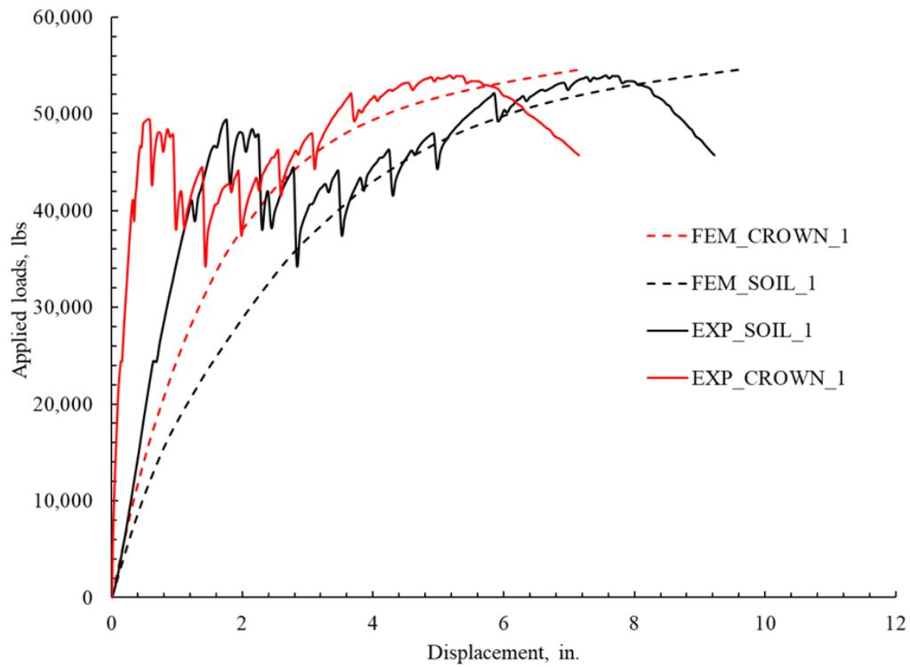
Figure 10E-7. Load displacement plot at the crown and settlement of soil below load pad for 1-in. thick arch polymeric liner.
