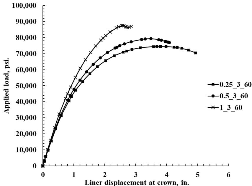
Figure 10D-1. Load displacement plot for 60-in. invert-cut circular CMP with 3 ft cover and 0.25-, 0.5-, and 1-in. thick polymeric circular liner.
