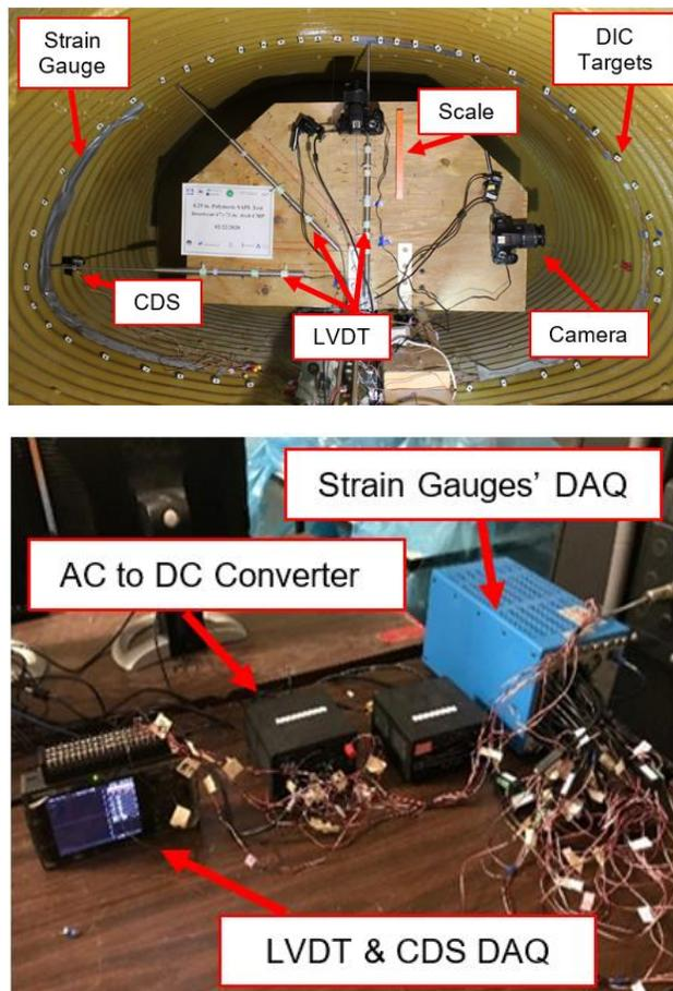
Figure 11-27. Instrumentation: (top) LVDTs, CDSs, DIC targets and cameras inside the pipe sample, (bottom) data acquisition systems.
