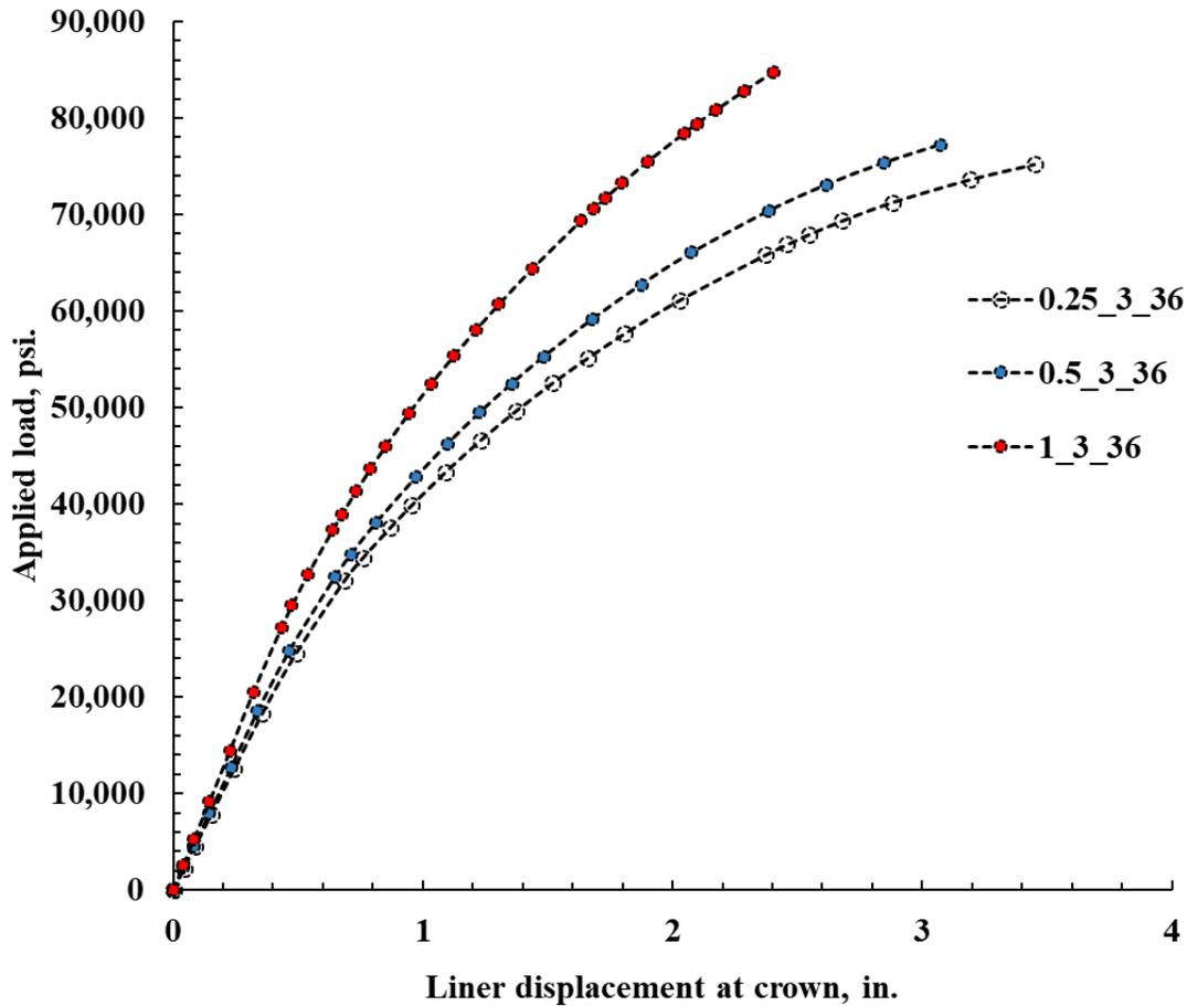
Figure 10E-19. Load displacement plot for invert-cut circular 36 in. CMPs with 3 ft cover and 0.25, 0.5, and 1 in. thick polymeric liner.
