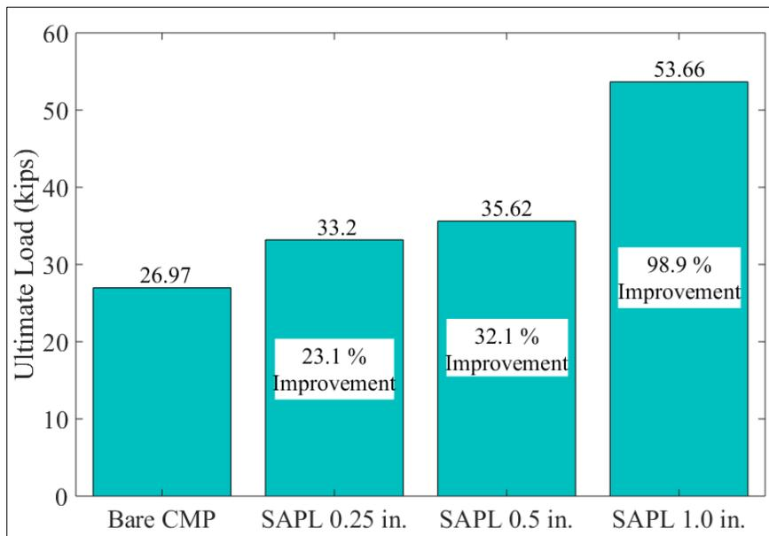
Figure 11-70. Fully Invert deteriorated CMP arch samples ultimate load carrying capacity improvement through SAPL application.
