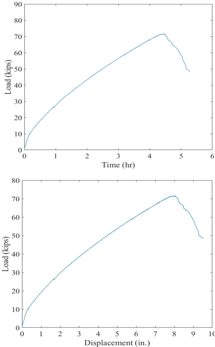
Figure 11-128. Invert-cut circular CMP renewed with 1-in. thick cementitious SAPL subjected to static live load: (top) load-time, and (bottom) load-soil displacement graphs.
