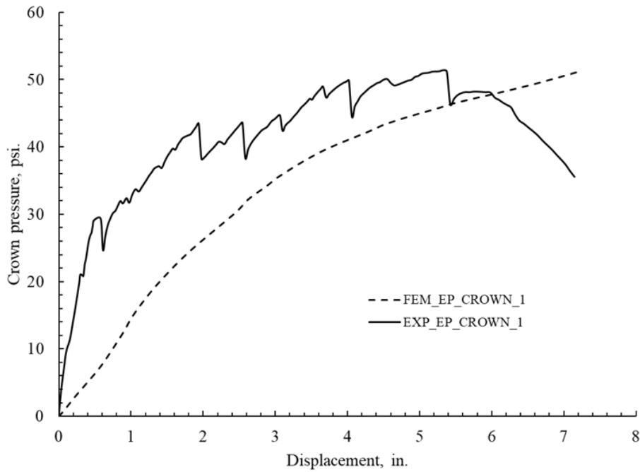
Figure 10E-8. Comparison of the Earth pressure with polymeric liner's crown disp., for 1-in. thick arch polymeric liner.
