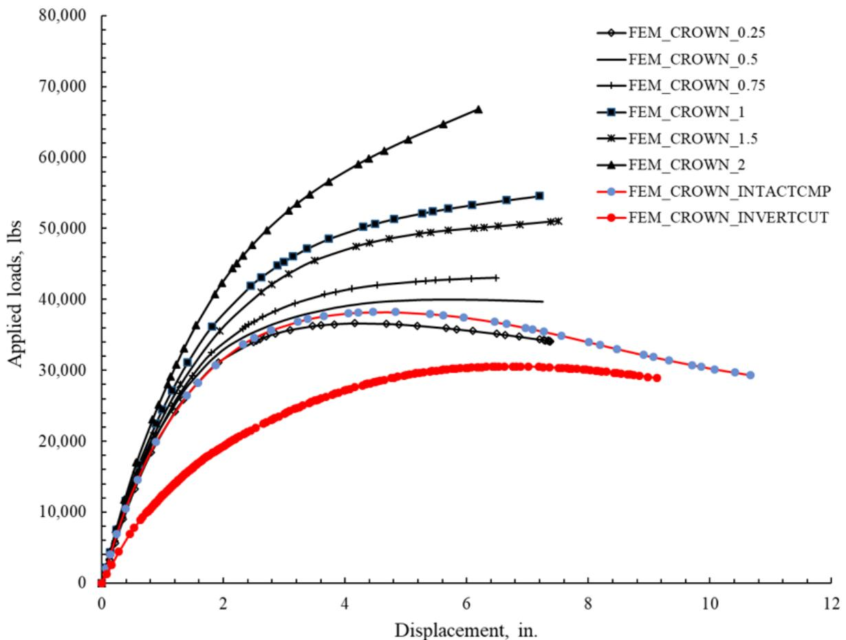
Figure 10-59. Comparison of the load-displacement plot at the crown obtained from all the FE results for arch CMP lined with polymeric SAPL.
