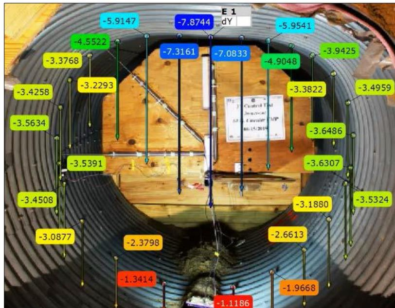
Figure 11-48. Results of DIC measurement at the end of the test (60-in. invert-cut circular CMP).
