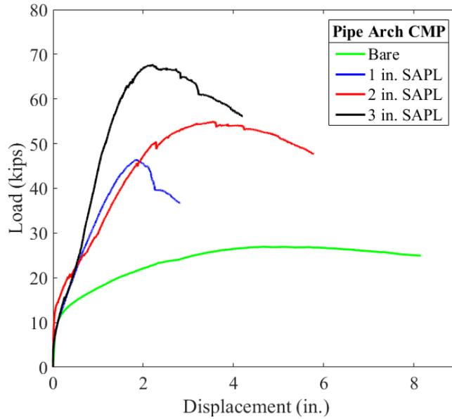
Figure 11-105. Load vs. crown displacement comparison graph.
