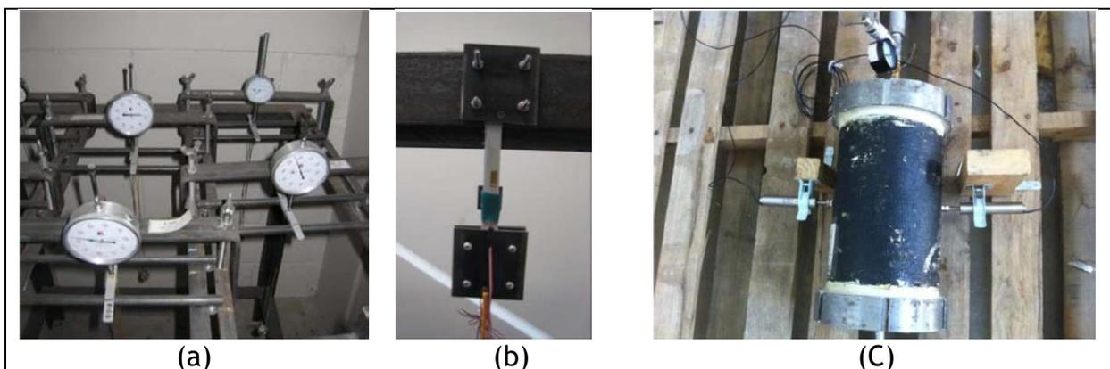
Figure 2-24. Comparison of spray-on lining methods using material property testing: (a) long-term flexural testing, (b) long-term creep tensile testing and (c) hydrostatic test setup (Motlagh et al. 2013).
