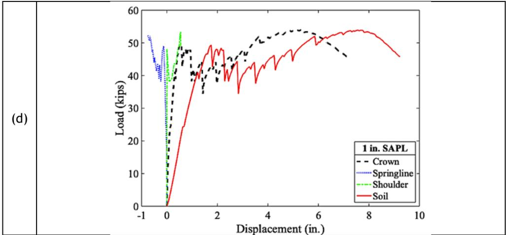
Figure 11-68. Bare and SAL renewed CMP arch samples Load-Displacement graphs: (a) invert-cut bare CMP arch, (b) 0.25 in. SAPL renewed CMP arch, (c) 0.5 in. SAPL renewed CMP arch, and (d) 1 in. SAPL renewed CMP arch.
