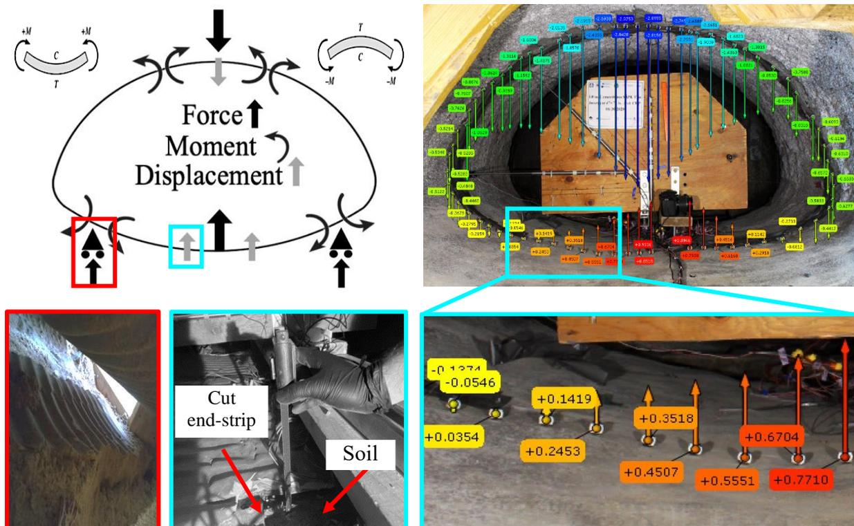
Figure 11-76. CMP arch behavior due to the vertical load, where the red boxes show the soil support under the pipe on the west haunch area and the blue boxes illustrates the pipe upward movement.
