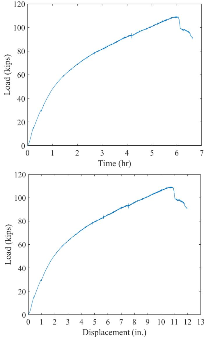
Figure 11-110. Invert-cut circular CMP renewed with 3-in. thick cementitious SAPL subjected to static live load: (top) load-time, and (bottom) load-soil displacement graphs.
