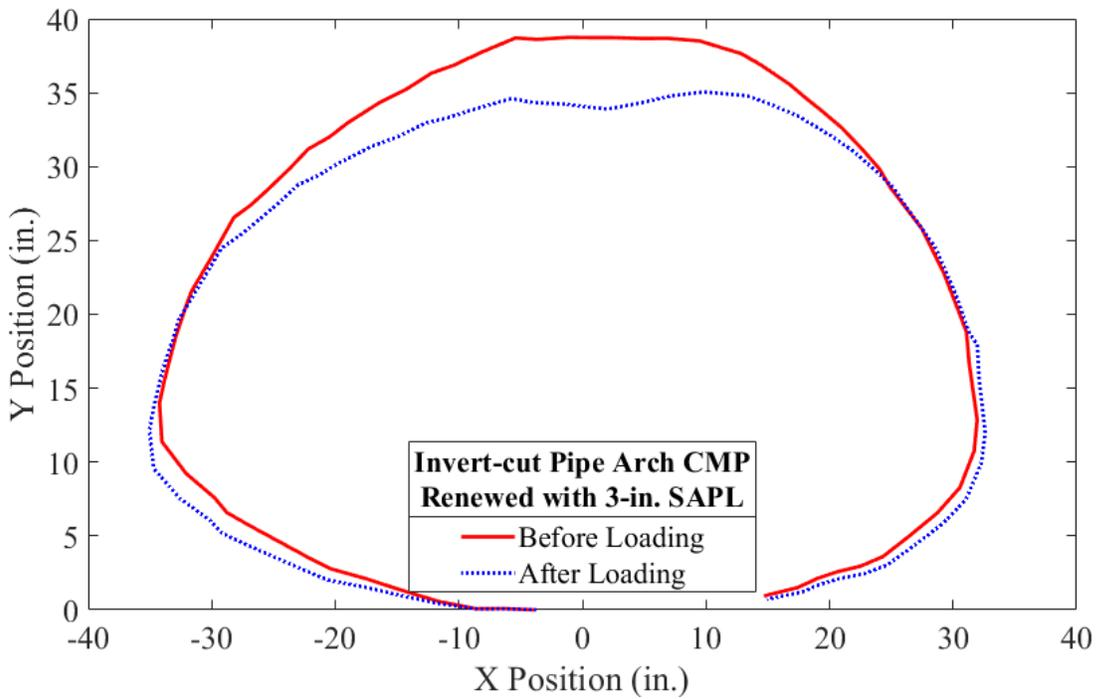
Figure 11-82. Pipe profiling using DIC for the 3-in. thick SAPL renewed invert-cut CMP arch.
