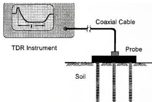
Figure 11-14. Measurement of soil moisture content using TDR method (Siddiqui & Drnevich, 1995).
