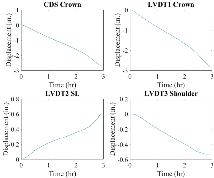
Figure 11-98. Mechanical sensors result for 1-in. thick SAPL renewed invert-cut CMP arch.
