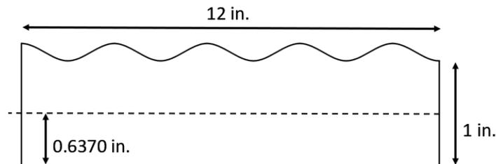
Figure 8-4 Cross-section on 1.0-inch-thick liner in soil box testing.
