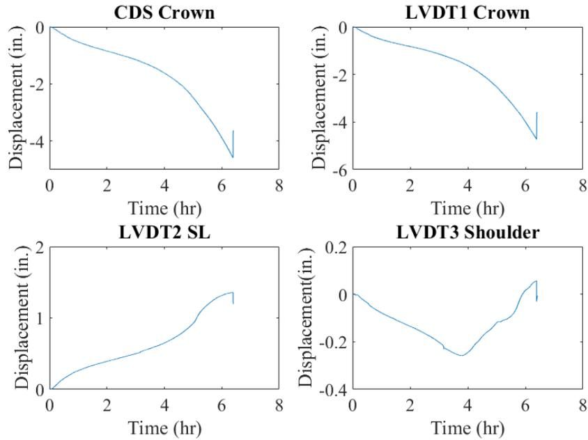
Figure 11-121. Mechanical sensors result for 2-in. thick SAPL renewed invert-cut circular CMP.
