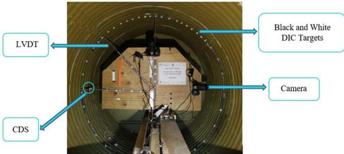
Figure 11-26. Instrumentation: LVDTs, CDSs, DIC targets and cameras inside the pipe sample.
