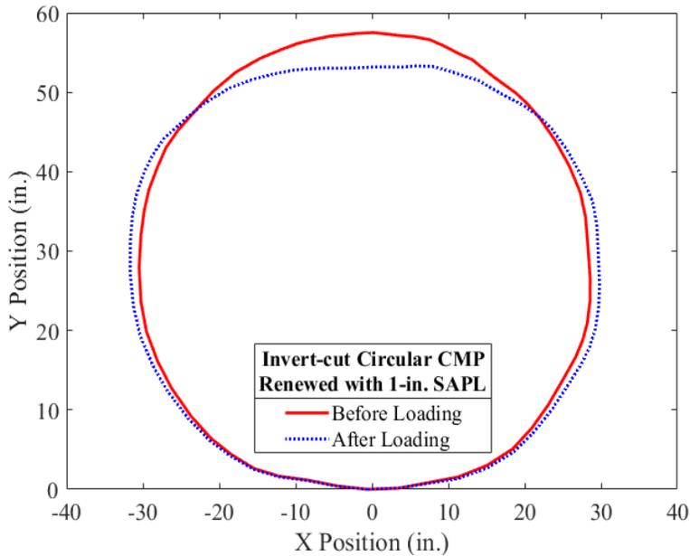
Figure 11-132. Pipe profiling using DIC for the 1-in. thick SAPL renewed invert-cut circular CMP.
