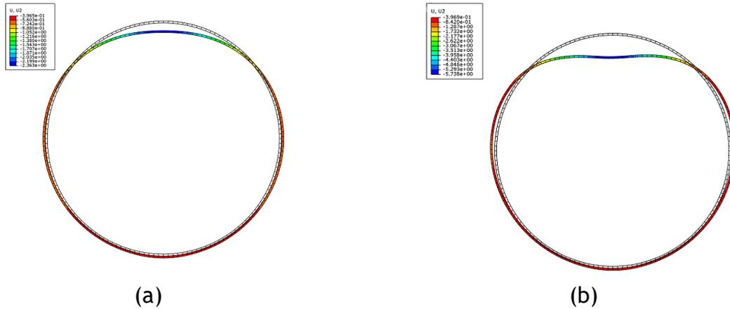
Figure 10B- 1. (a) Deformation of the liner at the appearance of the first plastic strain, and (b) Deformation of the liner at the ultimate load for 0.5 in. thick polymeric circular SAPL.
