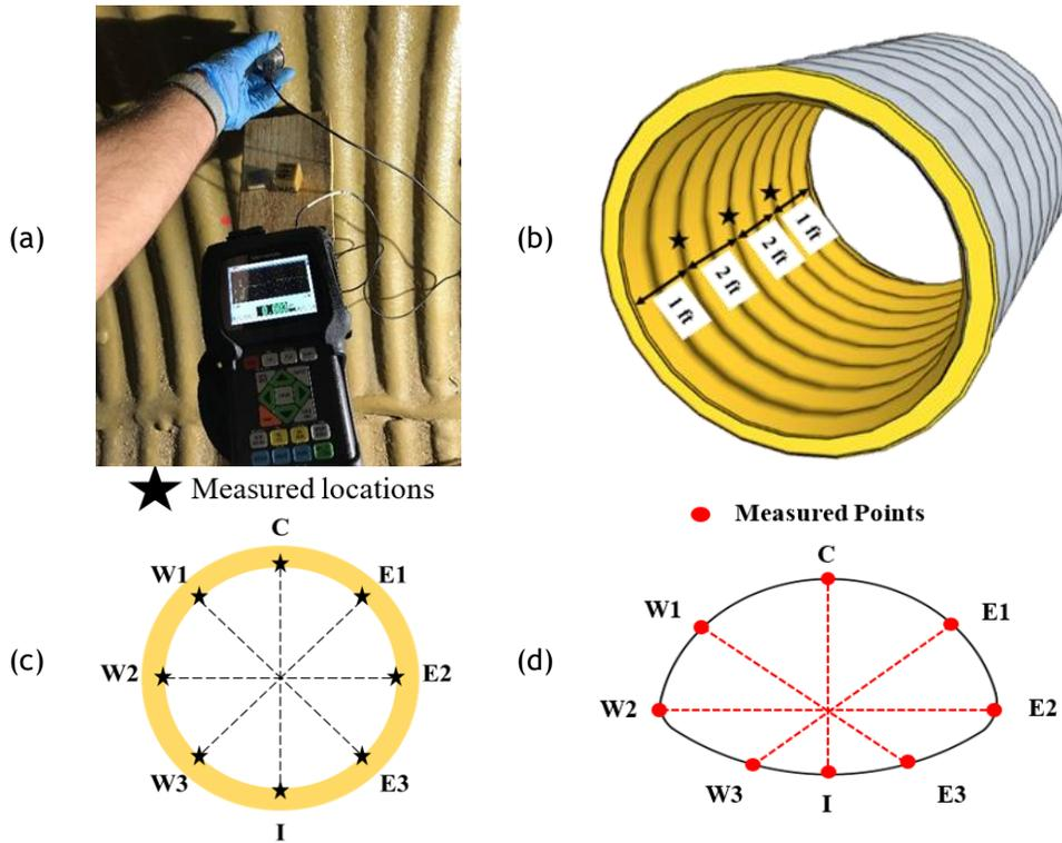
Figure 11-28. SAPL thickness measurement: (a) thickness gauge and calibration sample, (b) longitudinal measured locations, (c) circular CMP circumferential measured locations, and (d) CMP arch circumferential measured locations.
