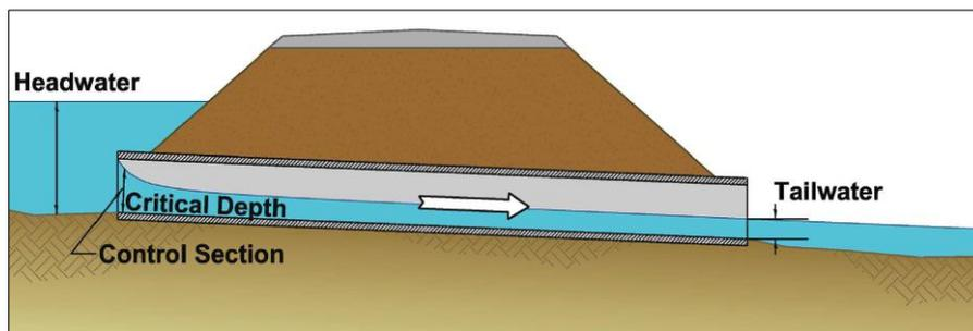
Figure 2-5. Typical “inlet control” flow section for a partly full culvert (FHWA 2012).
