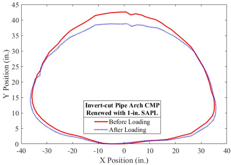
Figure 11-100. Pipe profiling using DIC for the 1-in. thick SAPL renewed invert-cut CMP arch.
