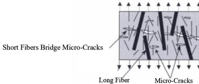
Figure 3-1. Bridging behavior of fiber reinforcements to limit the cracks, (Source: <https://theconstructor.org/concrete/hybrid-fiber-reinforced-concrete/17204/>).
