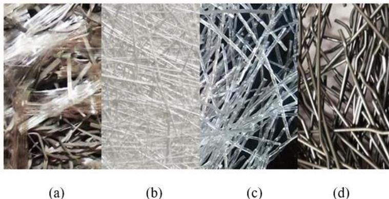
Figure 3-3. Macro fibers used in concrete lining; (a) polypropylene fibers, (b) fiberglass, (c) polyolefin fibers and (d) steel fibers.
