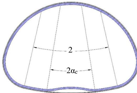
Figure 8-6 Pipe arch shape showing bottom arc angle.
