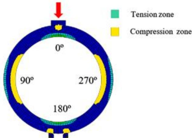
Figure 3-2. FEM analysis of an RCP under TBT setup: inner sides of crown (0°) and invert (180°) are in tension and need to be reinforced (Darabnough Tehrani 2016).
