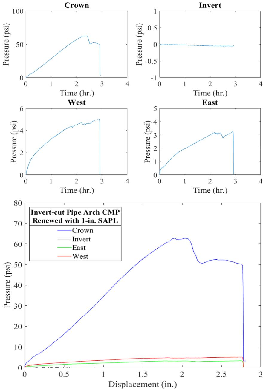
Figure 11-97. Earth pressure cell results for the 1-in. thick SAPL renewed invert-cut CMP arch with respect to: (top) time, and (bottom) crown displacement.
