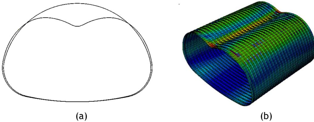
Figure 10-39. (a) Vertical diameter change from FEM after complete loading, and (b) ultimate Mises stress in around the arch CMP.
