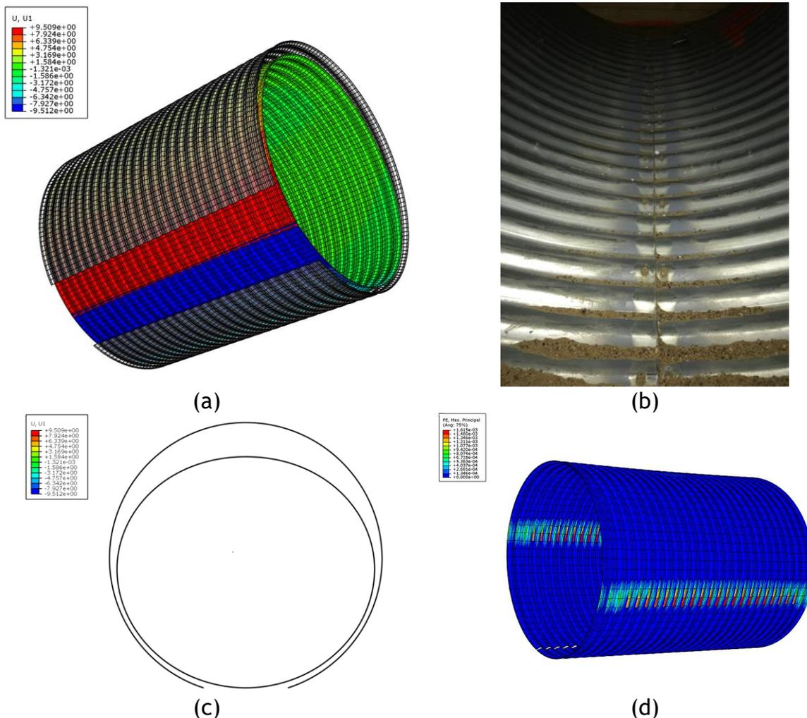
Figure 10-20. FEM exhibited a stiffer response and significantly over predict the load-bearing capacity. The load-displacement comparison for the invert-cut CMPs can be found in Appendix 10-A.
