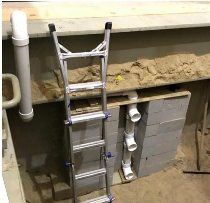
Figure 11-5. Soil box ventilation
