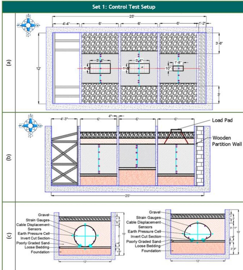
Figure 9. The CMPs' burial configuration (control test set): (a) plan view, (b) profile view of the aligned CMPs in the soil box, and (c) cross sectional view of both circular and CMP arch samples.
