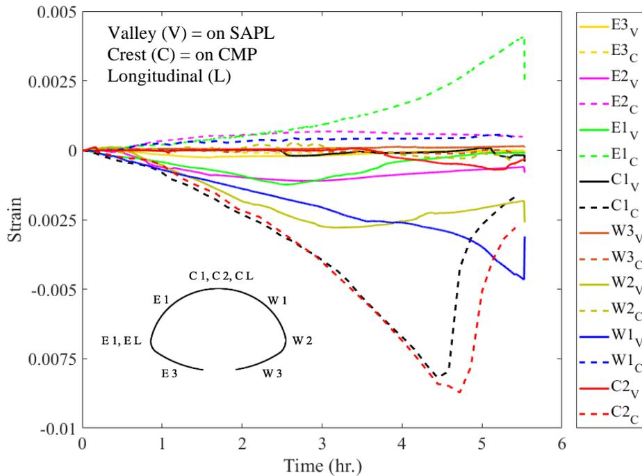
Figure 11-90. Strain gauges reading for 2-in. thick SAPL renewed invert-cut CMP arch.
