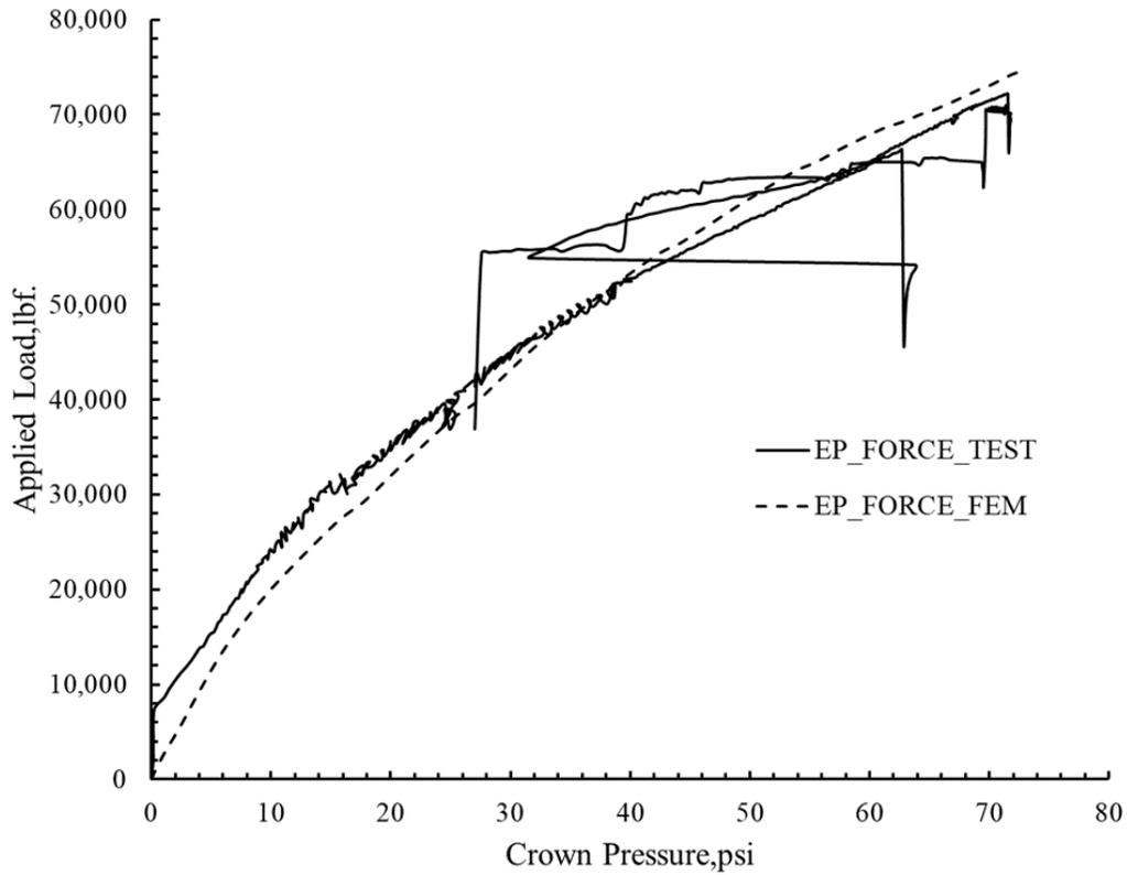
Figure 10B- 9. Comparison of the Earth pressure with applied load, for 1-in. thick polymeric circular liner.
