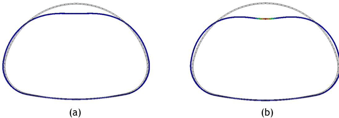
Figure 10E- 1. Deformation pattern at the first crack (a) and at ultimate crack, and (b) 0.5 in. thick arch polymeric liner.
