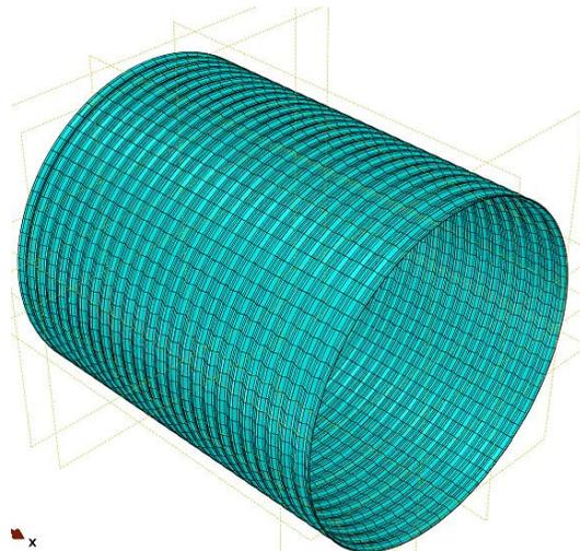
Figure 10-3. CMP model in FE.
