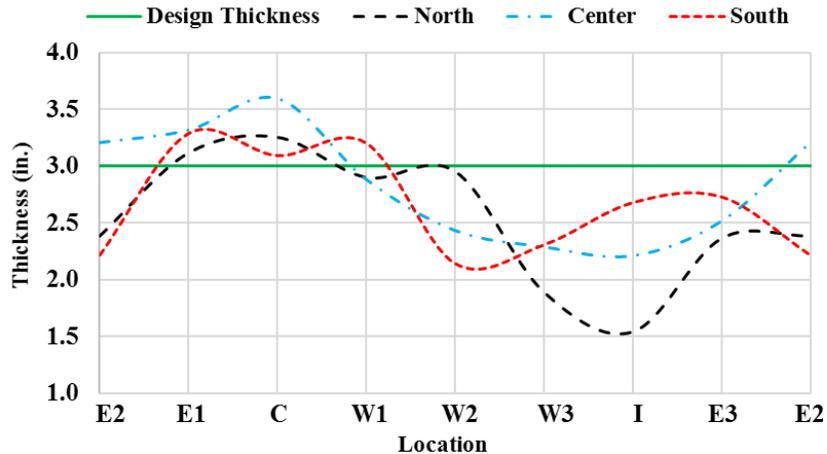
Figure 11-117. Thickness measurement for the 3-in. thick cementitious SAPL renewed circular CMP.
