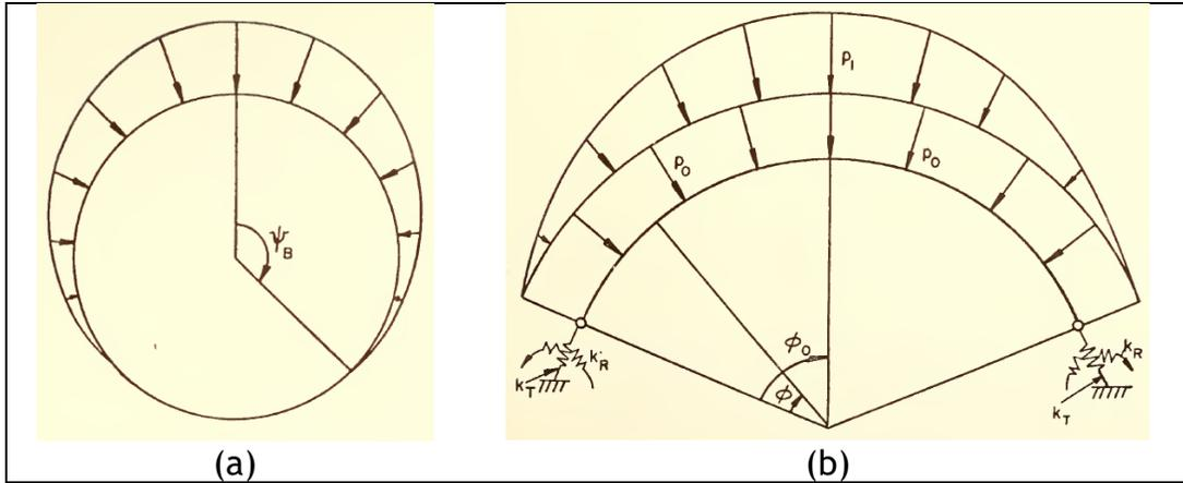
Figure 2-9. Active pressure distribution around circular conduit (Klöppel and Glock 1970; Leonards and Stetkar 1978).
