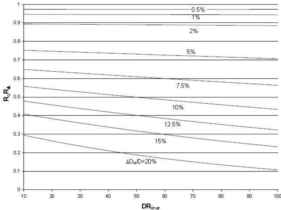
Figure 6-4. Buckling strength reduction for fractured sewer with close fitting liner (Source: Moore, 2008).
