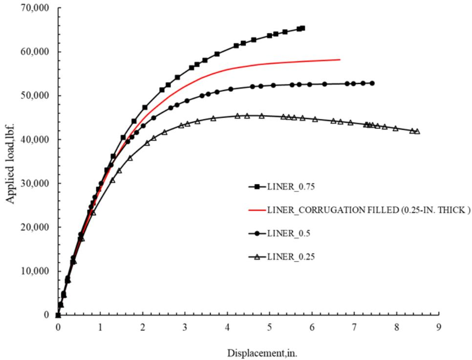
Figure 10-35. Load displacement plot from FE analysis for 0.25-in. thick (over the crest) polymeric SAPL.
