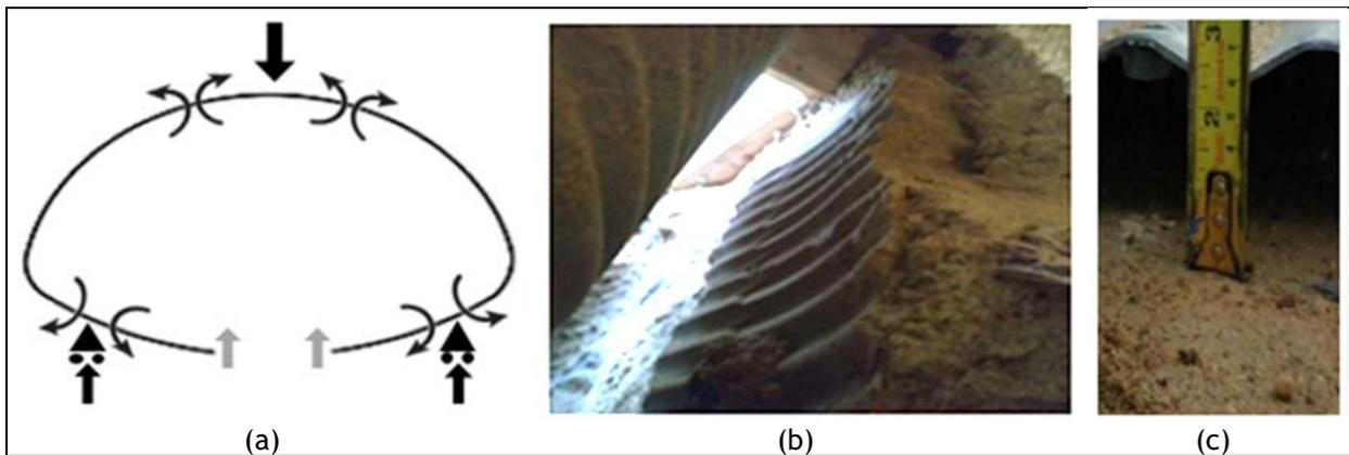
Figure 11-49. CMP arch movement due to the invert detachment: (a) the movement mechanism, and (b) the uplift of the invert-cut CMP arch after loading and soil compaction under the haunch area after exhuming the CMP.
