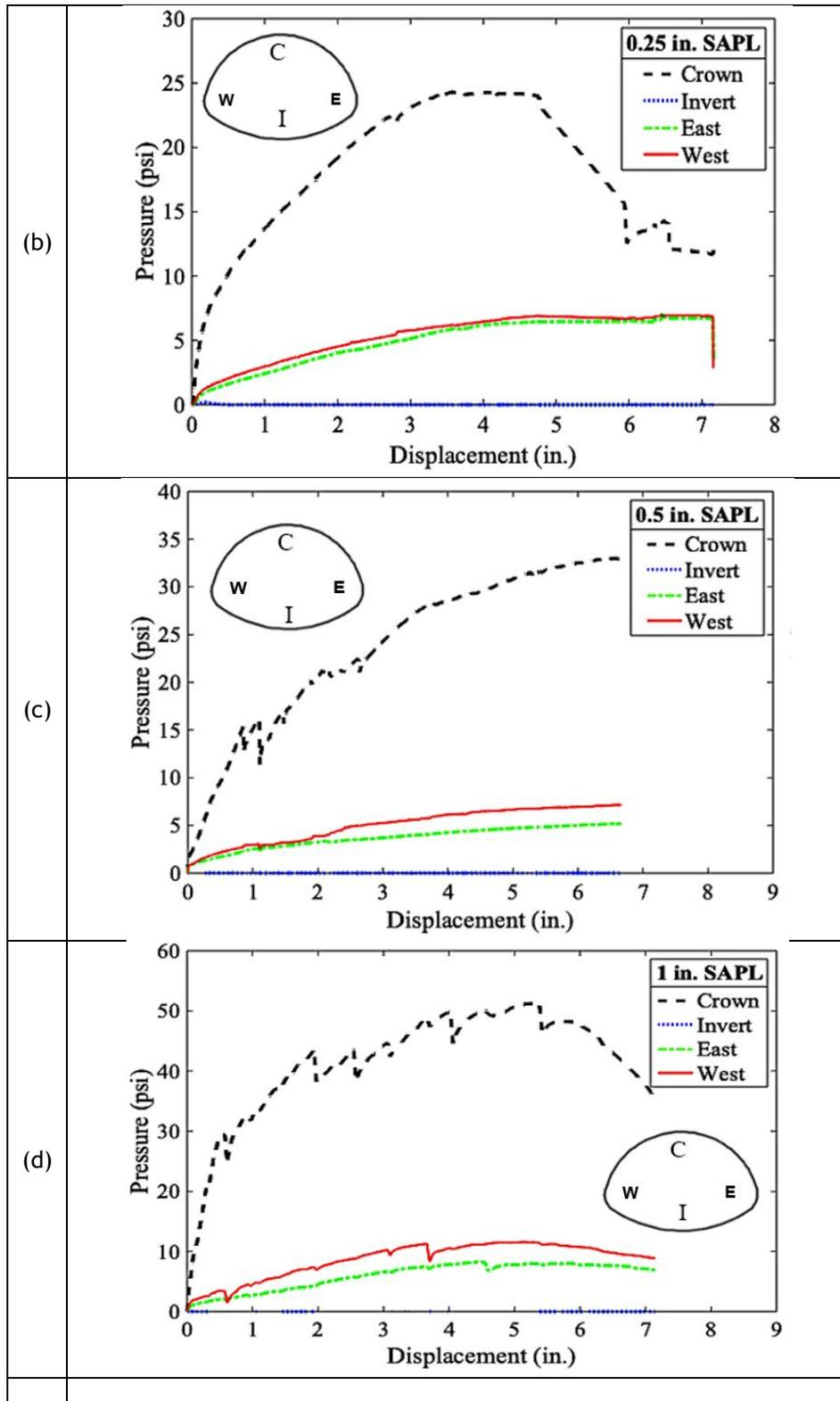
Figure 11-71. Pressure vs. crown displacement graphs: (a) invert-cut bare CMP arch, (b) 0.25 in. SAPL renewed CMP arch, (c) 0.5 in. SAPL renewed CMP arch, and (d) 1 in. SAPL renewed CMP arch.
