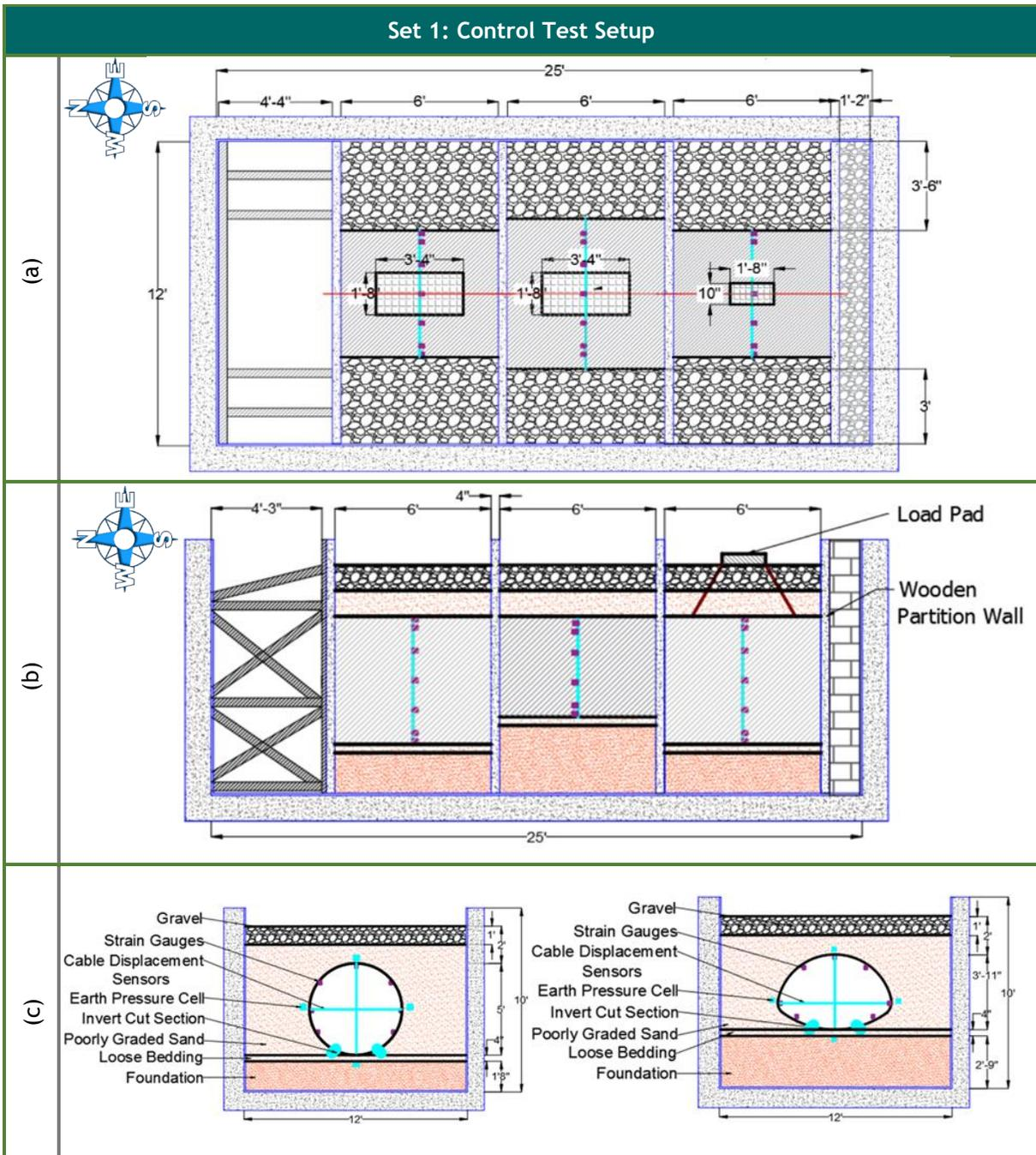
Figure 11-8. The CMPs' burial configuration (control test set): (a) plan view, (b) profile view of the aligned CMPs in the soil box, and (c) cross sectional view of both circular and CMP arch samples.
