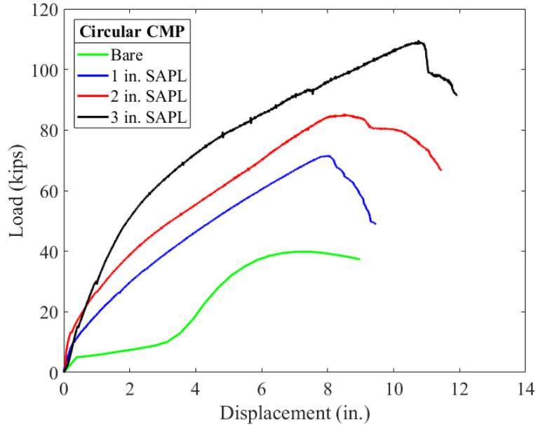
Figure 11-138. Load vs. soil surface settlement comparison graph.
