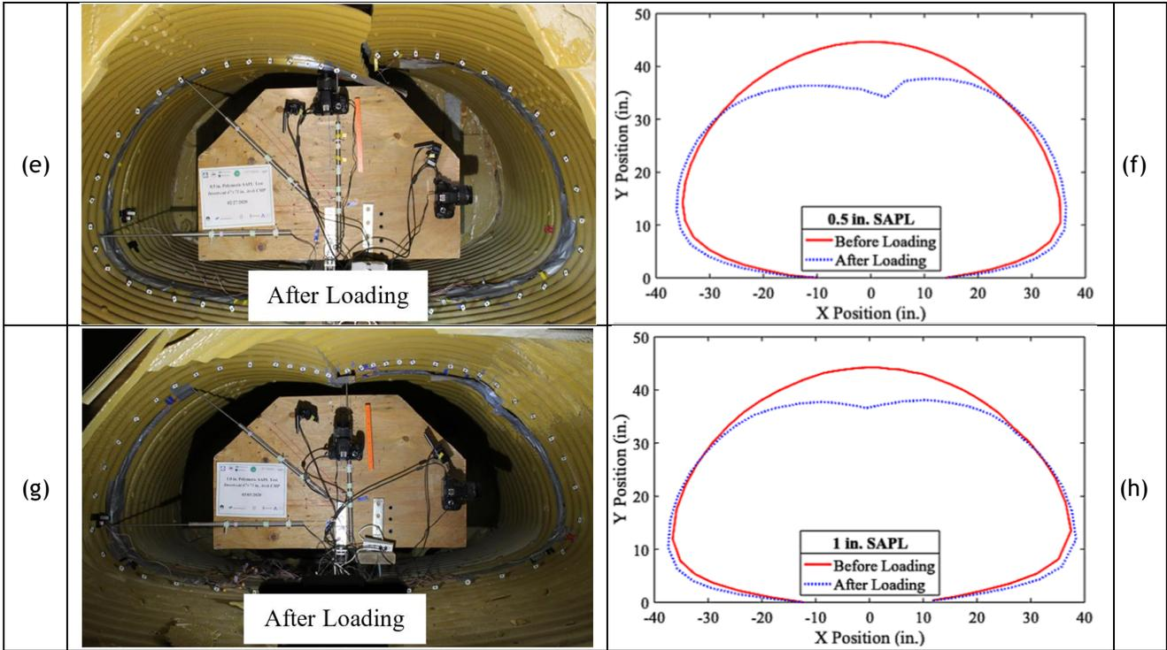
Figure 11-74. Pipe profiling using DIC results: (a) and (b) bare CMP arch, (c) and (d) 0.25 in. SAPL renewed CMP arch, (e) and (f) 0.5 in. SAPL renewed CMP arch, and (g) and (h) 1 in. SAPL renewed CMP arch.
