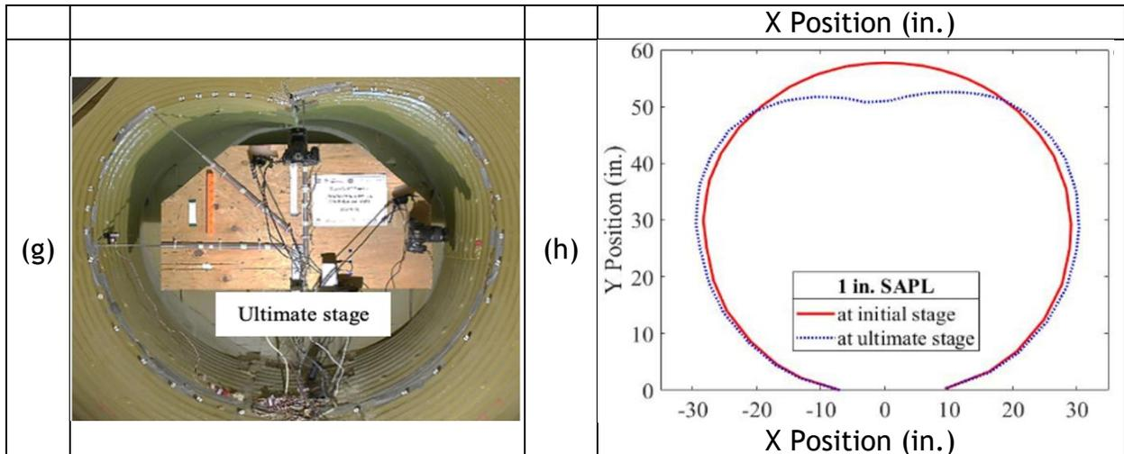
Figure 11-64. DIC results of SAPL renewed circular CMP: (a) and (b) bare CMP, (c) and (d) 0.25 in. SAPL renewed CMP, (e) and (f) 0.5 in. SAPL renewed CMP, (g) and (h) 1 in. SAPL renewed CMP.
