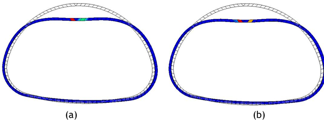
Figure 10E-5. Deformation of the liner at (a) 1<sup>st</sup> plastic strain (b) at ultimate load conditions for 1-in. thick arch polymeric liner.
