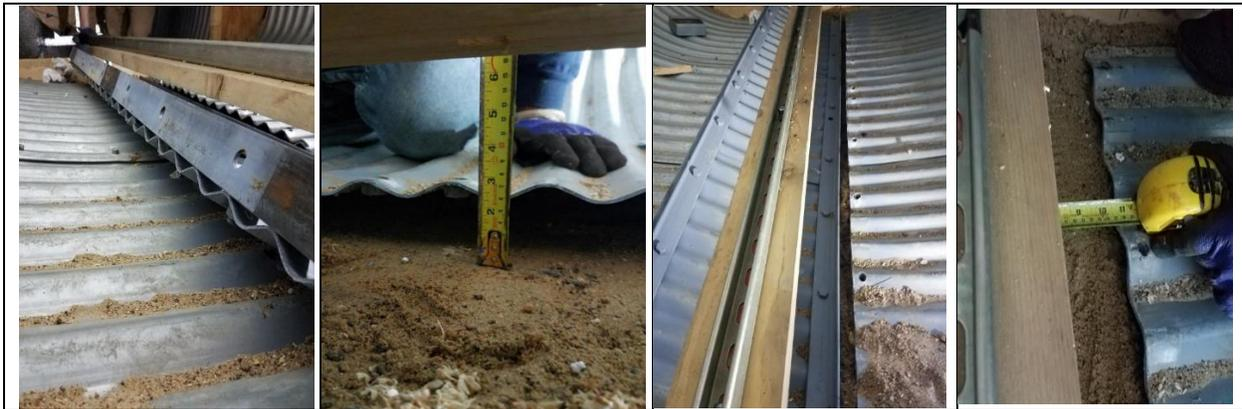
Figure 11-40. CMP movement due to the invert detachment (without any end strips) before loading.
