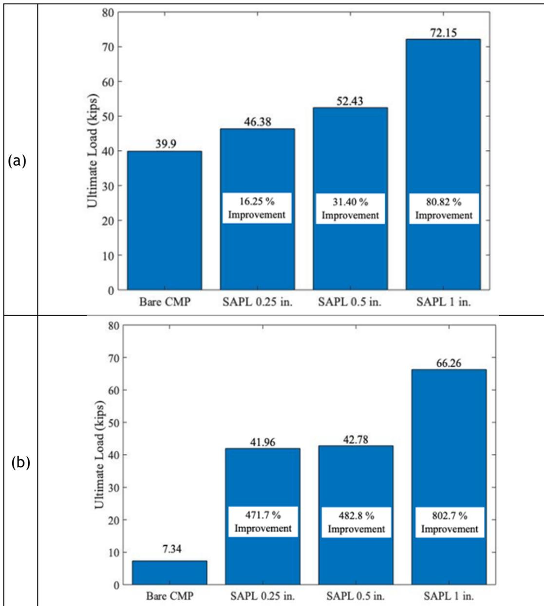
Figure 11-61. Load improvement by SAPL application: (a) ultimate load comparison of renewed SAPL circular CMPs with bare CMP, and (b) load comparison of renewed SAPL CMPs with bare CMP at 2 in. pipe deflection.
