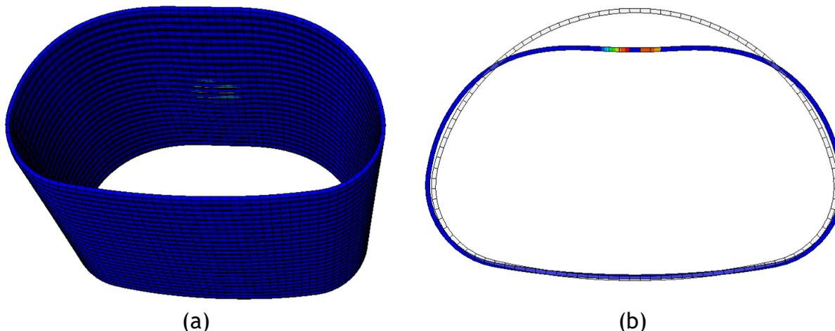
Figure 10-54. (a) Development of plastic strain in the inside liner for 0.75 in. thick arch liner (b) Deformation pattern of 0.75-in. thick arch polymeric SAPL.
