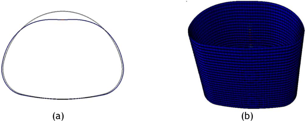
Figure 10-41. (a) Deformation of arch CMP at 1<sup>st</sup> plastic strain in the 0.25-in. thick arch liner, and (b) 1<sup>st</sup> plastic strain in 0.25-in. thick polymeric SAPL.
