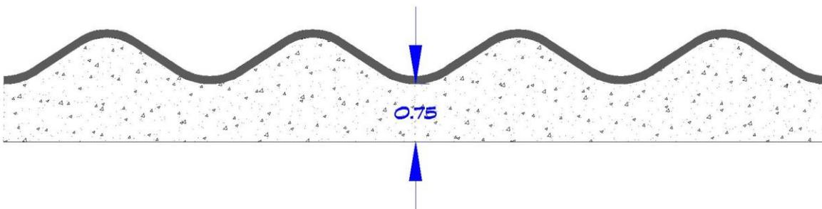
Figure 4-3.  $2\frac{2}{3}\times\frac{1}{2}$ -in. CMP profile lined with an SAPL.
