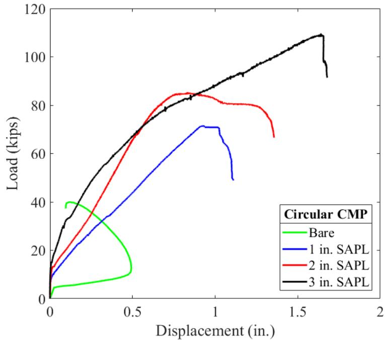
Figure 11-137. Load vs. springline displacement comparison graph.
