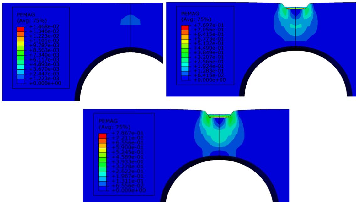
Figure 10-10. Progression of plastic strain under the load pad in soil ((a) at 1 in. settlement, (b) at 4 in. settlement (c) at 5 in. settlement
