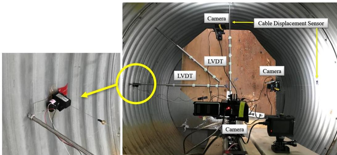
Figure 11-23. LVDTs and cable displacement sensors.
