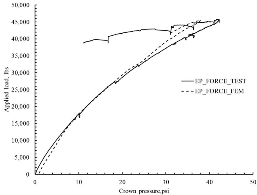
Figure 10-27. Comparison of the earth pressure at crown plotted against the applied load for 0.25 in. thick polymeric SAPL
