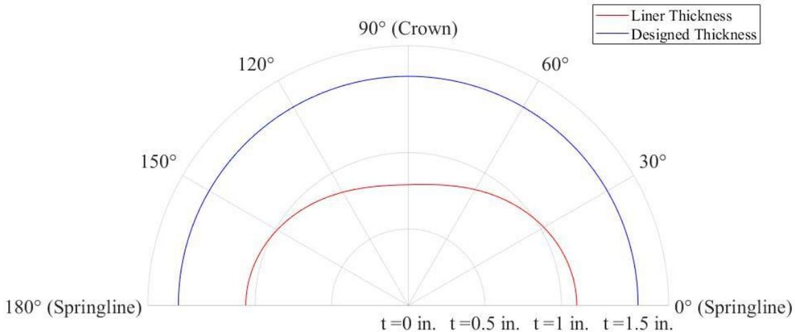
Figure 7-4. SAPL average installed thicknesses versus 1.5 in. design thickness inside an 84-in. diameter circular CMP.
