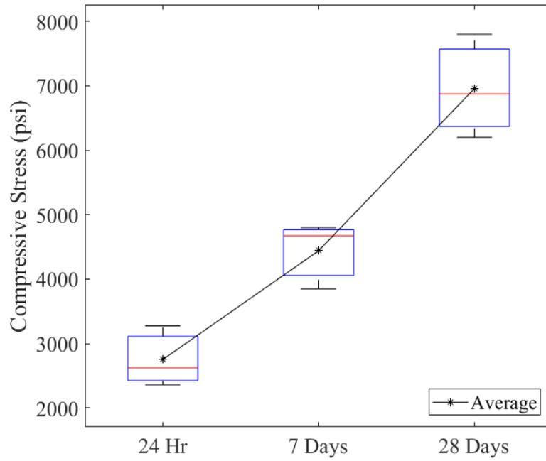
Figure 11-140. Cube samples taken from SAPL batch sprayed on circular CMPs.
