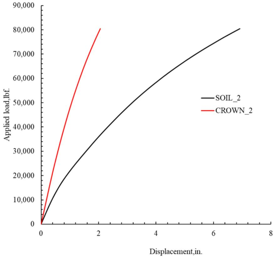
Figure 10B- 14. Load displacement plot from FE analysis for 2-in. thick polymeric circular liner.
