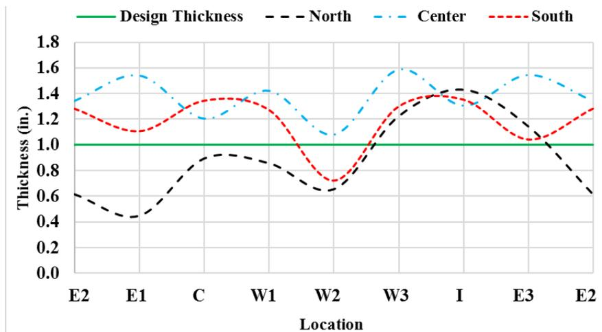
Figure 11-135. Thickness measurement for the 1-in. thick cementitious SAPL renewed circular CMP.
