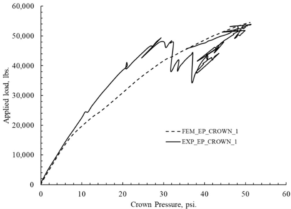
Figure 10E-9. Comparison of the earth pressure with applied load for 1-in. thick arch polymeric liner.
