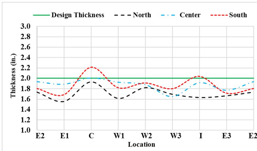
Figure 11-94. Thickness measurement for the 2-in. thick cementitious SAPL renewed CMP arch.
