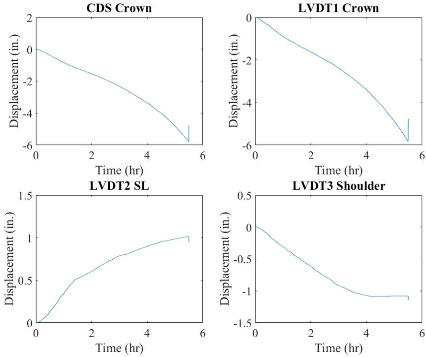
Figure 11-89. Mechanical sensors result for 2-in. thick SAPL renewed invert-cut CMP arch.
