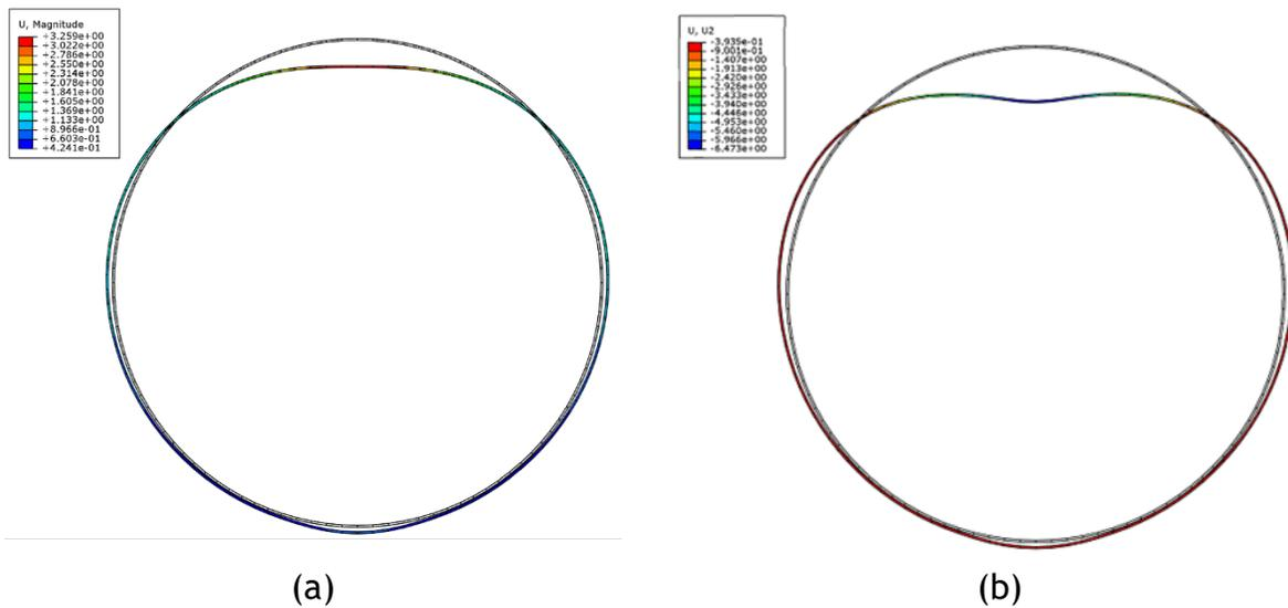
Figure 10-23. (a) Deformation of CMP at the time of the 1st plastic strain, and (b) Deformation of CMP at the ultimate load condition for 0.25 in. thick polymeric SAPL
