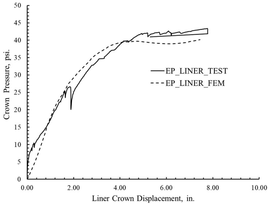
Figure 10B- 3. Comparison of the earth pressure with liner displacement at crown for 0.5 in. thick polymeric circular liner.
