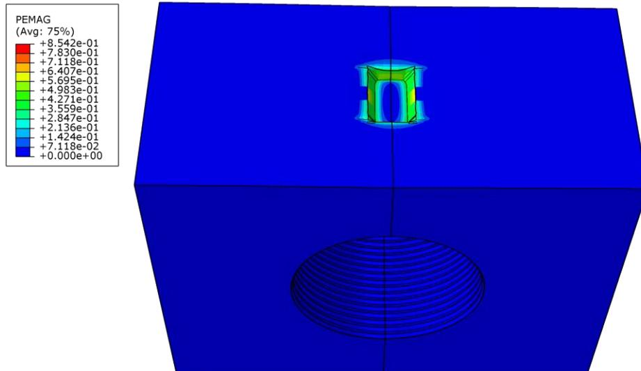
Figure 10-9. Plastic strain due to the soil failure in the loaded area at 5-inch settlement.
