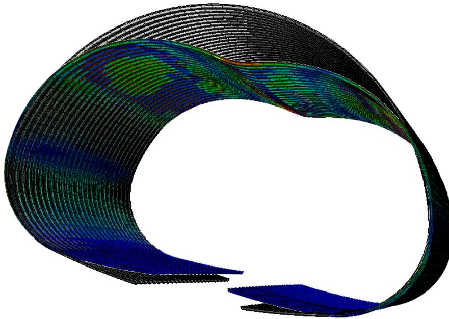
Figure 10-38. Deformation of the invert cut arch CMP from the FE model.
