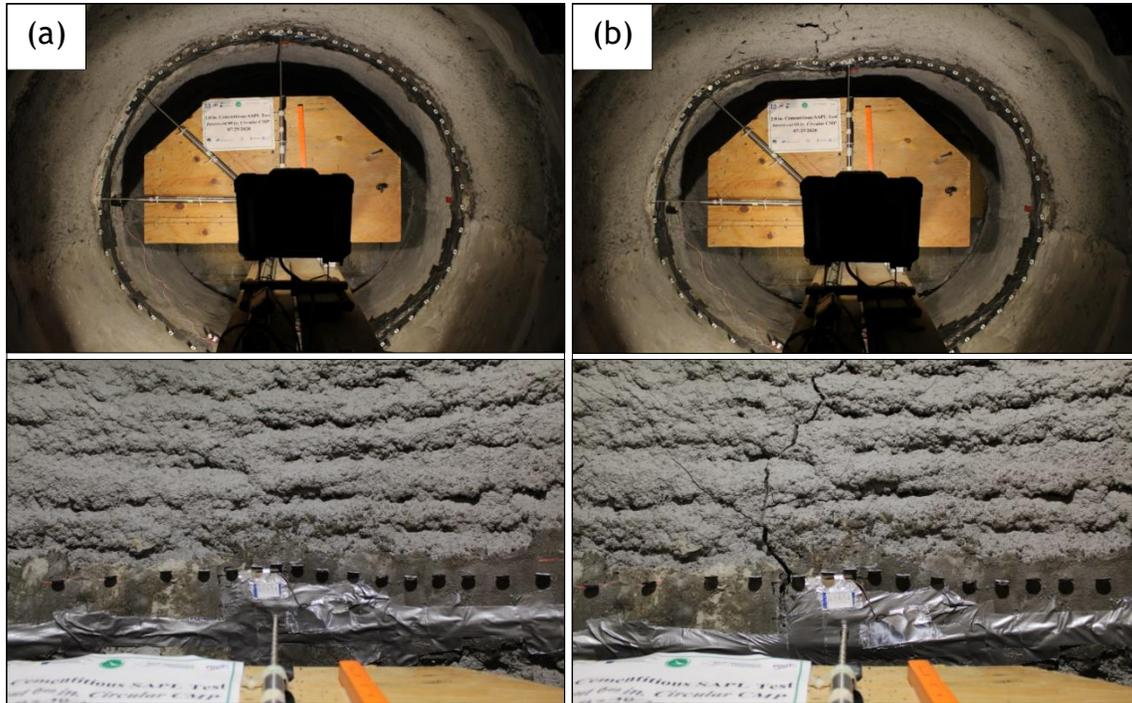
Figure 11-118. Invert-cut circular CMP renewed with 2 in. cementitious SAPL: (a) before loading, and (b) after loading.
