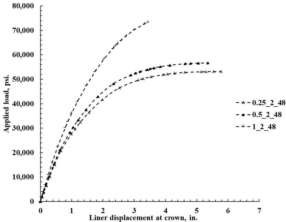
Figure 10E-15. Load displacement plot for Invert-cut Circular 48 in. CMPs with 2 ft cover and 0.25, 0.5, and 1 in. thick polymeric liner.
