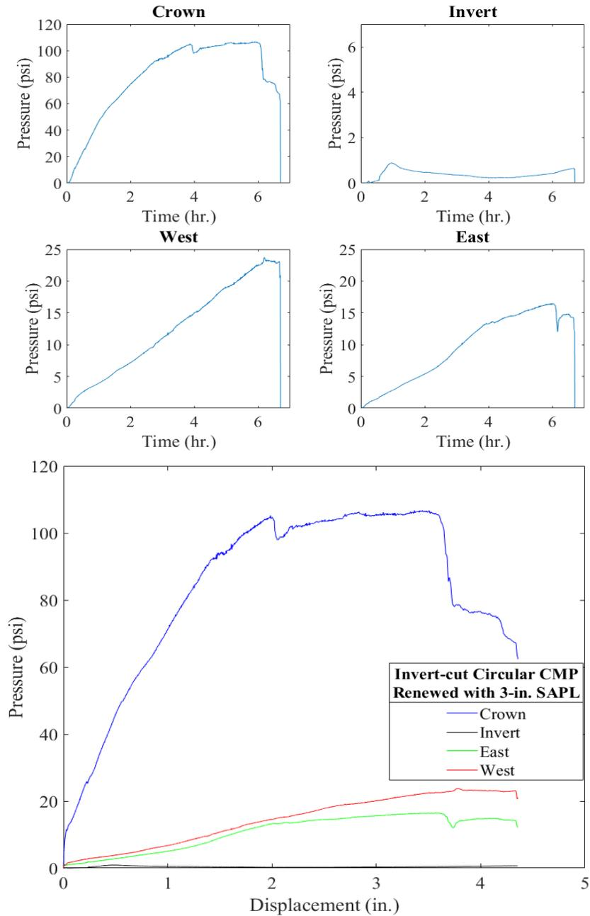
Figure 11-111. Earth pressure cell results for the 3-in. thick SAPL renewed invert-cut circular CMP with respect to: (top) time, and (bottom) crown displacement.
