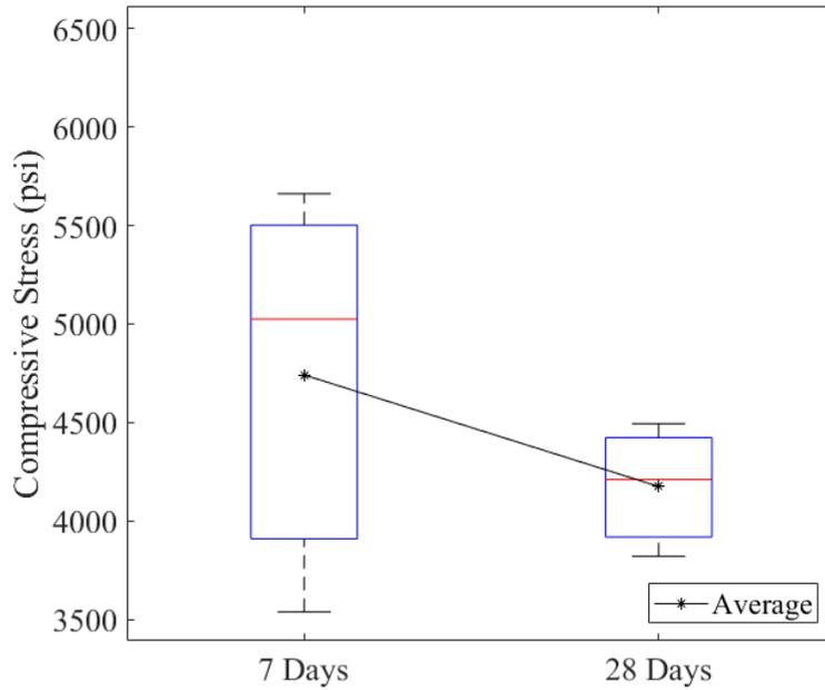
Figure 11-143. Box plot for the 6 × 12-cylinder samples taken from SAPL batch sprayed on circular CMPs.
