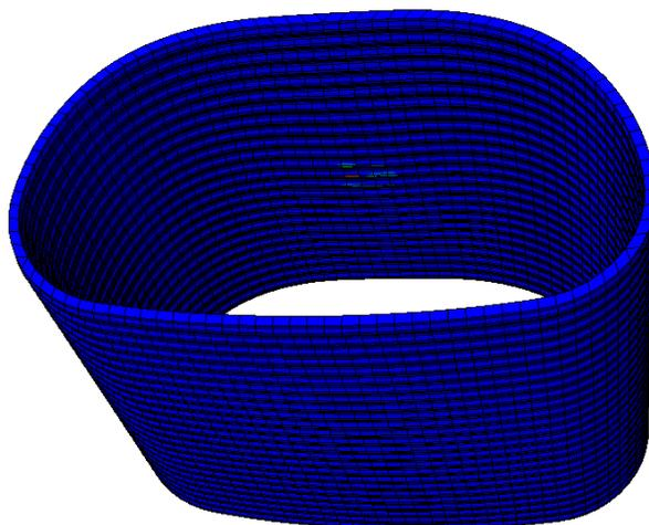
Figure 10-48. 1<sup>st</sup> plastic strain in the liner for 1-in. thick arch polymeric SAPL.
