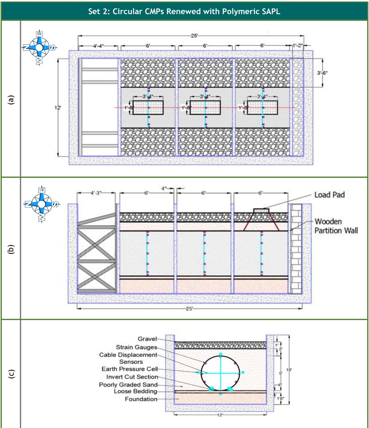
Figure 11-9. The CMPs' burial configuration (SAPL renewed testing): (a) plan view, (b) profile view of the aligned CMPs in the soil-box, and (c) cross sectional view of the circular CMP.
