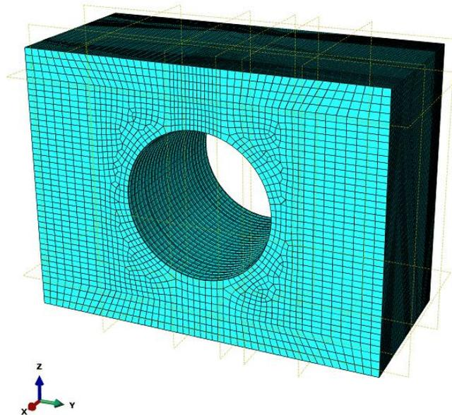
Figure 10-6. Mesh size distribution in the soil.
