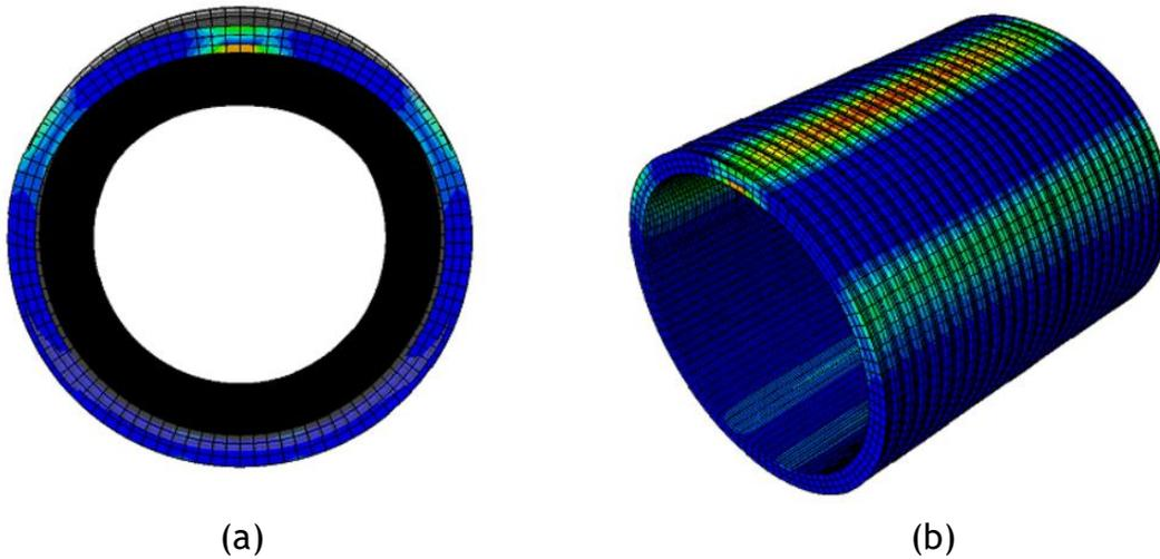
Figure 10F-9. (a) Deformation of 3 in. thick cementitious liner under ultimate load, and (b) crack location in 3 in. thick cementitious liner.
