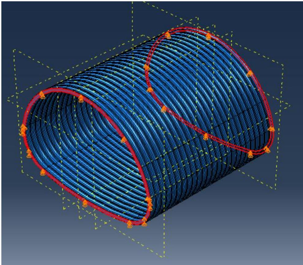
Figure 10-50. 1-in. thick polymeric SAPL liner showing the restriction of the vertical movement at two ends.
