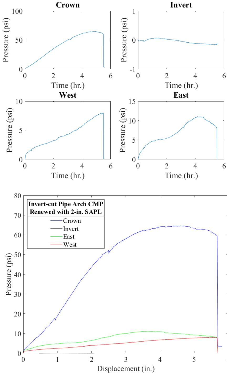
Figure 11-88. Earth pressure cell results for the 2-in. thick SAPL renewed invert-cut CMP arch with respect to: (top) time, and (bottom) crown displacement.
