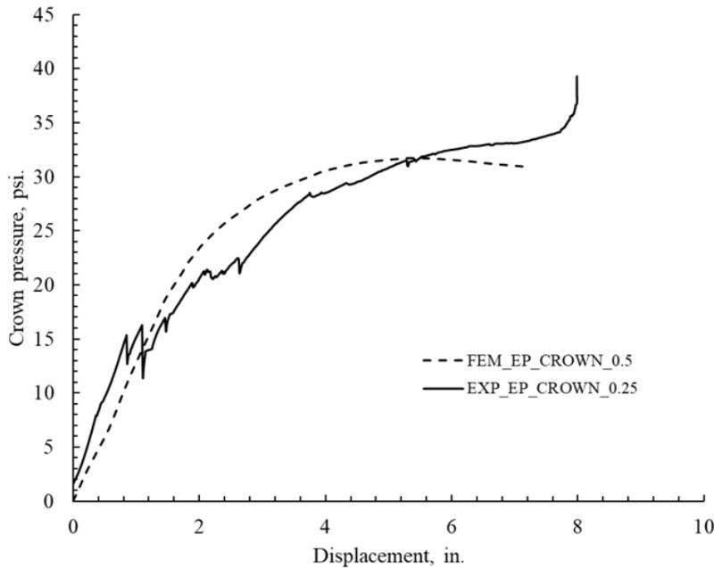
Figure 10E-3. Comparison of the earth pressure with liner displacement at crown for 0.5-in. thick arch polymeric liner.
