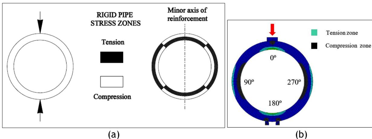
Figure 2-11. Rigid pipes under vertical loading: (a) rigid pipe stress zones (Hydraulics Manual M 23-03.06 2019), and (b) finite element modeling of a rigid reinforced concrete pipe (RCP) (Darabnough Tehrani 2016).
