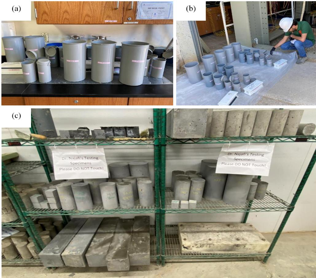
Figure 11-38. Mechanical properties testing samples: (a) compressive testing cylinders molds, (b) mold preparation, and (c) sample storage at a curing room.
