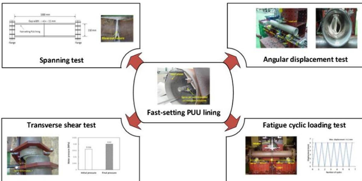
Figure 2-26. The structural behavior and performance of a fast-setting polyurea-urethane (PUU) SAPL as a structural lining material for rehabilitating water pipes (Ha et al. 2016).
