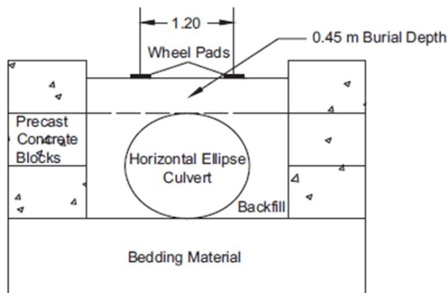
Figure 2-33. Cross section of culvert position and load applied (Tetreault et al. 2018).
