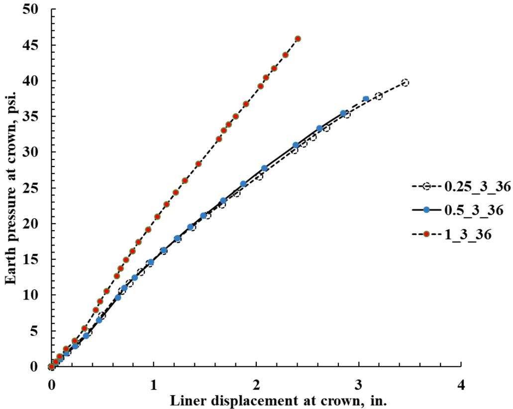
Figure 10E-20. Earth pressure at 4 in. above the crown vs. crown displacement for Invert-cut circular 36 in. CMPs with 3 ft cover and 0.25, 0.5, and 1 in. thick polymeric liner.
