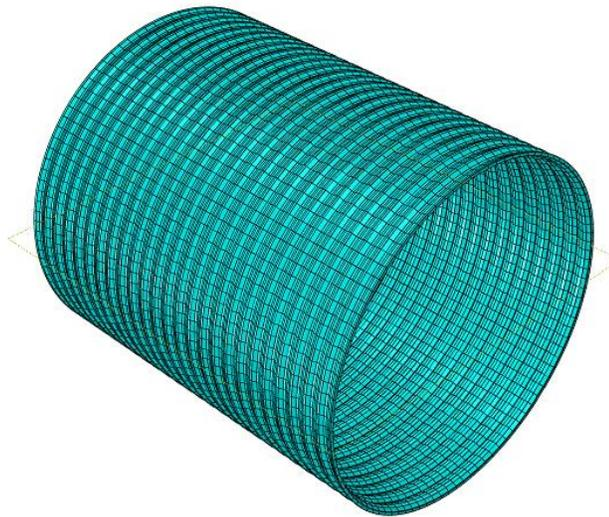
Figure 10-4. 1 in. liner model in FE.
