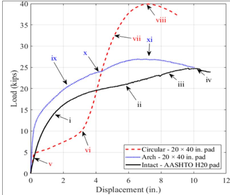
Figure 11-42. Control test: applied load through the steel load pad vs. soil settlement.
