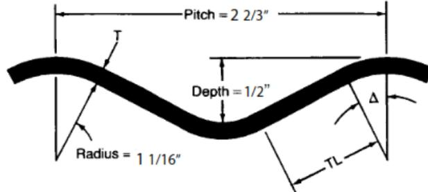
Figure 8-3 Typical corrugation profile showing tangent angle.
