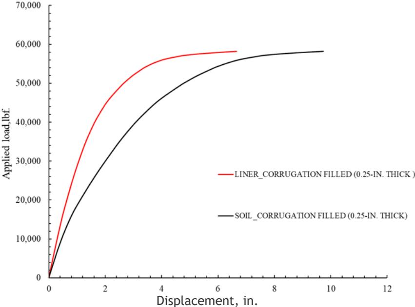
Figure 10-34. Load displacement plot for the liner displacement at crown and settlement of soil from FE analysis for 0.25-in. thick (filled over the crest) polymeric SAPL.
