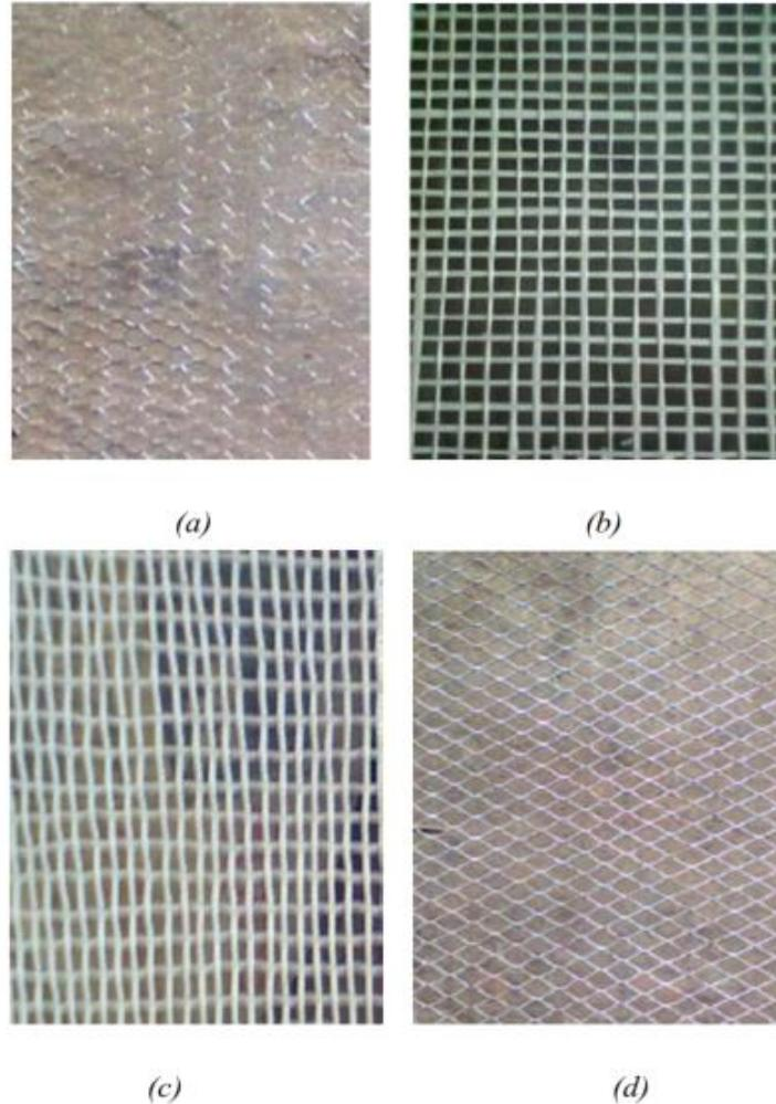
Figure 3-5. Types of Mesh. (a) Hexagonal Iron Mesh, (b) Woven PP, (c) Woven Nylon 66, (d) Expanded Metal Mesh.
