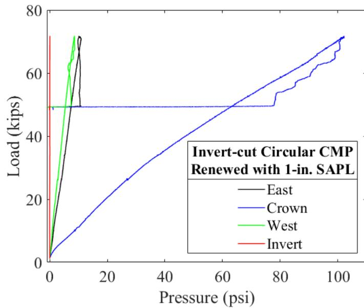
Figure 11-134. Load vs. pressure for the 1-in. thick SAPL renewed invert-cut circular CMP.
