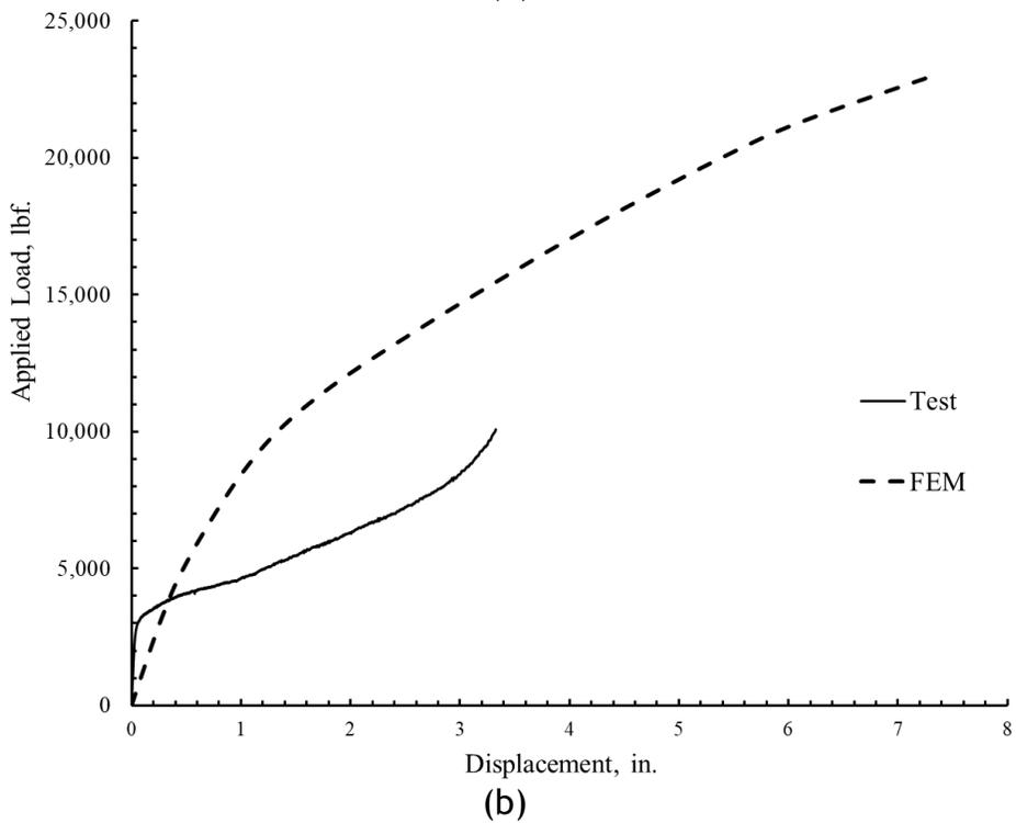
Figure 10A- 2. Load displacement for the soil movement just beneath the load pad (a) Comparison at the ultimate conditions, and (b) Comparison when the inverts just meet.
