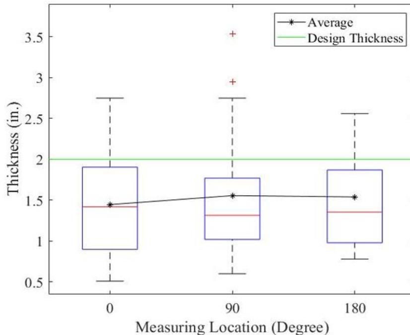
Figure 7-3. SAPL measured thicknesses versus 2 in. design thickness, (arch pipes renewed with cementitious SAPL)
