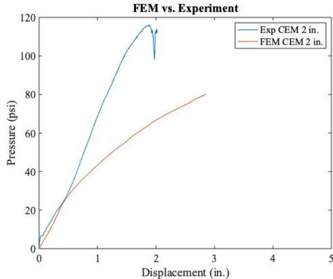
Figure 10F-5. Earth pressure 4 in. above the crown vs. crown displacement for 2-in. thick cementitious liner.
