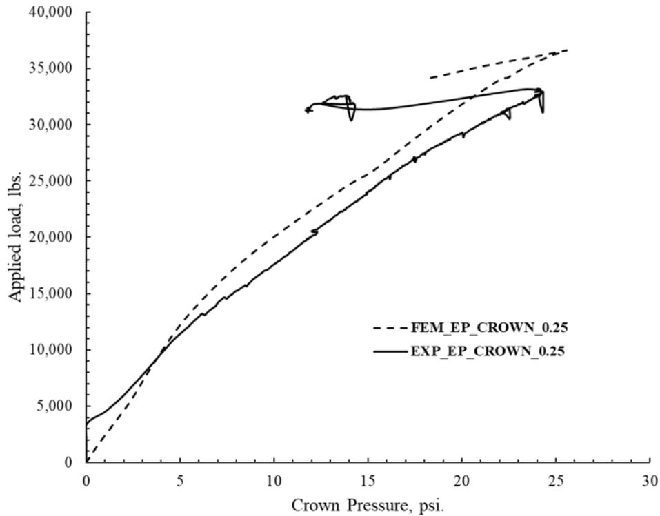
Figure 10-46. Comparison of the earth pressure at crown plotted against the applied load for 0.25-in. thick arch polymeric SAPL.
