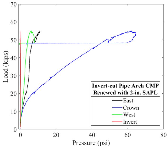
Figure 11-93. Load vs. pressure for the 2-in. thick SAPL renewed invert-cut CMP arch.
