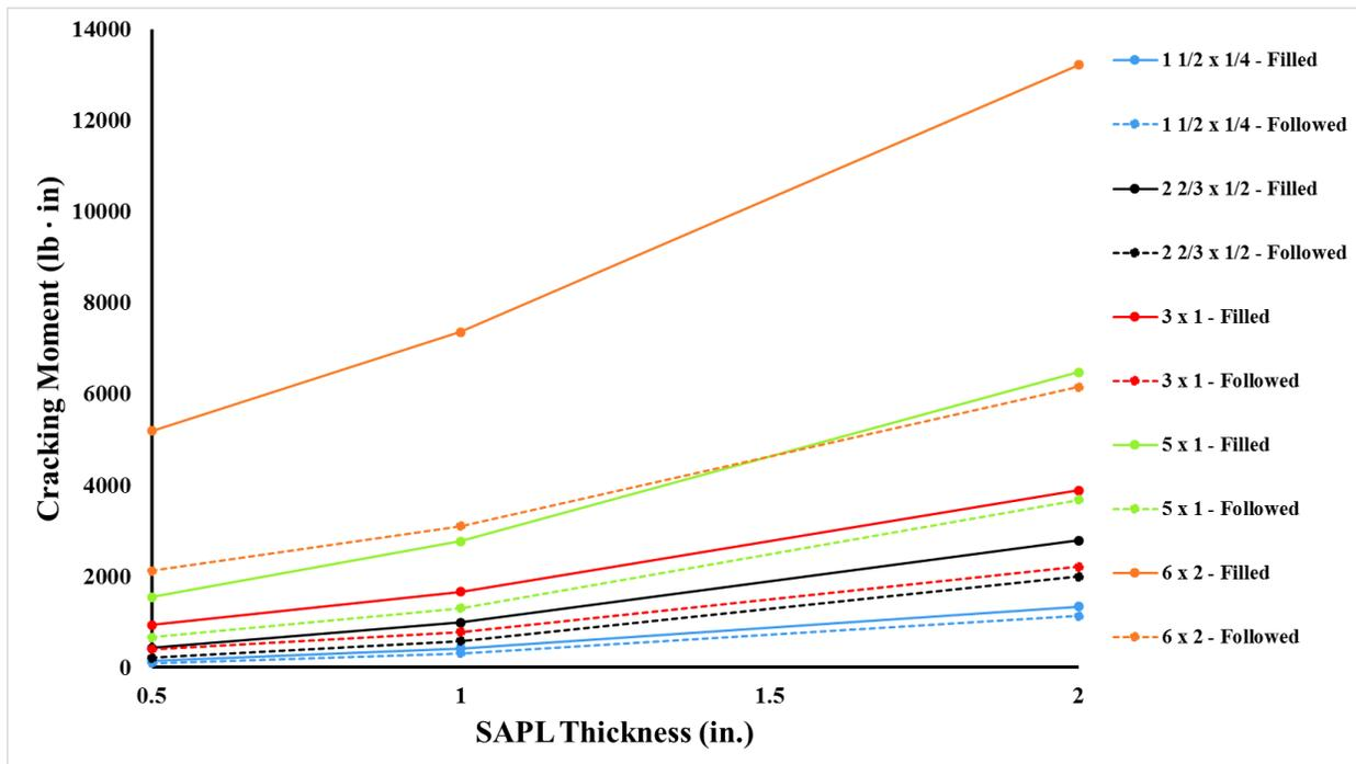
Figure 4-6. Cementitious SAPL thickness versus cracking moment.
