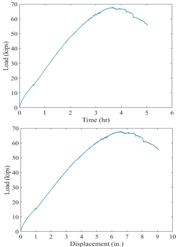
Figure 11-78. Invert-cut CMP arch renewed with 3-in. thick cementitious SAPL subjected to static live load: (top) load-time and (bottom) load-soil displacement graphs.
