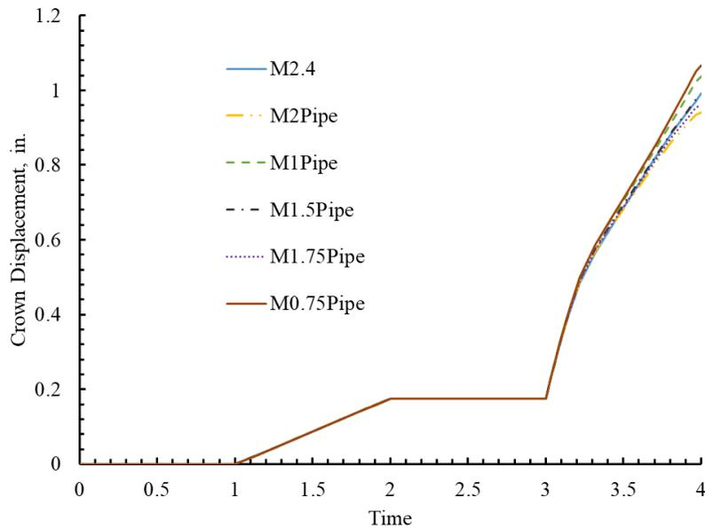
Figure 10-7. Load displacement plot for the pipe at the crown.
