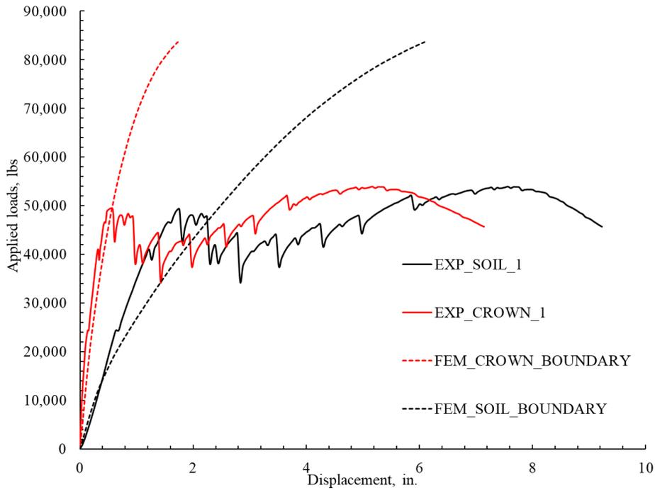
Figure 10-51. Load displacement curve comparison between FEM and Experiment for 1-in. thick SAPL with the boundary conditions at the end.
