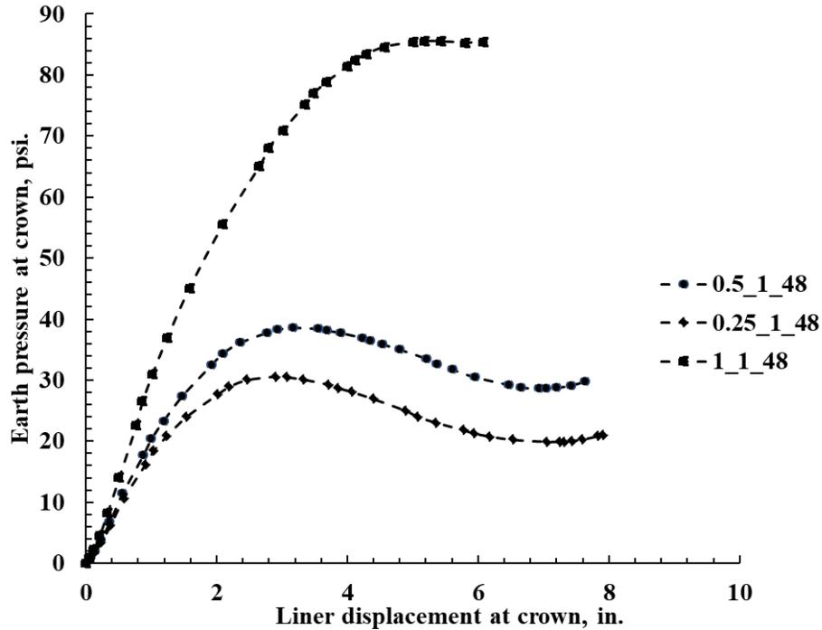
Figure 10E-18. Earth pressure at 4 in. above the crown vs. crown displacement for Invert-cut circular 48 in. CMPs with 1 ft cover and 0.25, 0.5, and 1 in. thick polymeric liner.
