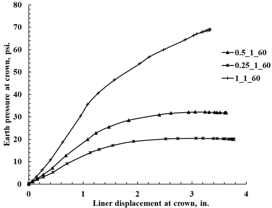
Figure 10D-4. Earth pressure at 4 in. above the crown vs. crown displacement for 60-in. invert-cut circular CMP with 1-ft cover and 0.25-, 0.5-, and 1-in. polymeric circular thick liner.
