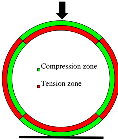
Figure 11-108. Compression and tension zones of a circular pipe subjected to a vertical load.
