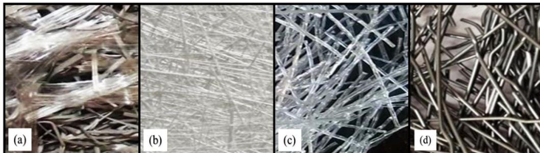
Figure 3. Macro-fibers used in concrete linings: (a) polypropylene fibers, (b) fiberglass, (c) polyolefin fibers, and (d) steel fibers.
