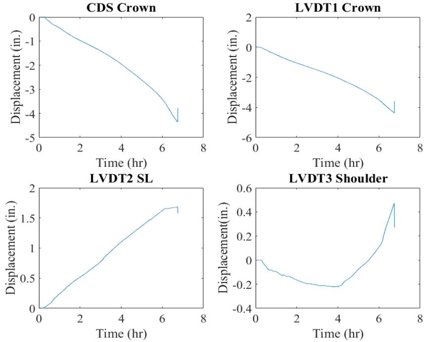
Figure 11-112. Mechanical sensors result for 3-in. thick SAPL renewed invert-cut circular CMP.
