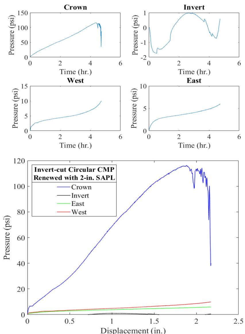
Figure 11-120. Earth pressure cell results for the 2-in. thick SAPL renewed invert-cut circular CMP with respect to: (top) time, and (bottom) crown displacement.
