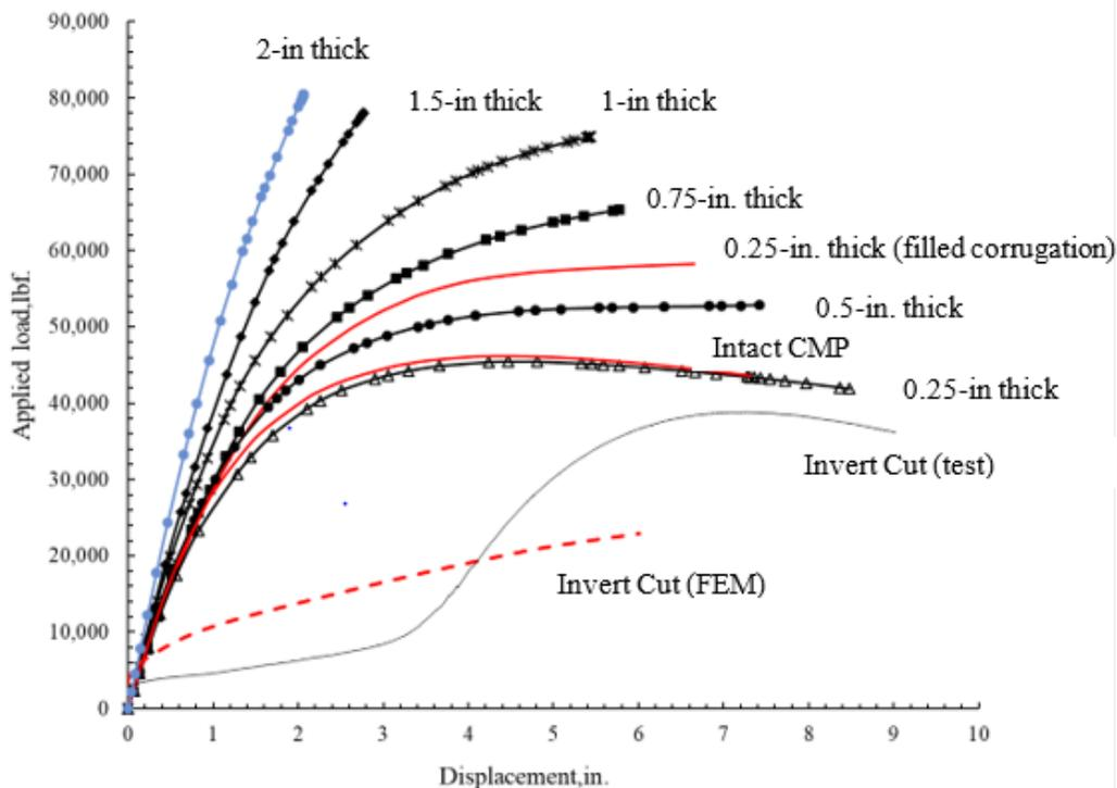
Figure 10-36. Comparison of the load-displacement plot at the crown obtained from all the FE results.
