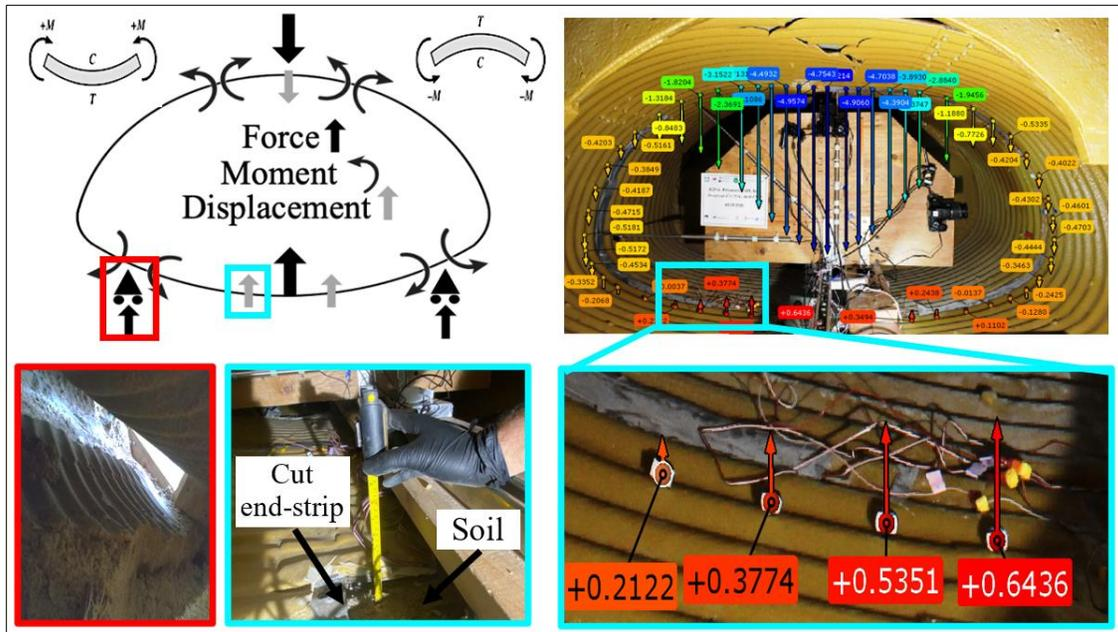
Figure 11-72. CMP arch behavior due to the vertical load, where the red boxes show the soil support under the pipe on the west haunch area and the blue boxes illustrates the pipe upward movement.
