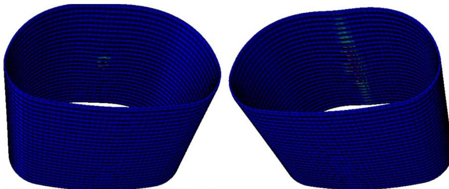
Figure 10-47. First plastic strain from FE model for 0.5-in. thick arch polymeric SAPL.
