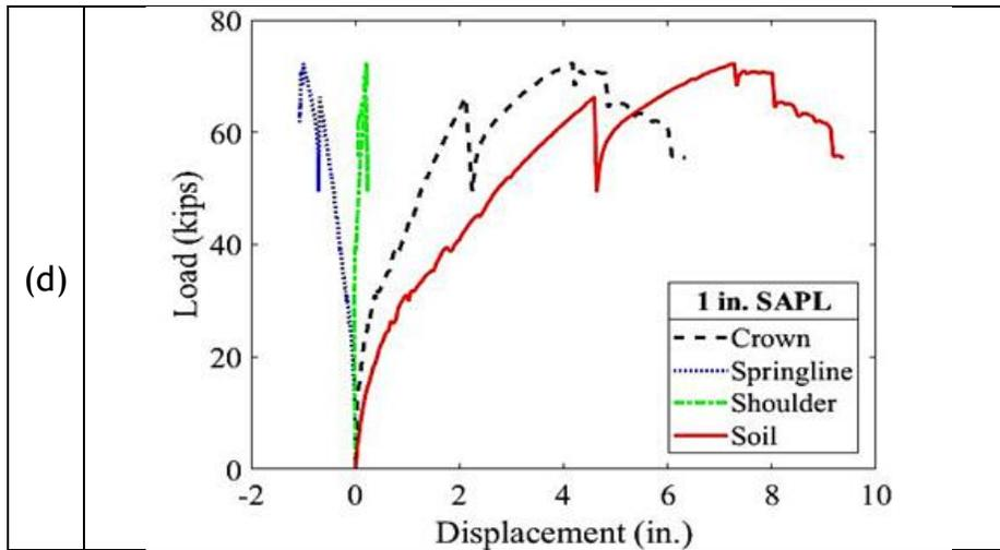
Figure 11-59. Load vs. displacement results for CMP samples and soil: (a) bare invert cut CMP, (b) 0.25 in. SAPL renewed CMP, (c) 0.5 in. SAPL renewed CMP and (d) 1 in. SAPL renewed CMP.
