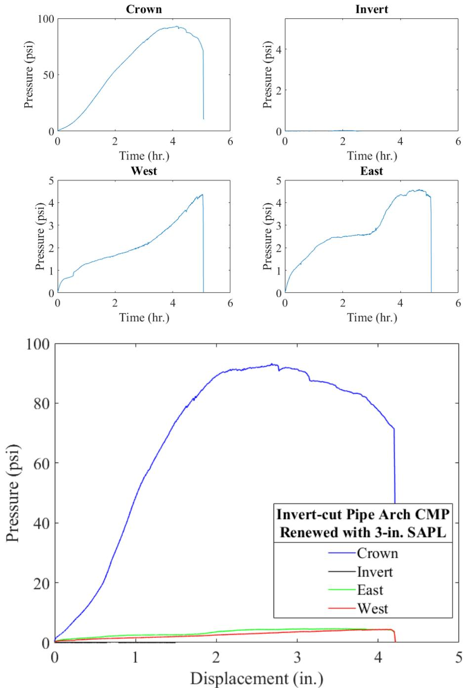
Figure 11-79. Earth pressure cell results for the 3-in. thick SAPL renewed invert-cut CMP arch with respect to: (top) time, and (bottom) crown displacement.
