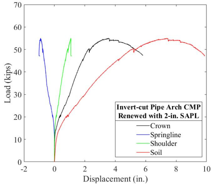
Figure 11-92. Load vs. displacement of the soil surface, crown, springline, and shoulder of the 2-in. thick SAPL renewed invert-cut CMP arch due to the applied static load.
