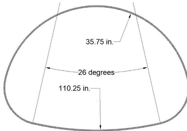
Figure 8-5 Key Dimensions of 47"x71" Pipe-arch
