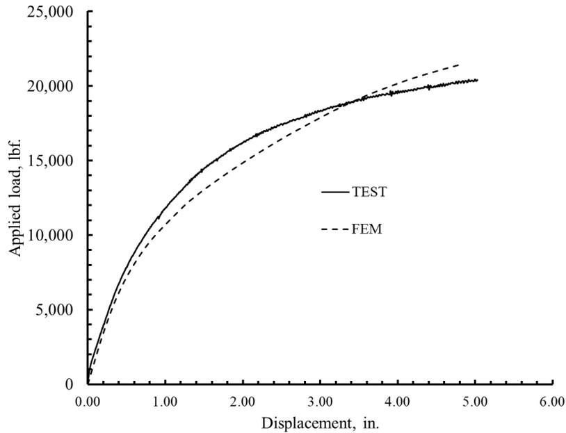
Figure 10-12. Load displacement curve for soil at 5-in. displacement of soil of intact CMP.
