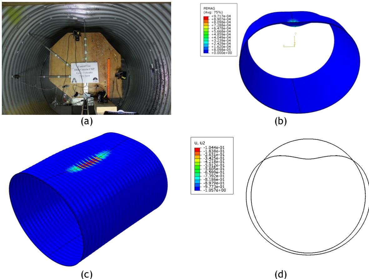
Figure 10-11. Plastic strain and deflection pattern in CMP (a) Experimental Result (b), (c) and (d)FEM Result (scaled up by 5 times).
