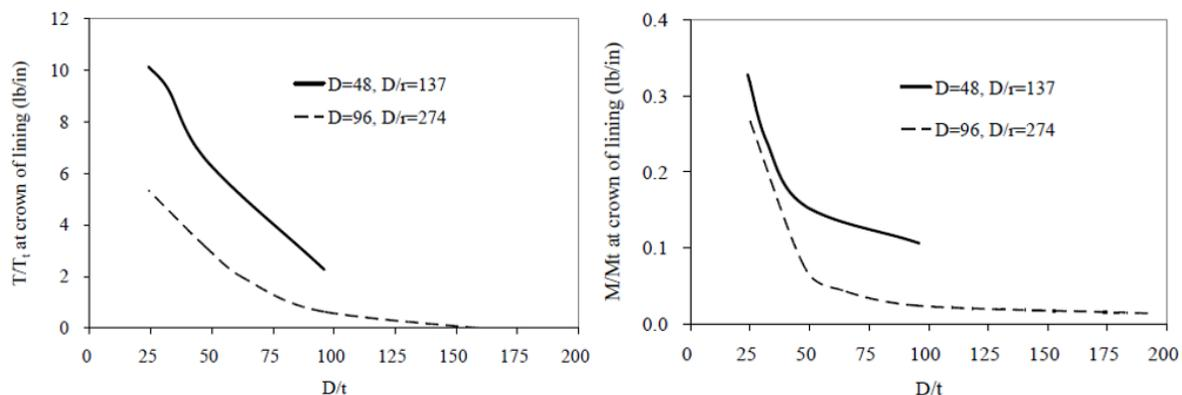
Figure 2-27. Axial forces, T (left) and bending moments, M (right) at the CMP crown (Davidson et al. 2008).
