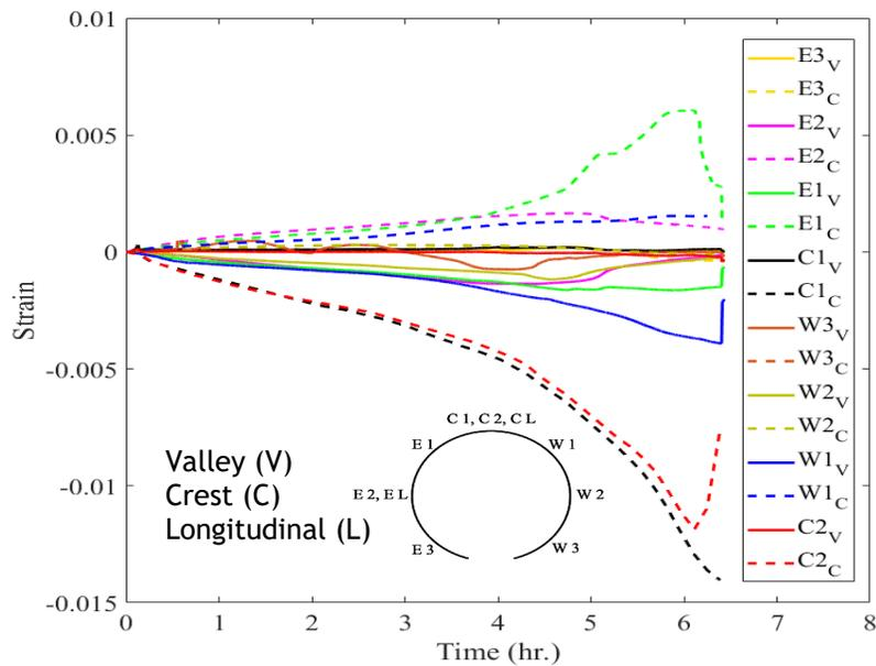
Figure 11-122. Strain gauges result for 2-in. thick SAPL renewed invert-cut circular CMP.
