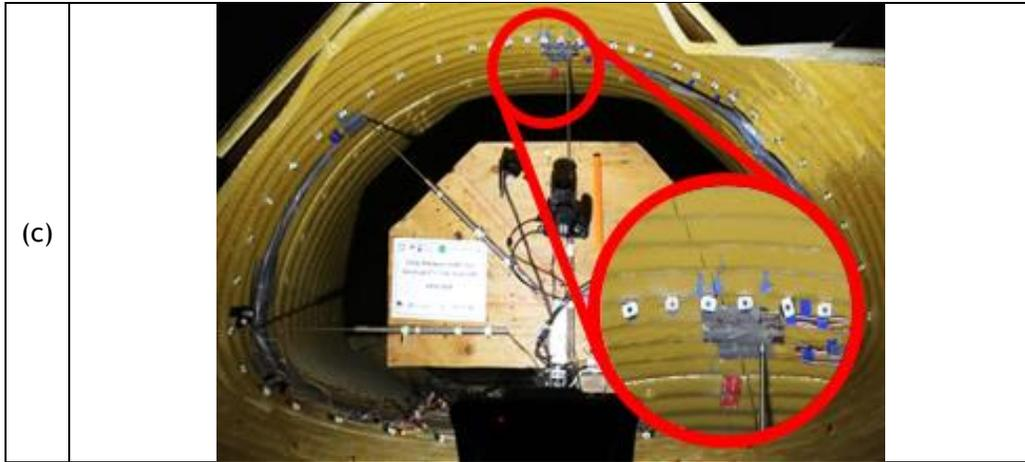
Figure 11-69. Formation of the first structural crack: (a) 0.25 in. SAPL renewed CMP arch at 29.32 kips, (b) 0.5 in. SAPL renewed CMP arch at 26.27 kips, and (c) 1 in. SAPL renewed CMP arch at 41.08 kips.
