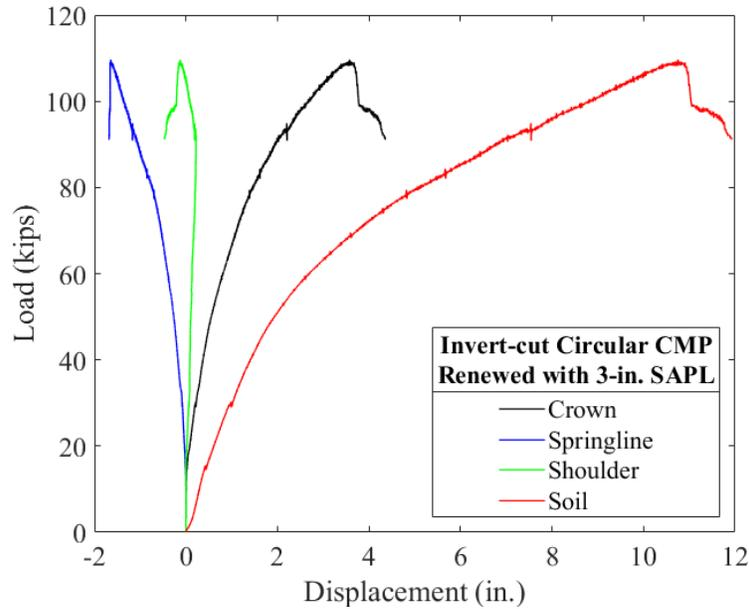
Figure 11-115. Load vs. displacement of the soil surface, crown, springline, and shoulder of the 3-in. thick SAPL renewed invert-cut circular CMP due to the applied static load.
