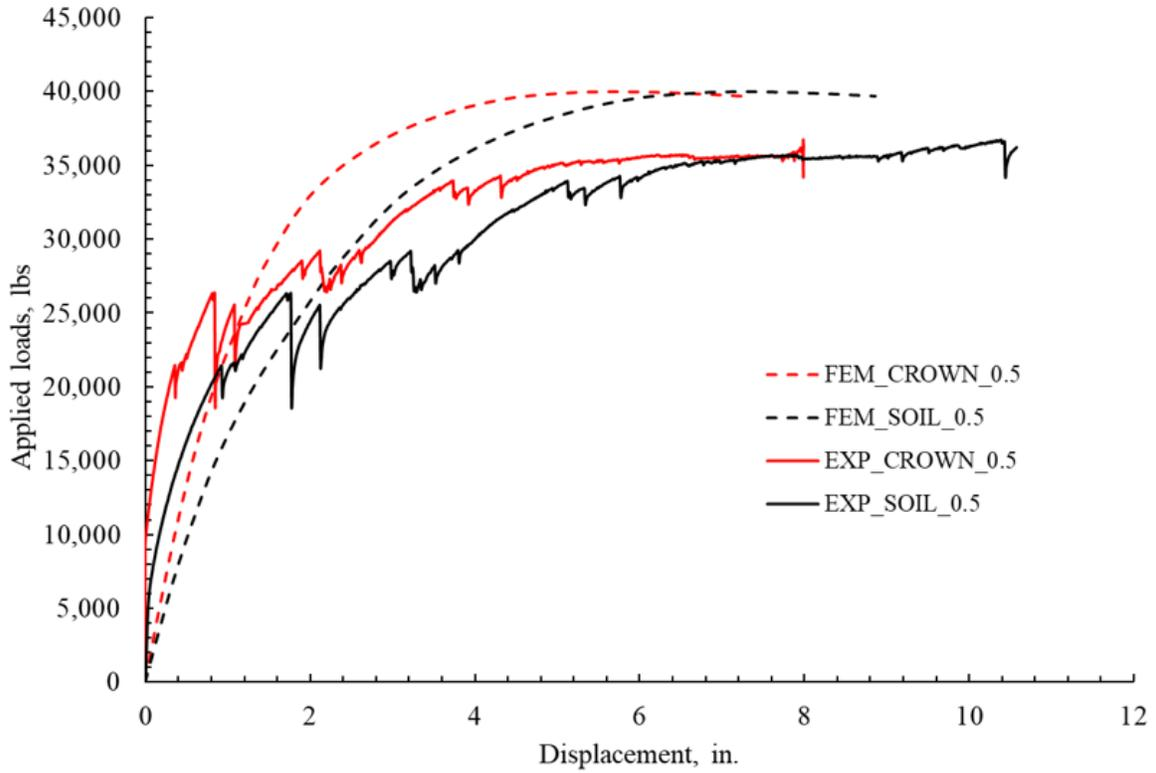
Figure 10E- 2. Comparison of load displacement plot for the 0.5-in. thick arch polymeric liner.
