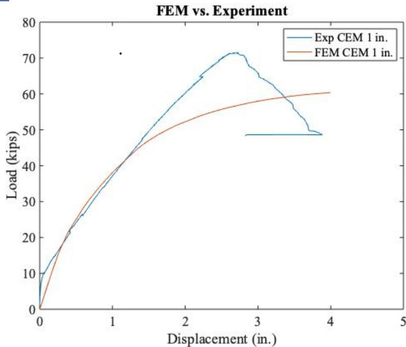
Figure 10F-1. Load displacement plot for 1-in. thick cementitious liner.
