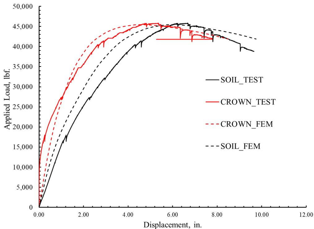
Figure 10-25. Comparison of the liner displacement at crown for 0.25 in. thick polymeric SAPL between experiment and FEM results.
