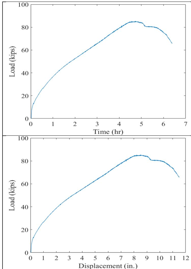
Figure 11-119. Invert-cut circular CMP renewed with 2-in. thick cementitious SAPL subjected to static live load: (top) load-time, and (bottom) load-soil displacement graphs.
