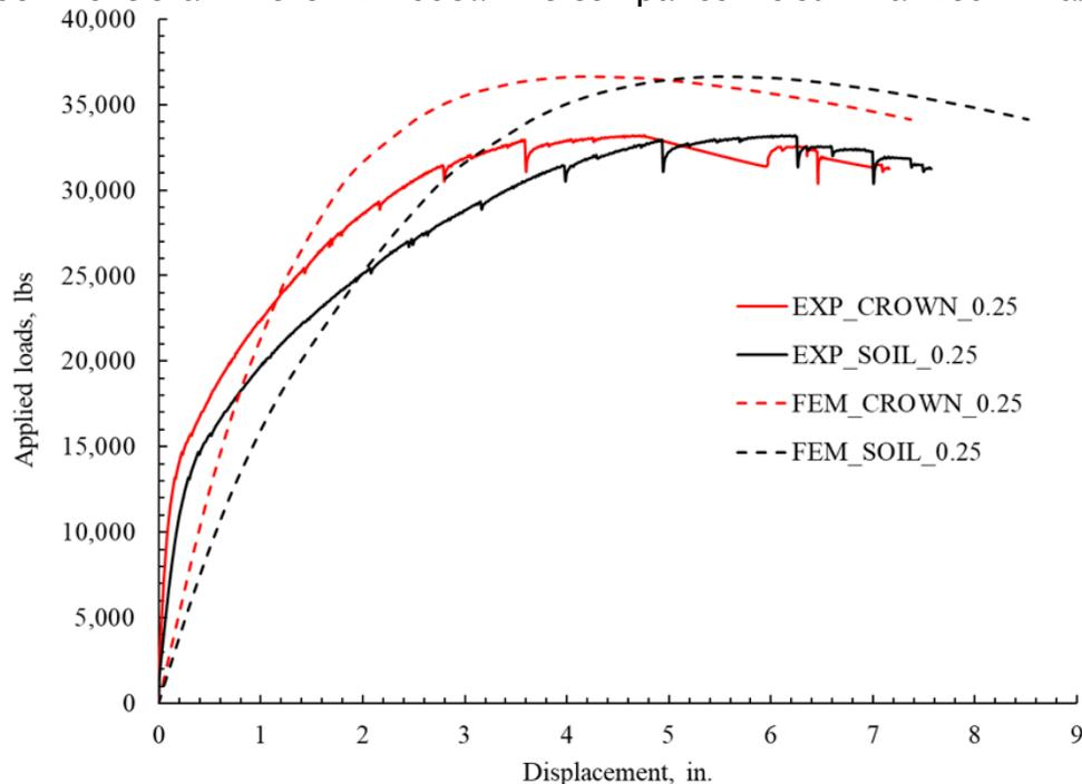
Figure 10-44. Comparison of the liner displacement at crown and soil settlement for 0.25 in. thick arch polymeric SAPL between Experiment and FEM results.
