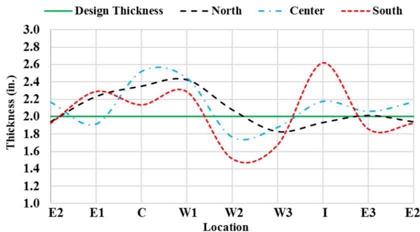
Figure 11-126. Thickness measurement for the 2-in. thick cementitious SAPL renewed circular CMP.
