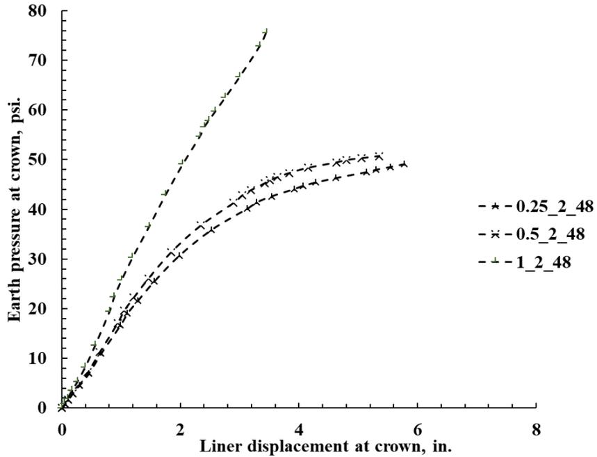
Figure 10E-16. Earth pressure at 4 in. above the crown vs. crown displacement for Invert-cut Circular 48 in. CMPs with 2 ft cover and 0.25, 0.5, and 1 in. thick polymeric liner.
