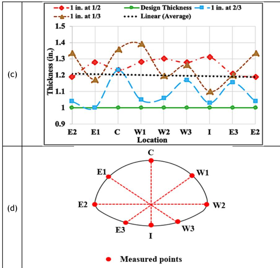
Figure 11-66. Thickness measurement results of polymeric SAPL renewed CMPAs: (a) quarter, (b) half, (c) one inch SAPL renewed CMP arch samples, and (d) measured locations in circumferential direction.
