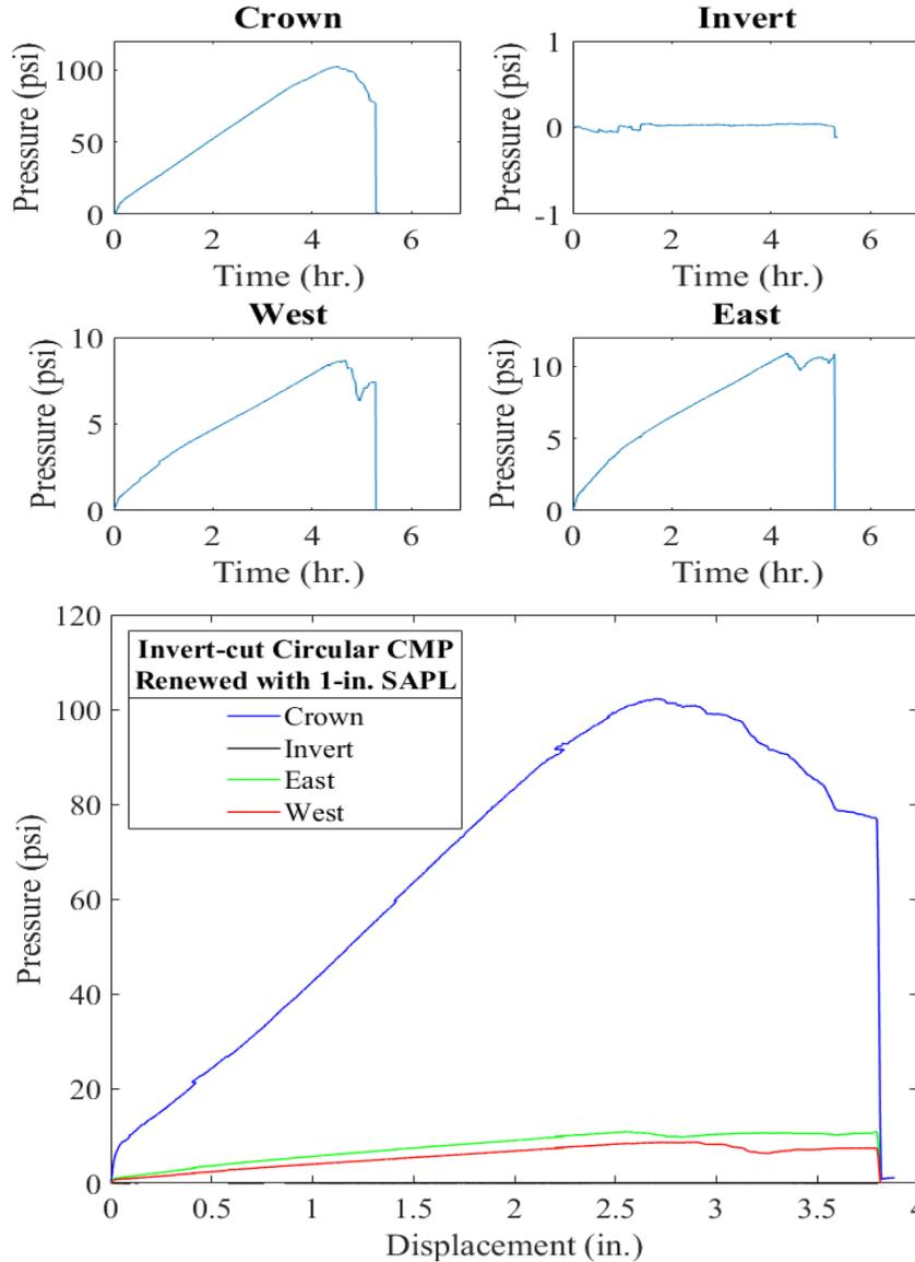
Figure 11-129. Earth pressure cell results for the 1-in. thick SAPL renewed invert-cut circular CMP with respect to: (top) time, and (bottom) crown displacement.
