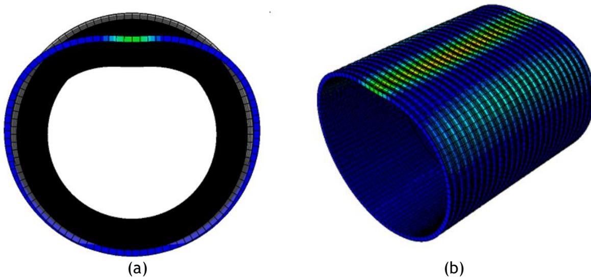
Figure 10F-3. (a) Deformation of 1-in. thick cementitious liner under ultimate load and (b) crack location in 1-in. thick cementitious liner.
