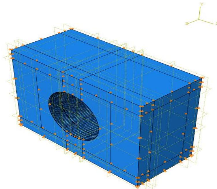
Figure 10-1. FE model of the soil-pipe-liner system.
