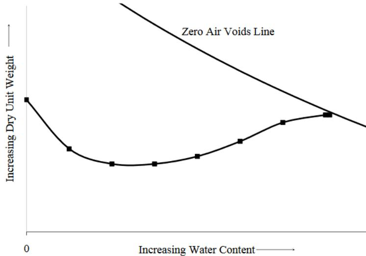
Figure 11-12. Compaction Curve for a Granular Soil (Drnevich, Evans, & Prochaska, July 2007).
