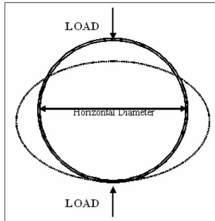
Figure 2-7. Deflection of a circular flexible pipe (Najafi 2008).
