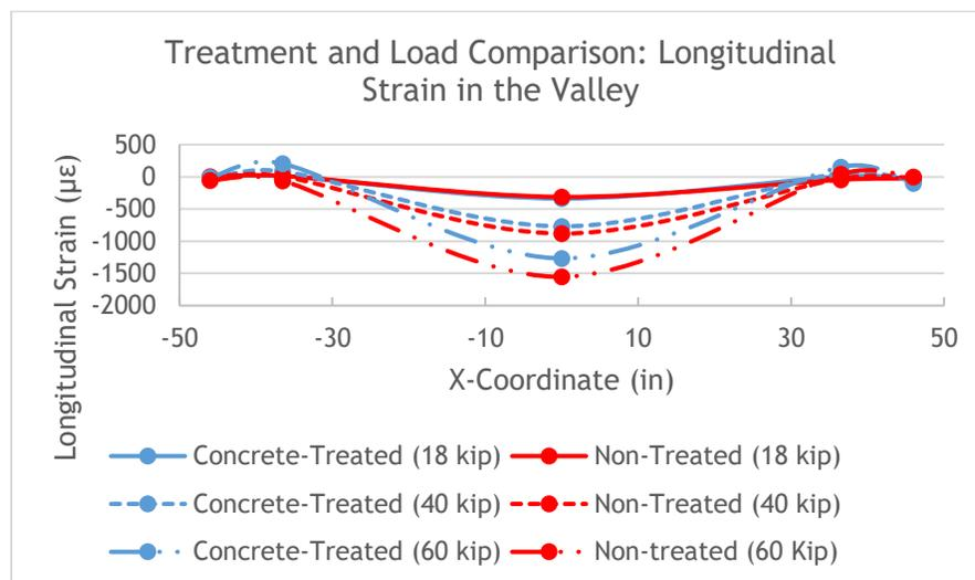
Figure 2-30. Comparison of longitudinal strain at valley of corrugation before and after paving (Sargand et al. 2015).
