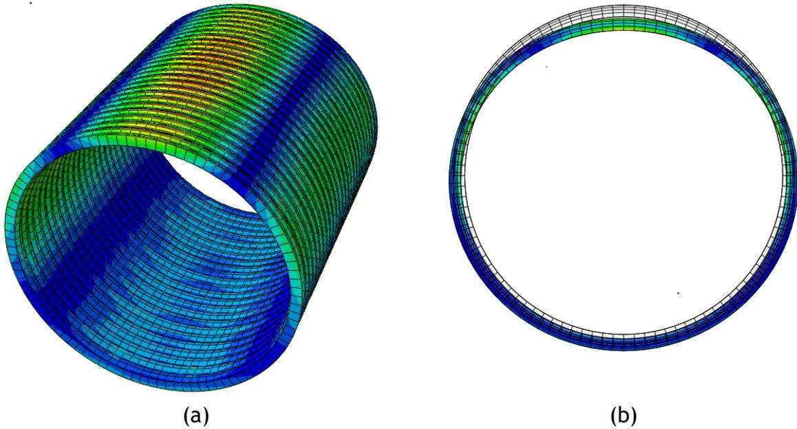
Figure 10B- 13. (a) Development of plastic strain, and (b) Deformation pattern for 2-in. thick polymeric circular liner.
