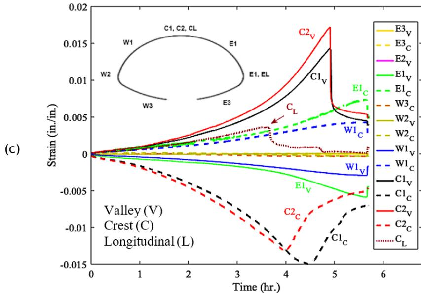
Figure 11-54. Results of strain gauges for the CMP control test: (a) intact circular CMP, (b) invert-cut circular CMP, and (c) invert-cut arch CMP.
