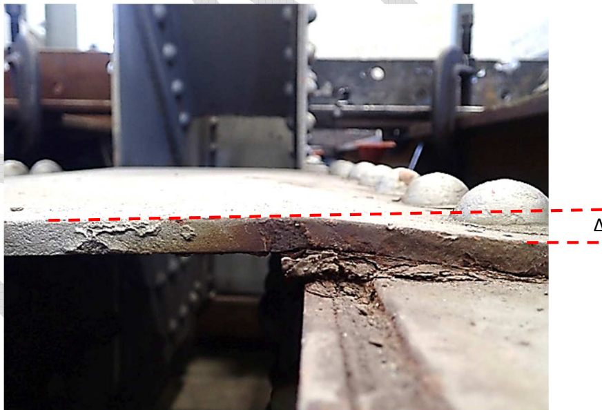
Figure 3.31 Specimen 6 end stay plate prior to testing showing pack rust-induced bending of the stay plate
