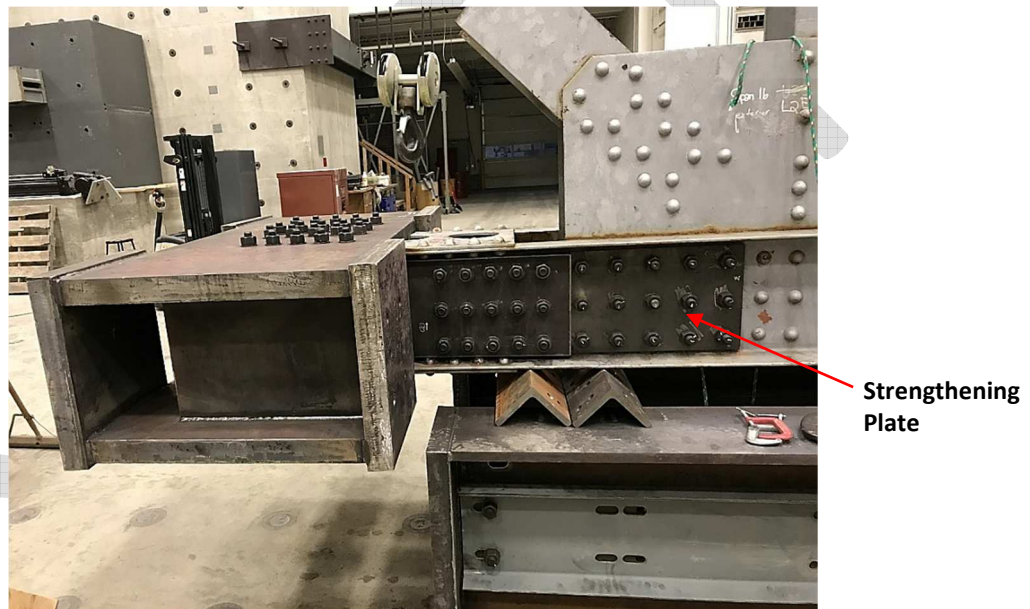
Figure 3.23. Connection at the reaction end of the specimen showing the additional plate
