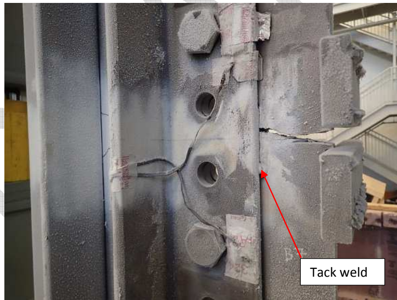
Figure 3.14 Fractured tack weld and center plate
