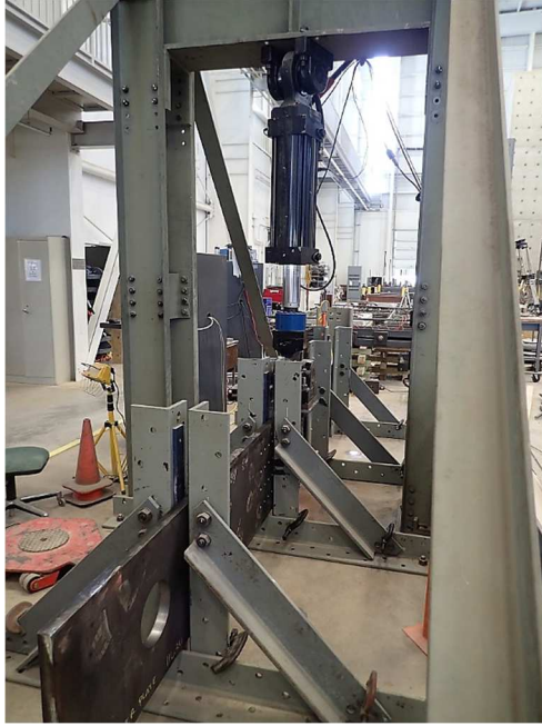
Figure 3.4 Fatigue station setup
