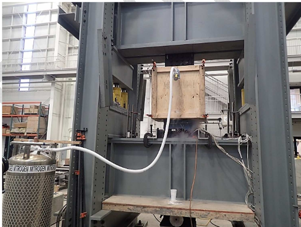
Figure 3.7 Cooling chamber used to reduce specimen toughness
