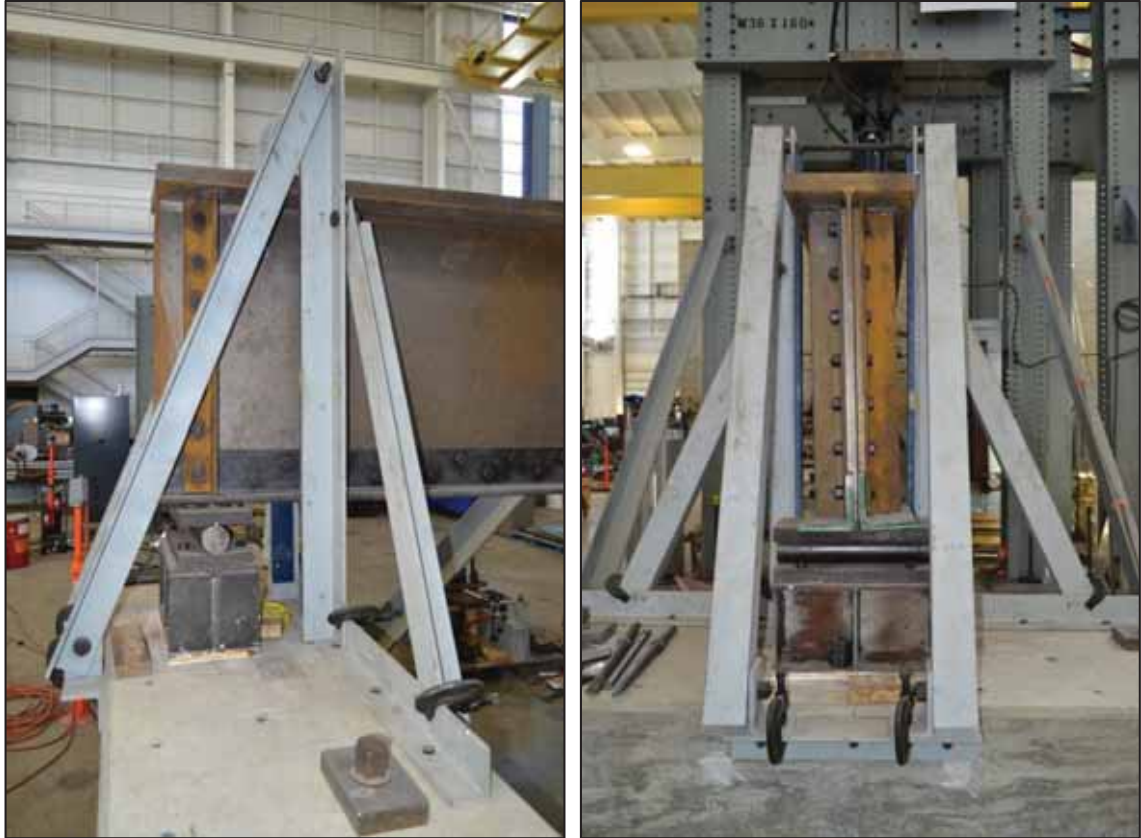
Figure 3-4 Lateral torsional bracing at specimen ends
