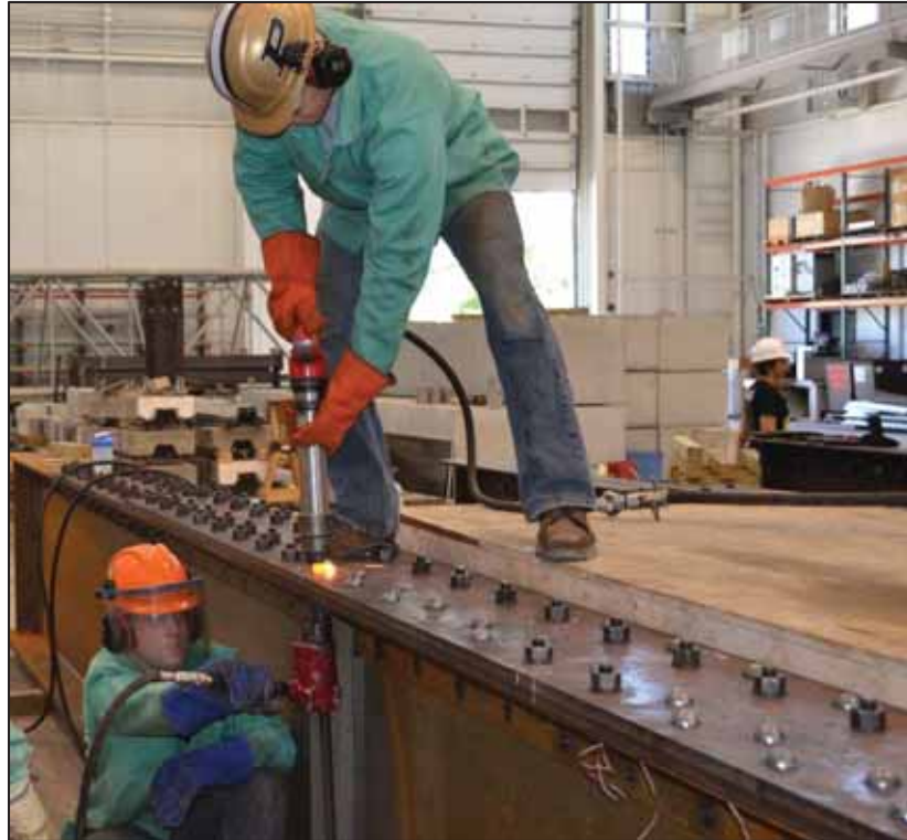
Figure 3-59 Specimen 36-3 fabrication: riveting cover plates
