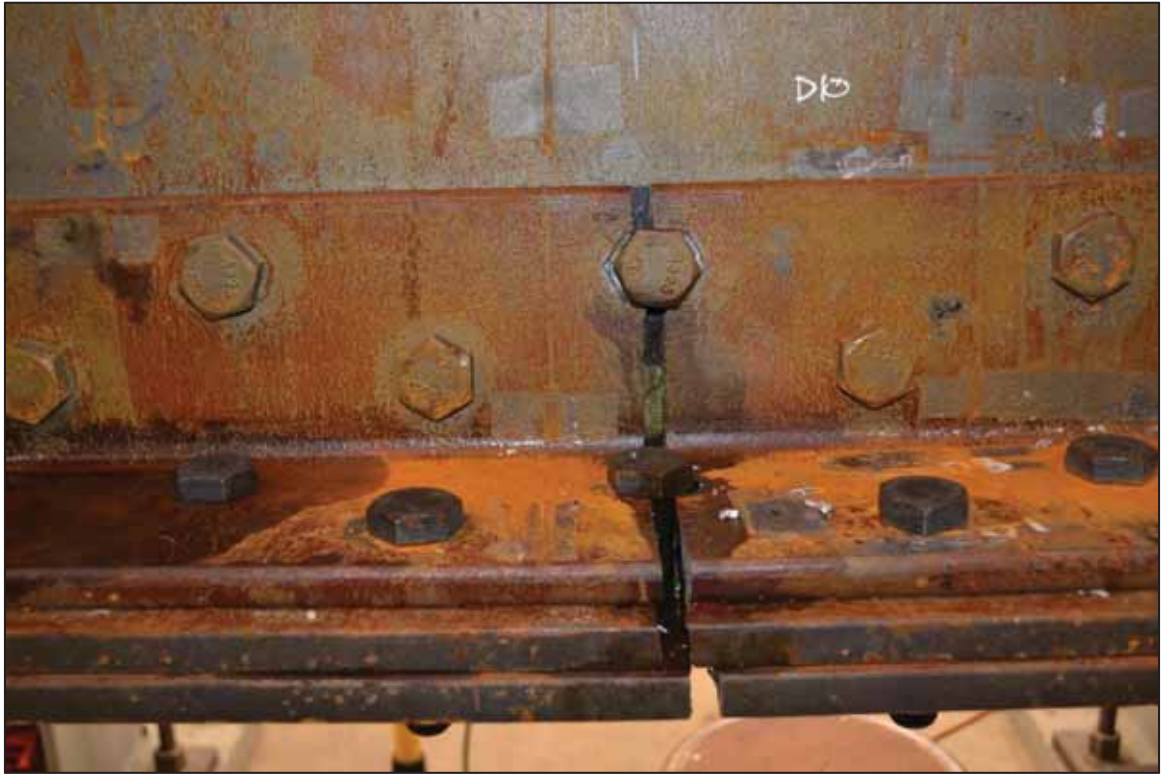
Figure 3-49 Specimen 36-1 fractured bottom flange components (east side)
