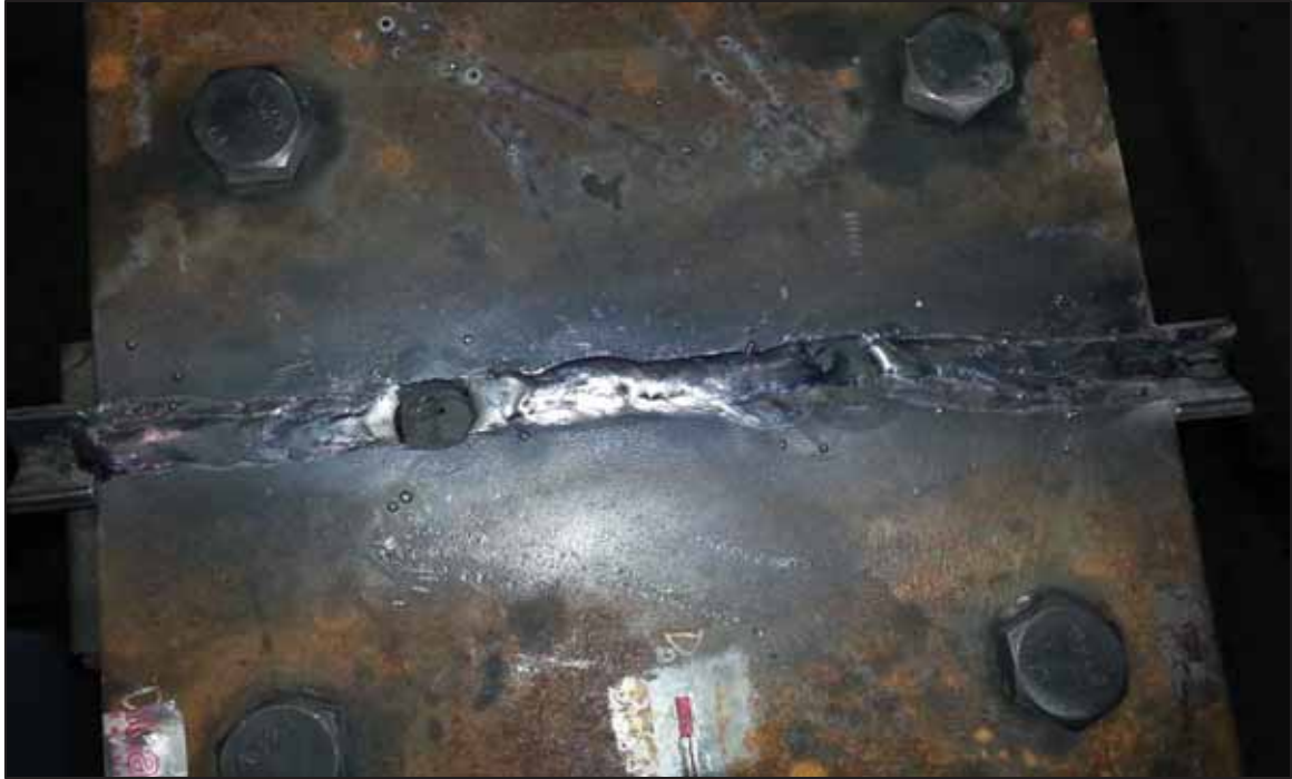
Figure 3-51 Specimen 36-2 welded lower cover plate
