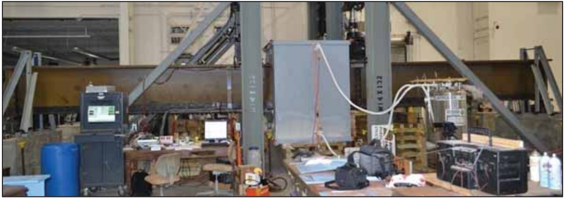
Figure 3-21 Temperature chamber installed on beam (side view)
