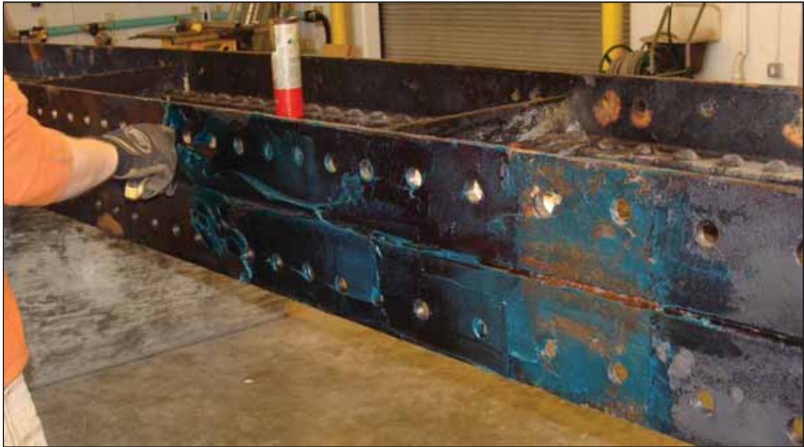
Figure 3-29 Specimen 23-1 application of grease between components
