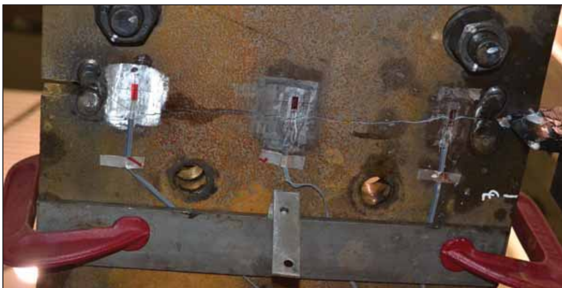
Figure 3-58 Specimen 46-4 fractured cover plate
