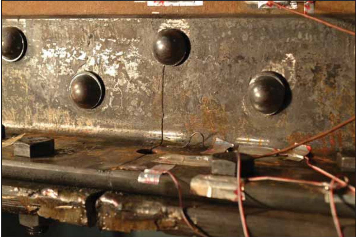
Figure 3-69 Specimen 30-1 fractured west flange angle
