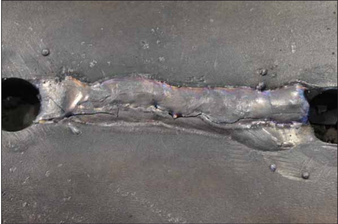
Figure 3-52 Specimen 36-2 cracks in lower cover plate weld
