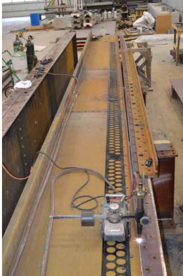
Figure 3-66 Specimen 30-1 web plate fabrication
