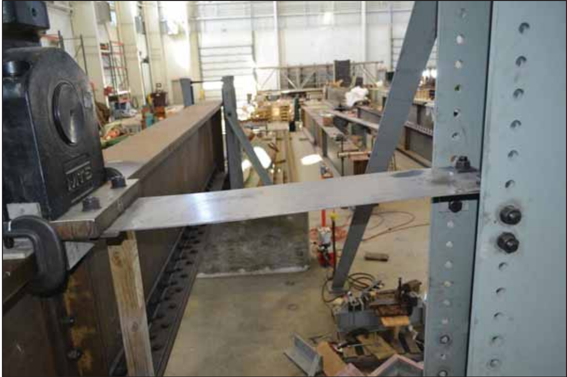
Figure 3-6 Lateral torsional buckling bracing (thin plate method)
