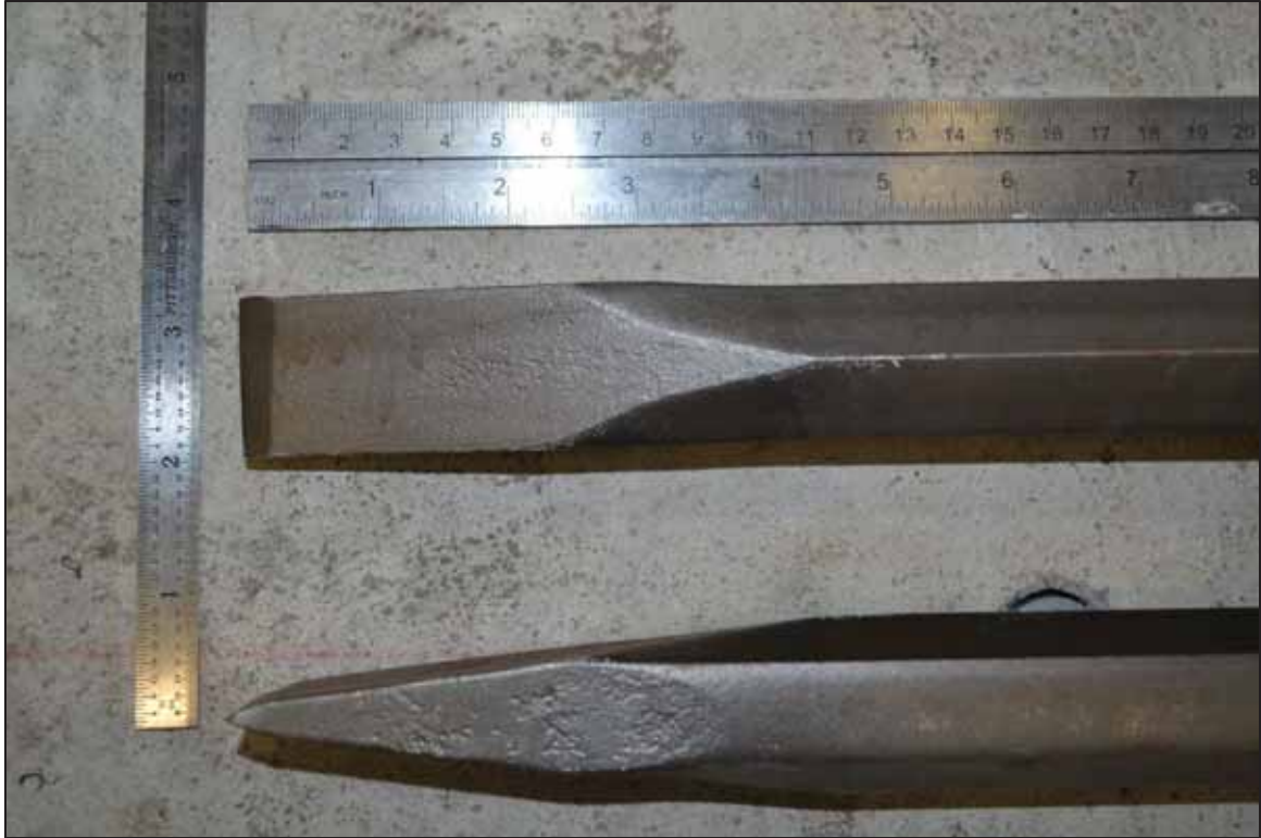
Figure 3-27 Wedge geometry
