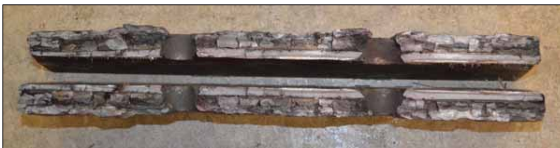
Figure 3-53 Specimen 36-2 lower cover plate failure surfaces
