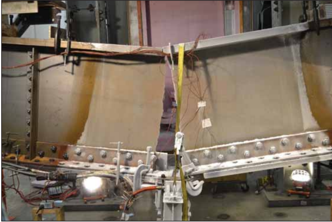
Figure 3-71 Fractured Specimen 36-5
