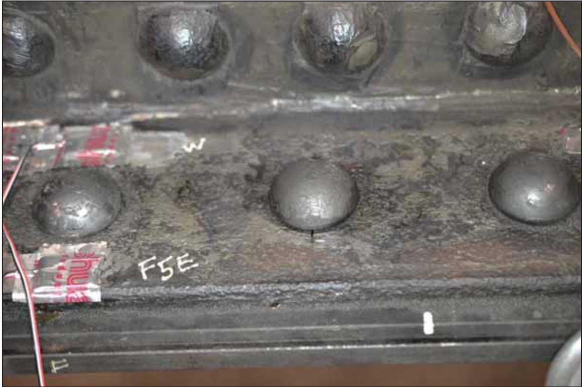
Figure 3-37 Crack growth from Specimen 23-3 hole notch
