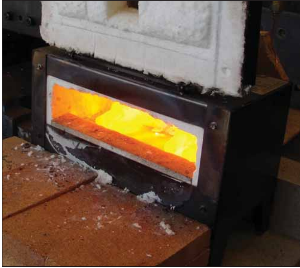
Figure 3-9 Propane fueled rivet forge
