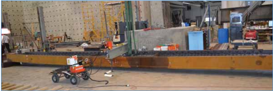
Figure 3-61 Specimen 36-4 cold worked top flange
