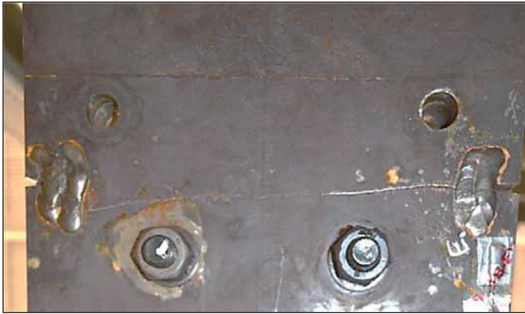
Figure 3-60 Specimen 36-3 fractured lower cover plate
