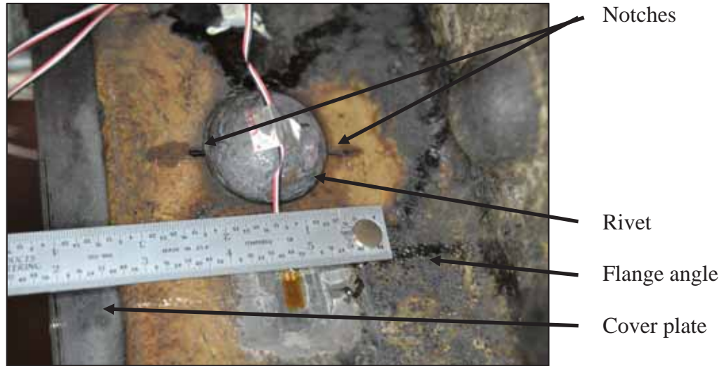
Figure 3-33 Specimen 23-2 hole notches
