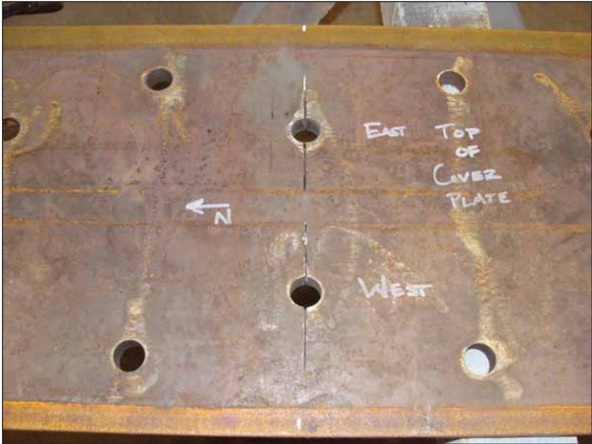
Figure 3-39 Specimen 46-1 cover plate hole notches
