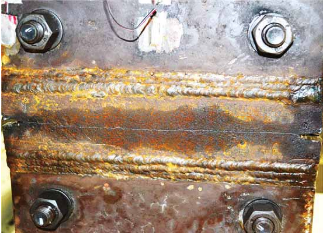
Figure 3-67 Specimen 30-1 fractured cover plate
