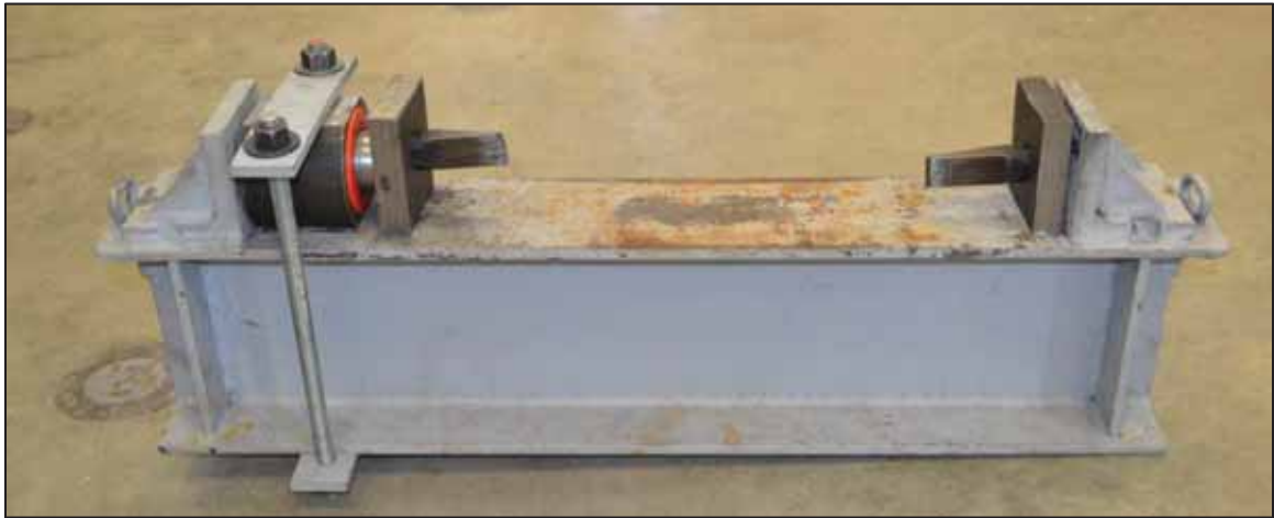
Figure 3-25 Driven wedge apparatus
