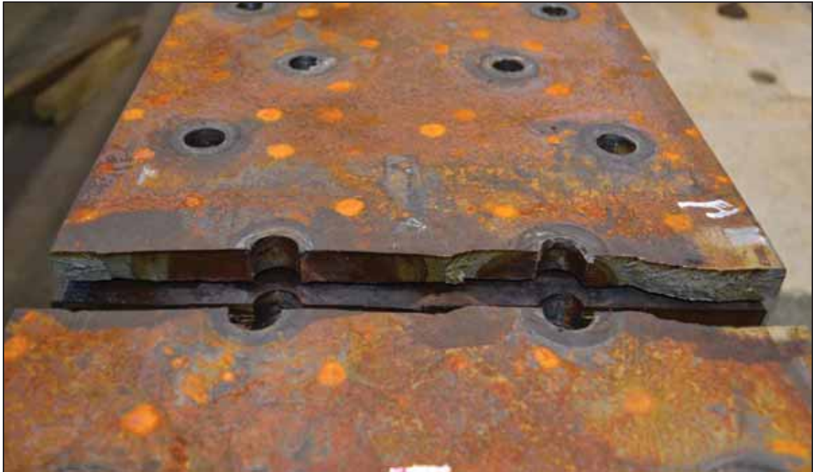
Figure 3-50 Specimen 36-1 fractured bottom flange components (bottom view)
