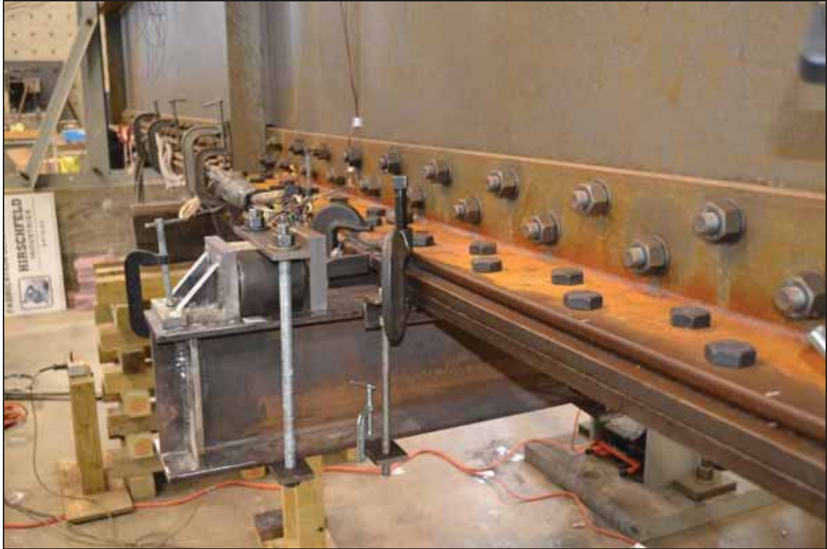
Figure 3-26 Driven wedge apparatus installed on Specimen 36-2
