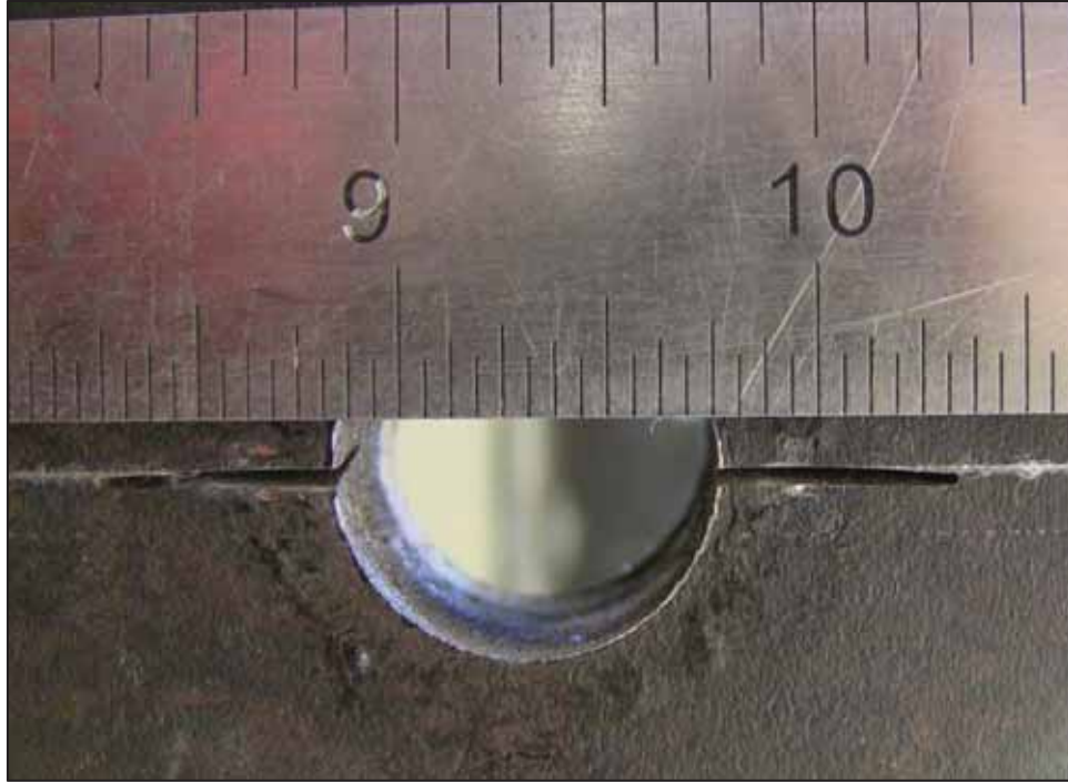
Figure 3-12 Typical hole notch with Dremel 409 cutting wheel
