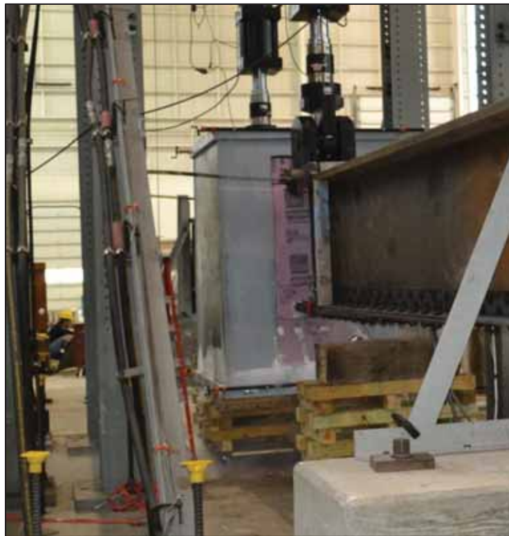
Figure 3-22 Temperature chamber installed on beam (end view)
