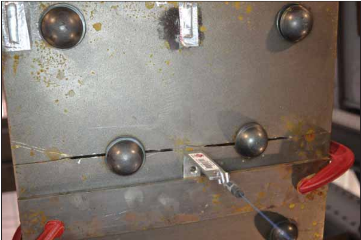
Figure 3-45 Specimen 46-3 fractured cover plate (from below)
