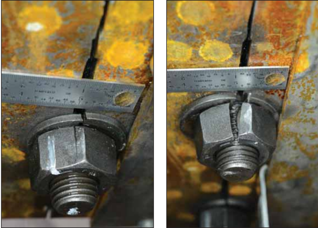
Figure 3-41 Specimen 46-1 cracked nuts
