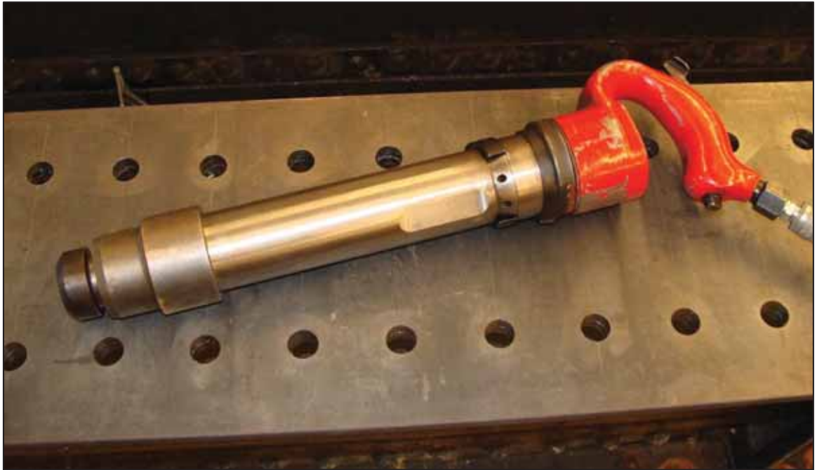
Figure 3-7 Chicago Pneumatic CP-80RB Rivet Buster
