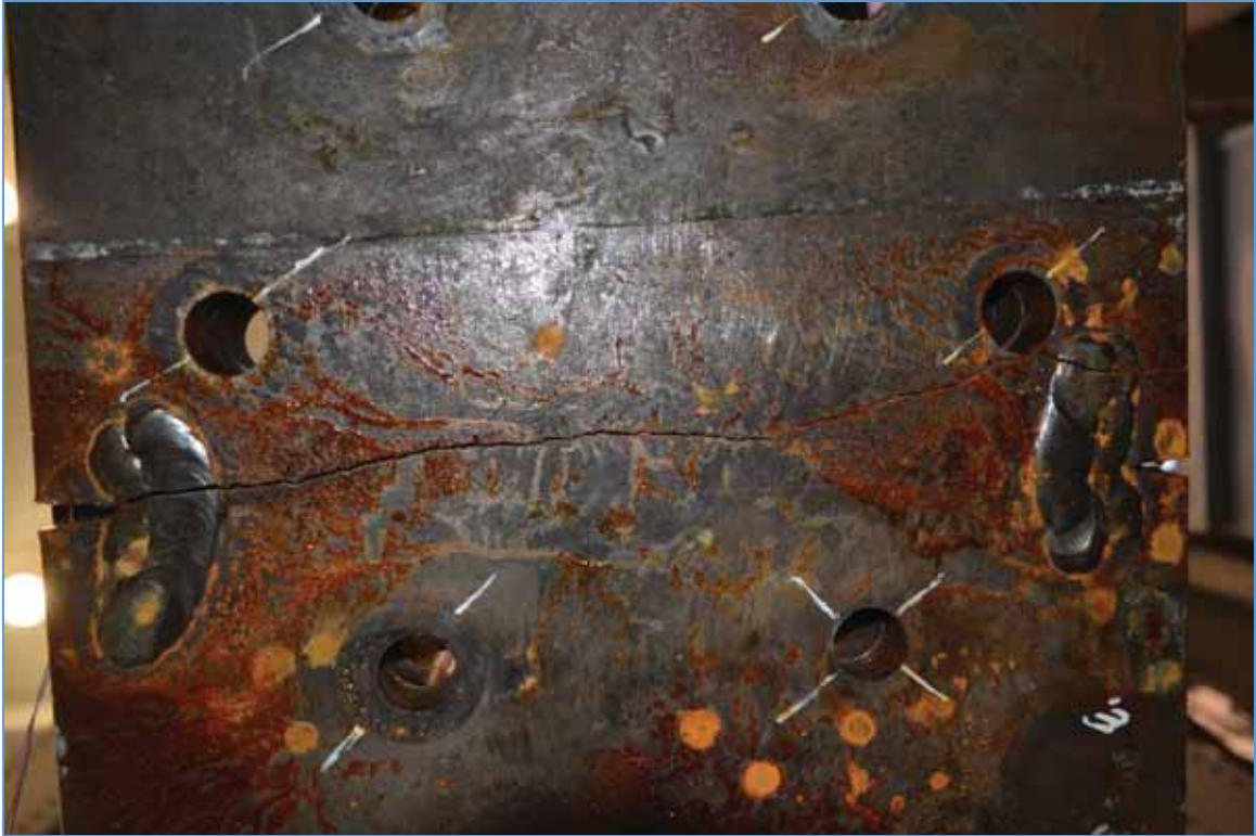
Figure 3-62 Specimen 36-4 fractured cover plate
