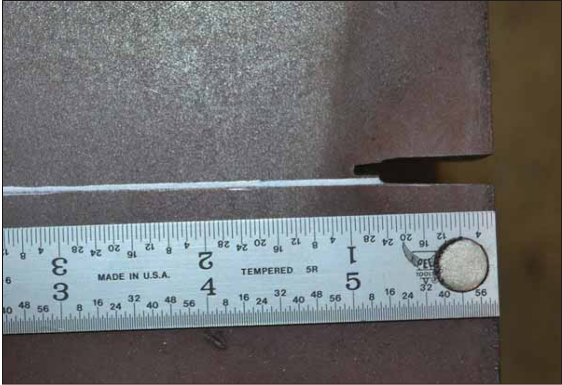
Figure 3-13 Typical edge notch geometry
