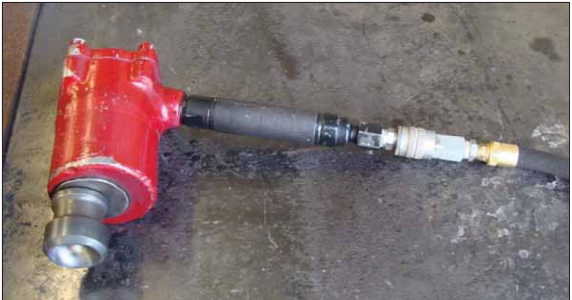
Figure 3-8 Chicago Pneumatic CP-AA-Offset holder-on
