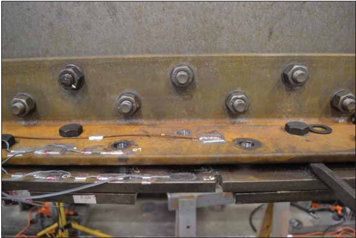
Figure 3-54 Specimen 36-2 notched upper cover plate
