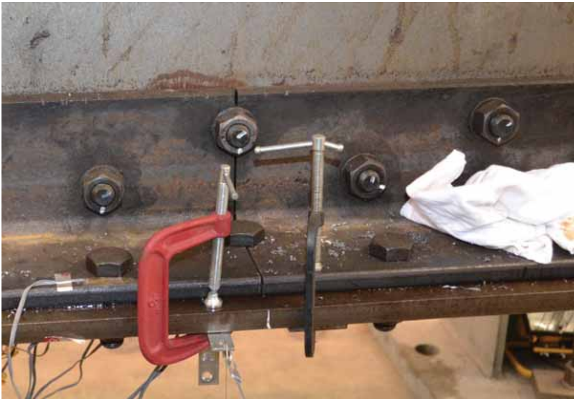
Figure 3-63 Specimen 46-5 severed flange angle
