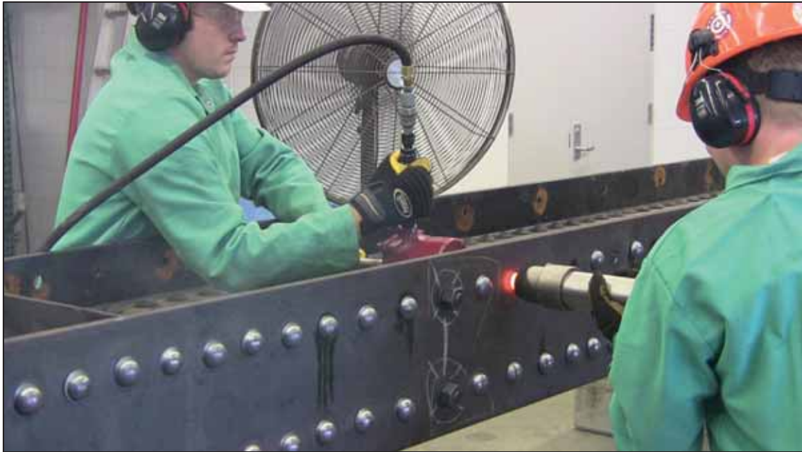
Figure 3-16 Cover plate installation on historical specimens
