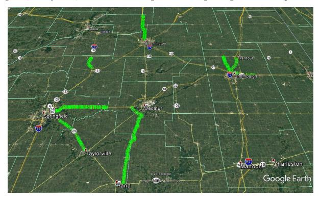
Figure 6. Color-coded estimated structural condition of tested roads in 2015 with Good (green), Fair (yellow), and Poor (red) ratings (© 2016 Google Image Landsat / Copernicus).
