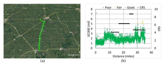
Figure 18. Identified Strong (green) and Weak (red) sections on US51S based on thresholds obtained from Table 2: (a) Google Earth plot (© 2016 Google Image Landsat / Copernicus); (b) scatter plot
