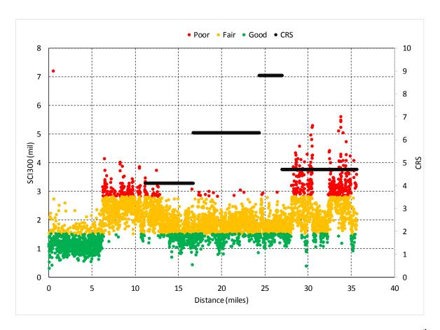
Figure 19 Classification of structural condition on US51S south based on percentile: 25<sup>th</sup> percentile and lower represents good structural condition and 90<sup>th</sup> percentile and higher represents poor structural condition
