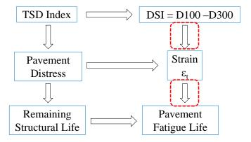
Figure 21. Link between DSI and estimated pavement fatigue life.
