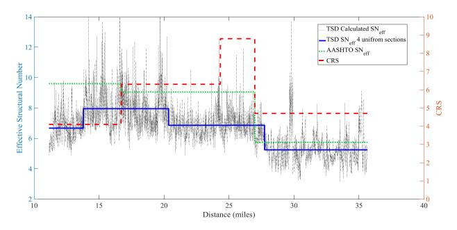
Figure 13. Calculated SNeff on US51 South with measurements collected in 2015 (https://goo.gl/maps/kNaJGaddG5w).
