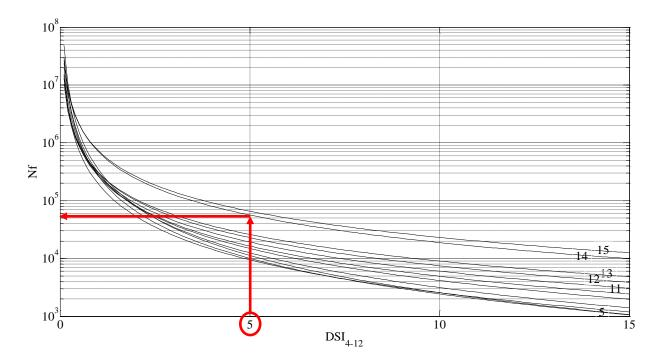
Figure 22. Fatigue life curves for TSD DSI (Number on the curves represent AC layer thickness).
