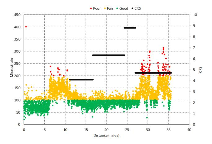
Figure 20. Estimated tensile strain at bottom of asphalt layer on US51S
