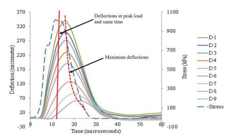
Figure 17 Example of FWD time history from LTPP section 169034 taken from Chatti et al. (2017)
