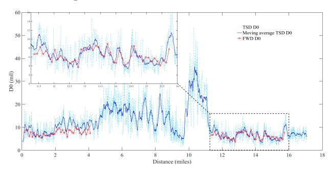
Figure 15 Comparison of TSD D0 and FWD D0 on R29 East (https://goo.gl/maps/UmevQei4yYk)
