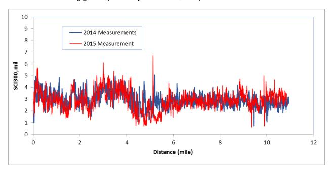
Figure 10. Temperature corrected repeated TSD tests (SCI300) on Champaign CH1
