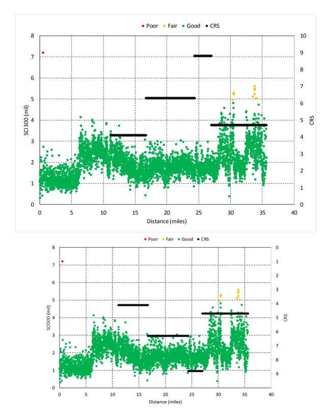
Figure 12. Comparison of TSD SCI300 measurements collected in 2015 and CRS on US51 (https://goo.gl/maps/kNaJGaddG5w).
