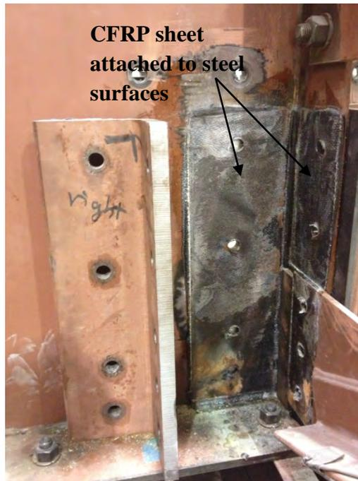
**Figure B.71: Trial 2: view of the interior face of the girder's web**
