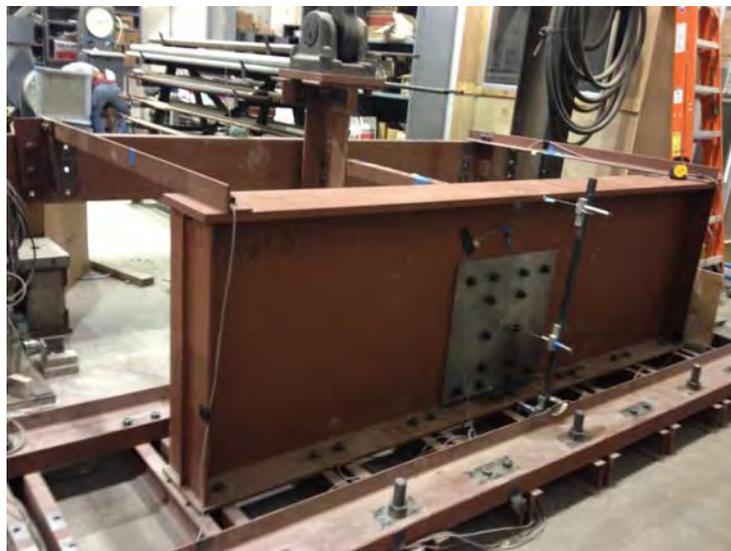
**Figure B.68: View on the exterior face of the girder's web with a steel back plate**
