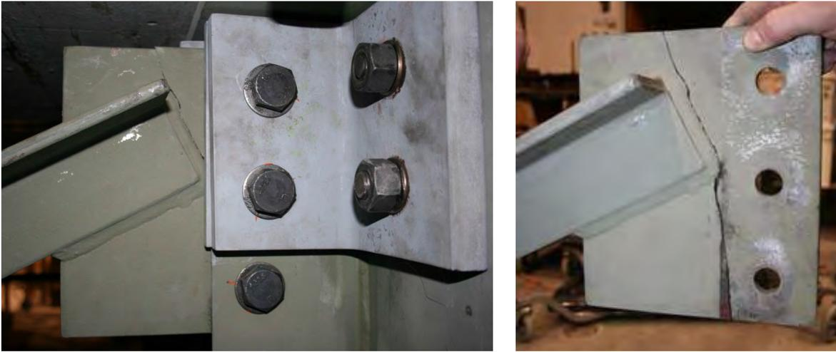
**Figure A.33: North cross frame failure during Trial 4N**
