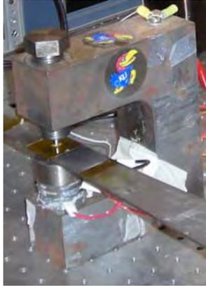
**Figure C.13: PICK tool being used to treat a steel tensile fatigue specimen**
