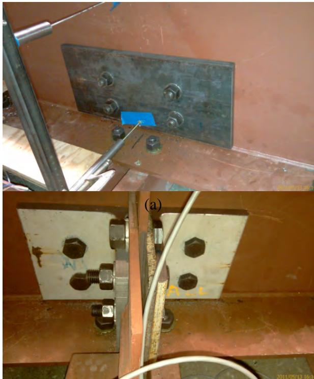
**Figure A.8: Angles-with-plate retrofit**
