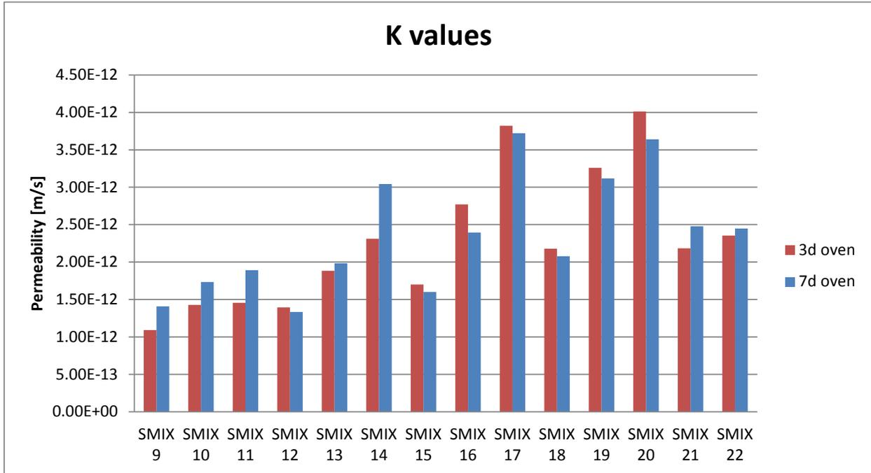
**Figure 6: Permeability – Sulfate mixtures**
