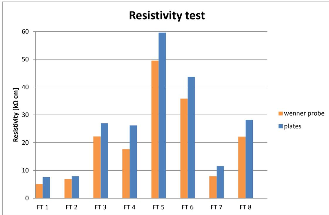
In order to compare the results of the two measurement methodologies, the conversion from resistance (measured with the two electrodes method) to resistivity has been done. Moreover, it has been taken into account a geometric correction factor assumed to be equal to  $K=1.9$ .
