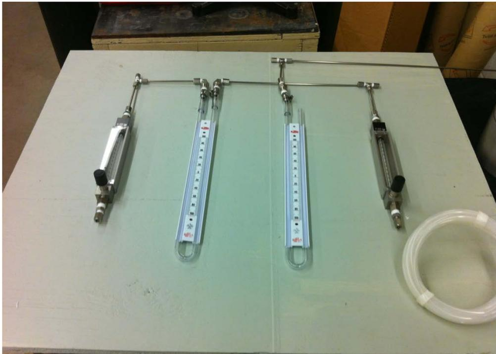
**Figure 12: Swiss Permeability instrument**
