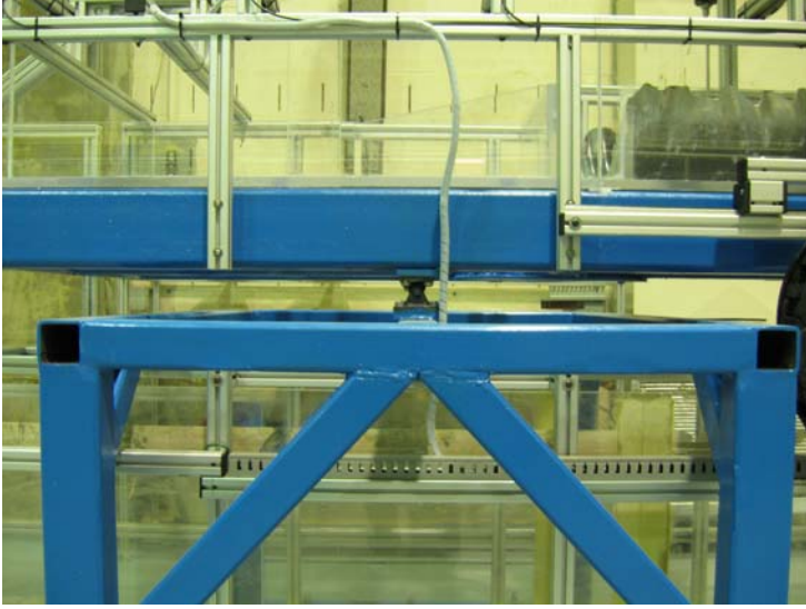
Figure 2: Pivot point of the culvert flume
