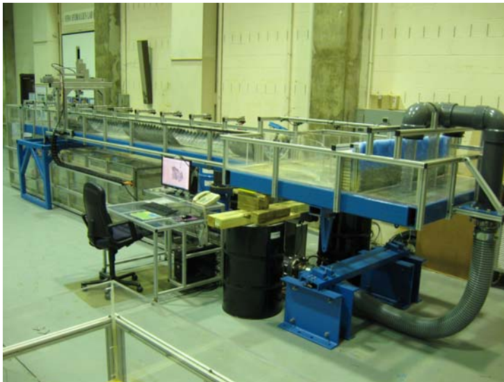
Figure 1: Ongoing construction to add a tilting mechanism to the culvert flume.
