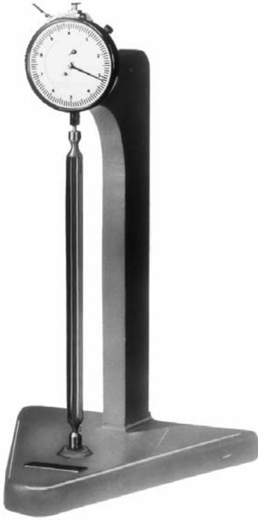
**Figure 2.3 – Mechanical Dial Gage Length Comparator**
