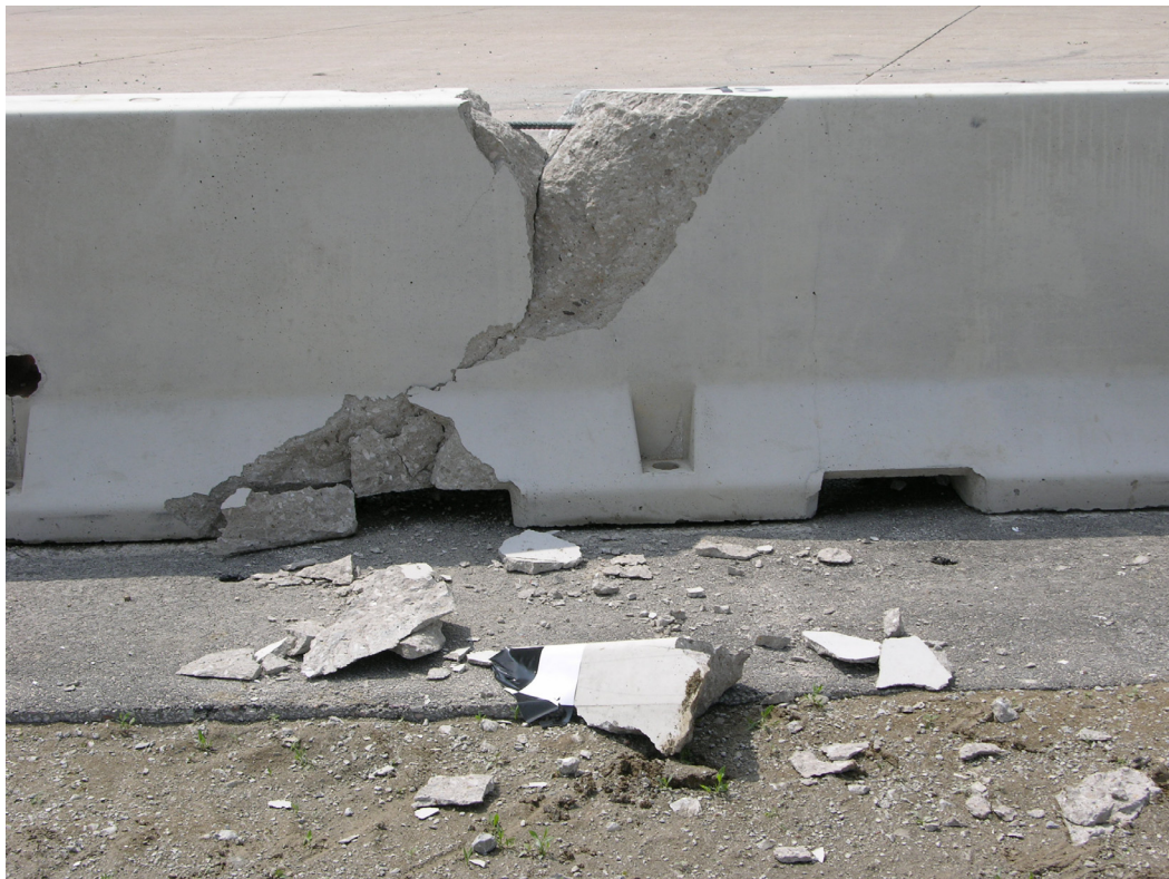
Figure 56. System Damage, Test FTB-2
