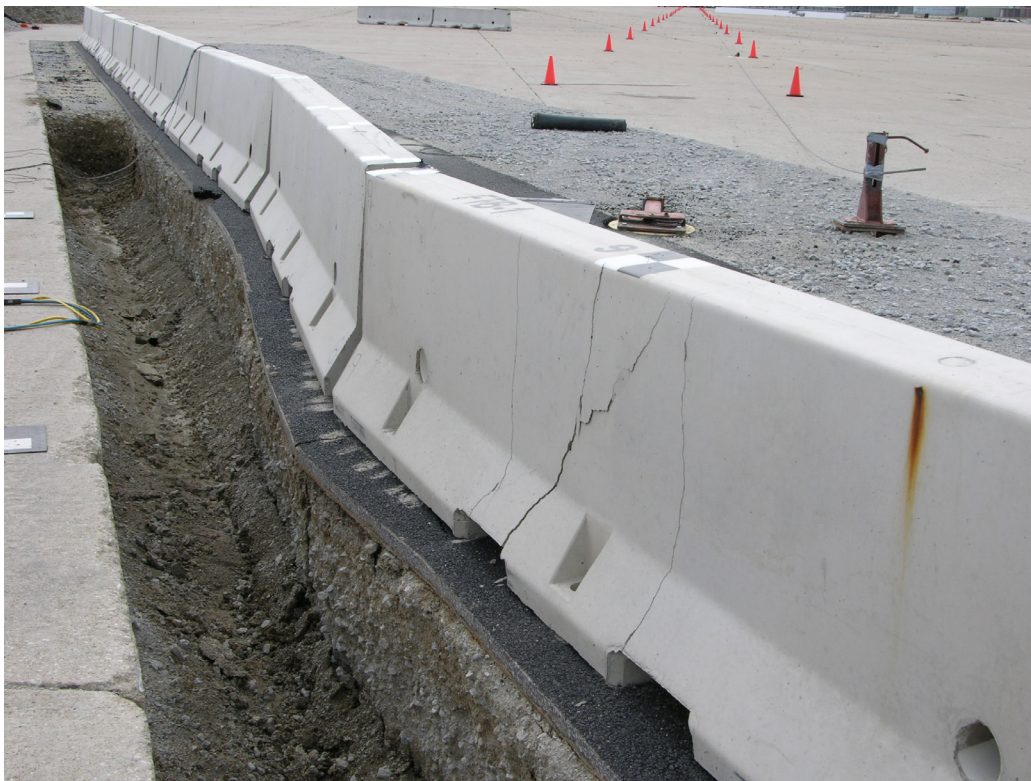
Figure 28. System Damage, Test FTB-1
