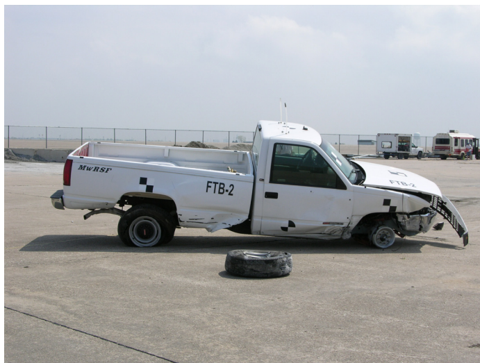
Figure 57. Vehicle Damage, Test FTB-2
