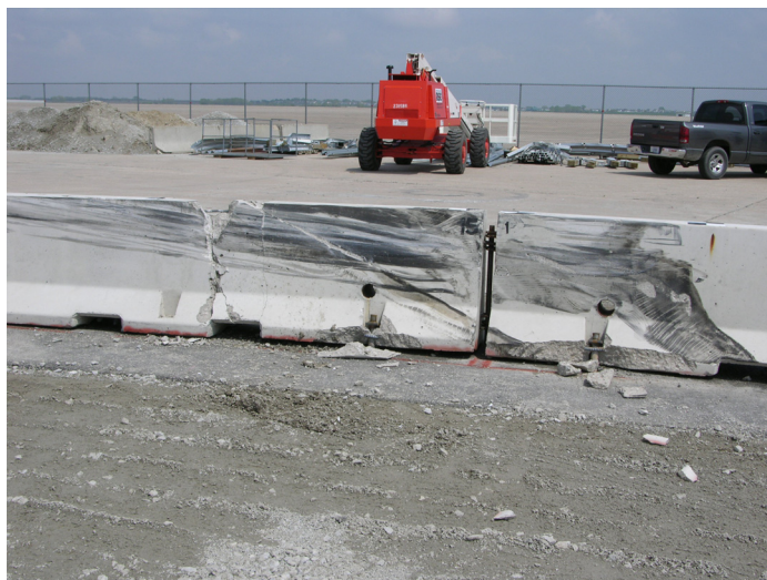
Figure 55. System Damage, Test FTB-2
