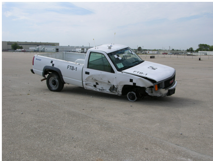
Figure 30. Vehicle Damage, Test FTB-1
