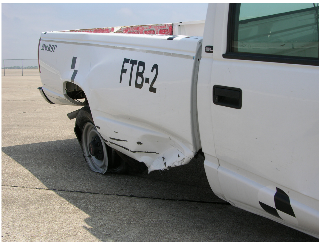
Figure 58. Vehicle Damage, Test FTB-2
