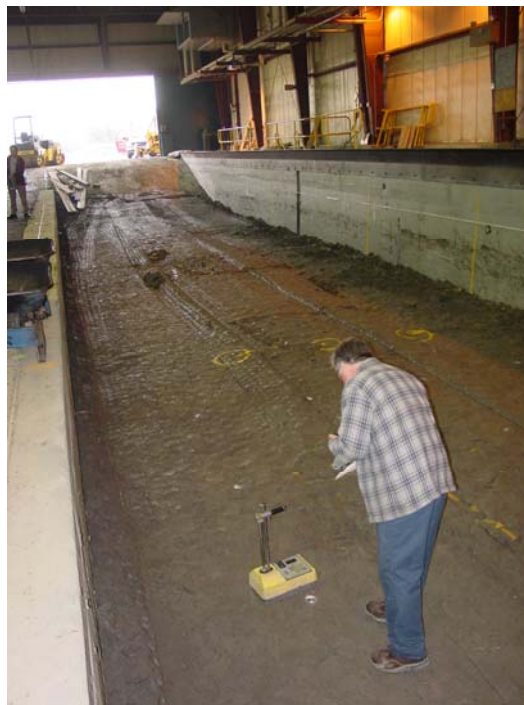
Figure 19. Nuclear moisture-density gauge measurements.
