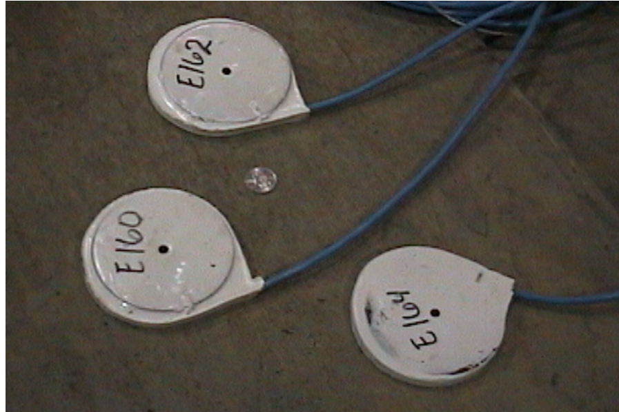
Figure 8. εmu coils to measure longitudinal and transversal deformations.
