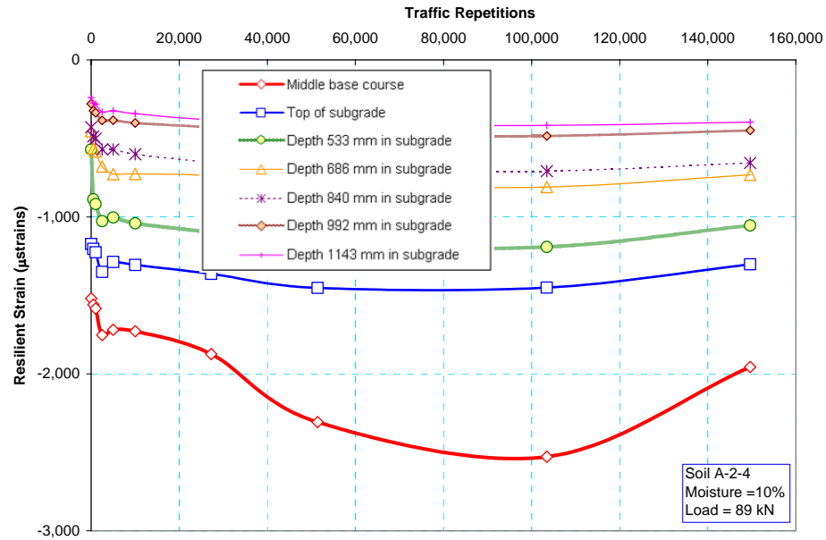
Figure 43b. Resilient strain with subgrade soil type A-2-4 at 10% moisture content and 89 kN HVS load.
