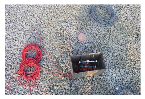
Figure 15. Installation of vibrating wire strain gage with steel box
