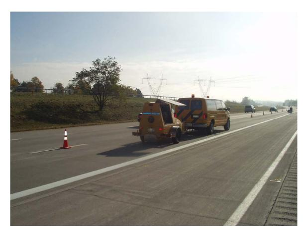
Figure 17. Falling Weight Deflectometer attached to a van
